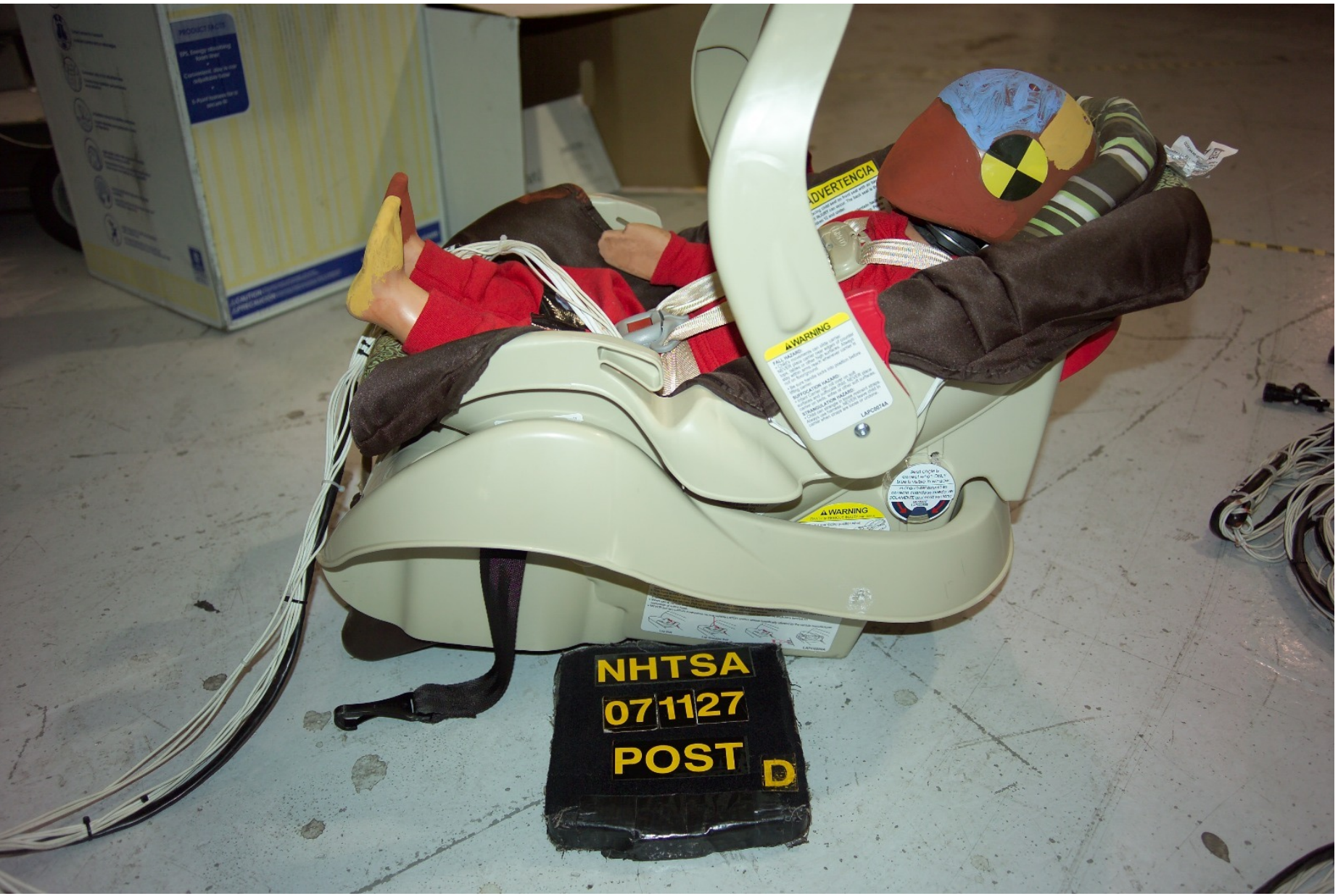
Figure D-28 Post-Test Left Side View of Right Rear CRS
