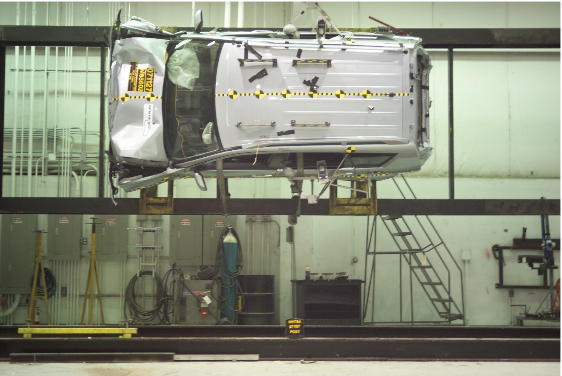
Figure A-85 EMVSS 301 Rollover View at 90°
