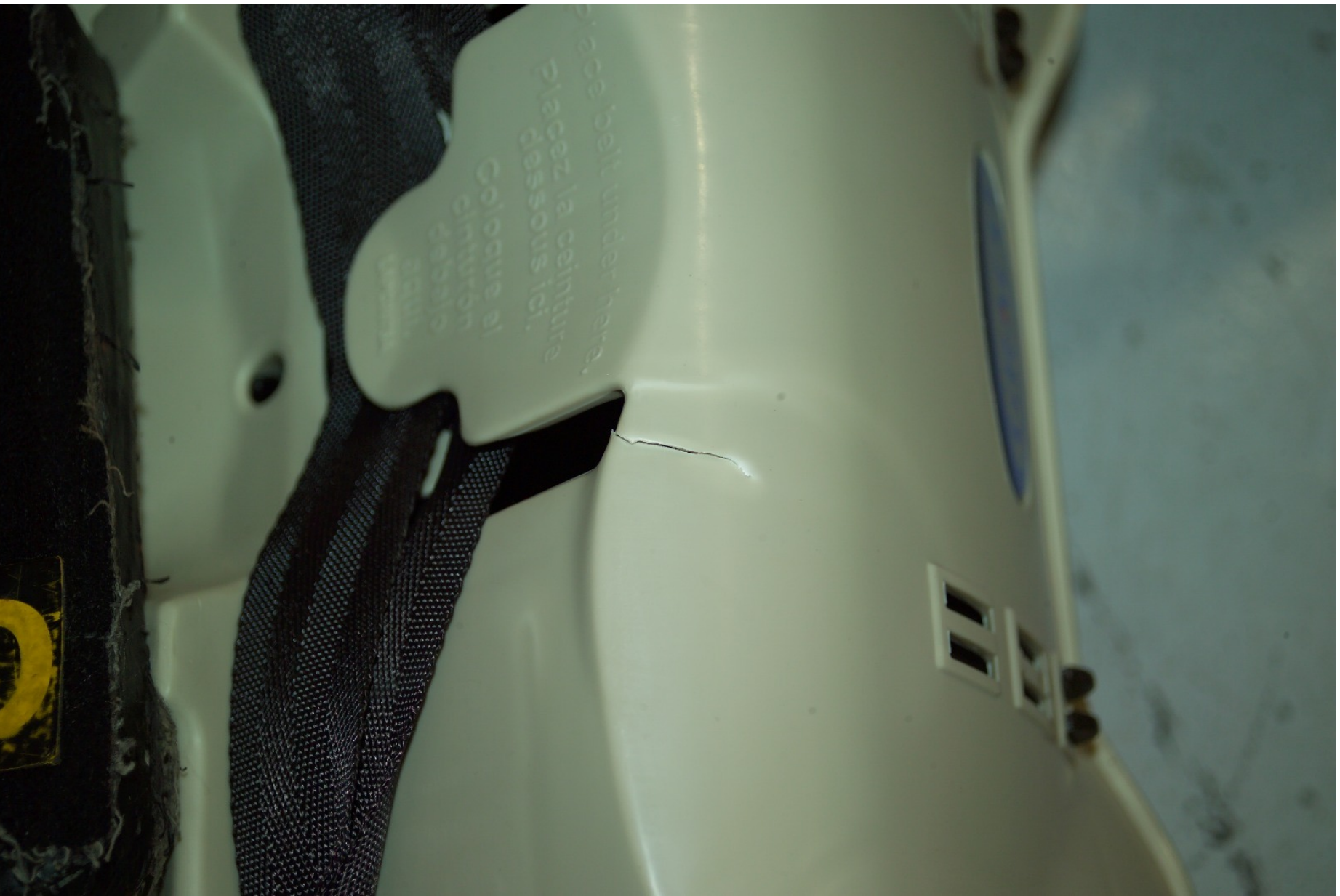
Figure D-44 Post-Test Right Rear CRS Base -View 3
