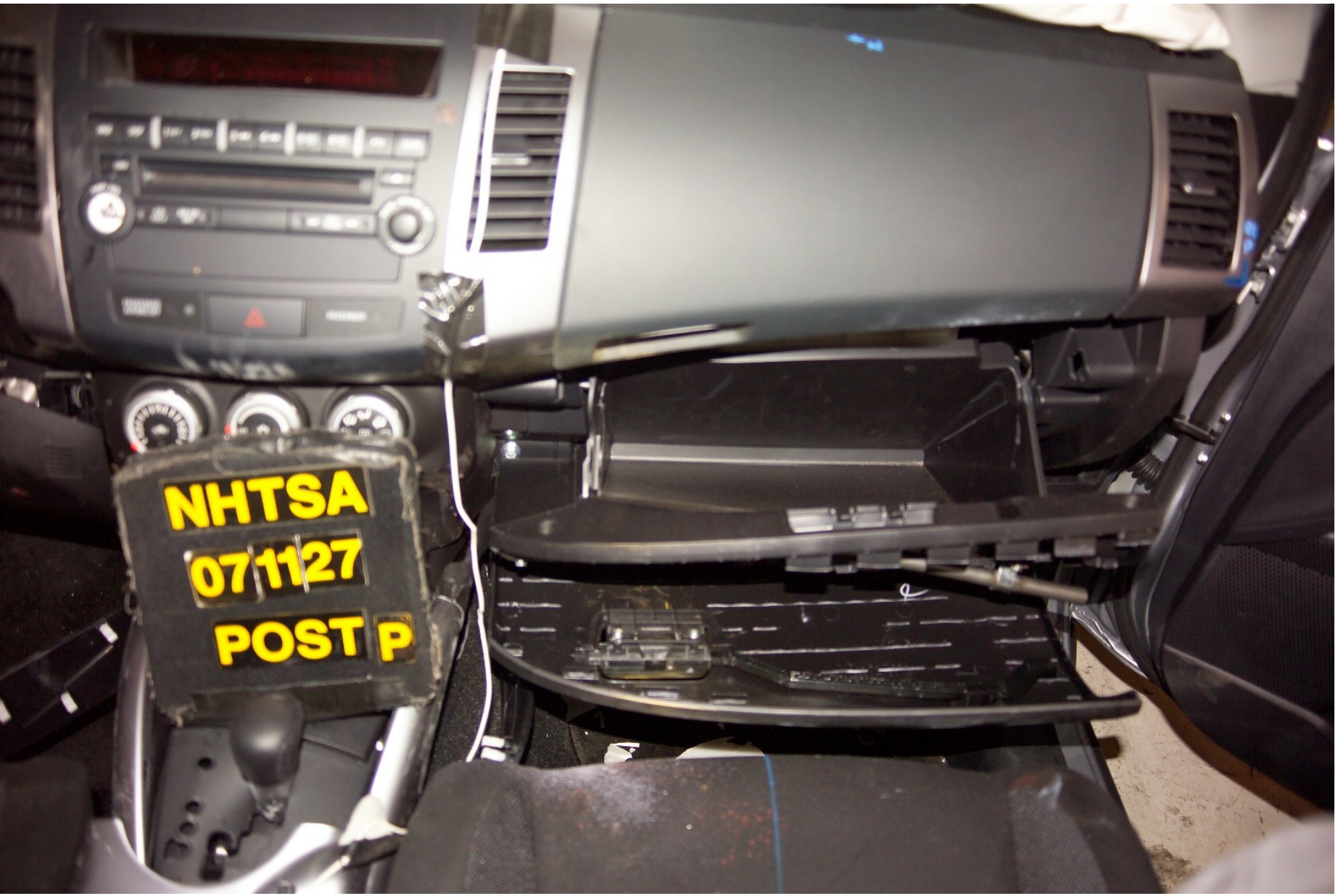
Figure A-78 Post-Test Glove Box Damage View
