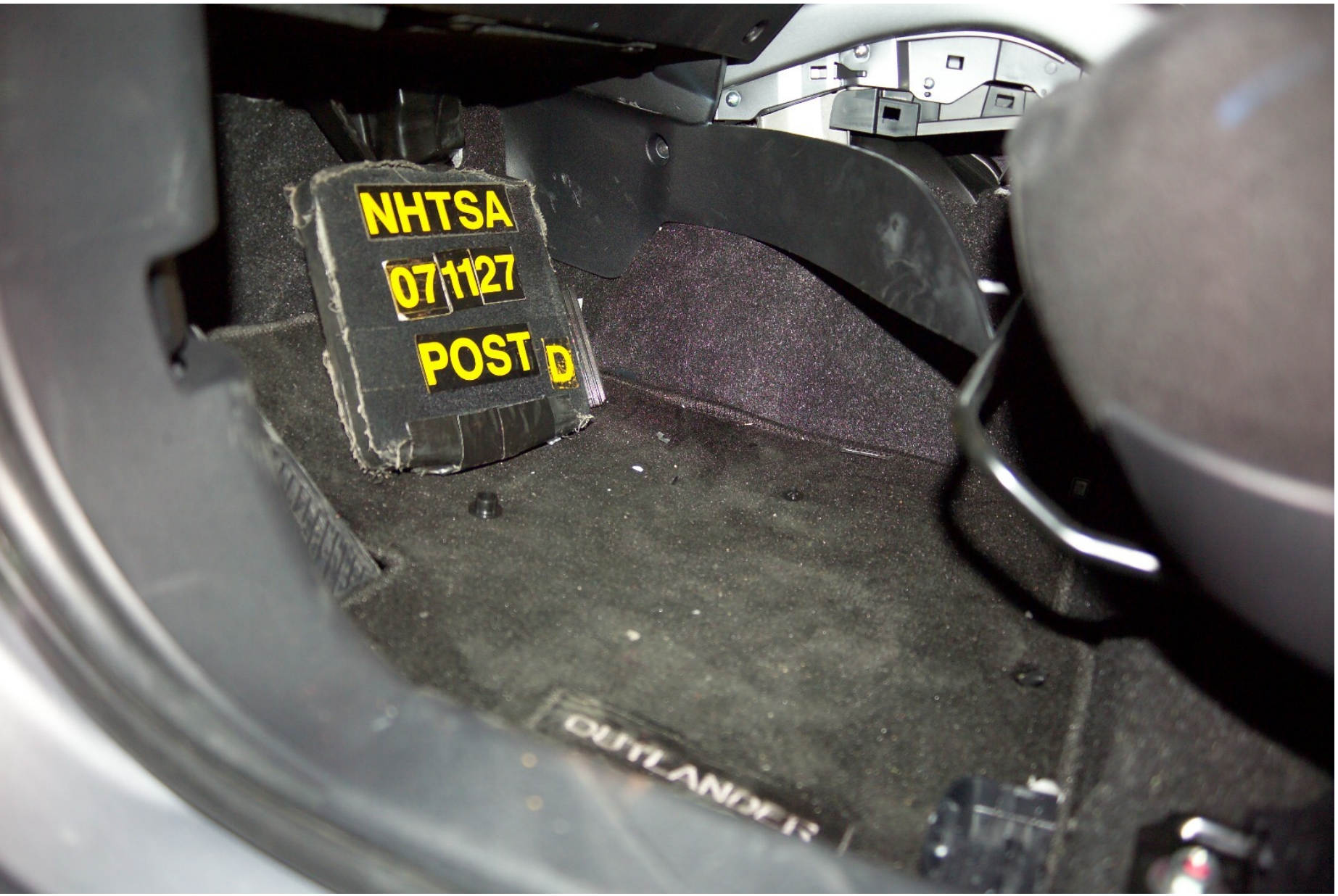
Figure A-63 Post-Test Driver Floorboard Deformation View
