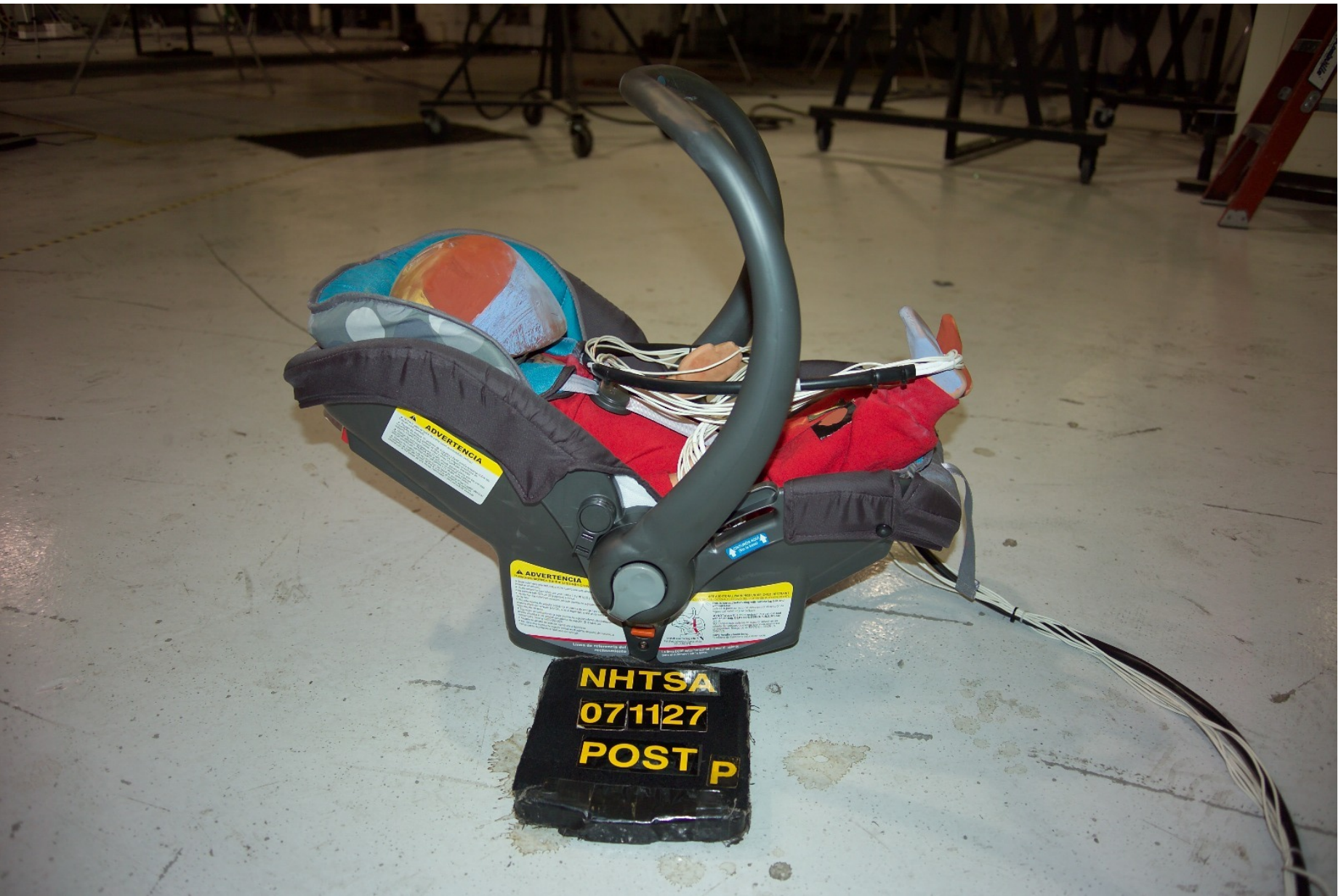
Figure D-8 Post-Test Right Side View of Left Rear CRS
