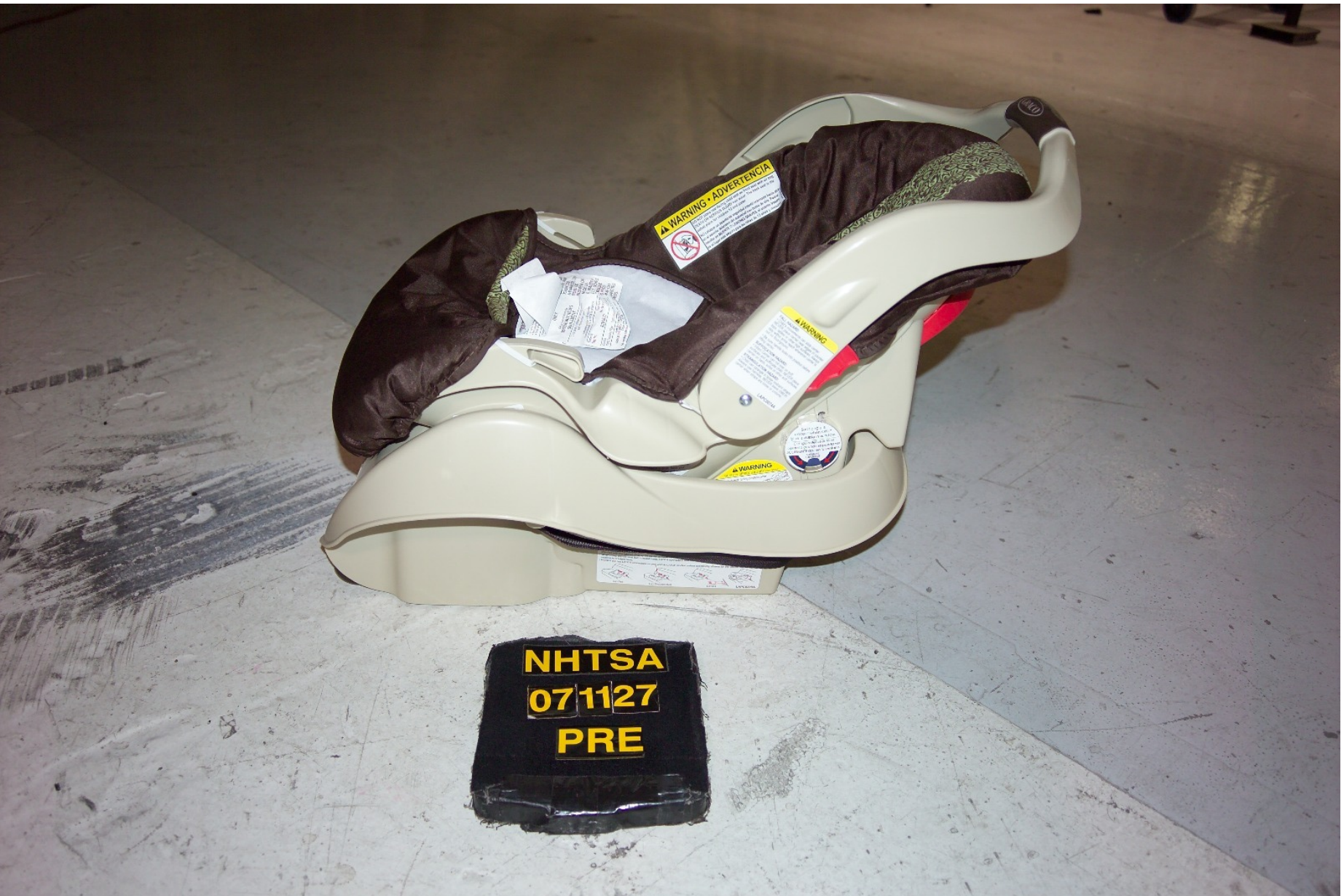
Figure D-27 Pre-Test Left Side View of Right Rear CRS
