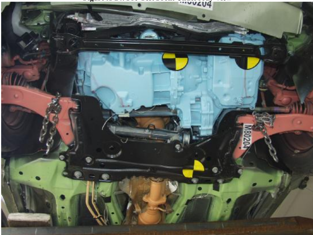
Figure A-25: Post-Test Front Underbody View
