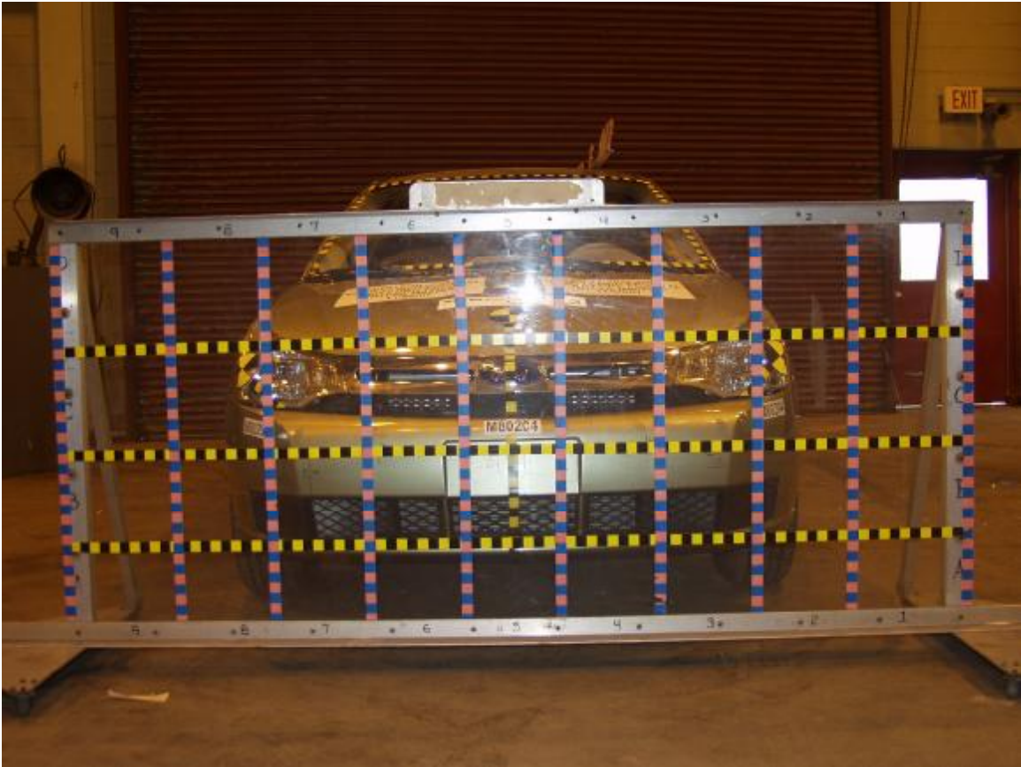
Figure A-1: Load Cell Locations
