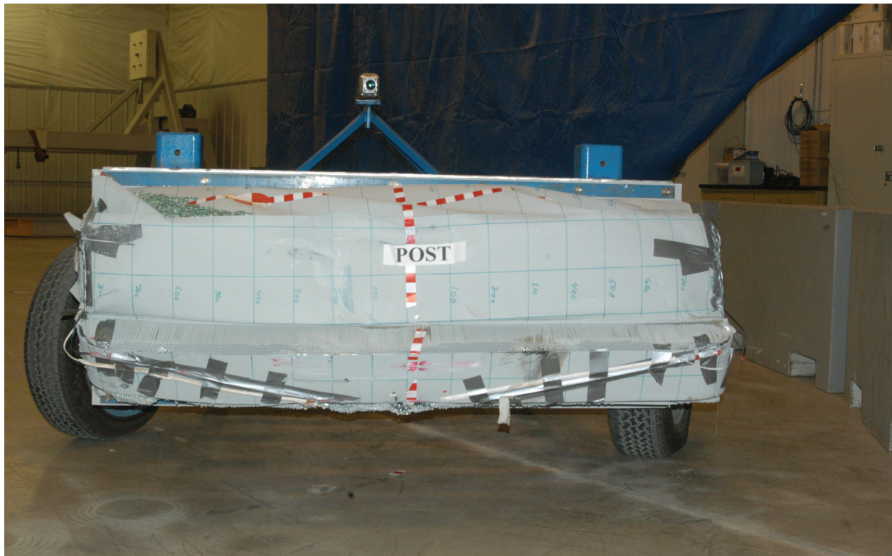
Figure A-52: Post test front view of MDB barrier face
