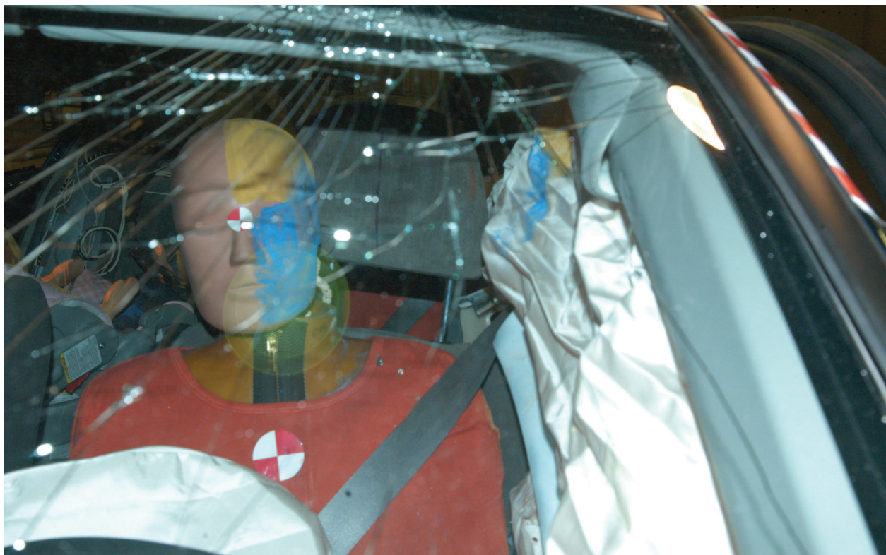
Figure A-38: Post test driver shoulder clearance
