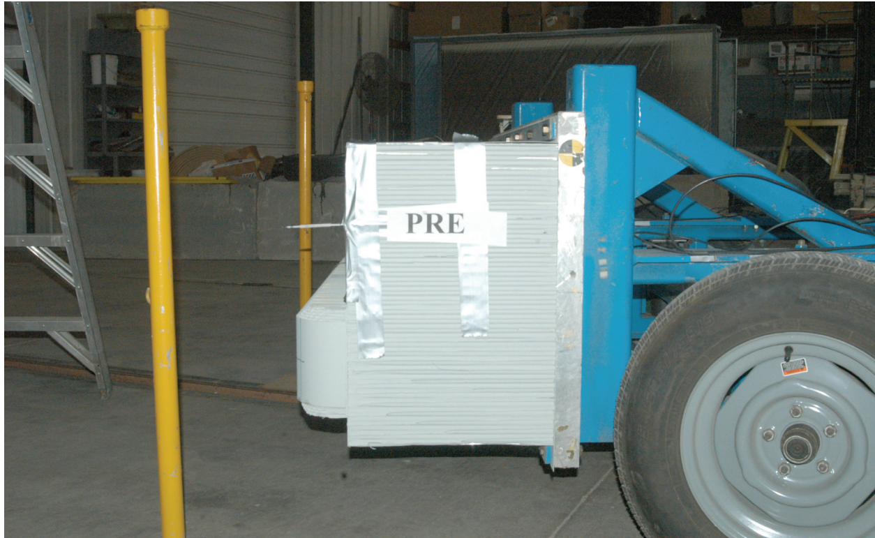
Figure A-57: Pre test left side view of MDB barrier face
