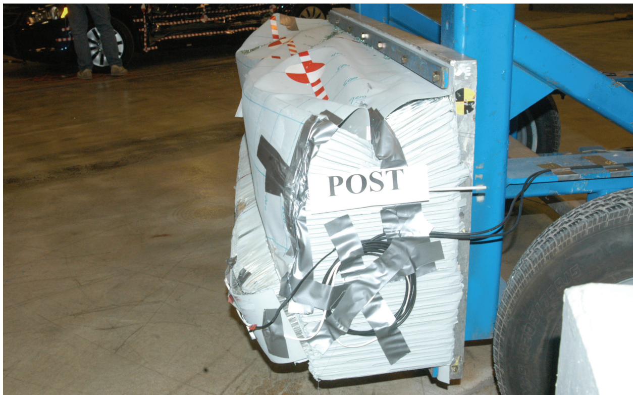
Figure A-58: Post test left side view of MDB barrier face
