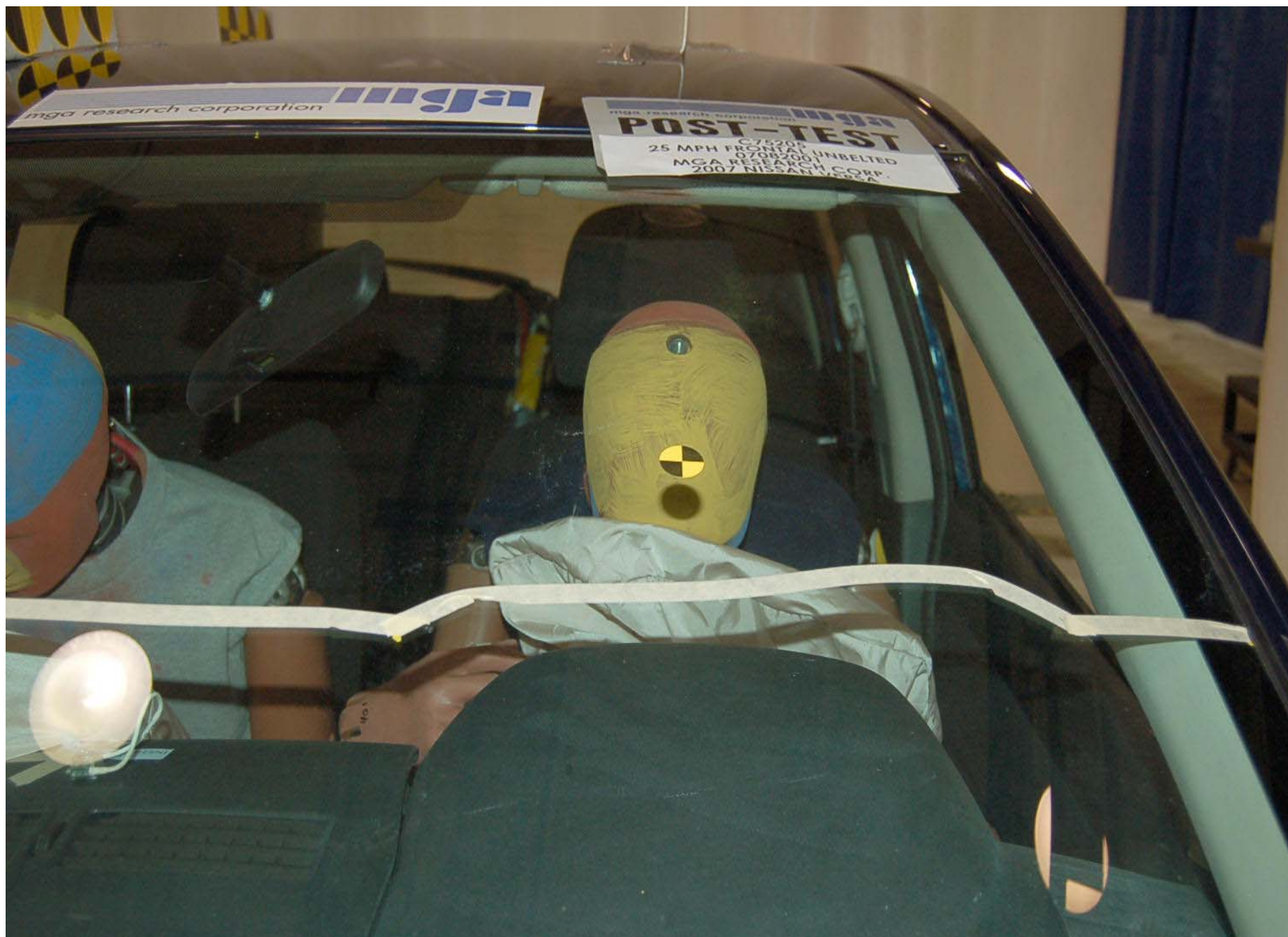
Post-Test Driver Dummy Front View (head position)
