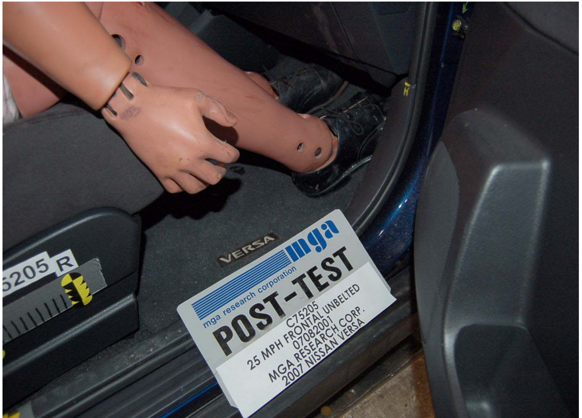
Post-Test Passenger Dummy Feet Position
