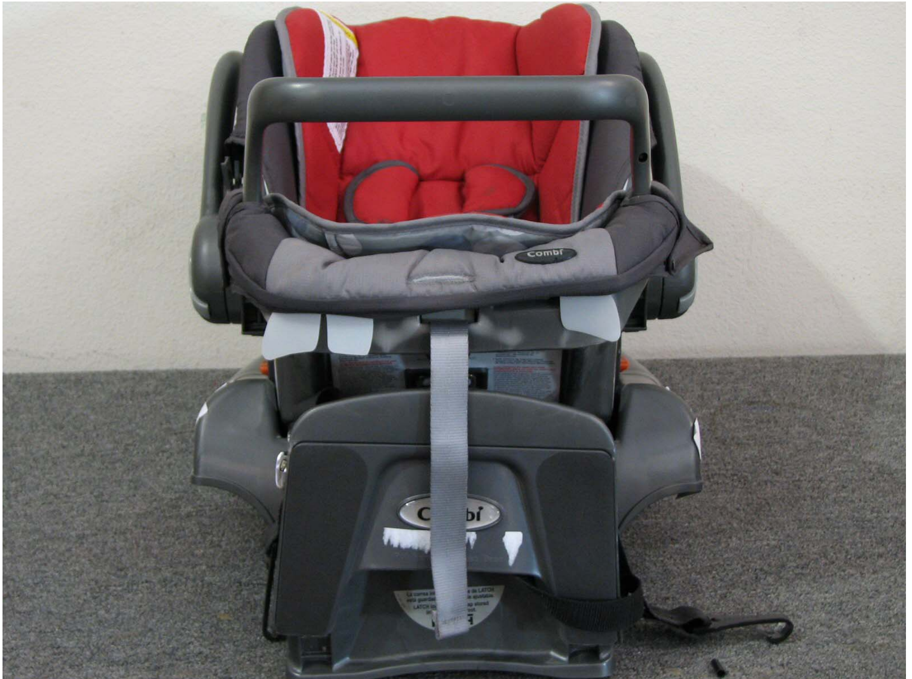
Figure D2-21: Post-Test Frontal View of Position 4 CRS
