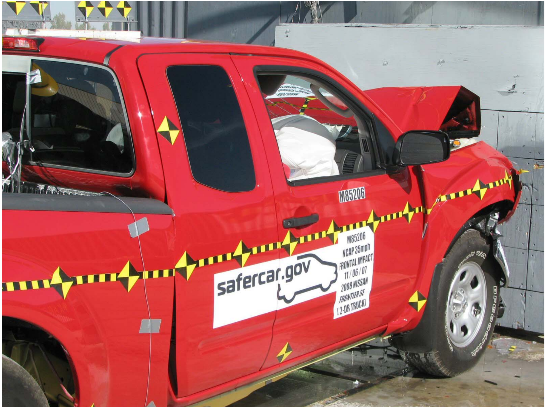
Figure A-17: Post-Test Right Side \frac{3}{4} View of Doors After Impact
