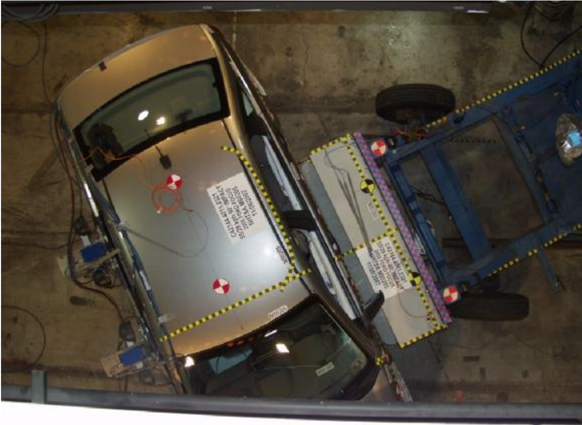
Figure A-31: Pre-Test Overhead View of Aligned MDB and Vehicle
