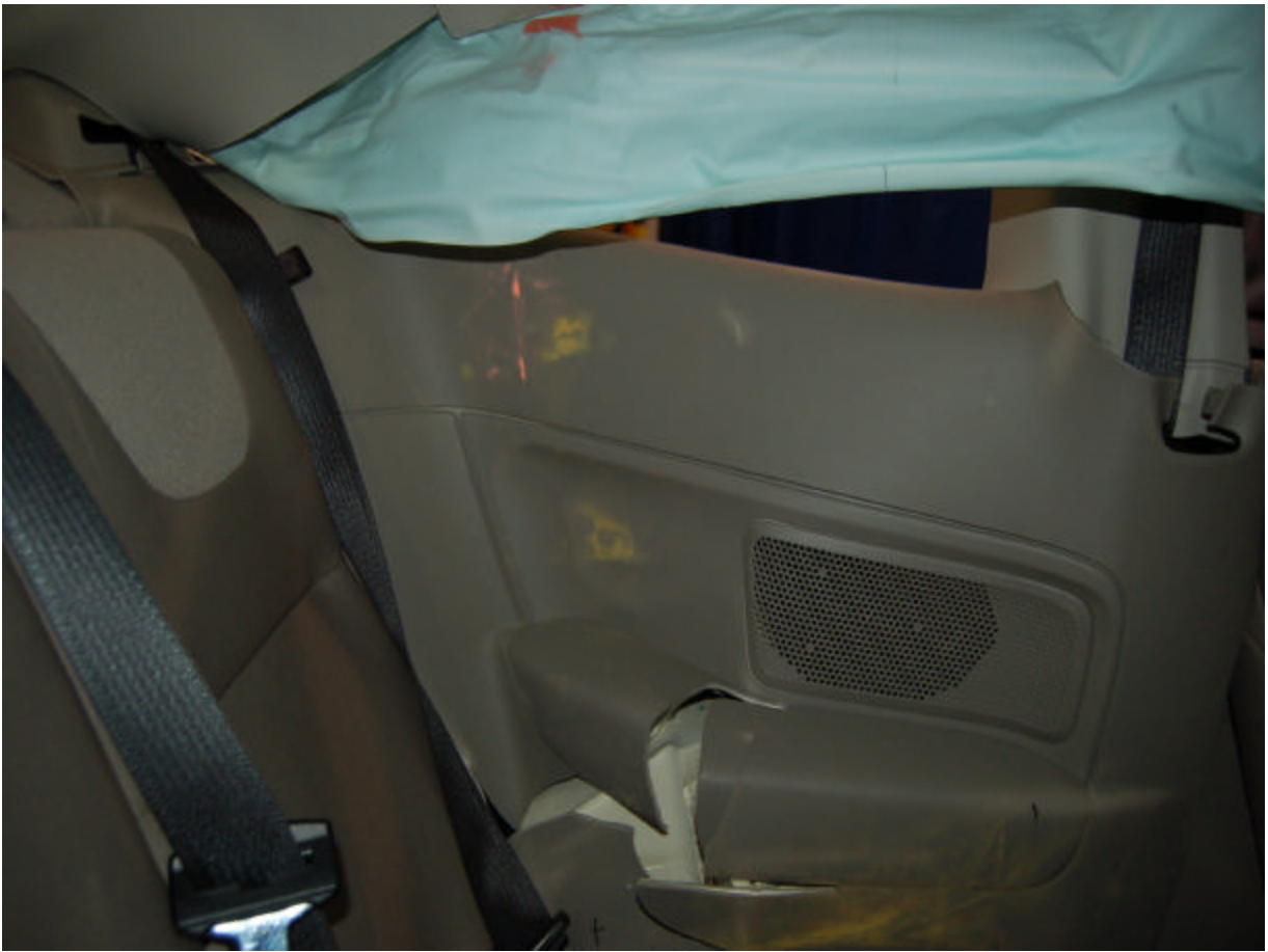
Post-Test Passenger Dummy Upper Torso Contact
