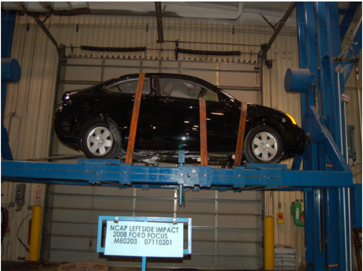
Vehicle on Rollover Device (360 Degrees)
