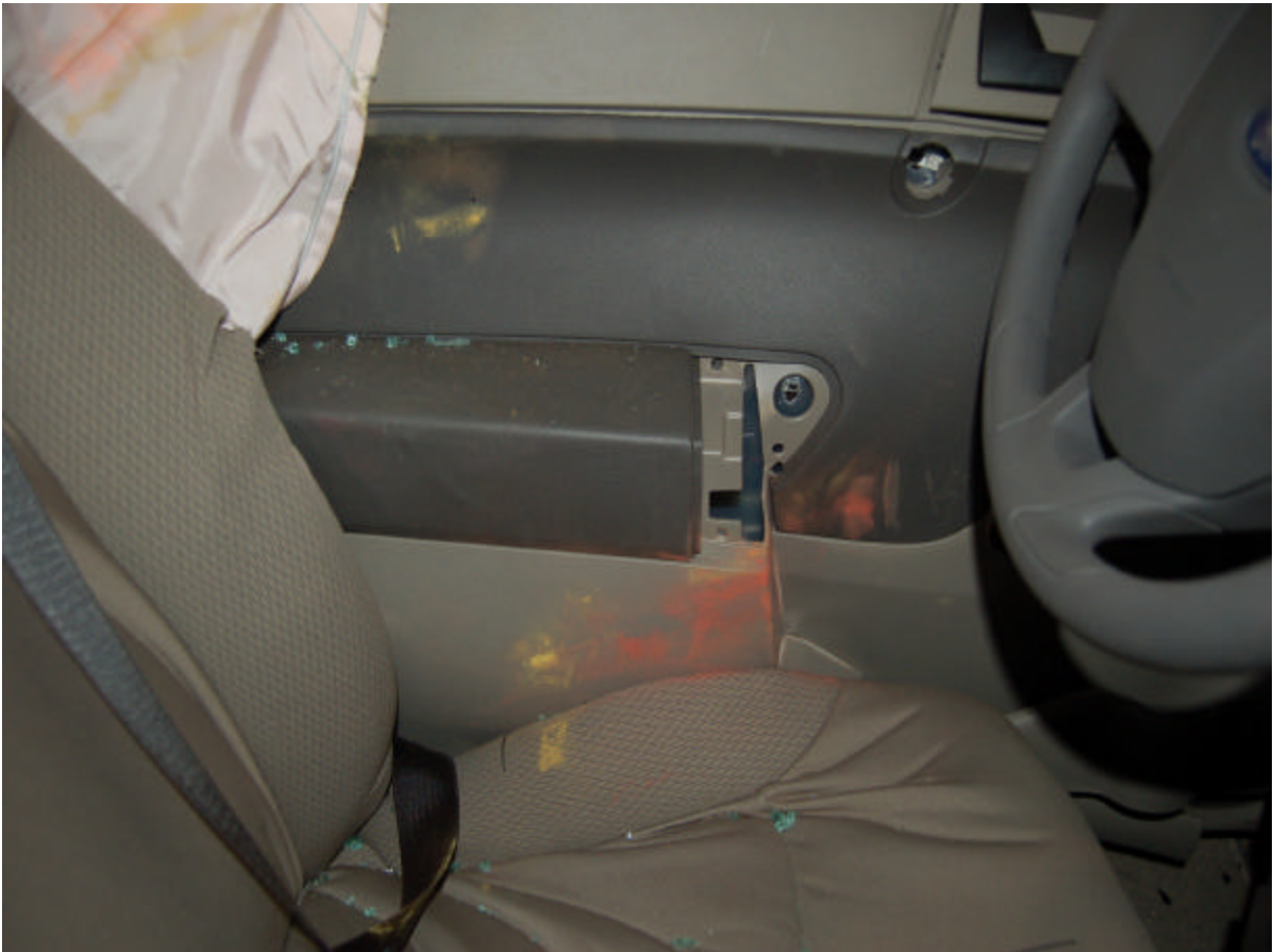
Post-Test Driver Dummy Lower Torso Contact
