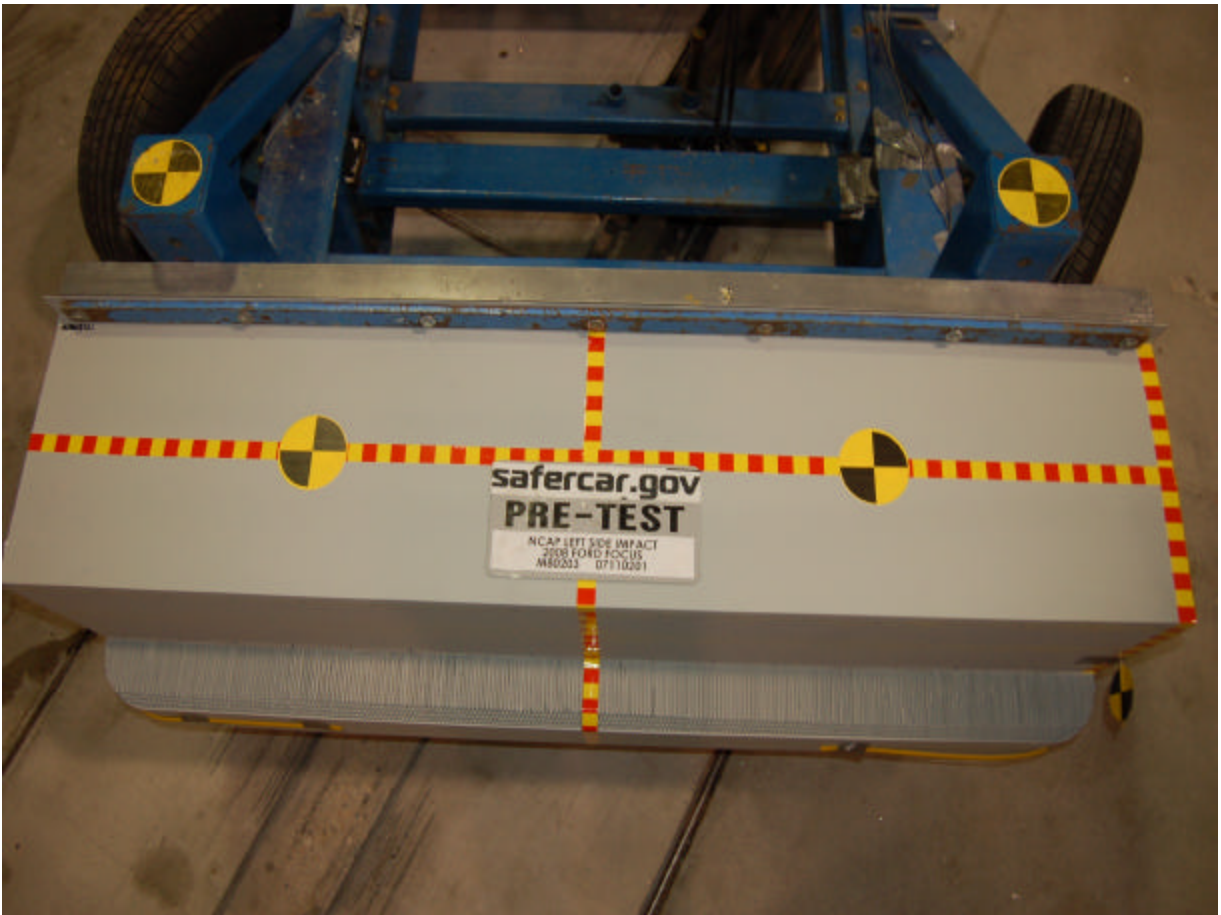
Pre-Test Top View of Deformable Barrier
