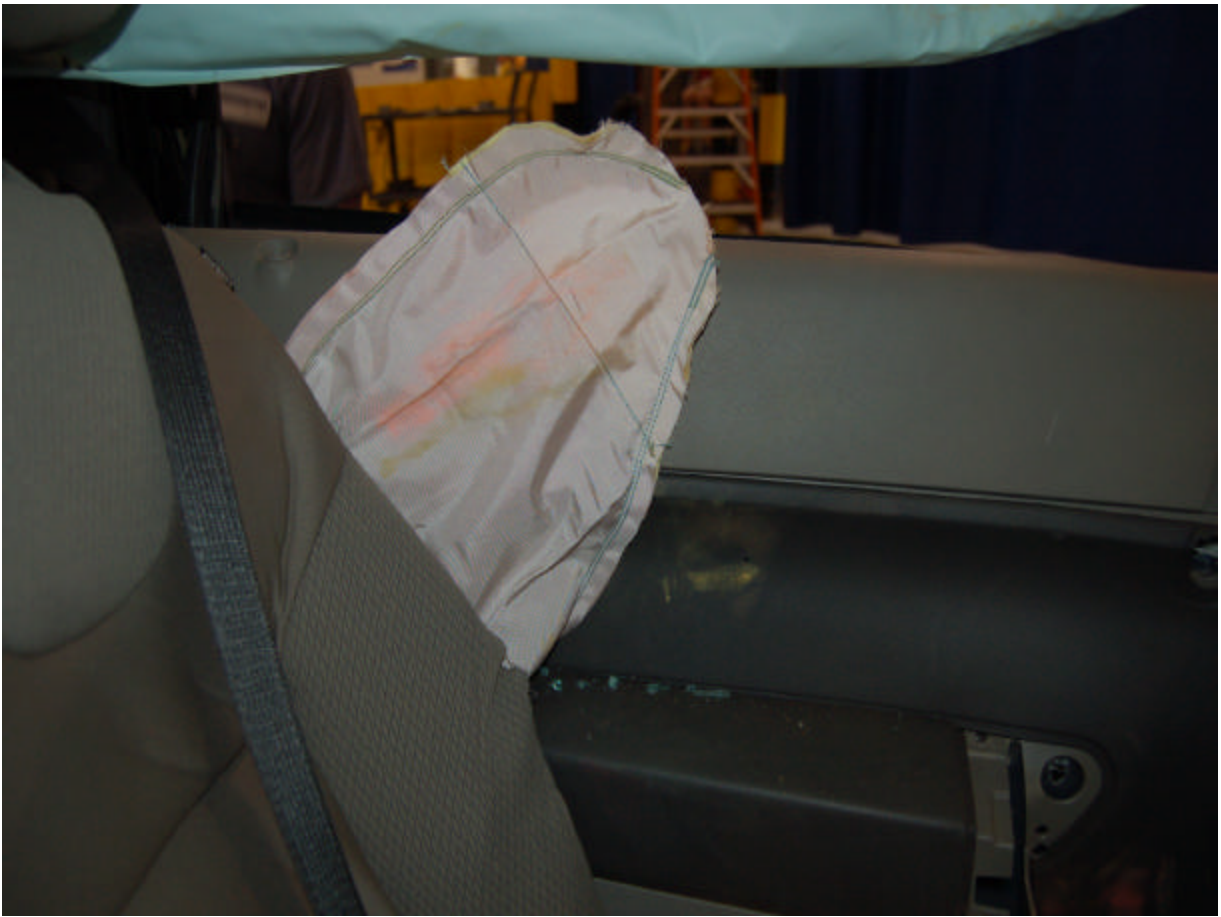
Post-Test Driver Dummy Upper Torso Contact
