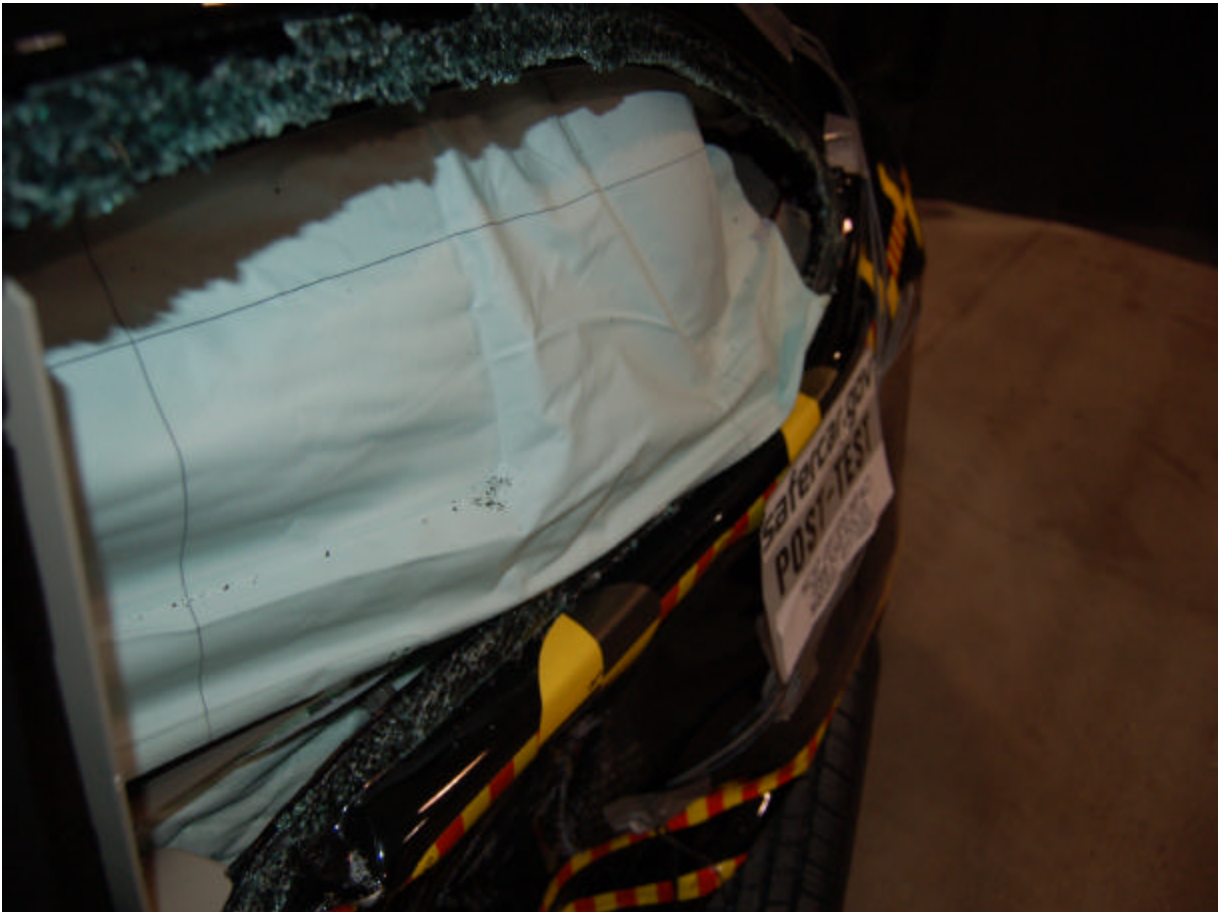
Post-Test Passenger Dummy Clearance From Door
