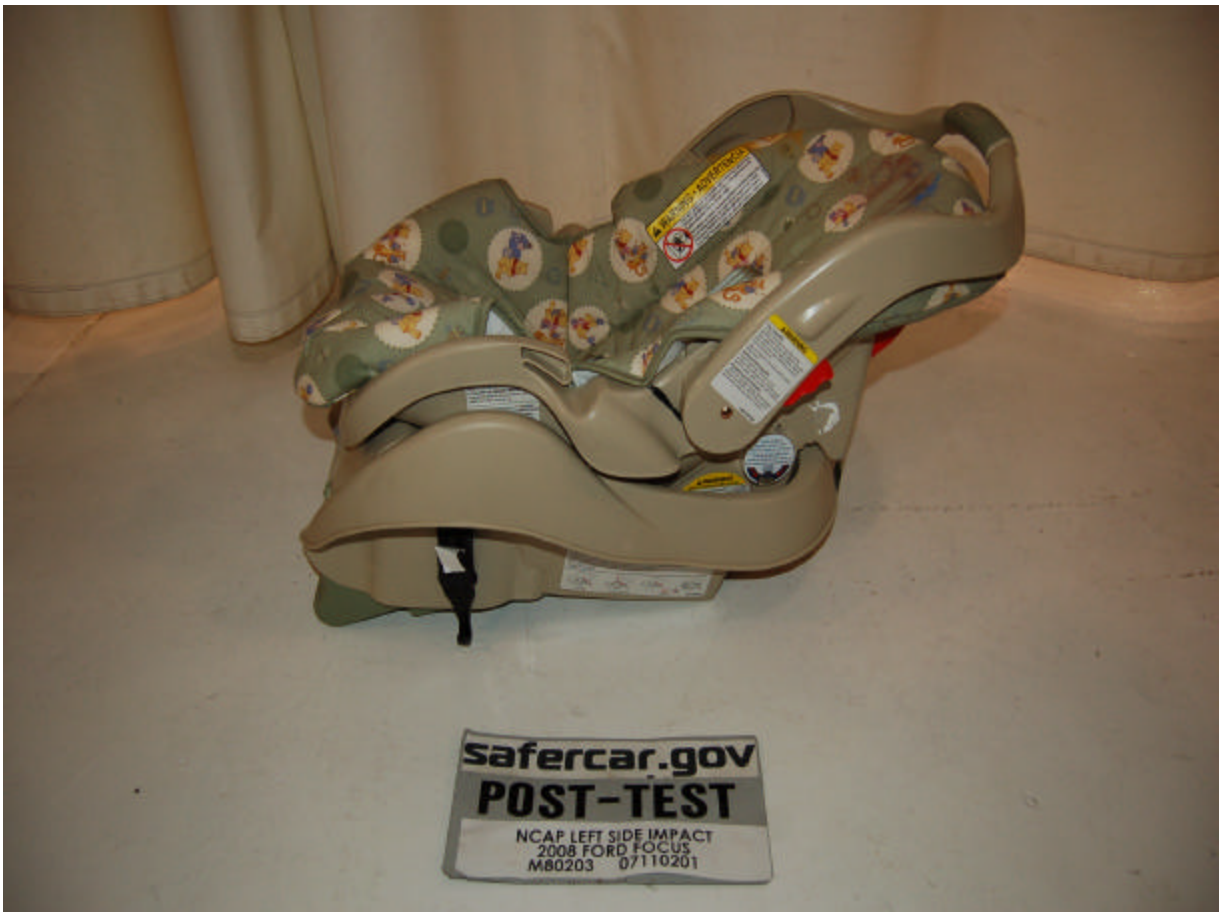
Post-Test Left Side View of Position 3 CRS
