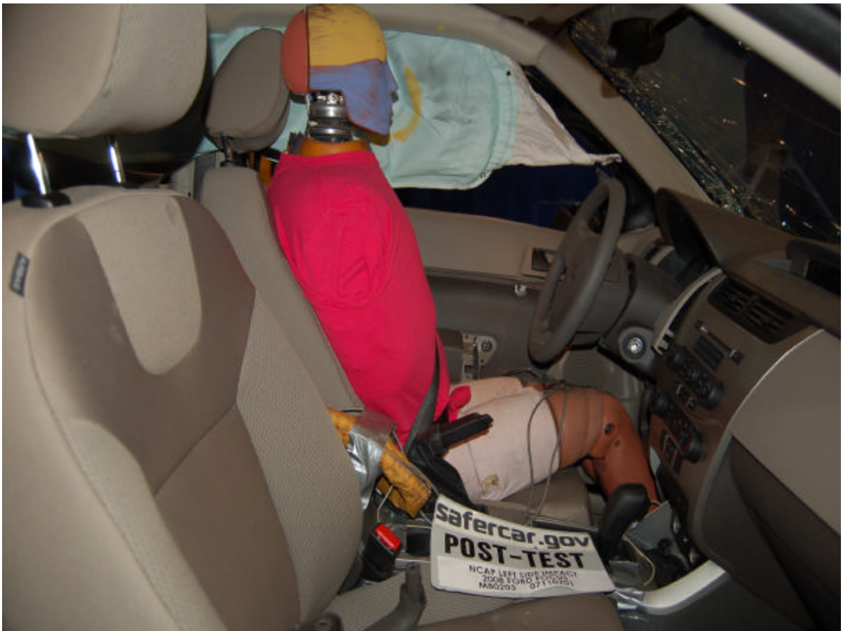
Post-Test Driver Dummy Right Side View
