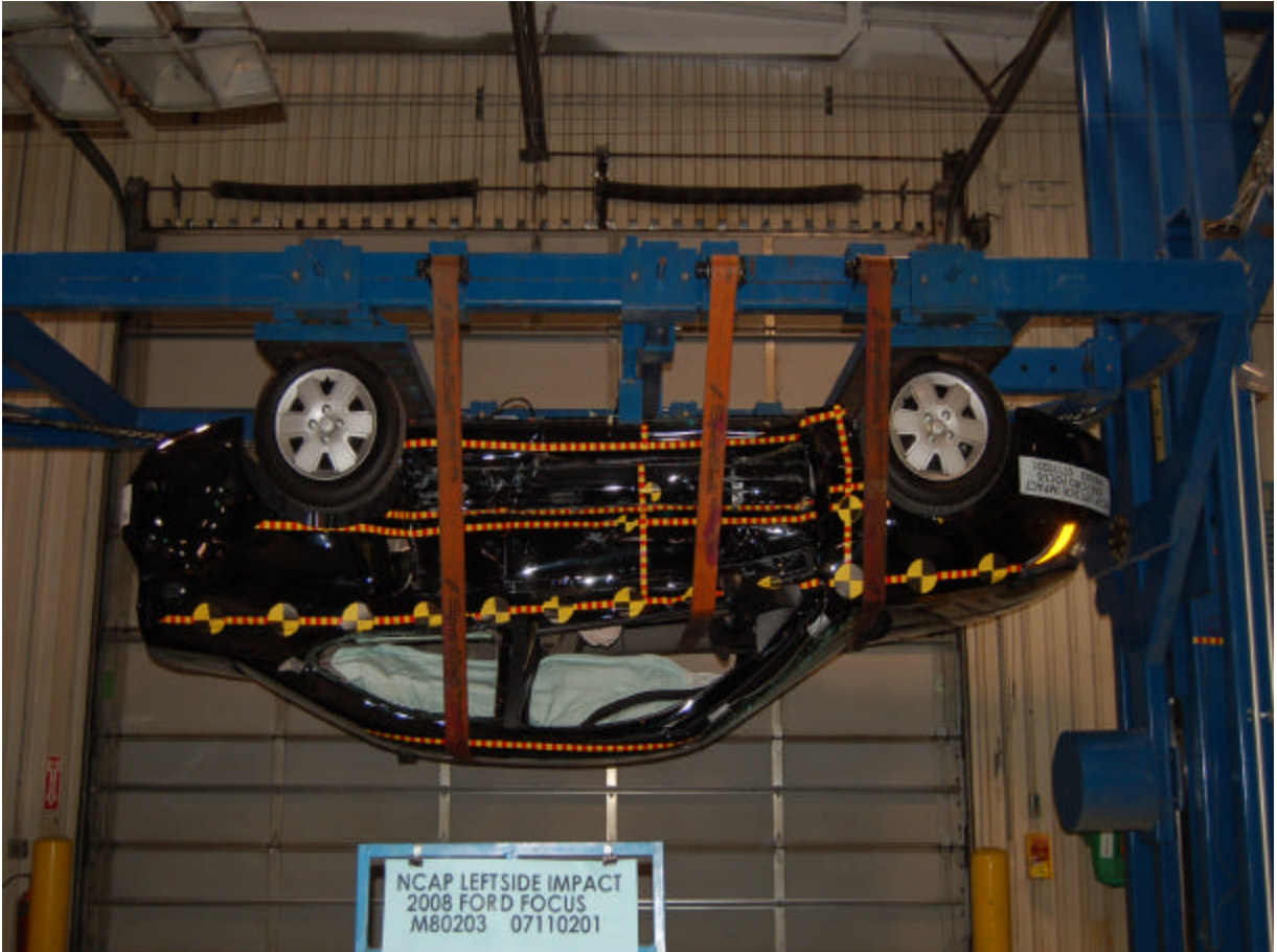
Vehicle on Rollover Device (180 Degrees)
