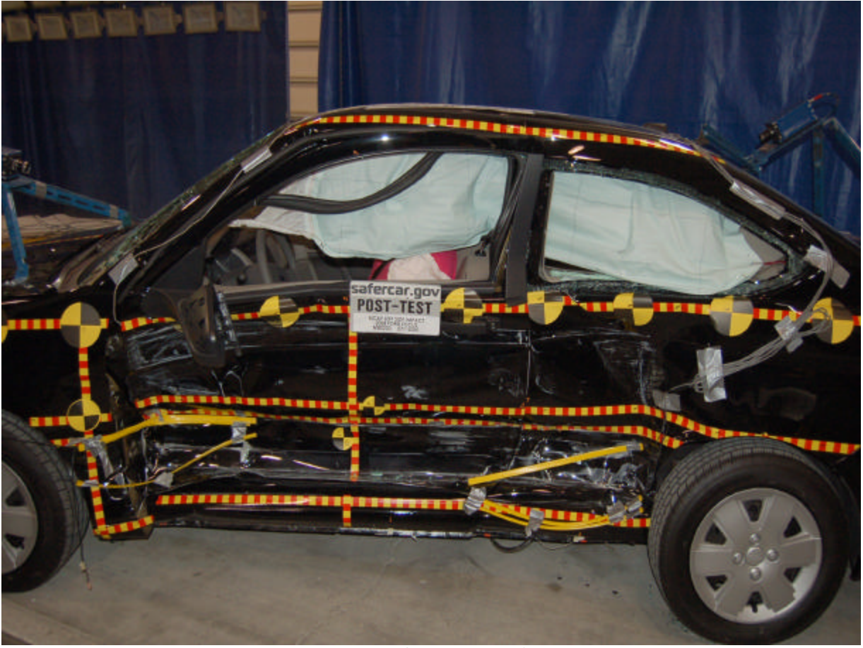
Post-Test Left Side Impact Close-up
