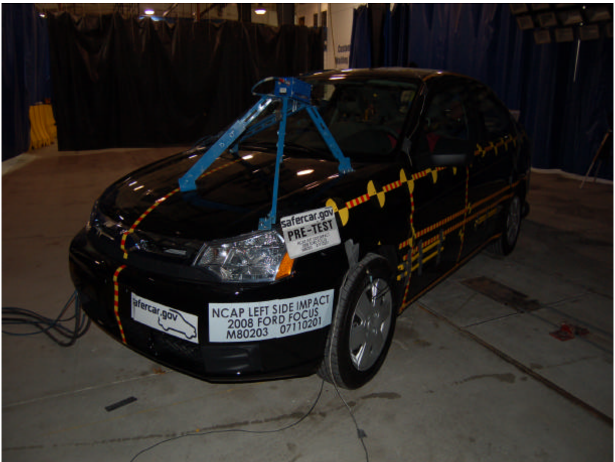
Pre-Test Left Front \frac{3}{4} View
