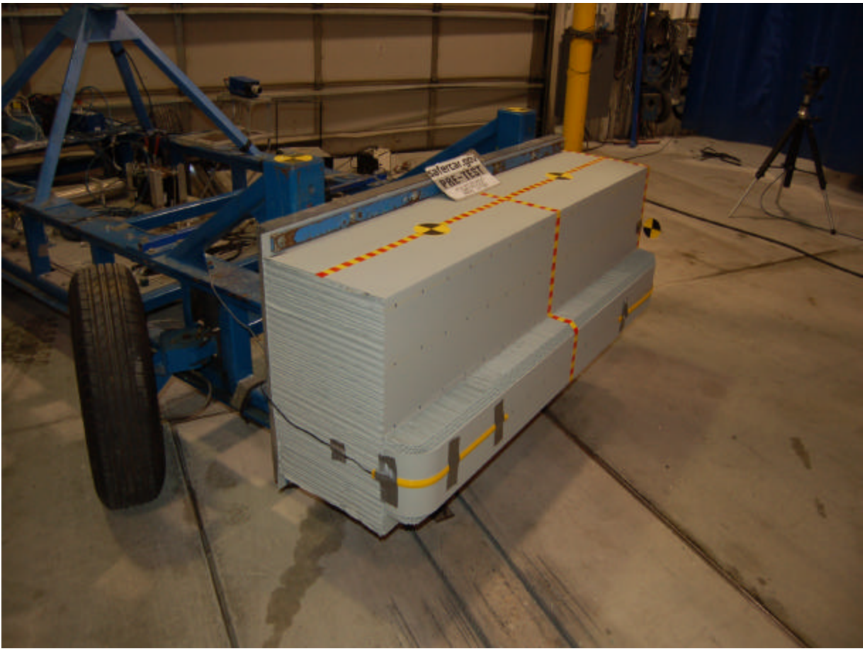
Pre-Test Right Side View of Deformable Barrier
