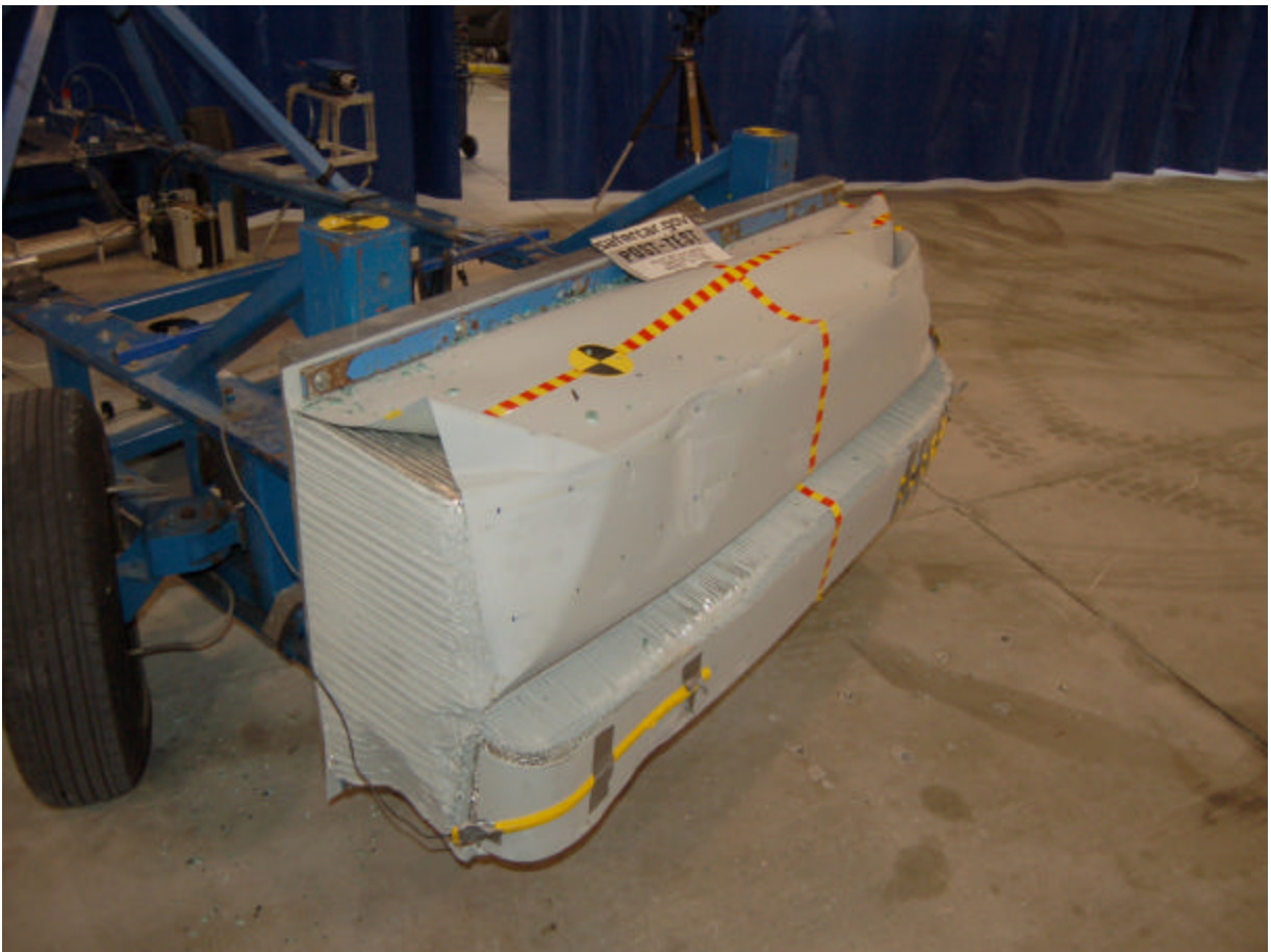
Post-Test Right Side View of Deformable Barrier
