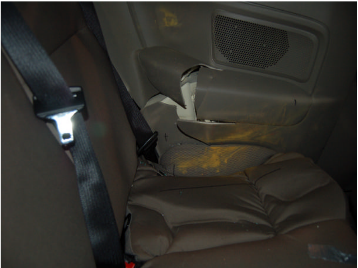
Post-Test Passenger Dummy Lower Torso Contact
