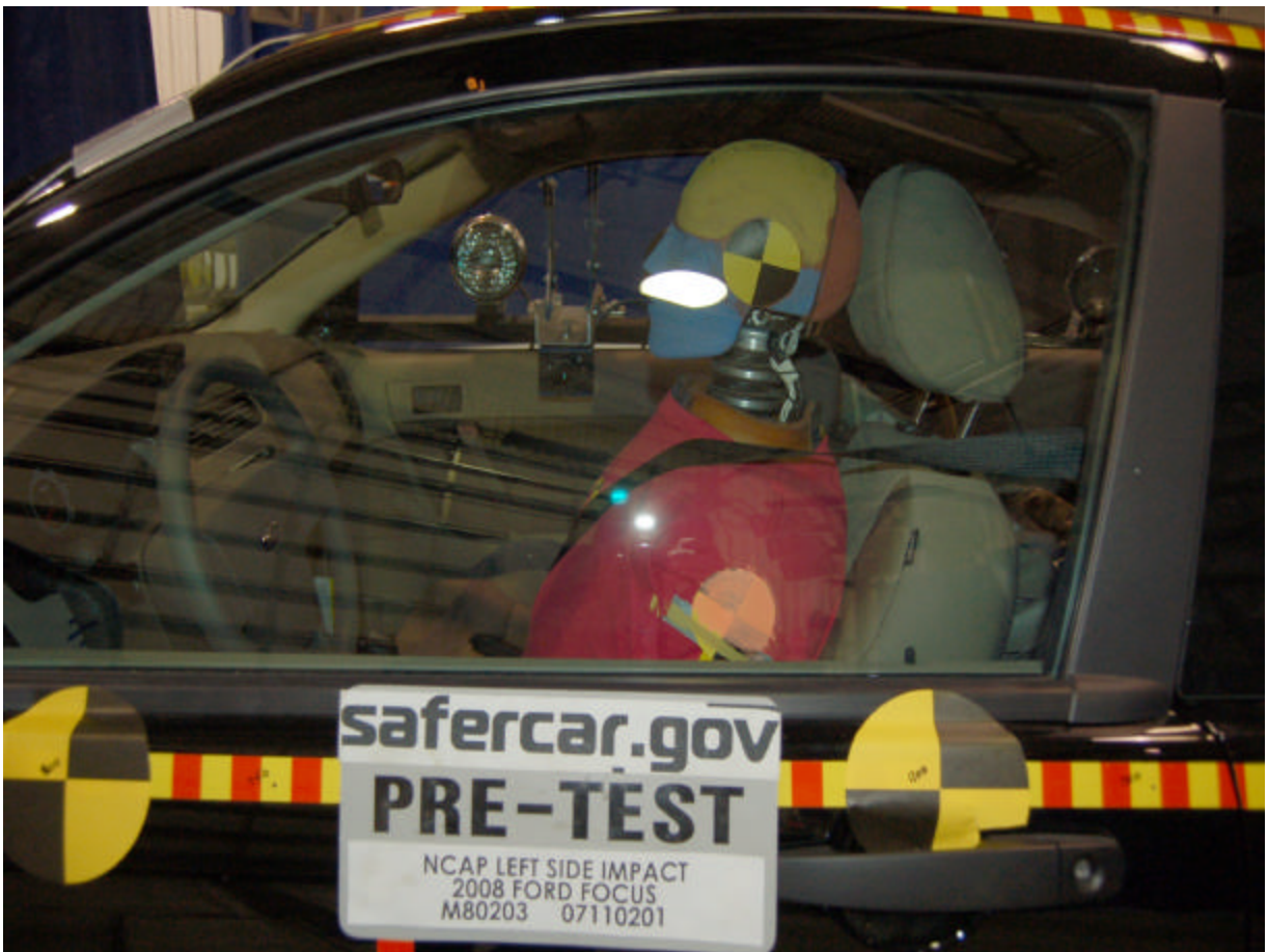
Pre-Test Driver Dummy (Through Window)
