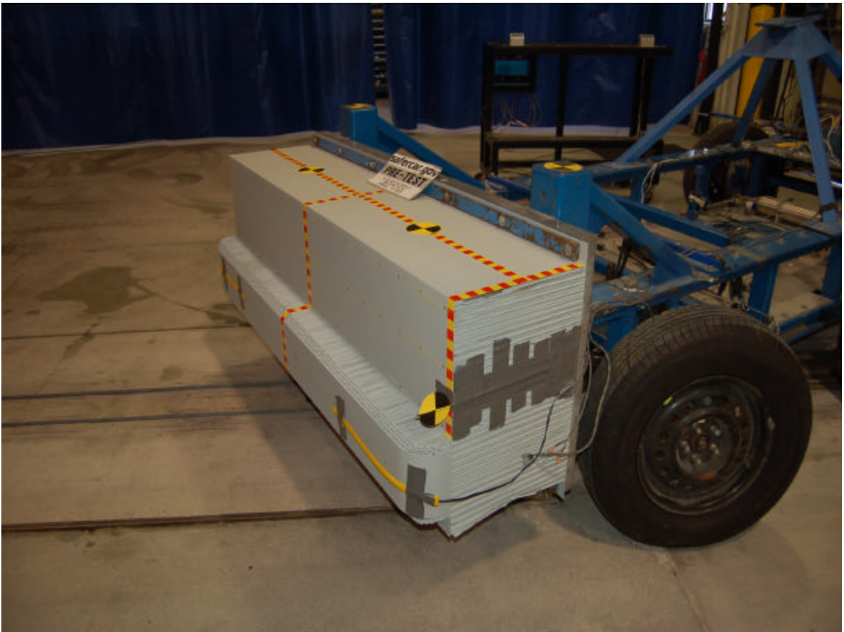
Pre-Test Left Side View of Deformable Barrier
