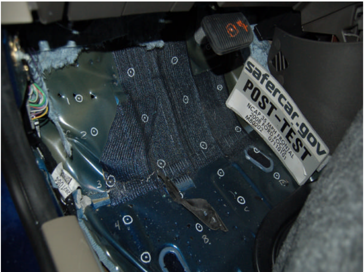
Post-Test Driver Side Floor Pan
