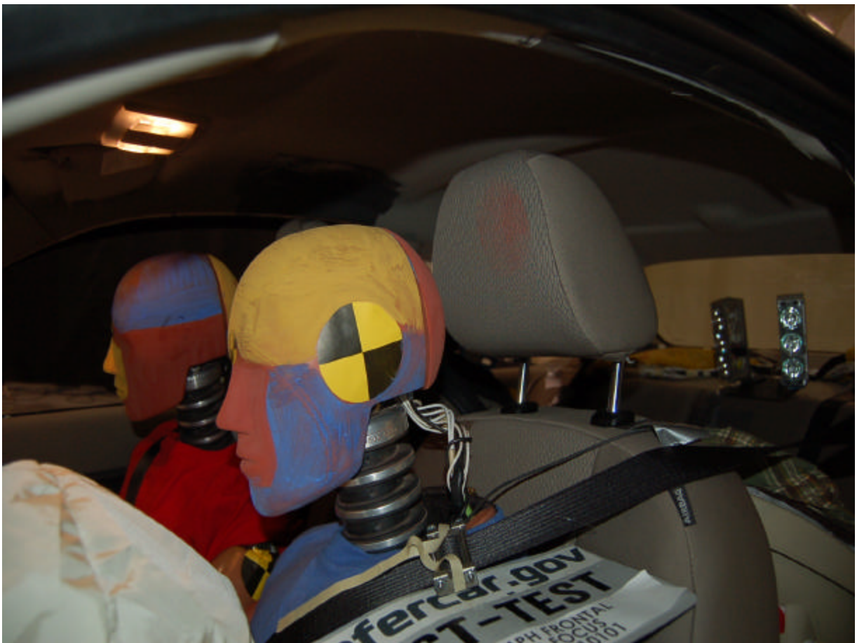
Post-Test Driver Dummy Head Contact (headrest)
