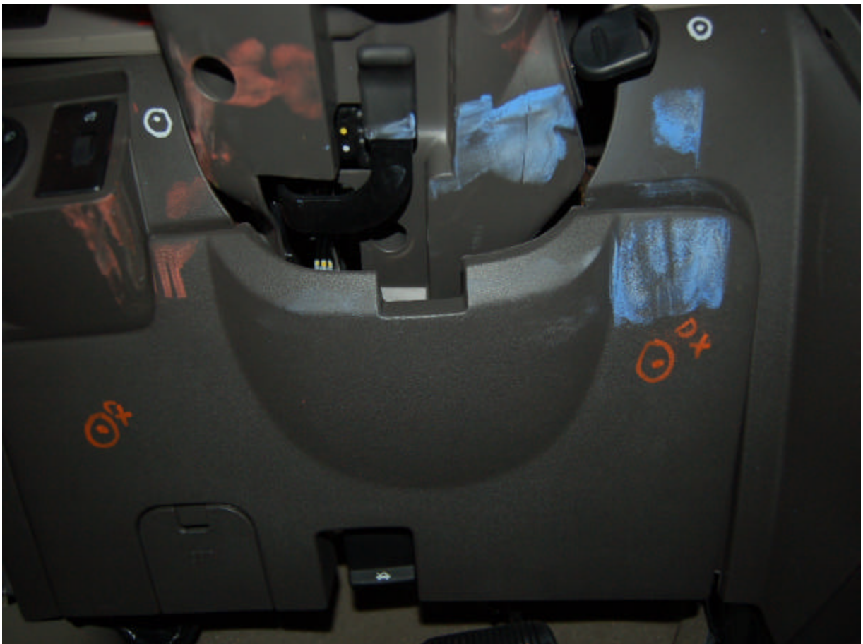
Post-Test Driver Dummy Knee Contact
