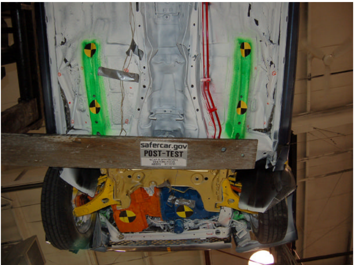
Post-Test Front Underbody View
