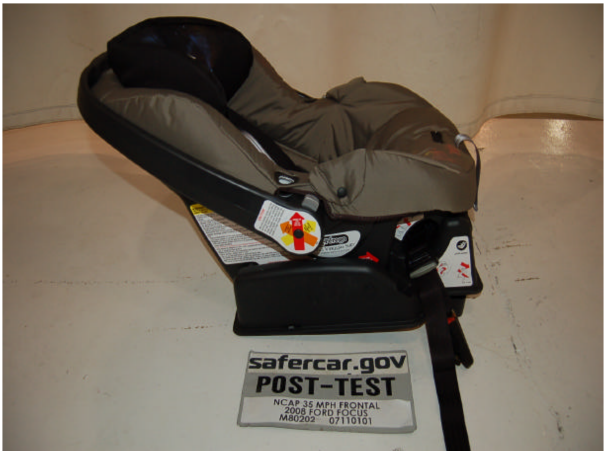
Post-Test Right Side View of Position 3 CRS
