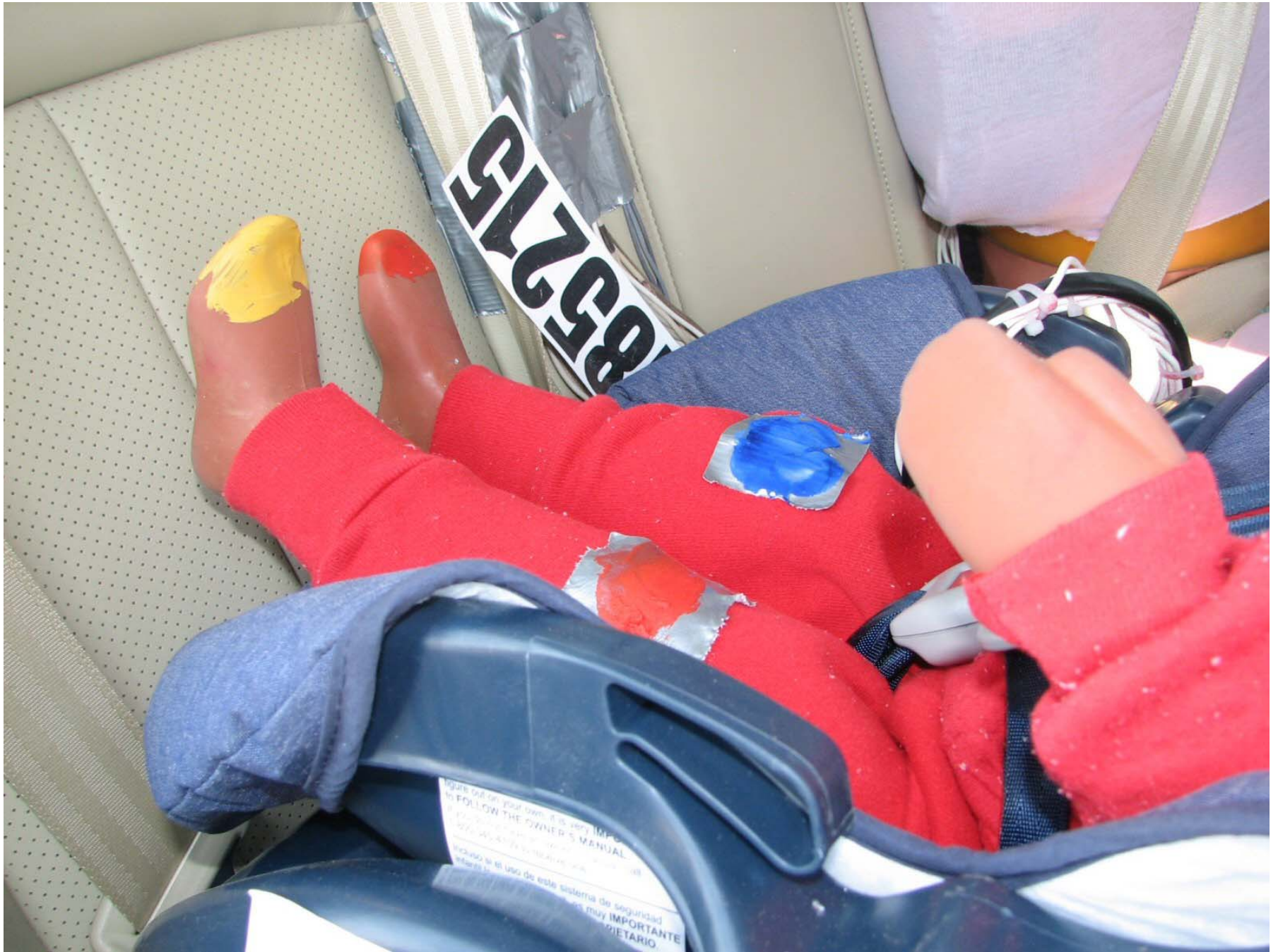
Figure D2-18: Post-Test Position 3 Dummy Legs
