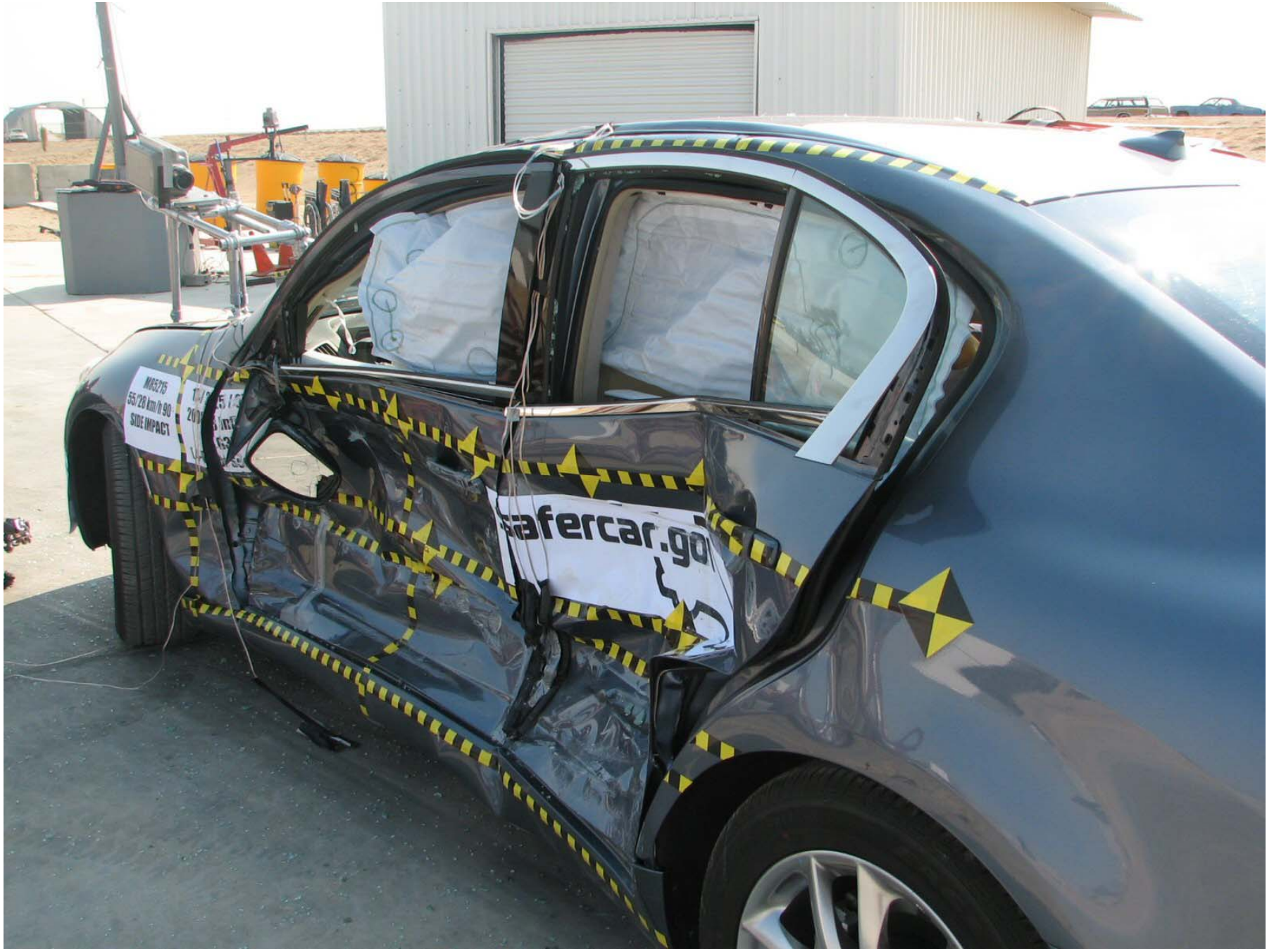
Figure A-30: Post-Test Rear 3/4 View of Left Side Door
