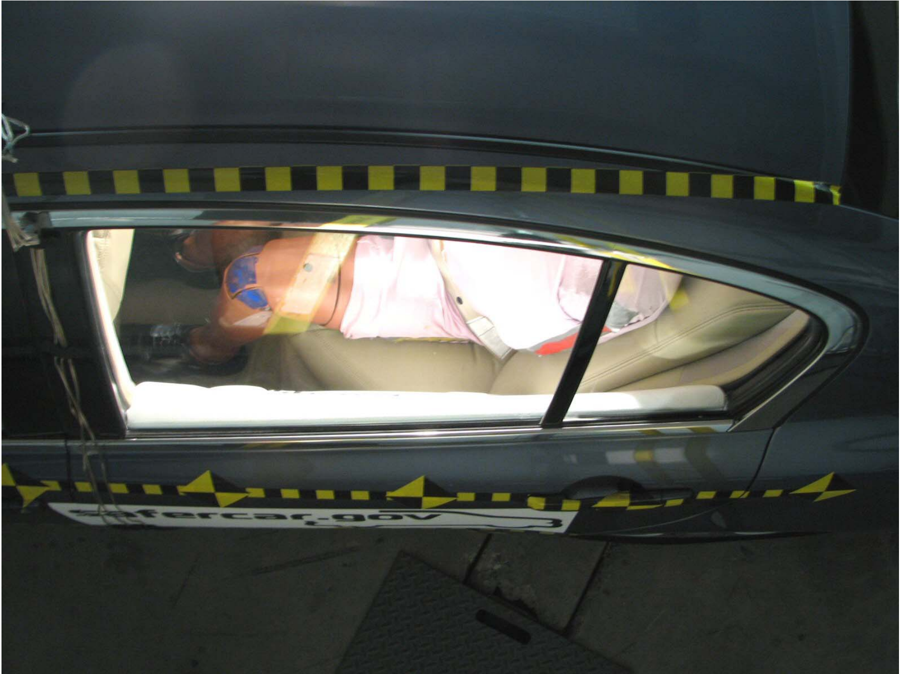
Figure A-47: Pre-Test Passenger Dummy Clearance From Door
