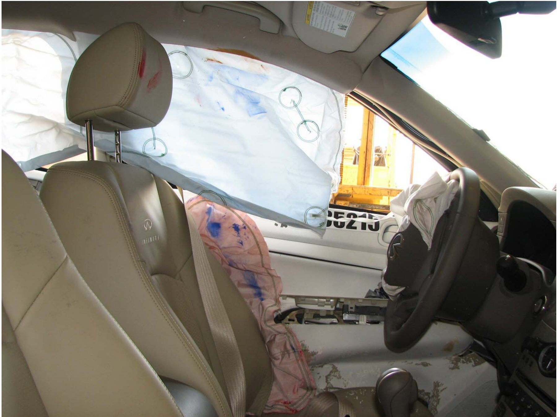
Figure A-43: Post-Test Front Door Panel (Interior)
