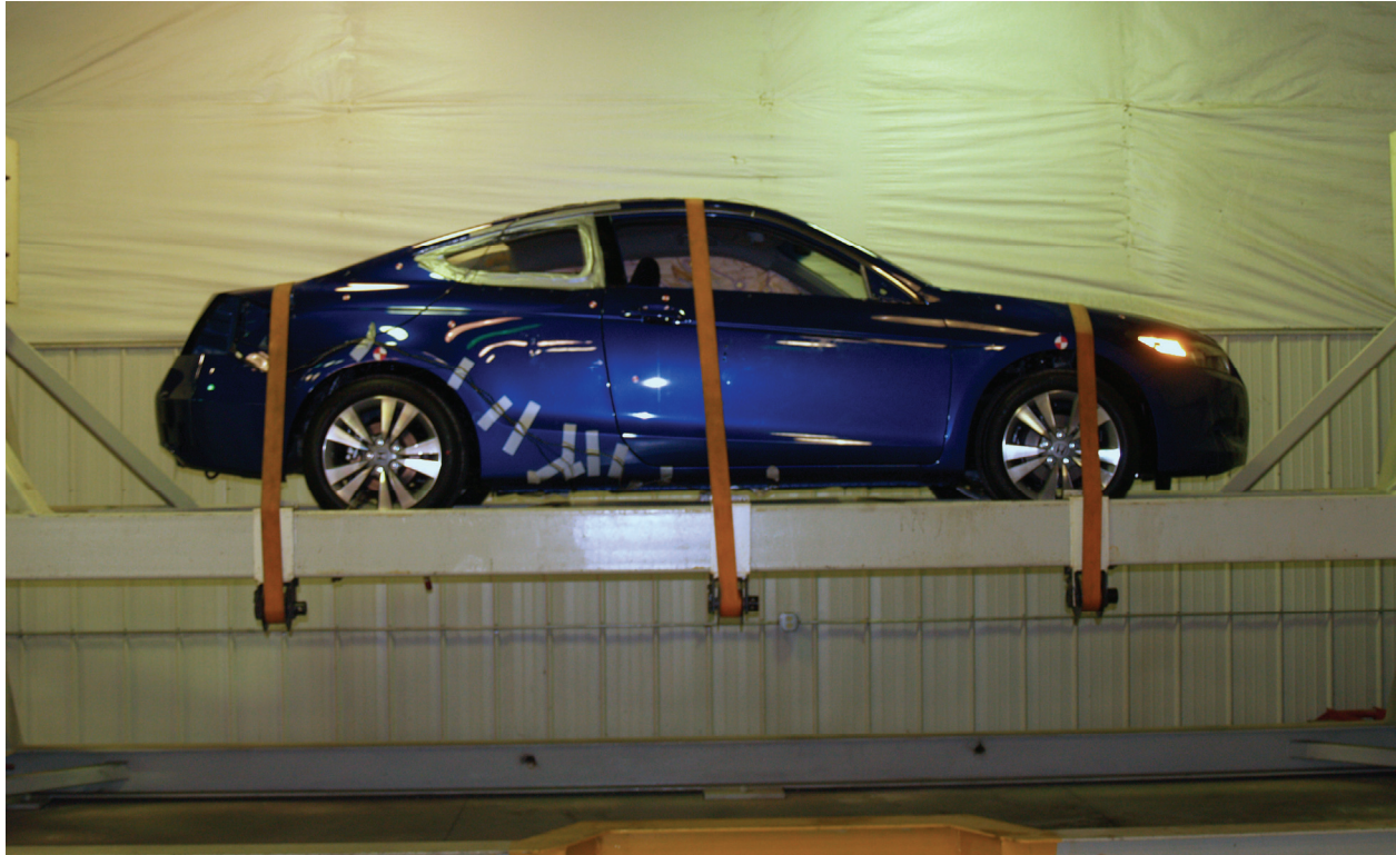
Figure A-57: FMVSS 301 0 degrees
