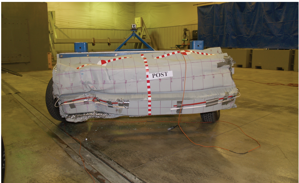
Figure A-50: Post test front view of MDB barrier face
