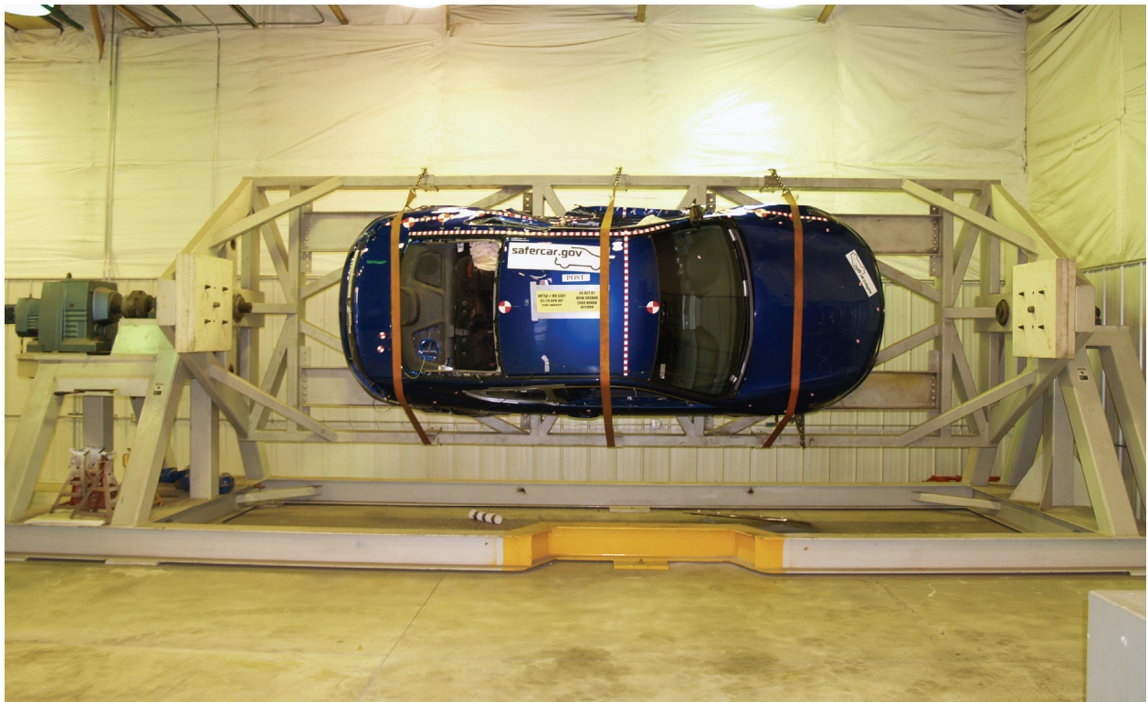
Figure A-60: FMVSS 301 270 degrees
