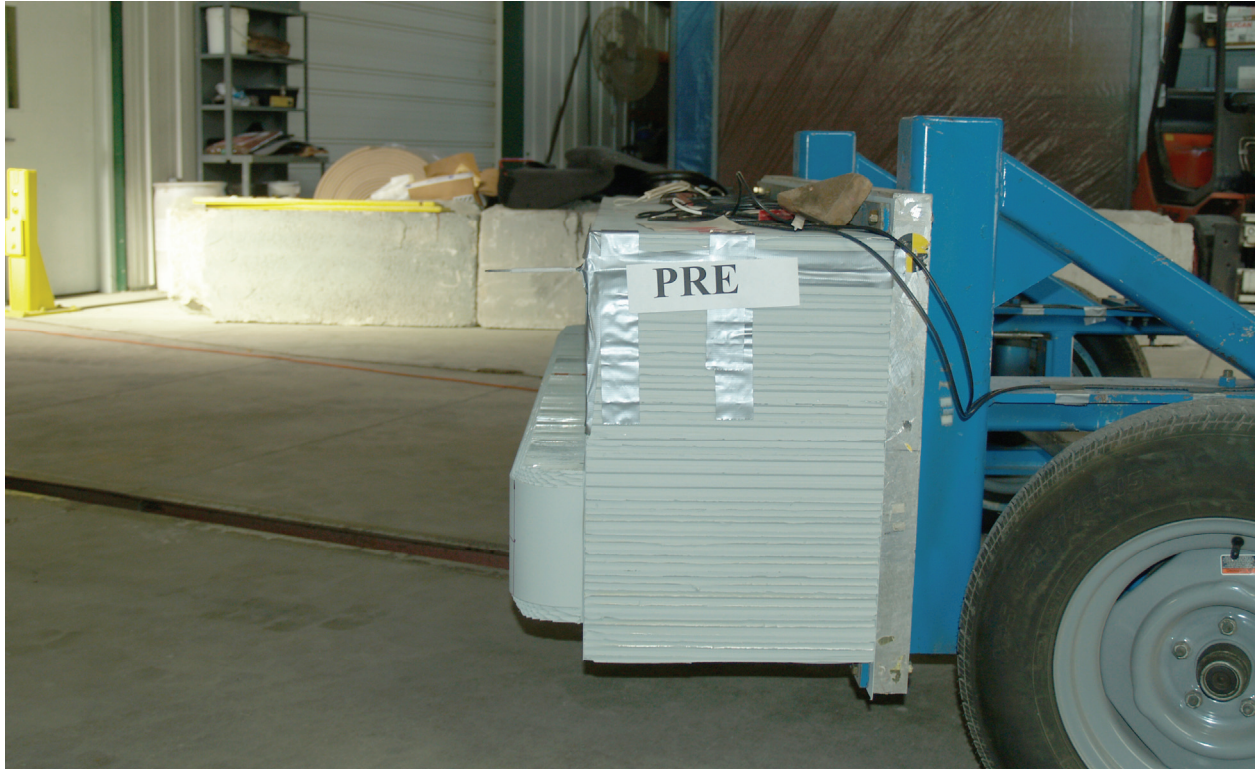
Figure A-55: Pre test left side view of MDB barrier face
