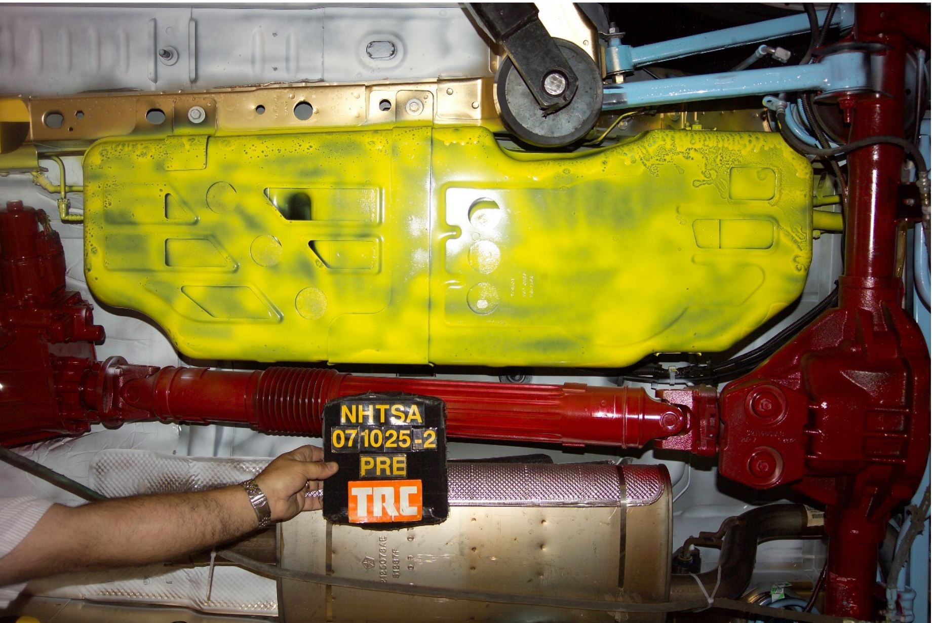
Figure A-29 Pre-Test Fuel Tank View
