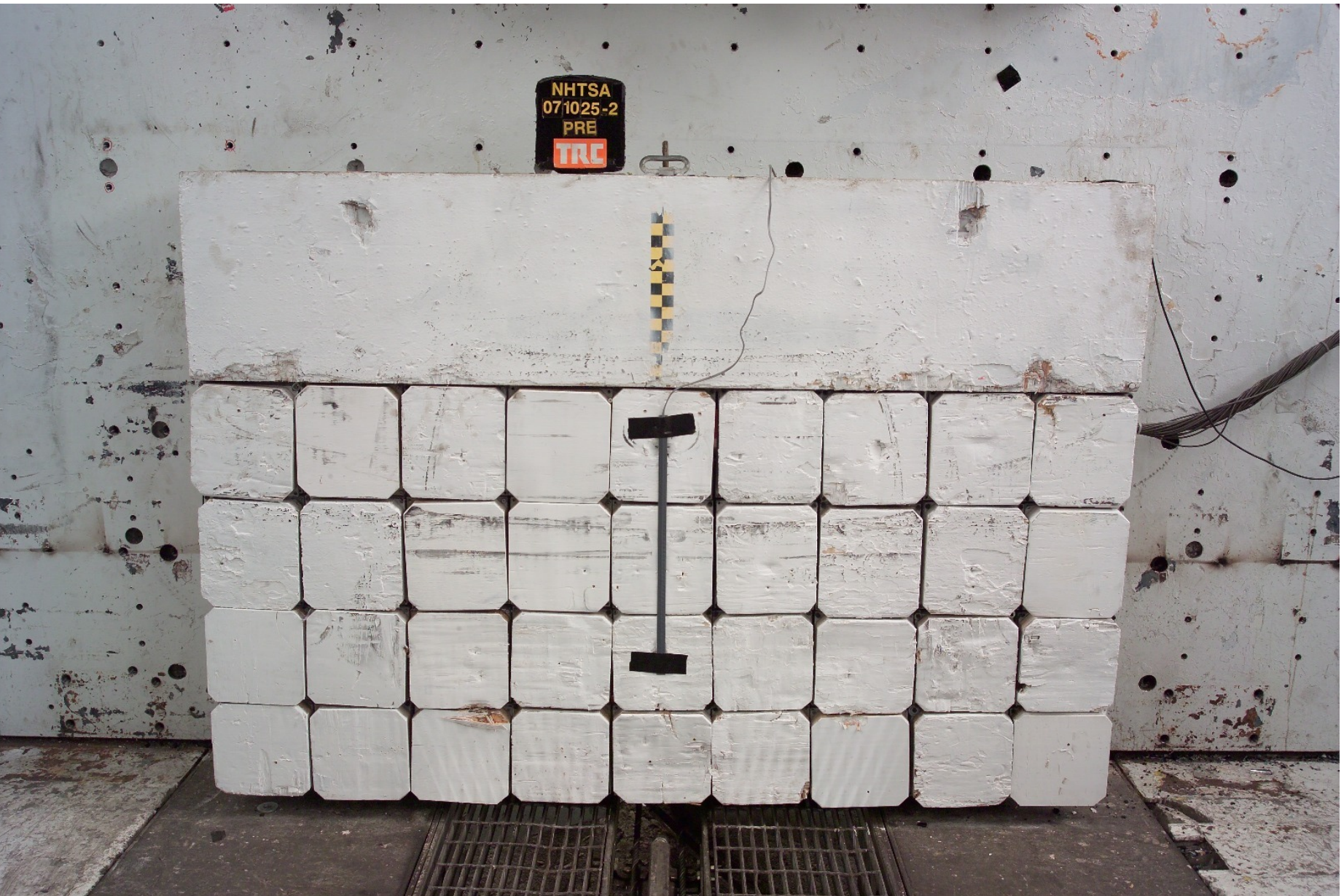
Figure A-72 Pre-Test Barrier Front View
