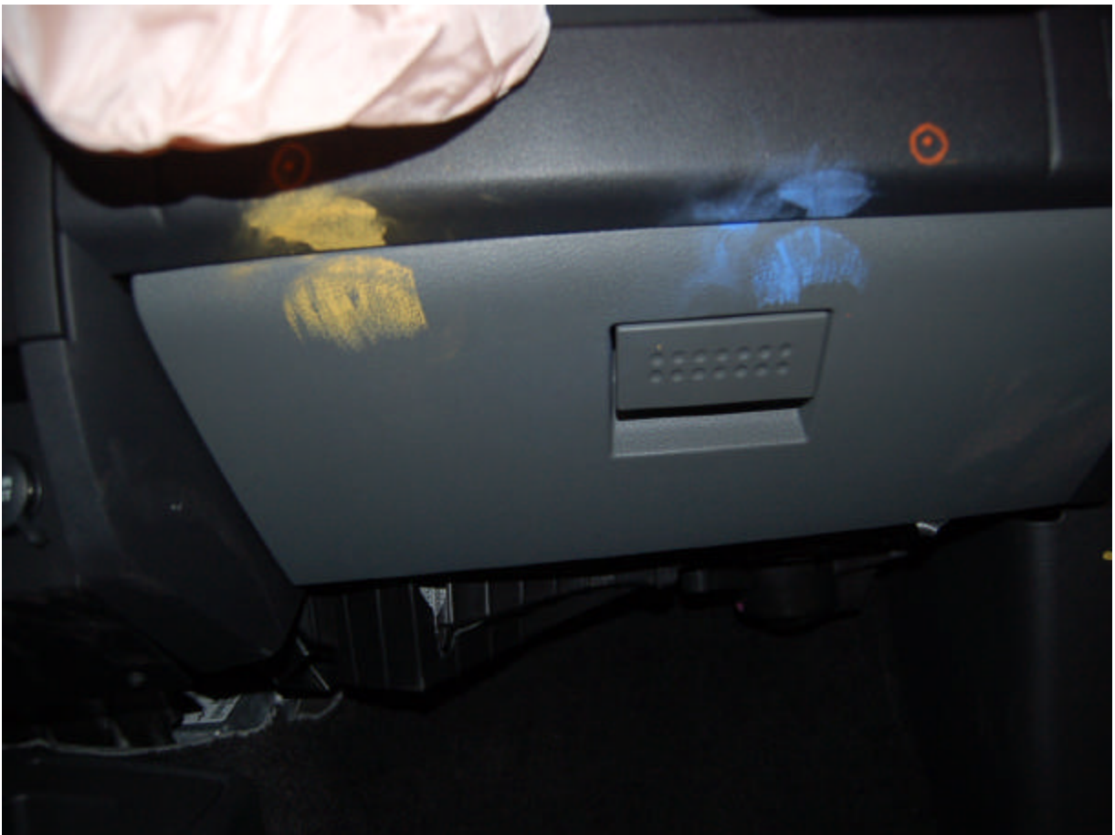
Post-Test Passenger Dummy Knee Contact
