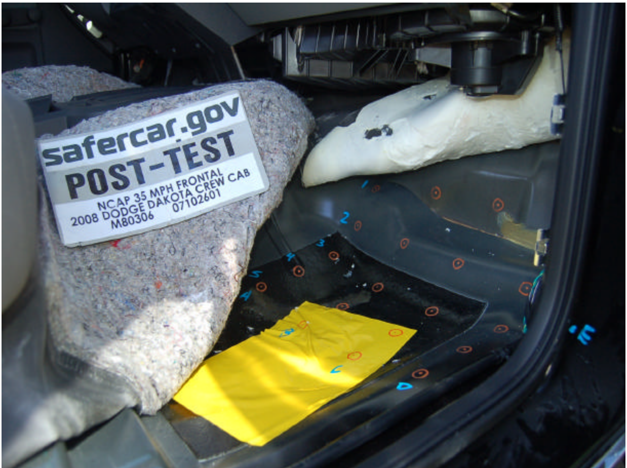
Post-Test Passenger Side Floor Pan
