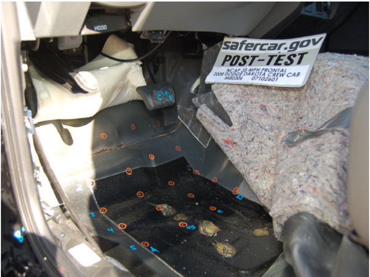
Post-Test Driver Side Floor Pan
