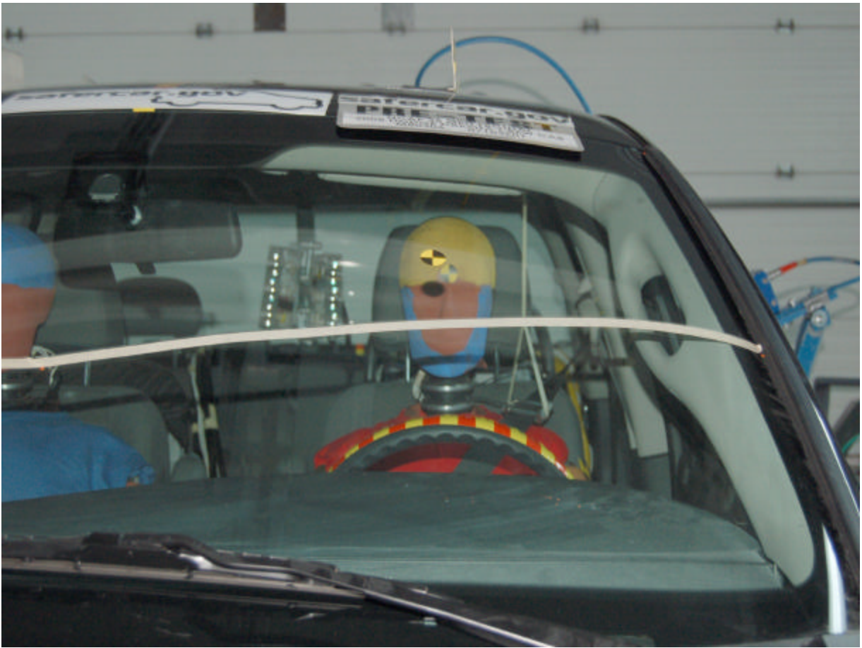
Pre-Test Driver Dummy Front View (Head Position)
