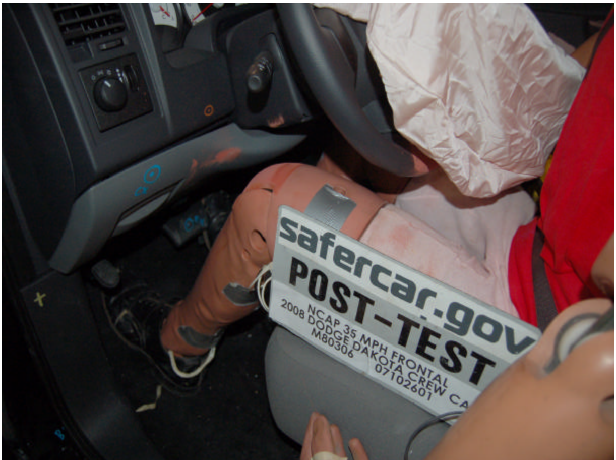
Post-Test Driver Side Knee Bolster
