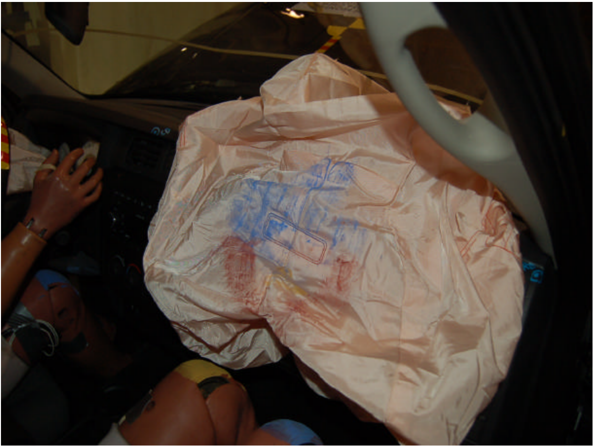
Post-Test Passenger Dummy Airbag Contact
