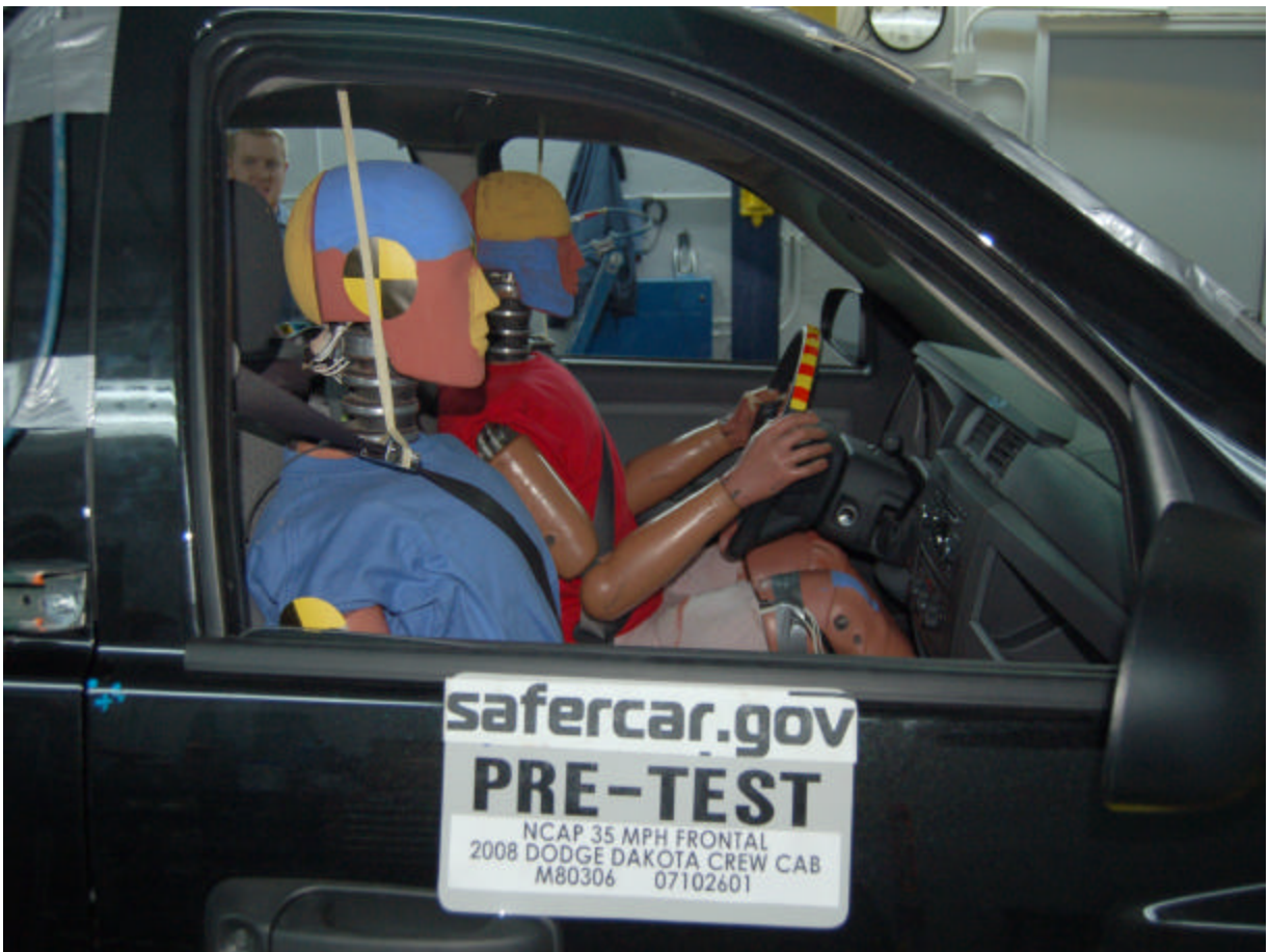
Pre-Test Passenger Dummy (Through Window)
