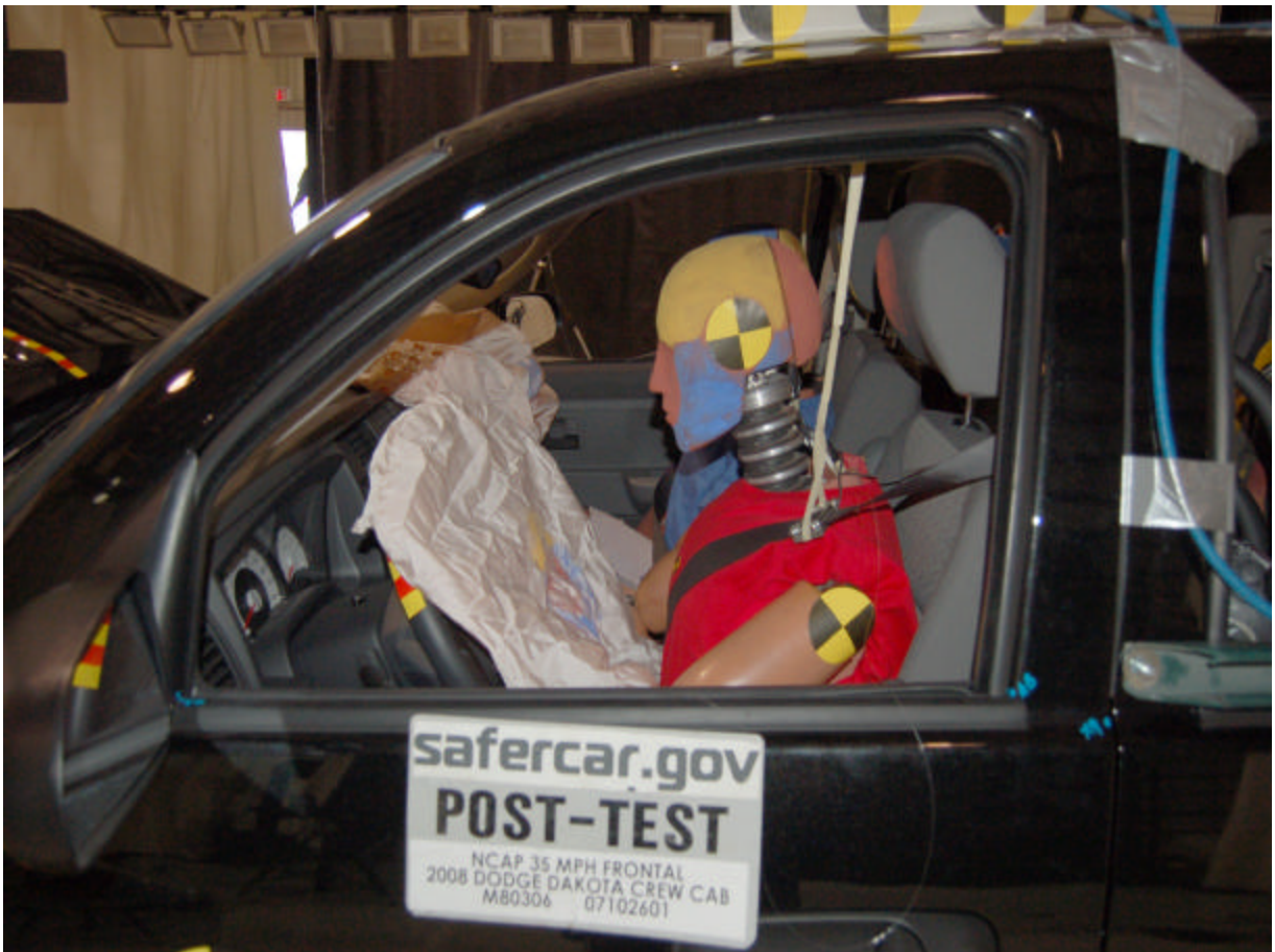
Post-Test Driver Dummy (Through Window)
