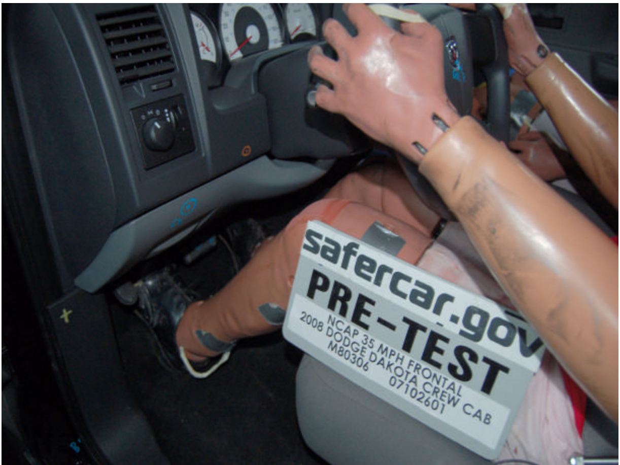
Pre-Test Driver Side Knee Bolster
