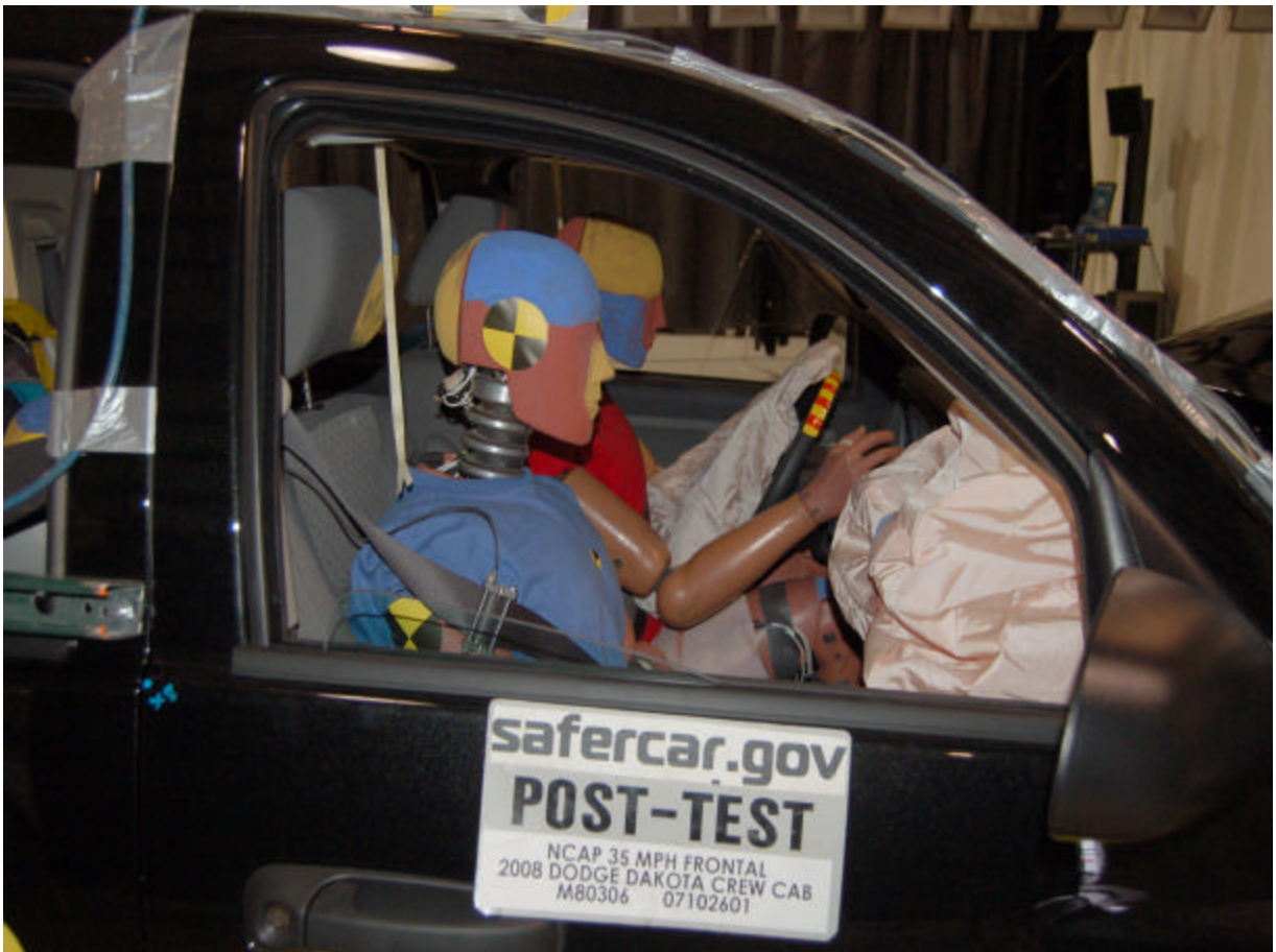
Post-Test Passenger Dummy (Through Window)
