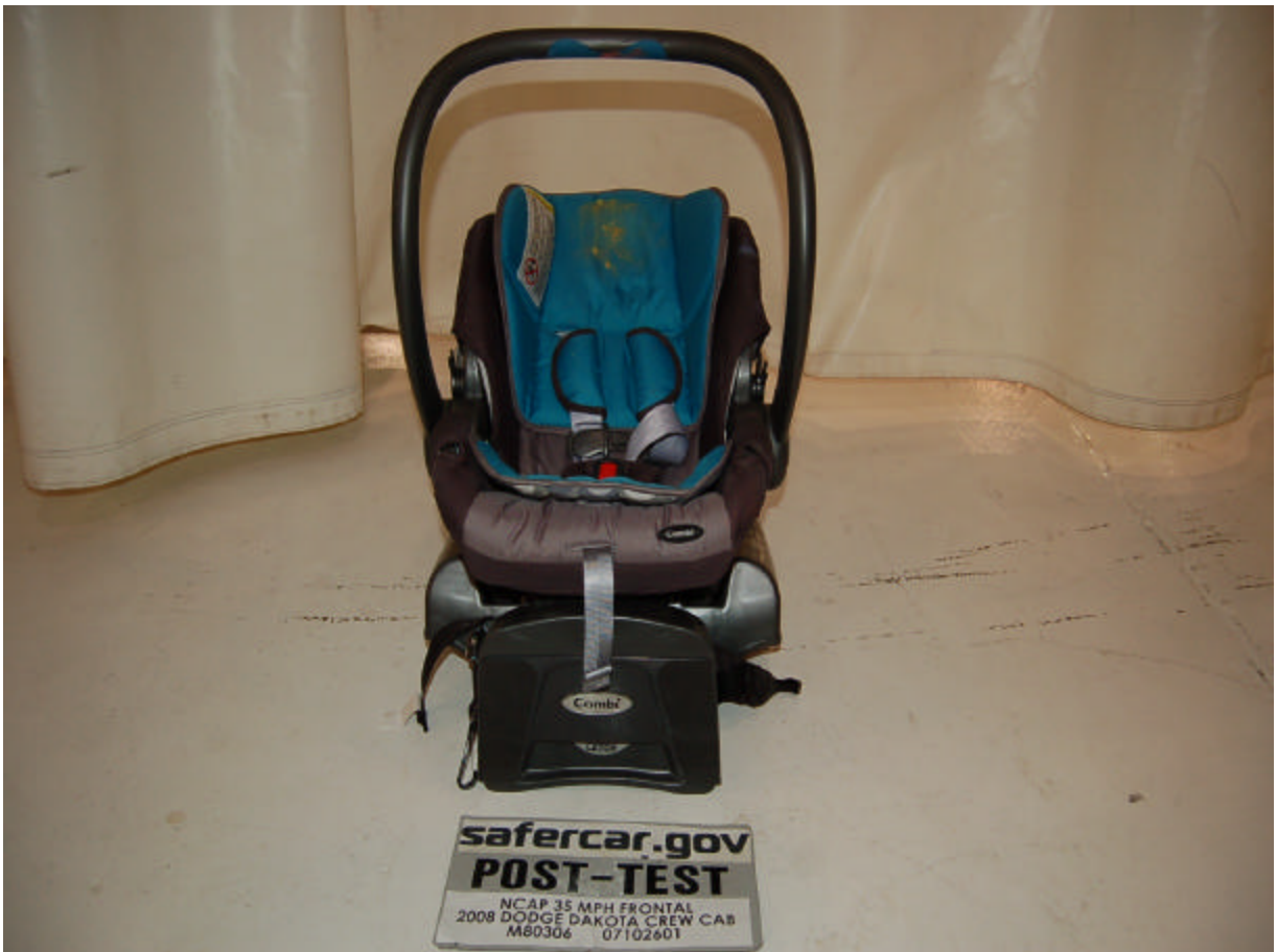
Post-Test Front View of Position 4 CRS
