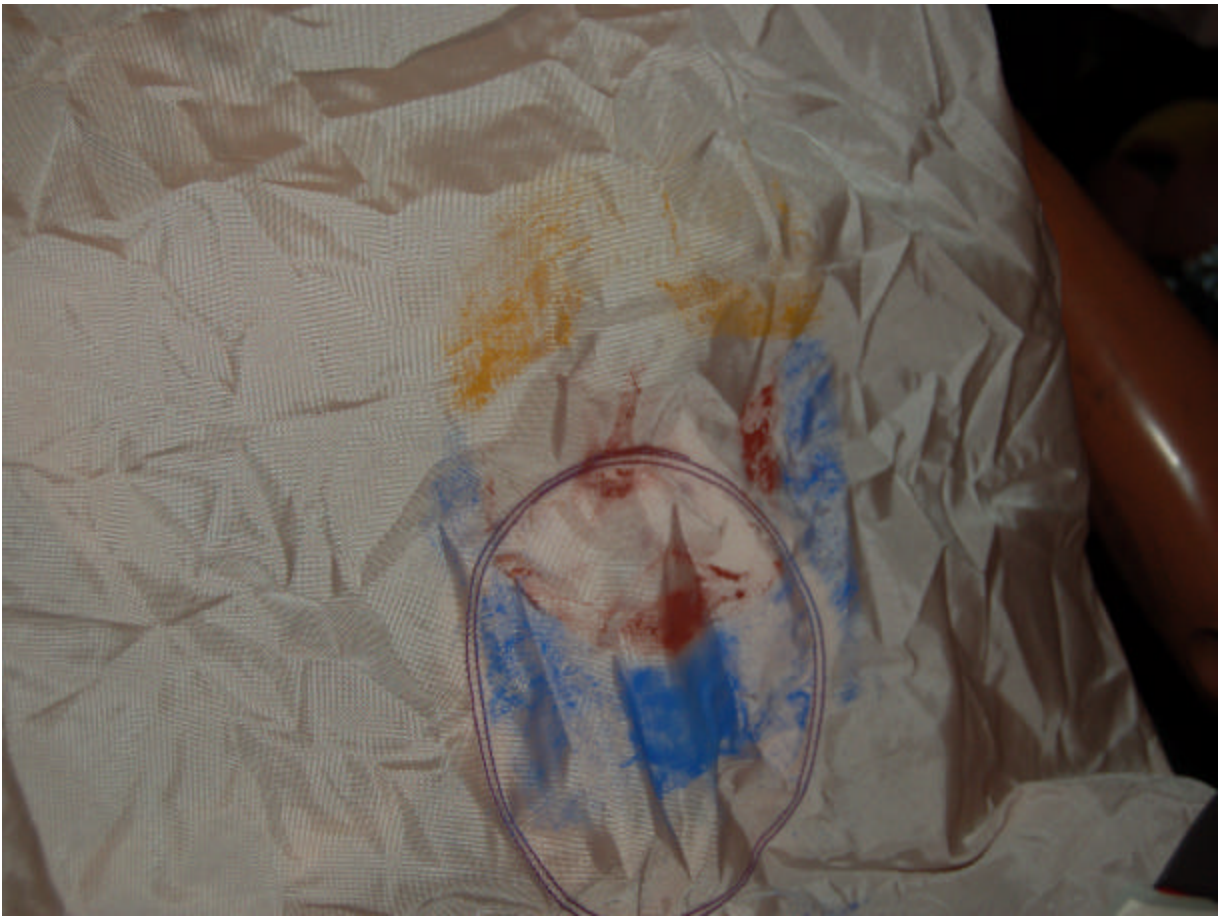
Post-Test Driver Dummy Airbag Contact
