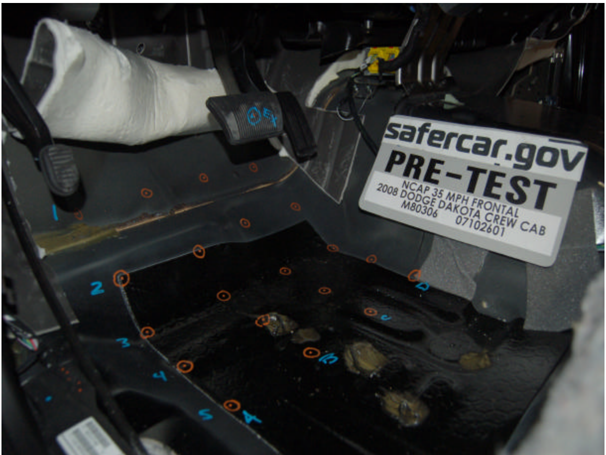
Pre-Test Driver Side Floor Pan
