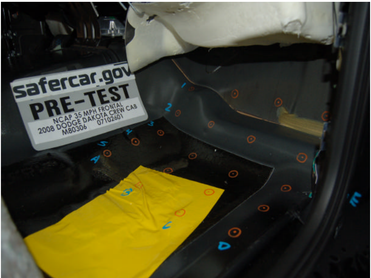
Pre-Test Passenger Side Floor Pan
