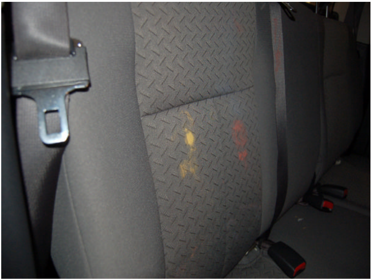
Post-Test Position 3 Foot Contact
