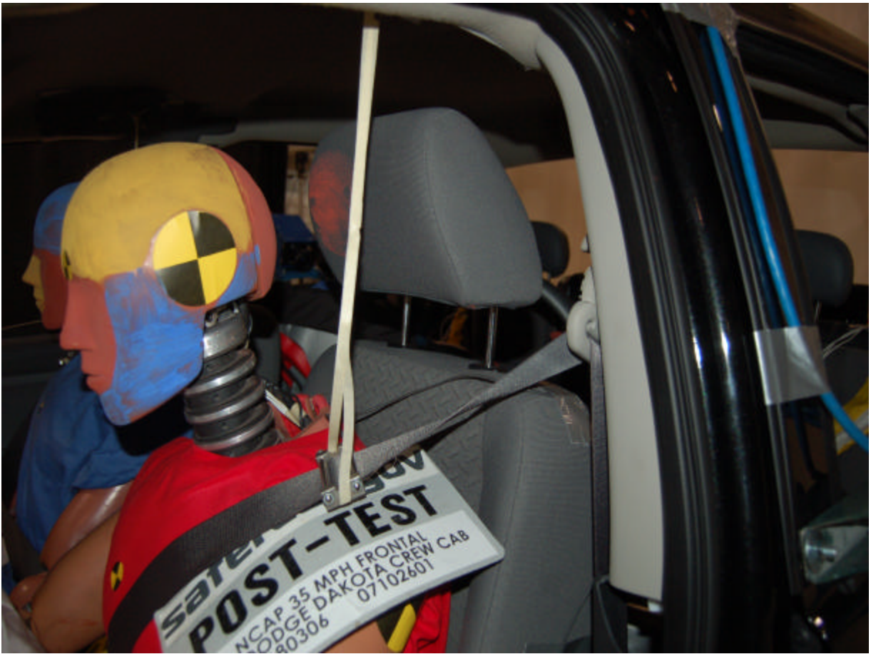
Post-Test Driver Dummy Head Contact (headrest)
