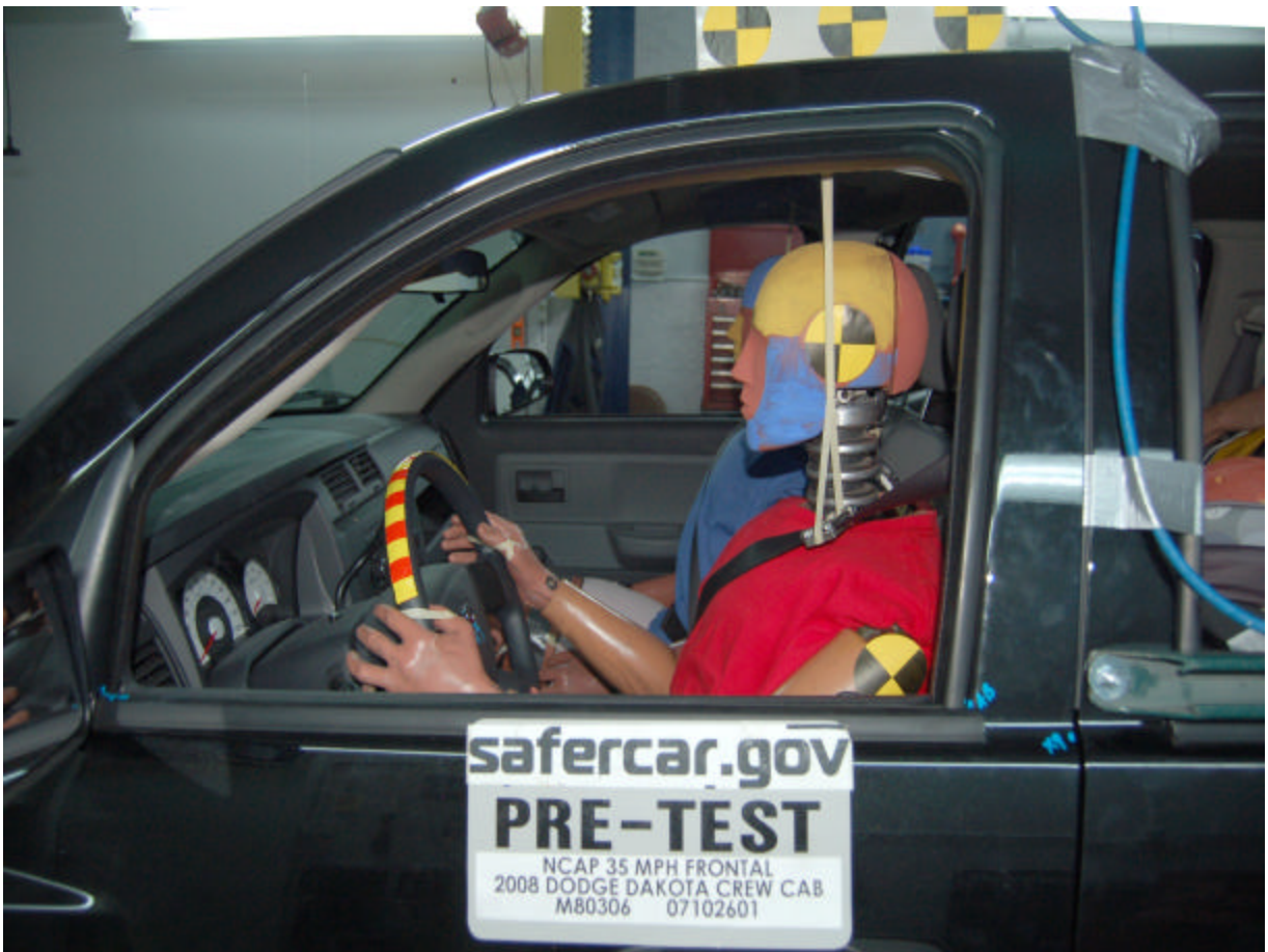
Pre-Test Driver Dummy (Through Window)
