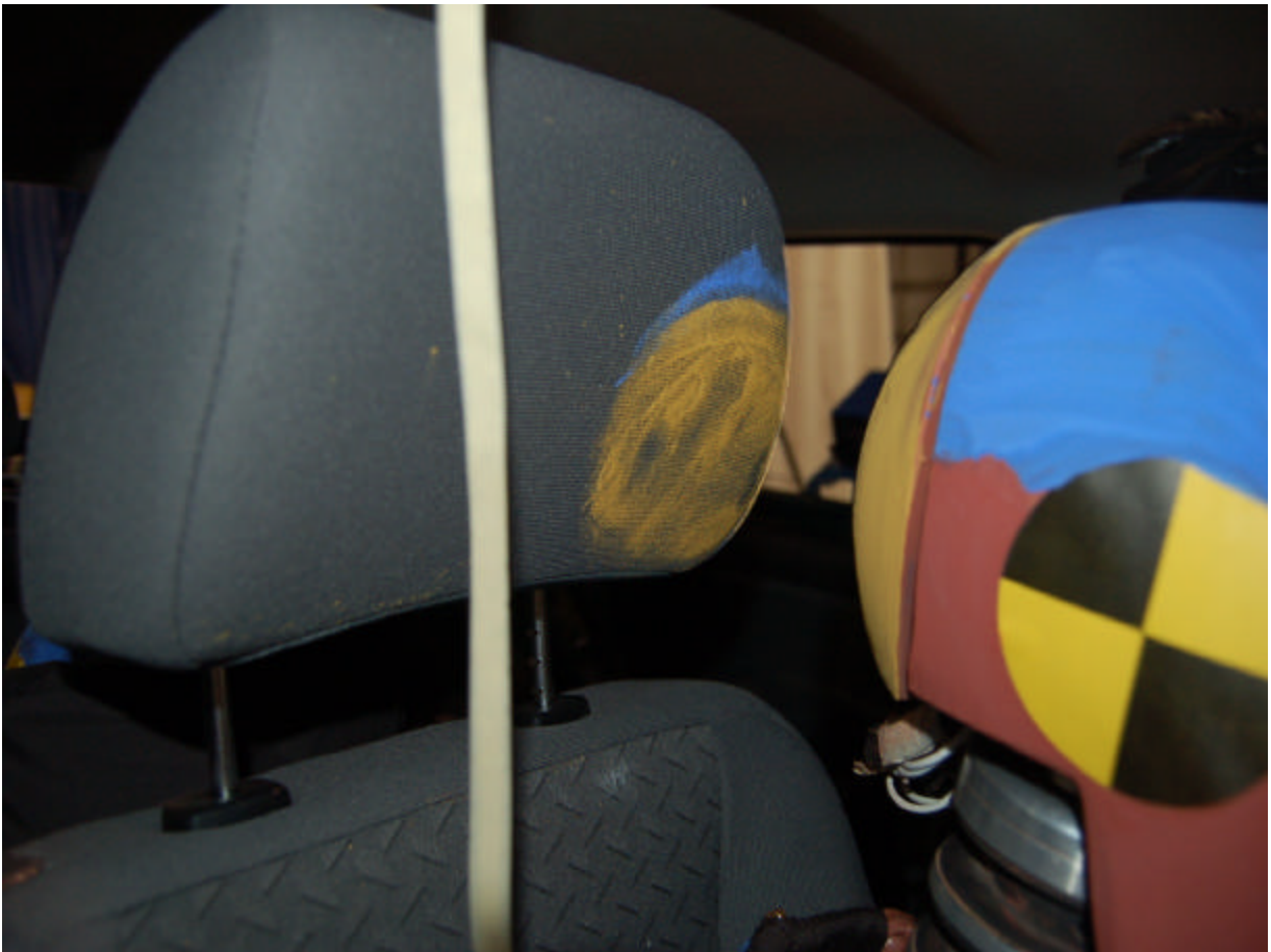
Post-Test Passenger Dummy Head Contact (headrest)
