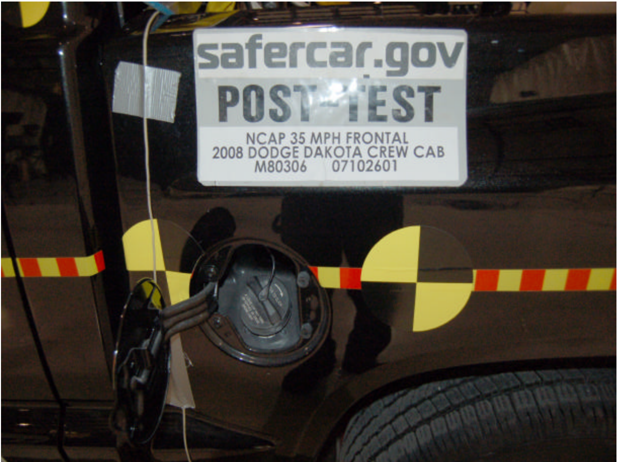
Post-Test Fuel Cap View
