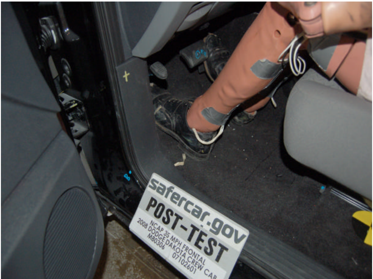
Post-Test Driver Dummy Feet
