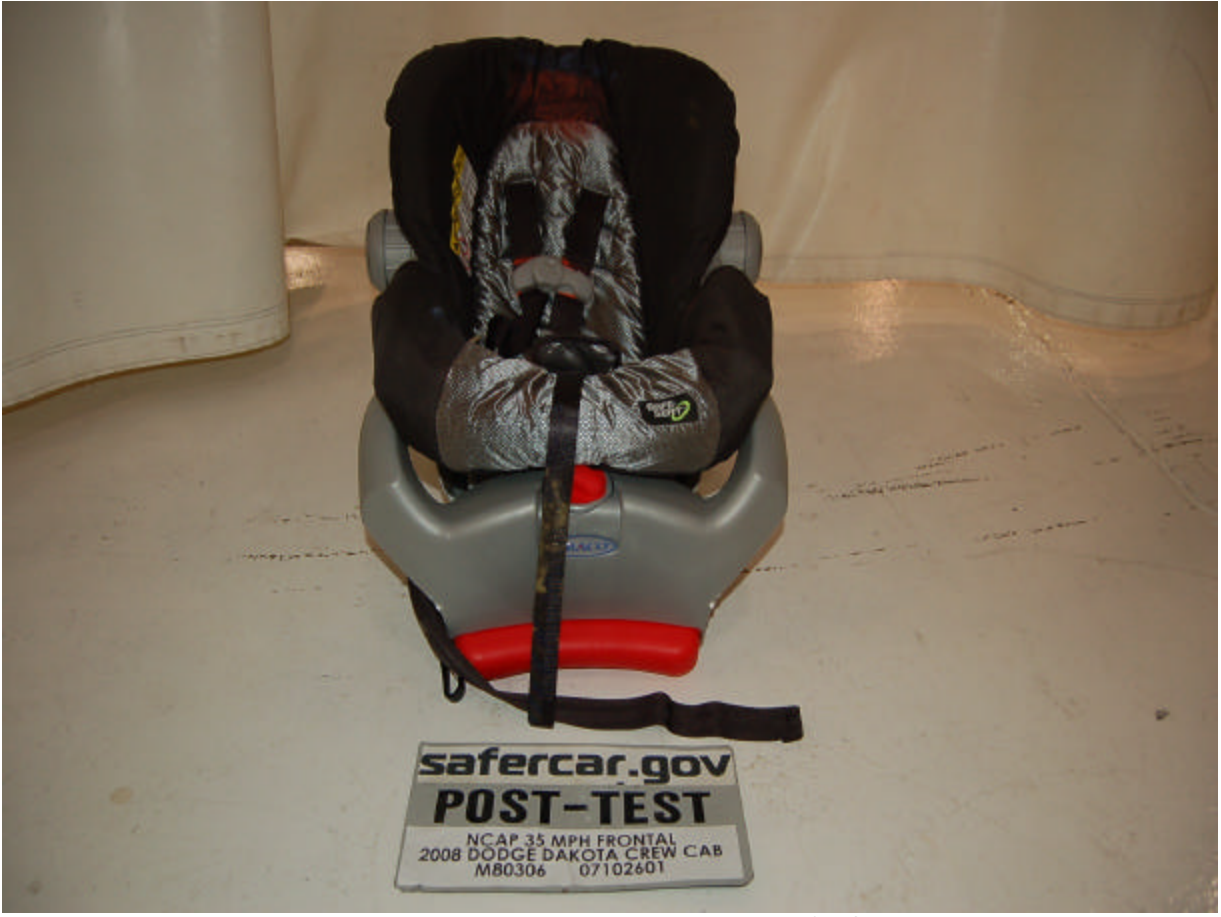
Post-Test Front View of Position 3 CRS
