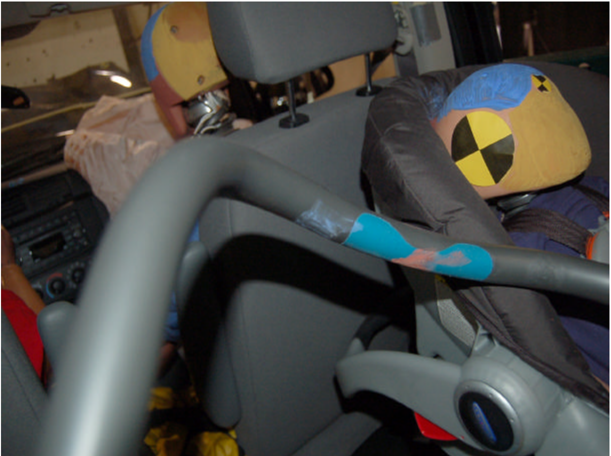
Post-Test Position 4 Foot Contact (Handle of CRS)
