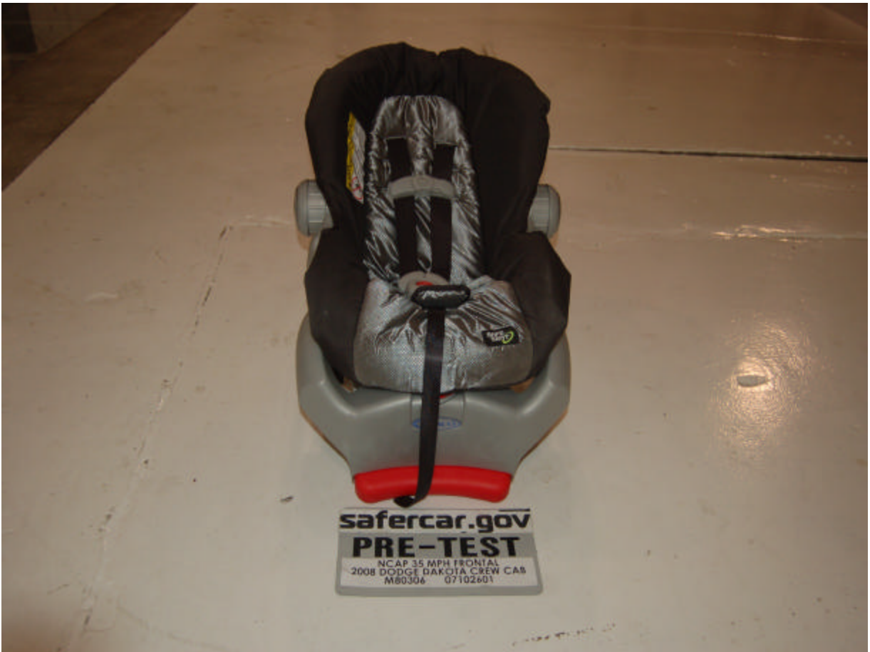
Pre-Test Front View of Position 3 CRS
