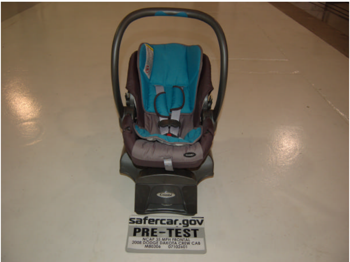
Pre-Test Front View of Position 4 CRS
