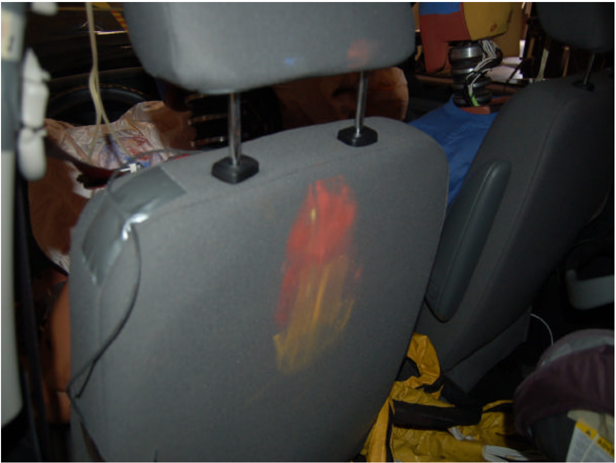
Post-Test Position 4 Head Contact (Driver Seatback)
