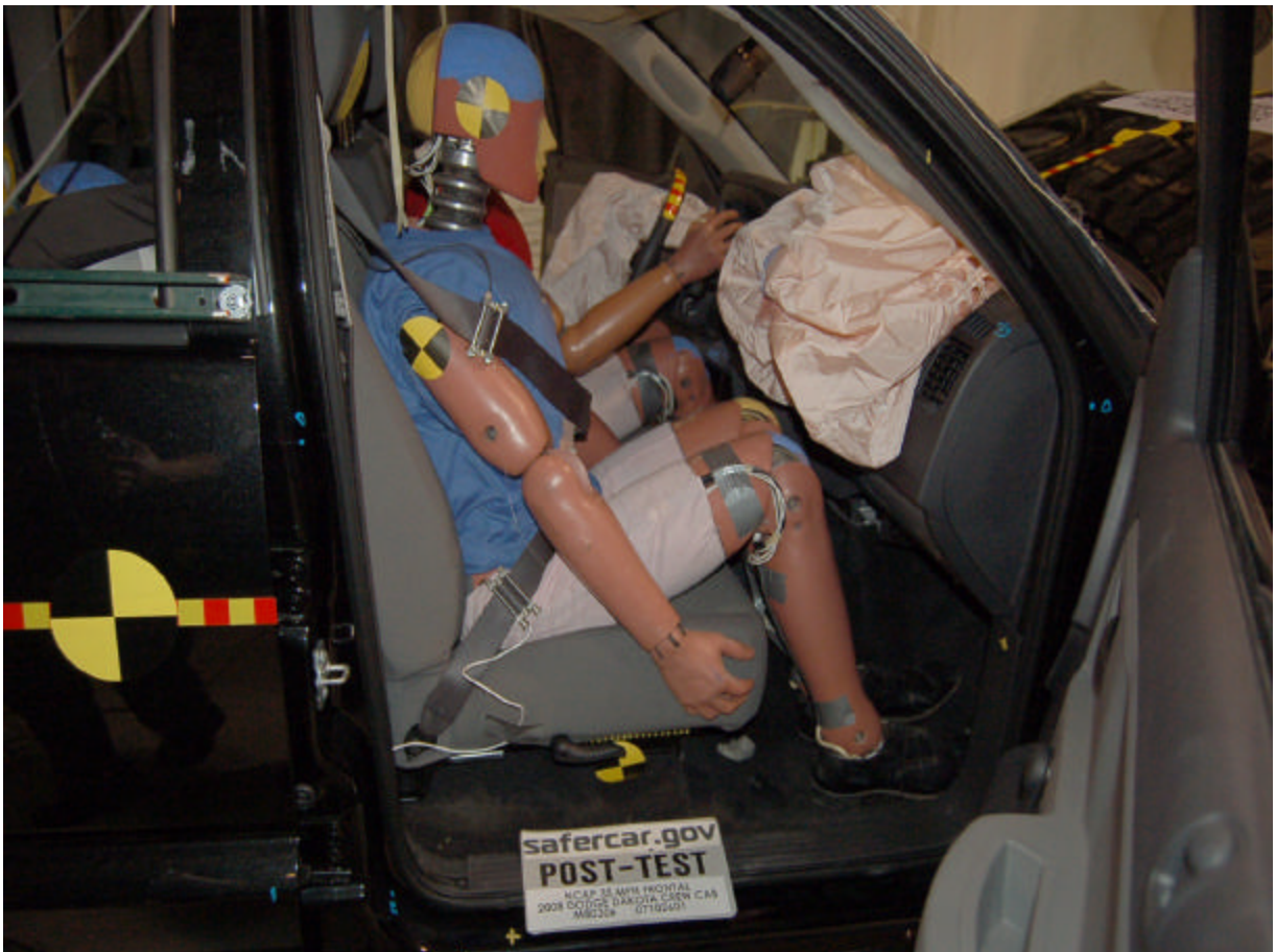
Post-Test Passenger Dummy (Door Open)
