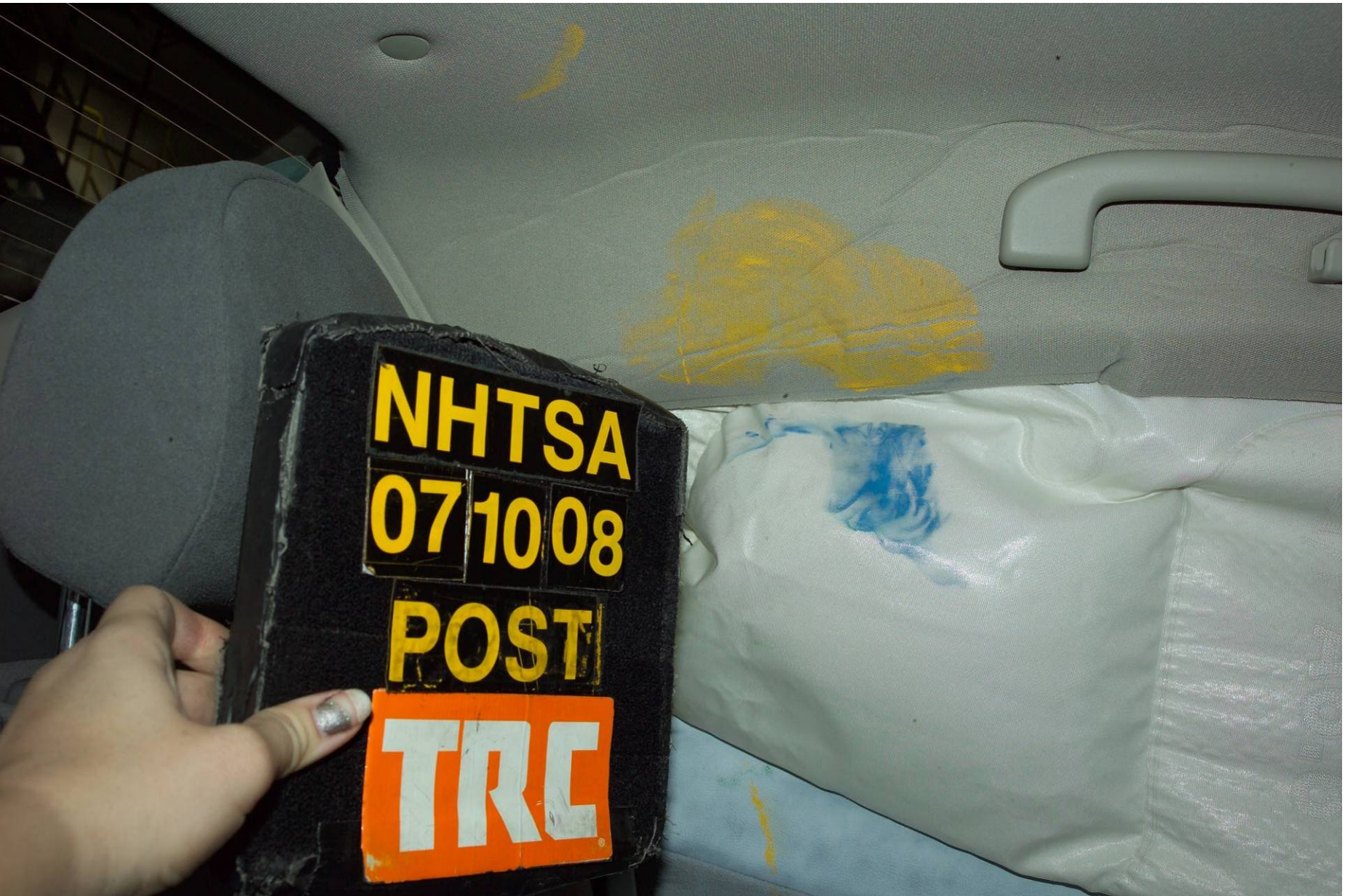
Figure A-66 Post-Test Rear SID Contact – View 1
