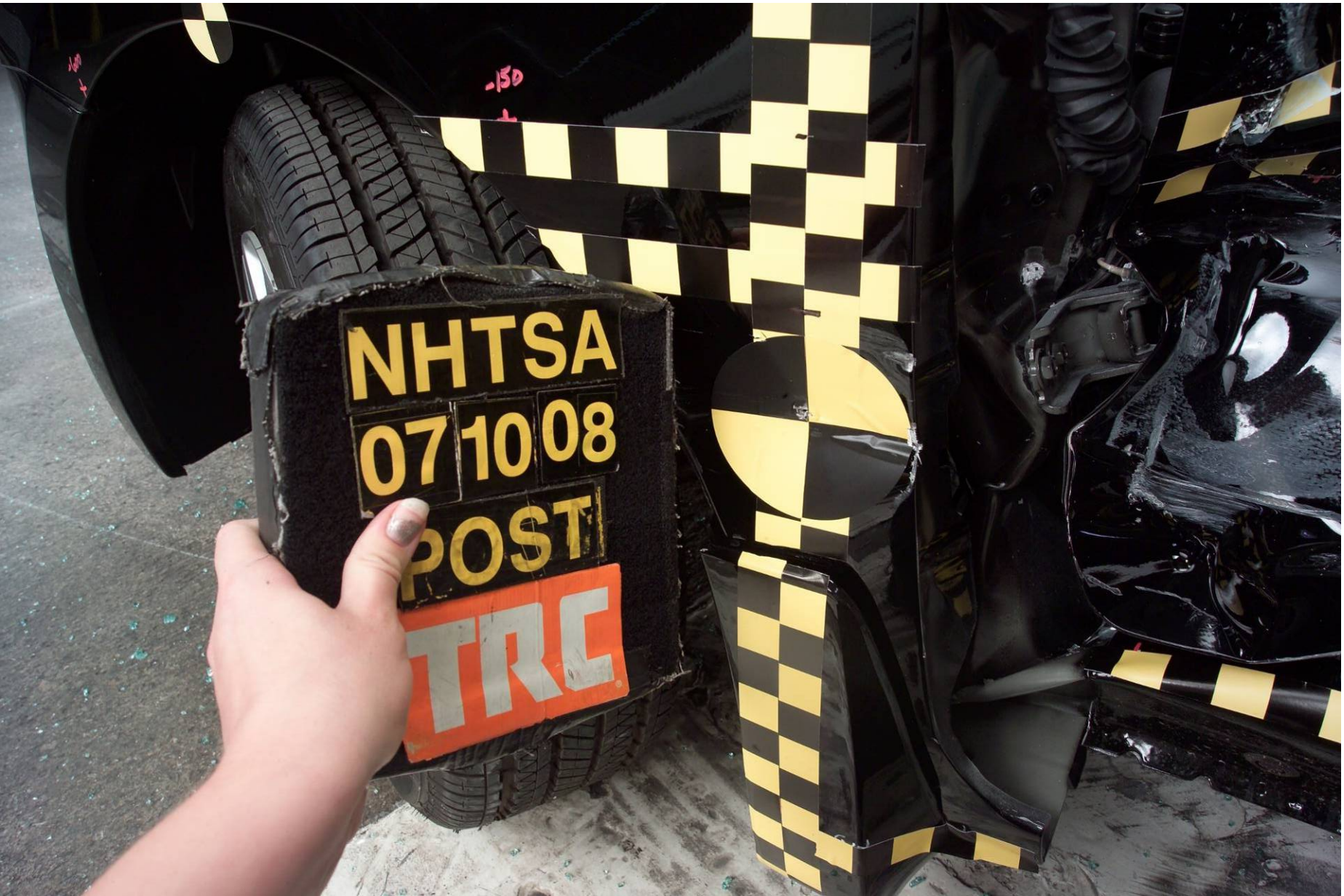
Figure A-70 Post-Test Primary Impact Point View
