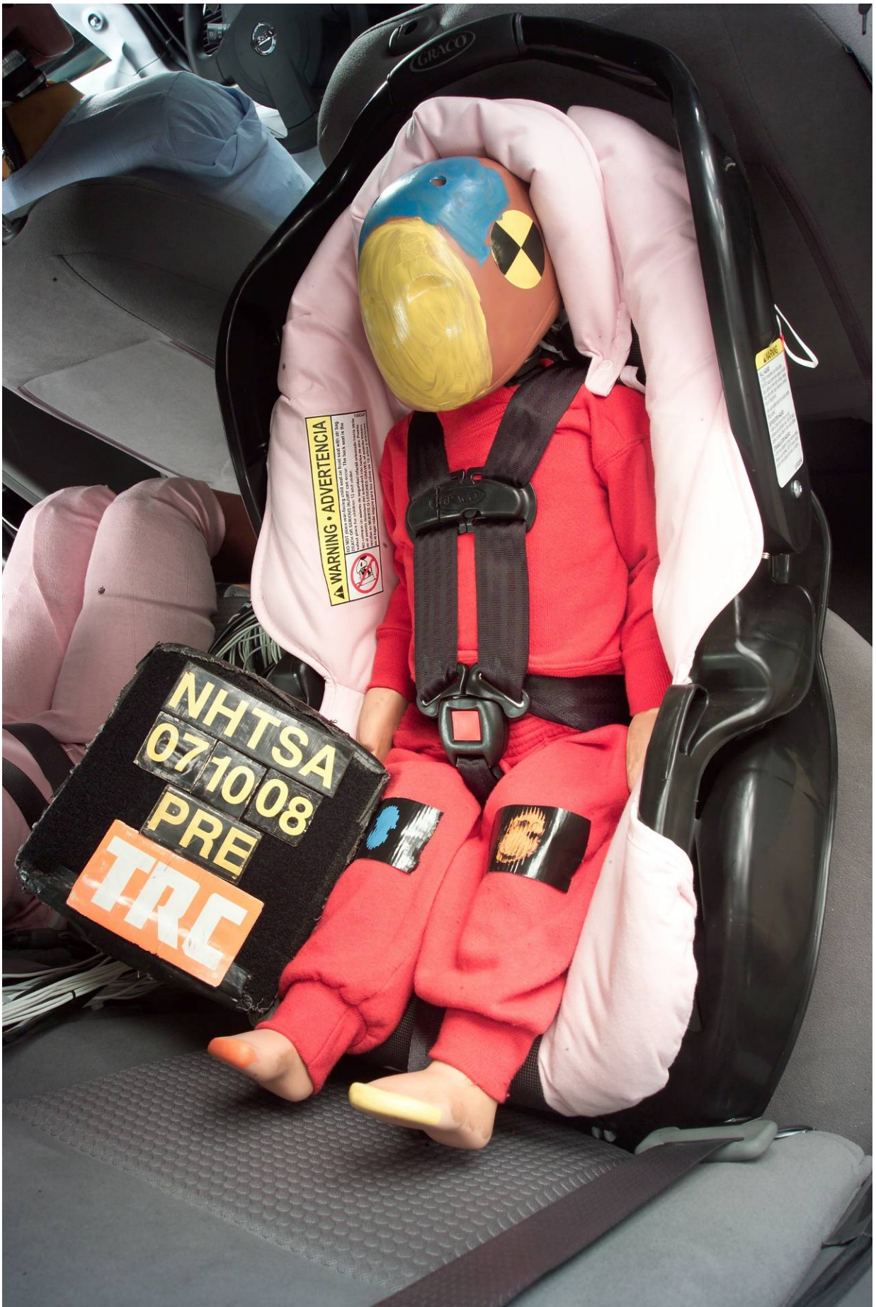
Figure D-1 Pre-Test Front View of Right Rear Dummy
