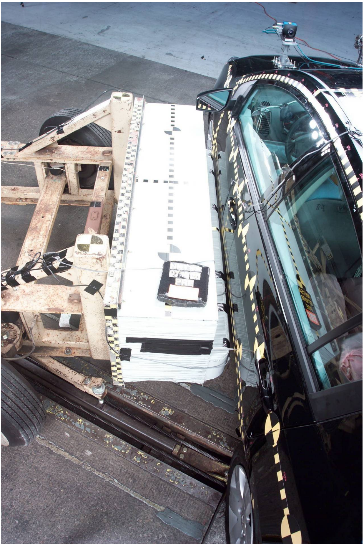
Figure A-74 Pre-Test Overhead View of MDB with Impactor Face in Position
