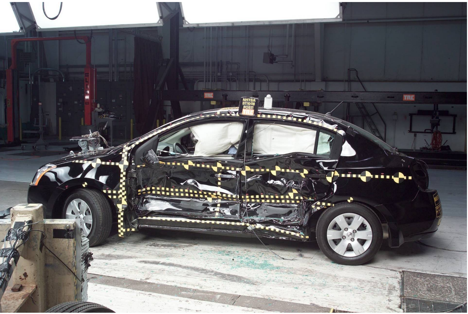
Figure A-10 Post-Test Impacted Side View of Test Vehicle
