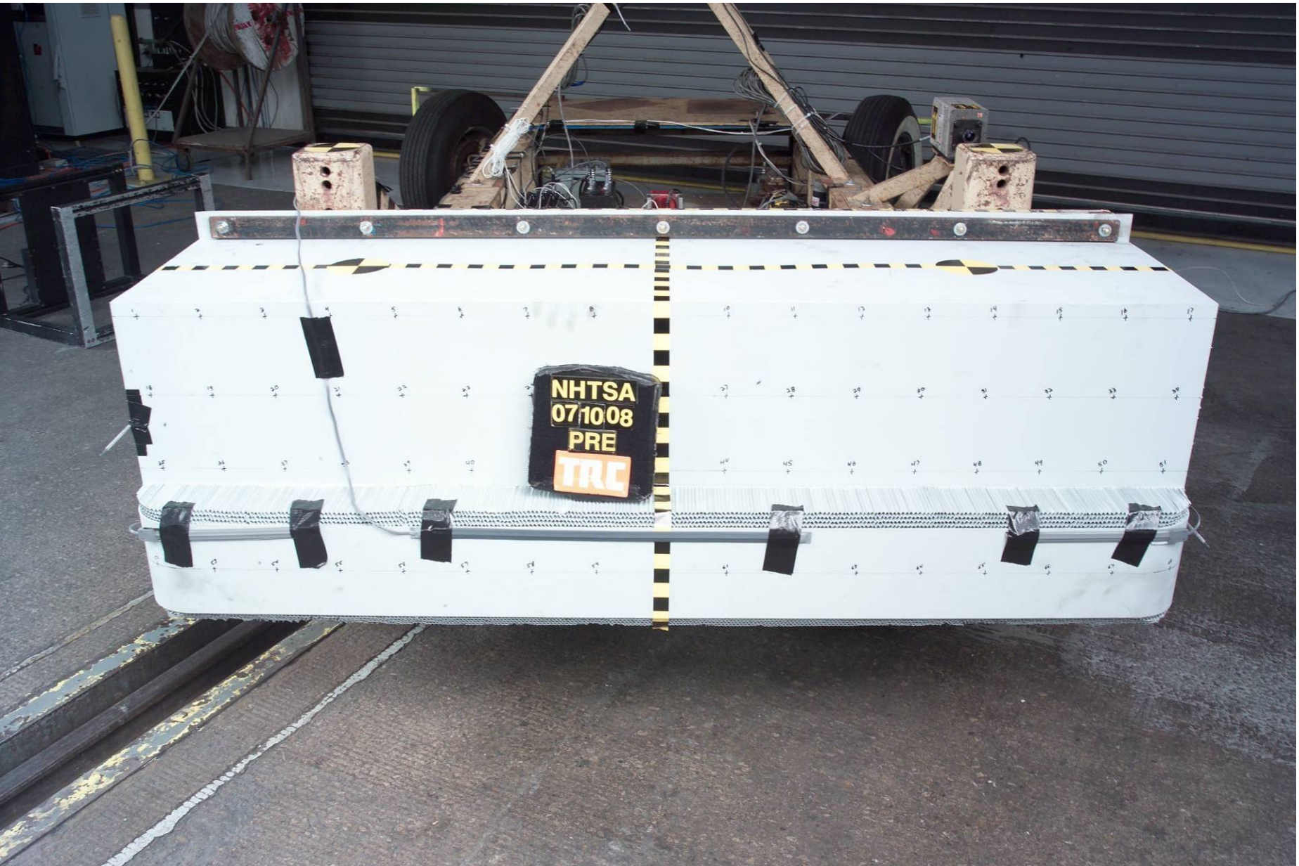
Figure A-42 Pre-Test View of MDB Showing Contact Switches in Place
