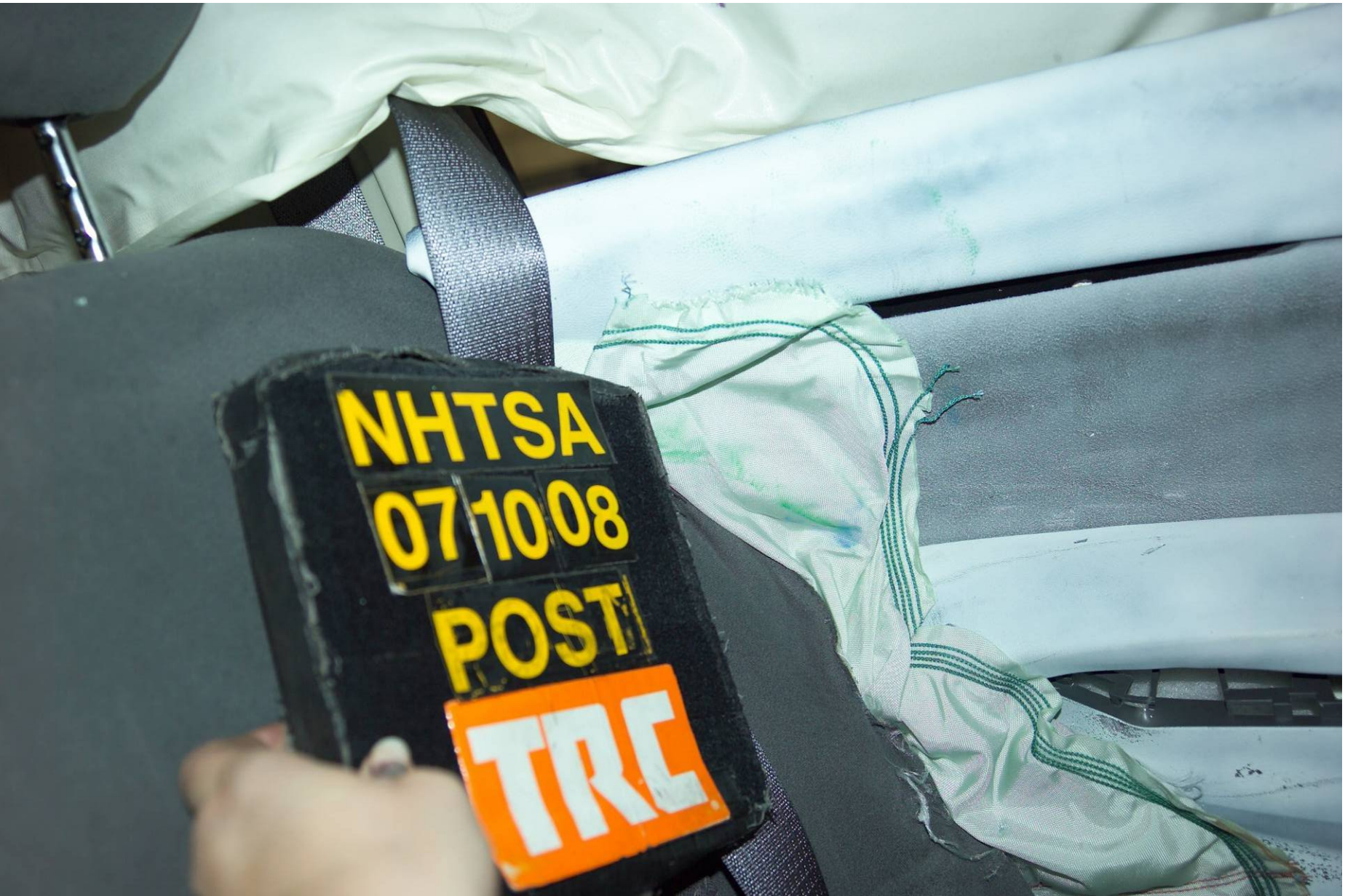
Figure A-63 Post-Test Front SID Contact – View 2
