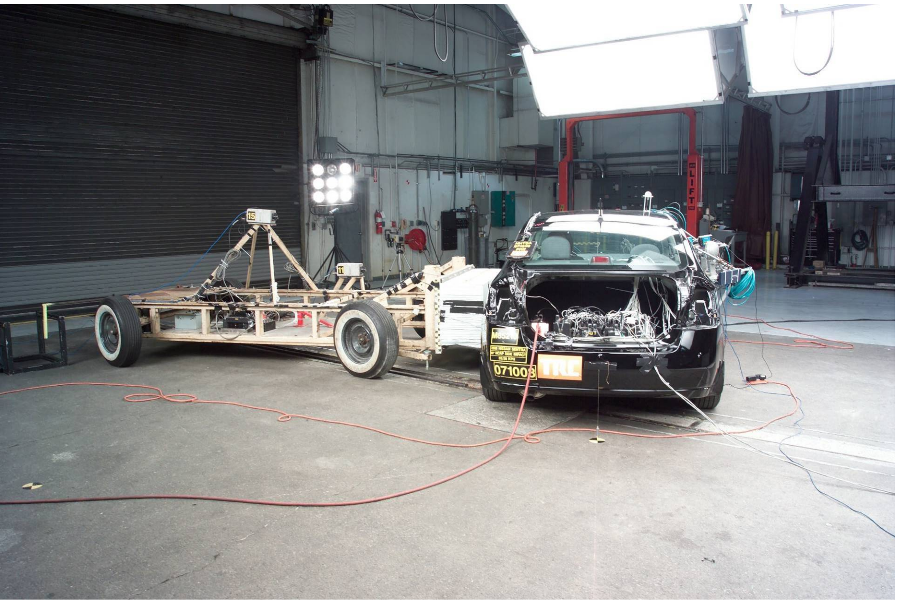
Figure A-71 Pre-Test Right Side View of MDB with Impactor Face in Position
