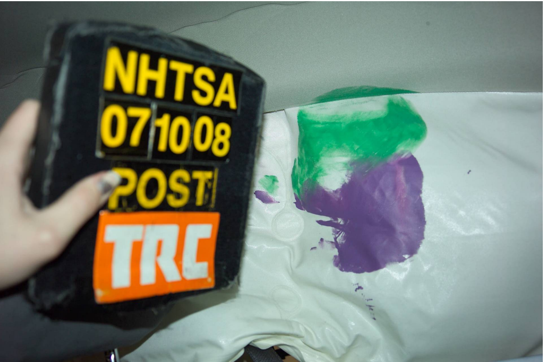
Figure A-62 Post-Test Front SID Contact – View 1
