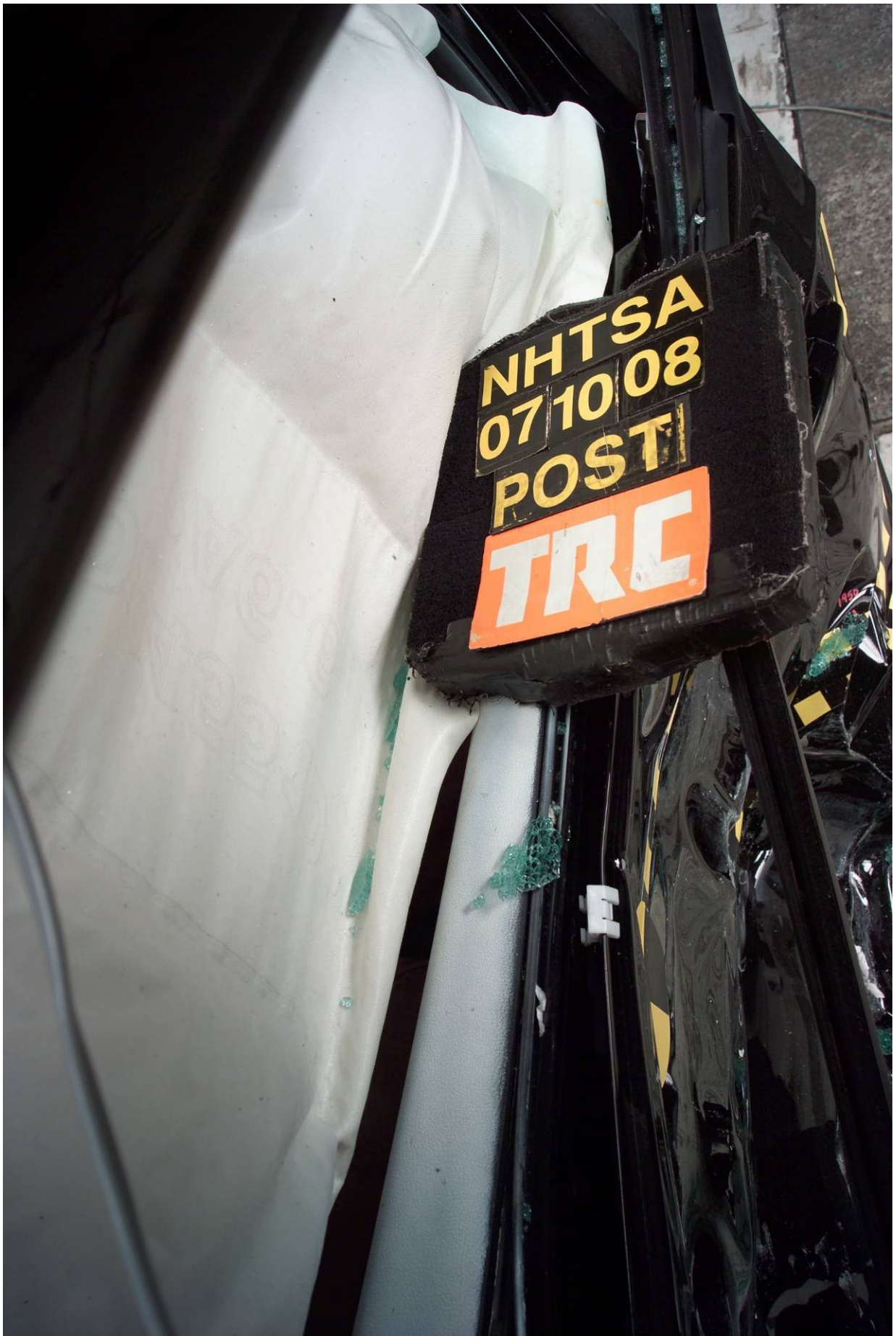
Figure A-59 Post-Test Left View of Rear SID and Door Clearance
