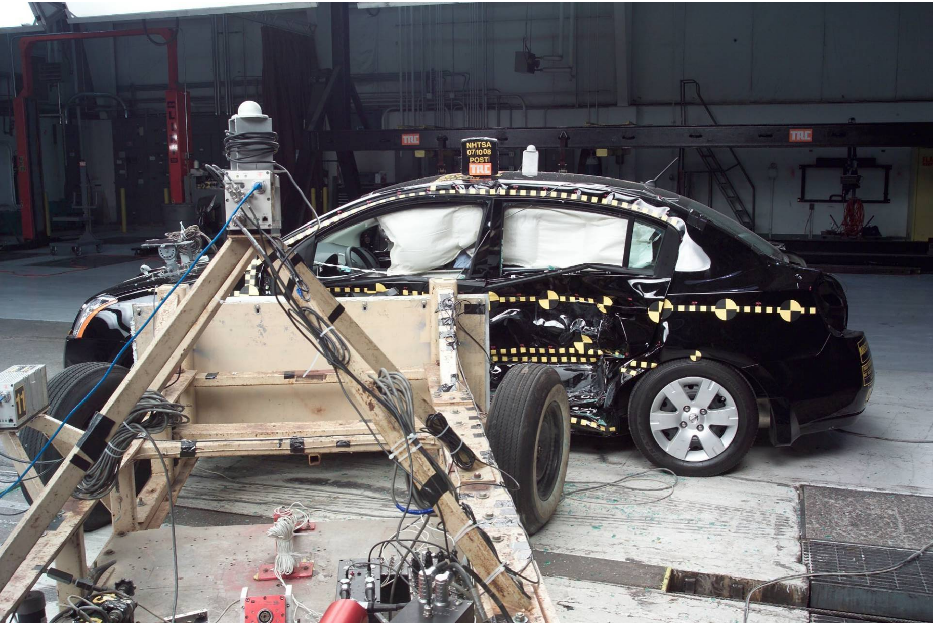
Figure A-8 Post-Test Impacted Side View of Test Vehicle with Barrier
