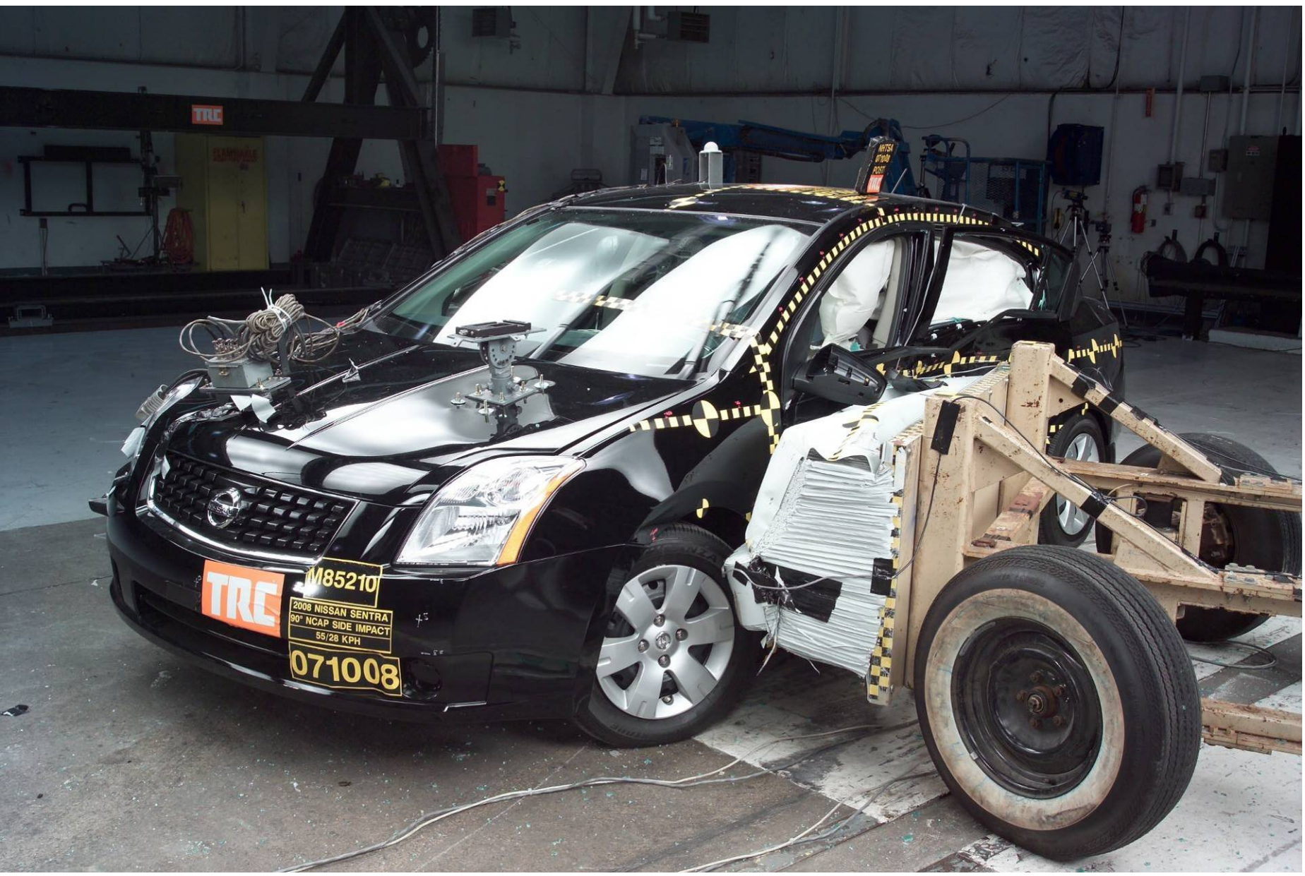
Figure A-4 Post-Test Left Front View of Test Vehicle with Barrier
