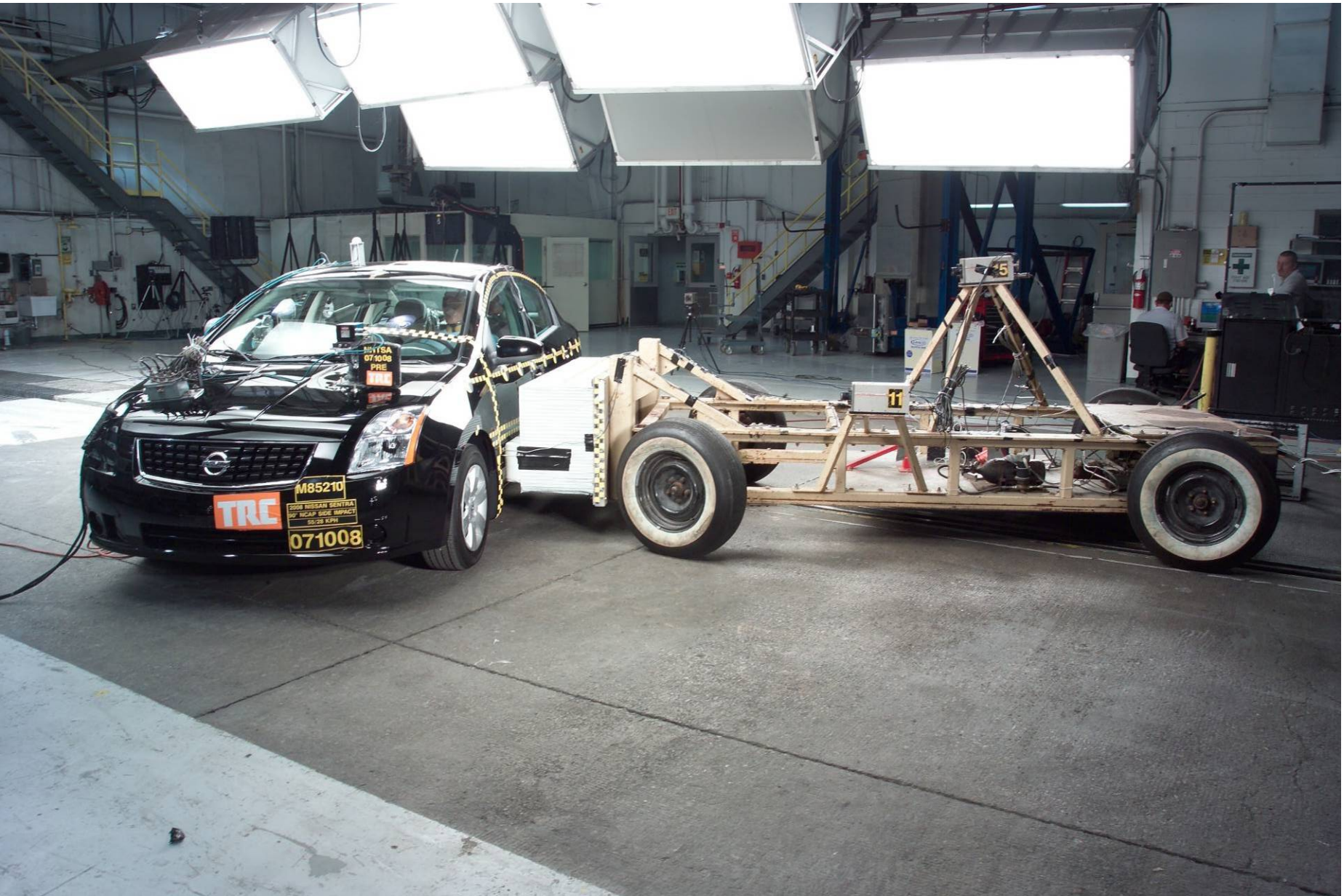
Figure A-68 Pre-Test Left Side View of MDB with Impactor Face in Position
