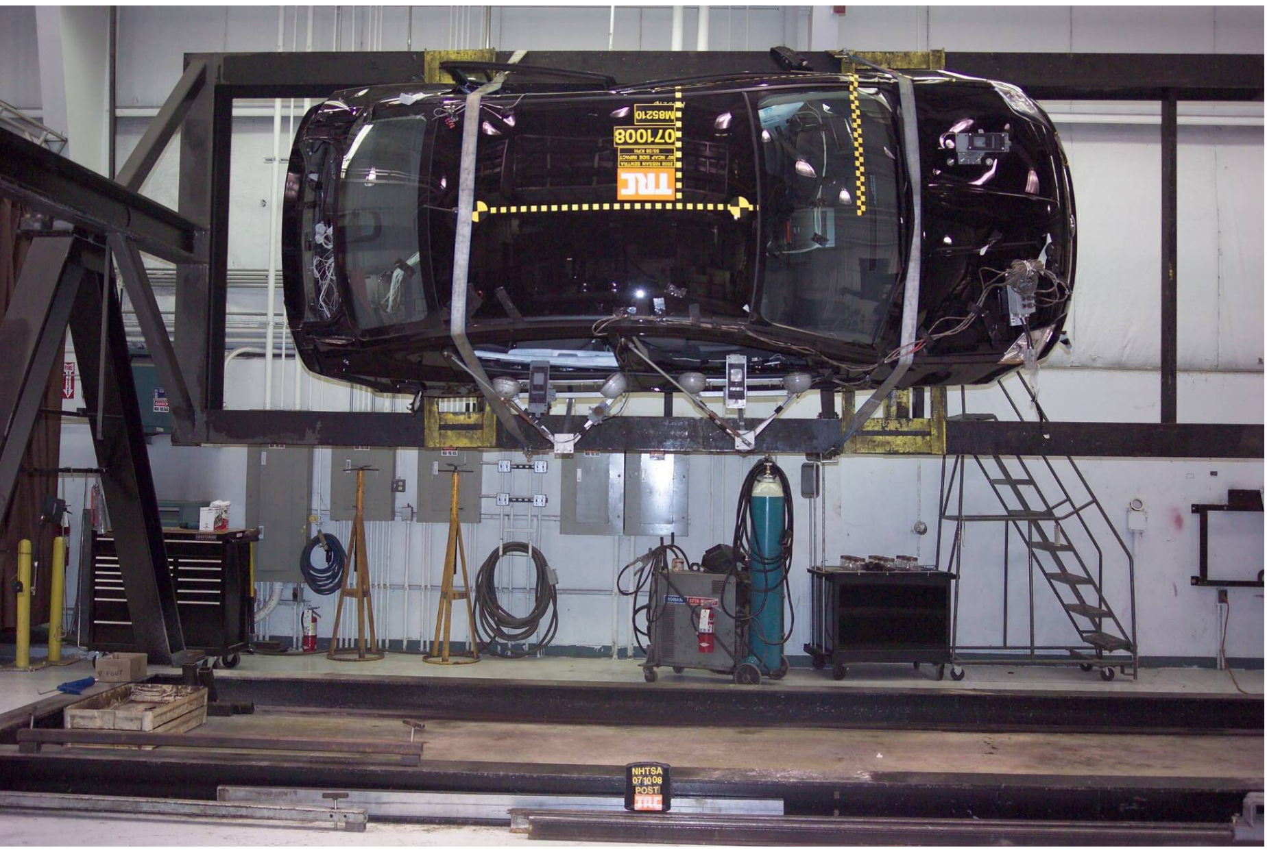
Figure A-82 FMVSS 301 Rollover View at 90°
