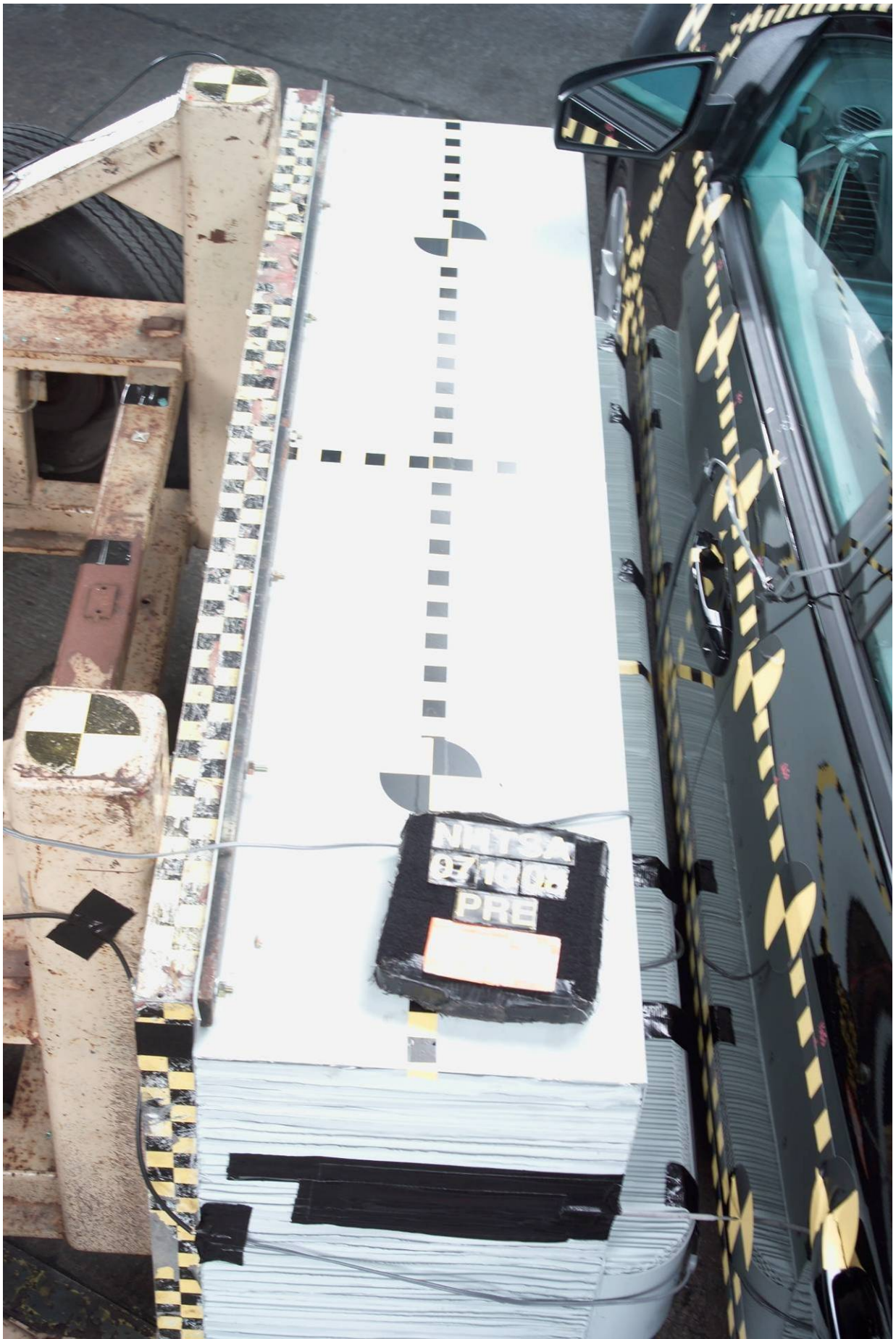
Figure A-44 Pre-Test Overhead View of MDB Aligned with Vehicle
