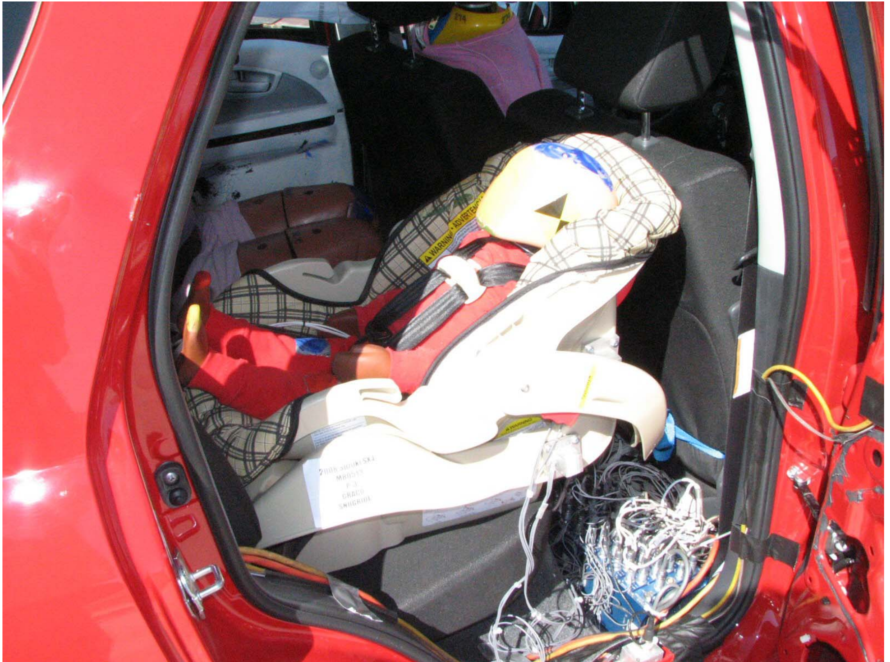
Figure D2-15: Post-Test Position 3 Right Side View
