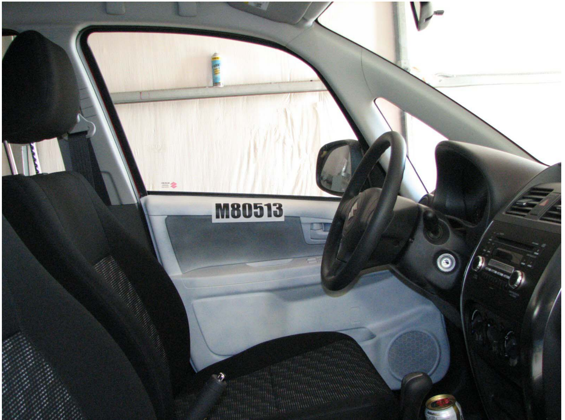
Figure A-42: Pre-Test Front Door Panel (Interior)
