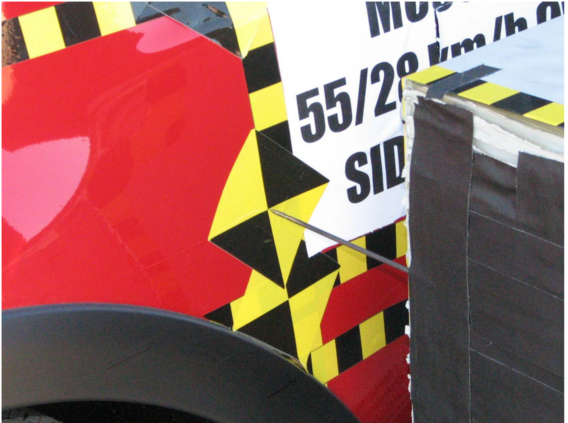
Figure A-25: Pre-Test Left Impact Point
