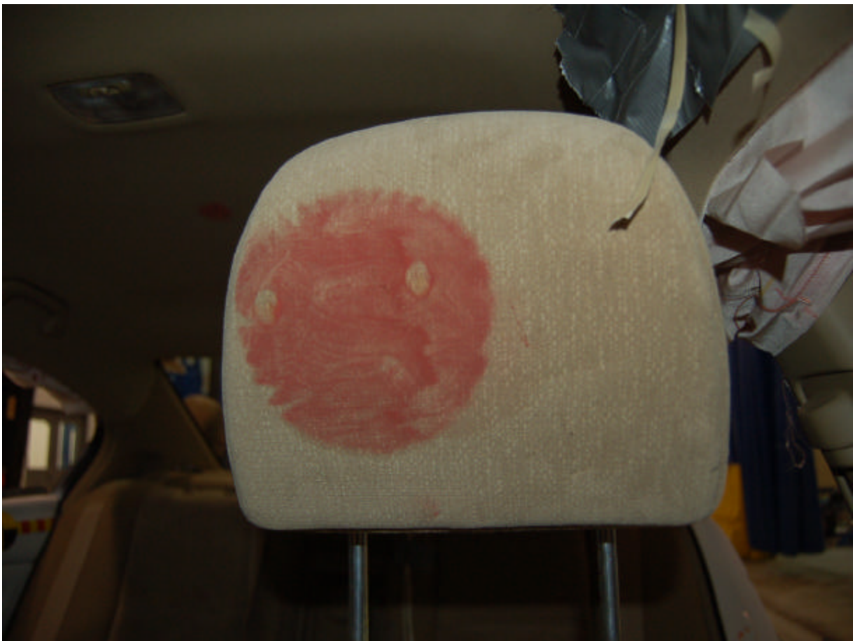
Post-Test Driver Dummy Head Contact (headrest)
