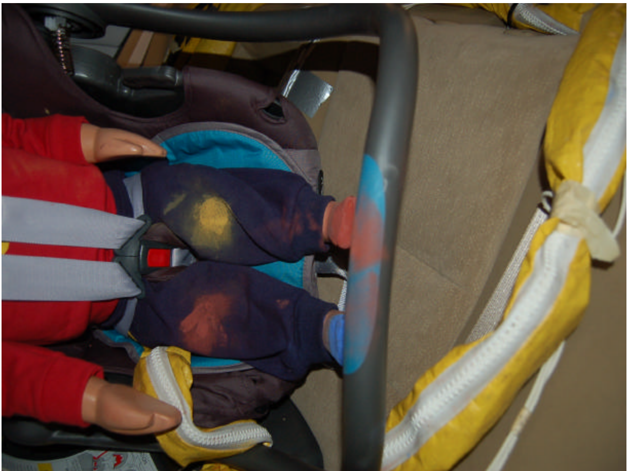
Post-Test Position 4 Head Contact (Handle of CRS)
