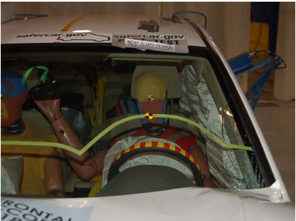
Post-Test Driver Dummy Front View (Head Position)
