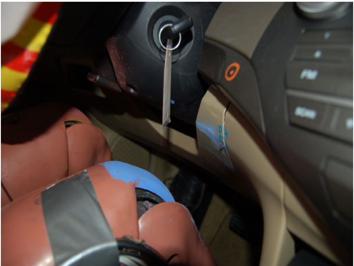
Post-Test Driver Dummy Right Knee Contact
