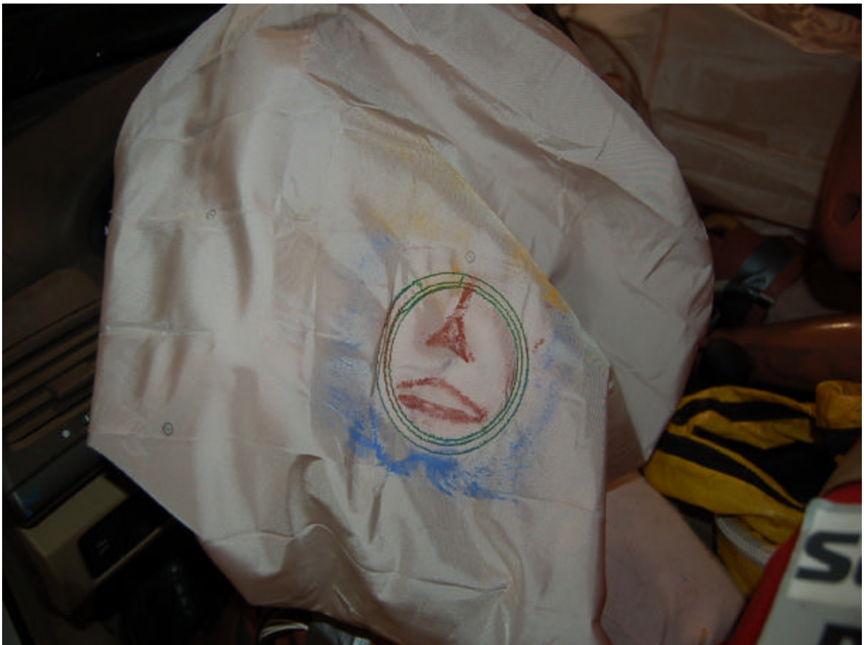
Post-Test Driver Dummy Airbag Contact
