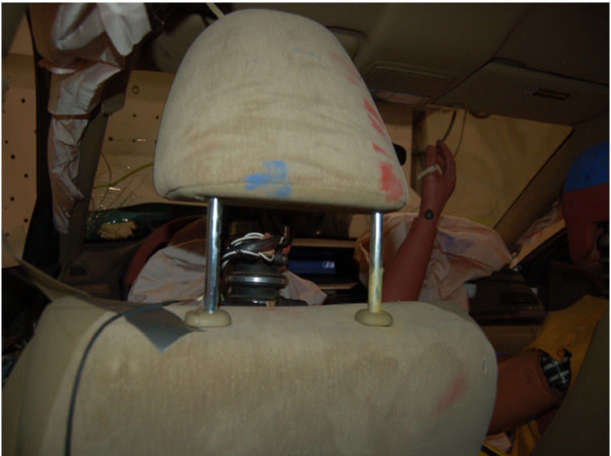
Post-Test Position 4 Foot Contact (Driver Headrest)
