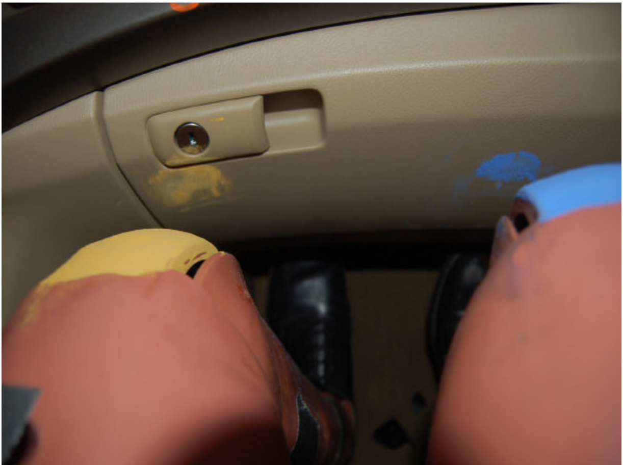
Post-Test Passenger Dummy Knee Contact
