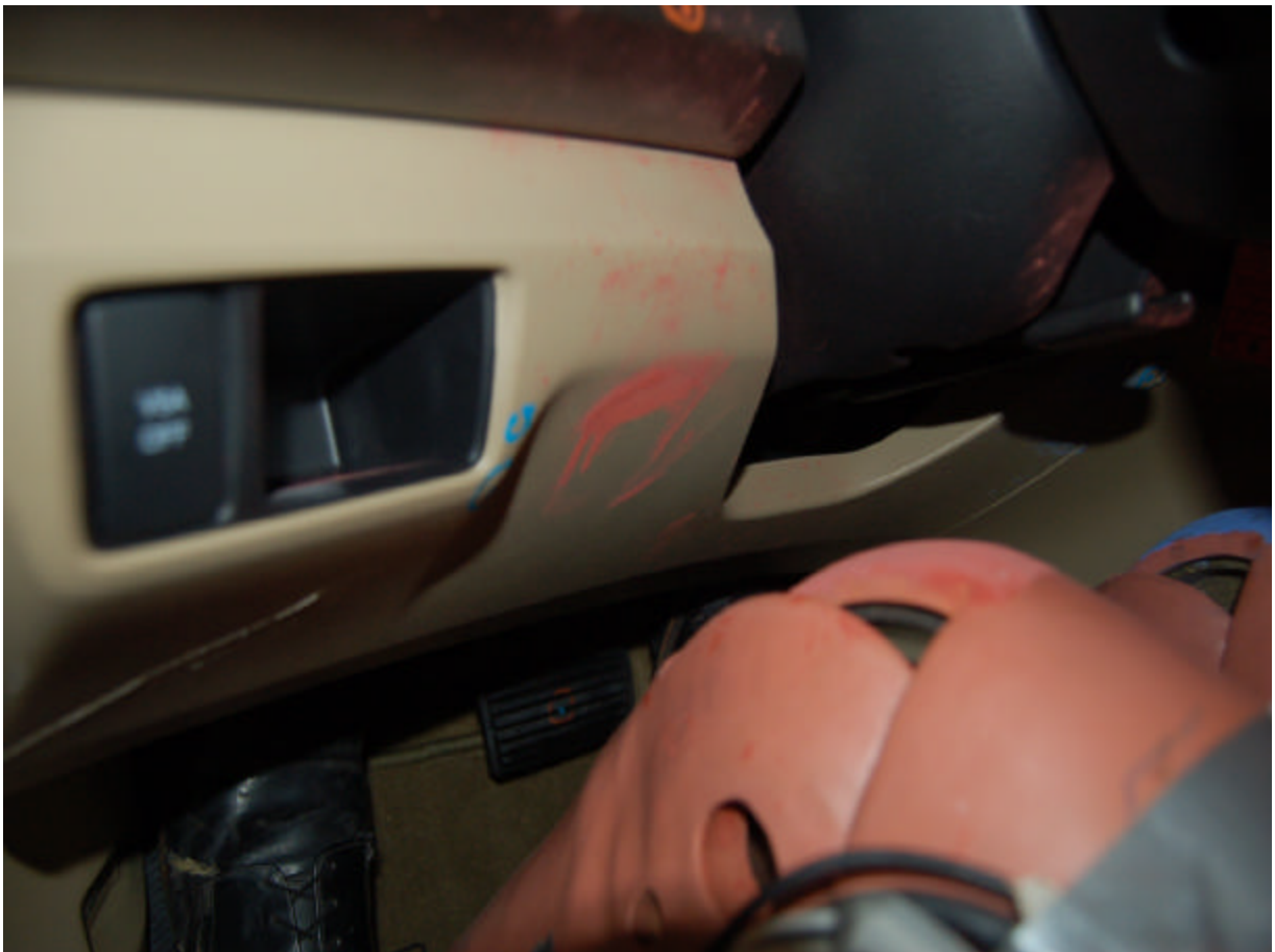
Post-Test Driver Dummy Left Knee Contact
