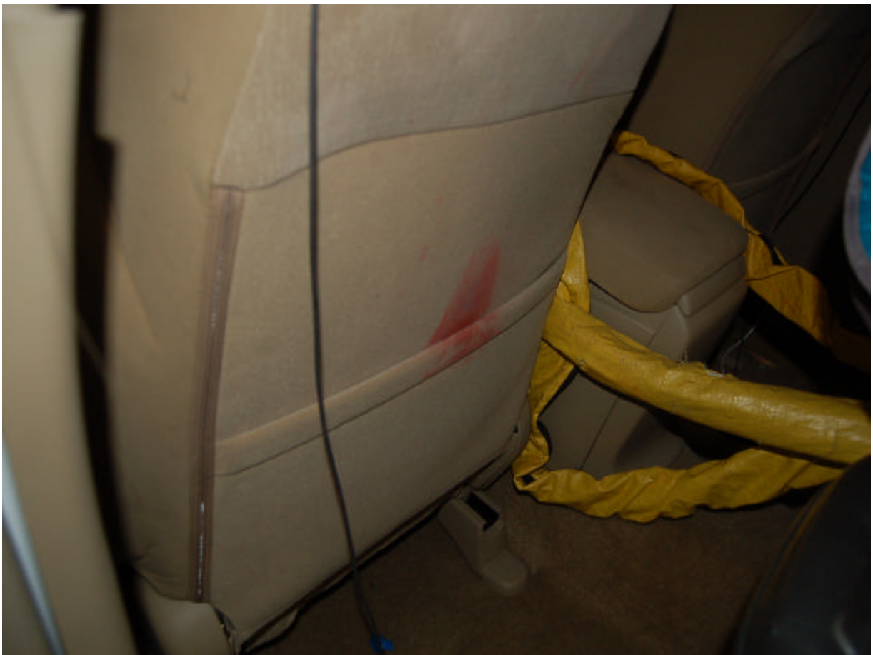
Post-Test Position 4 Head Contact (Driver Seatback)
