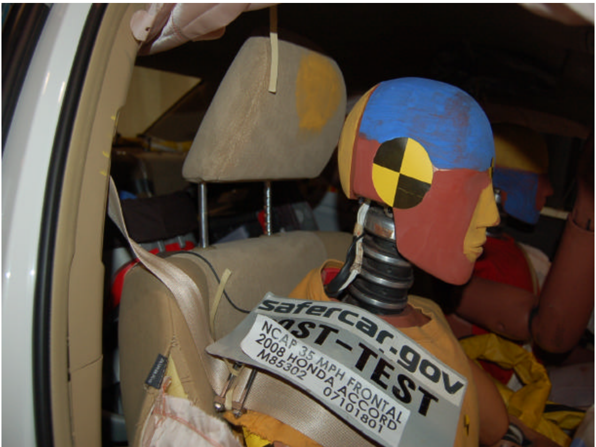
Post-Test Passenger Dummy Head Contact (headrest)
