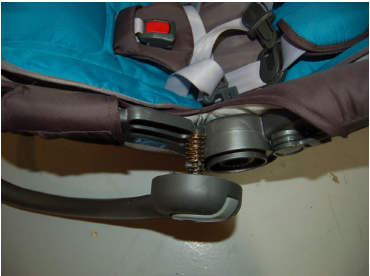
Post-Test Position 4 CRS Damage
