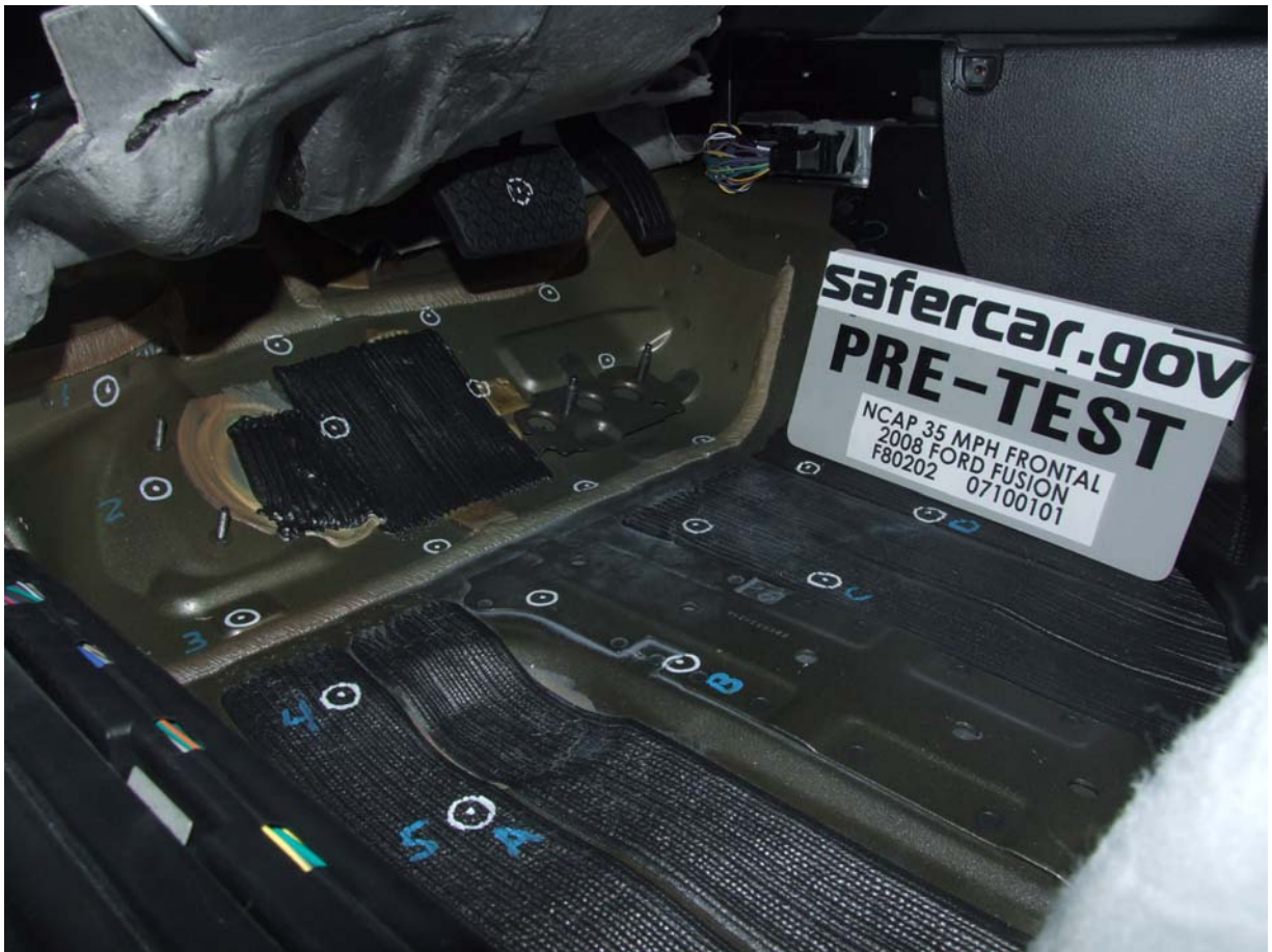
Pre-Test Driver Side Floor Pan
