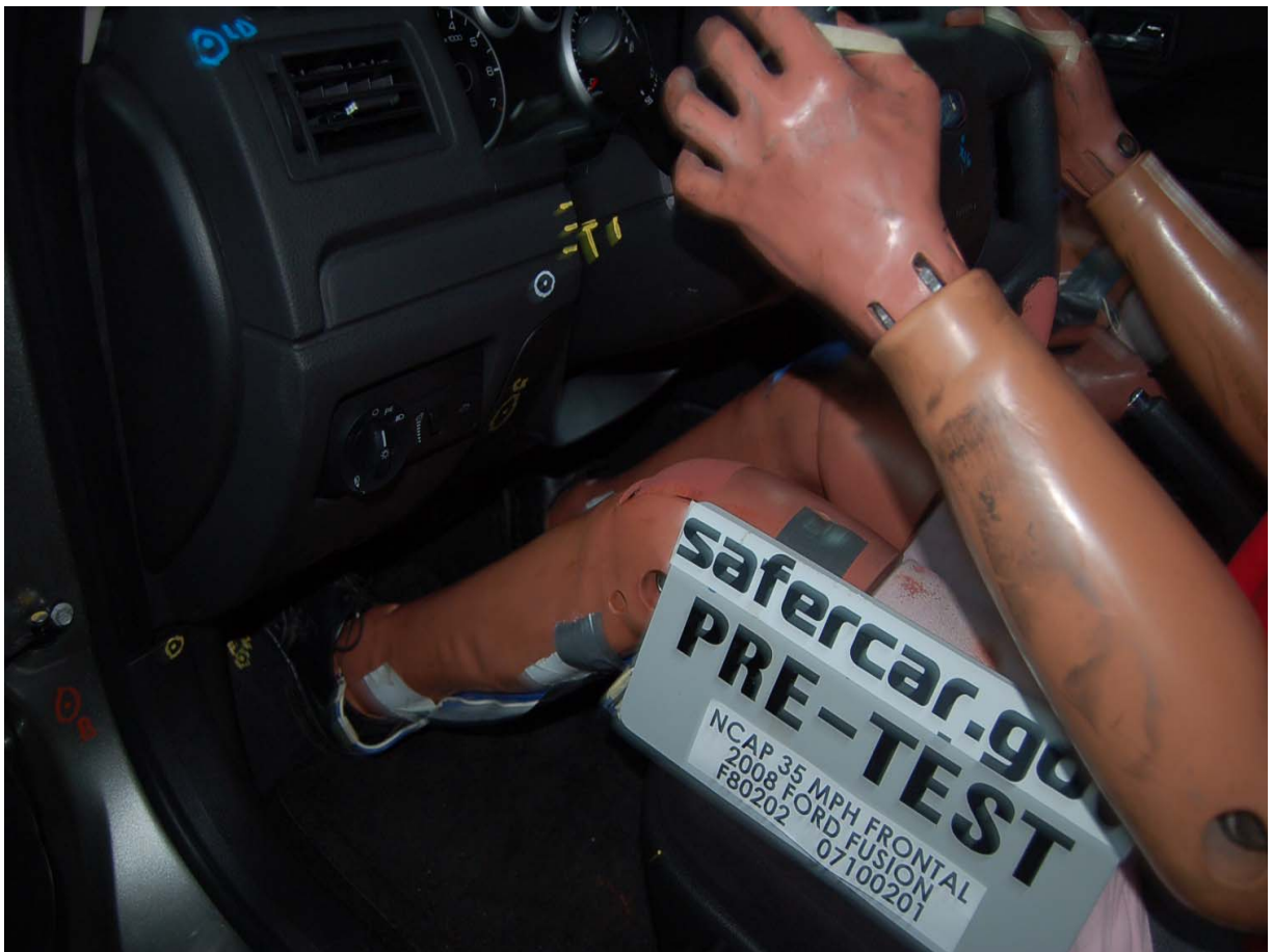
Pre-Test Driver Side Knee Bolster
