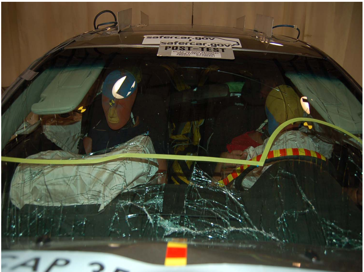
Post-Test Windshield View
