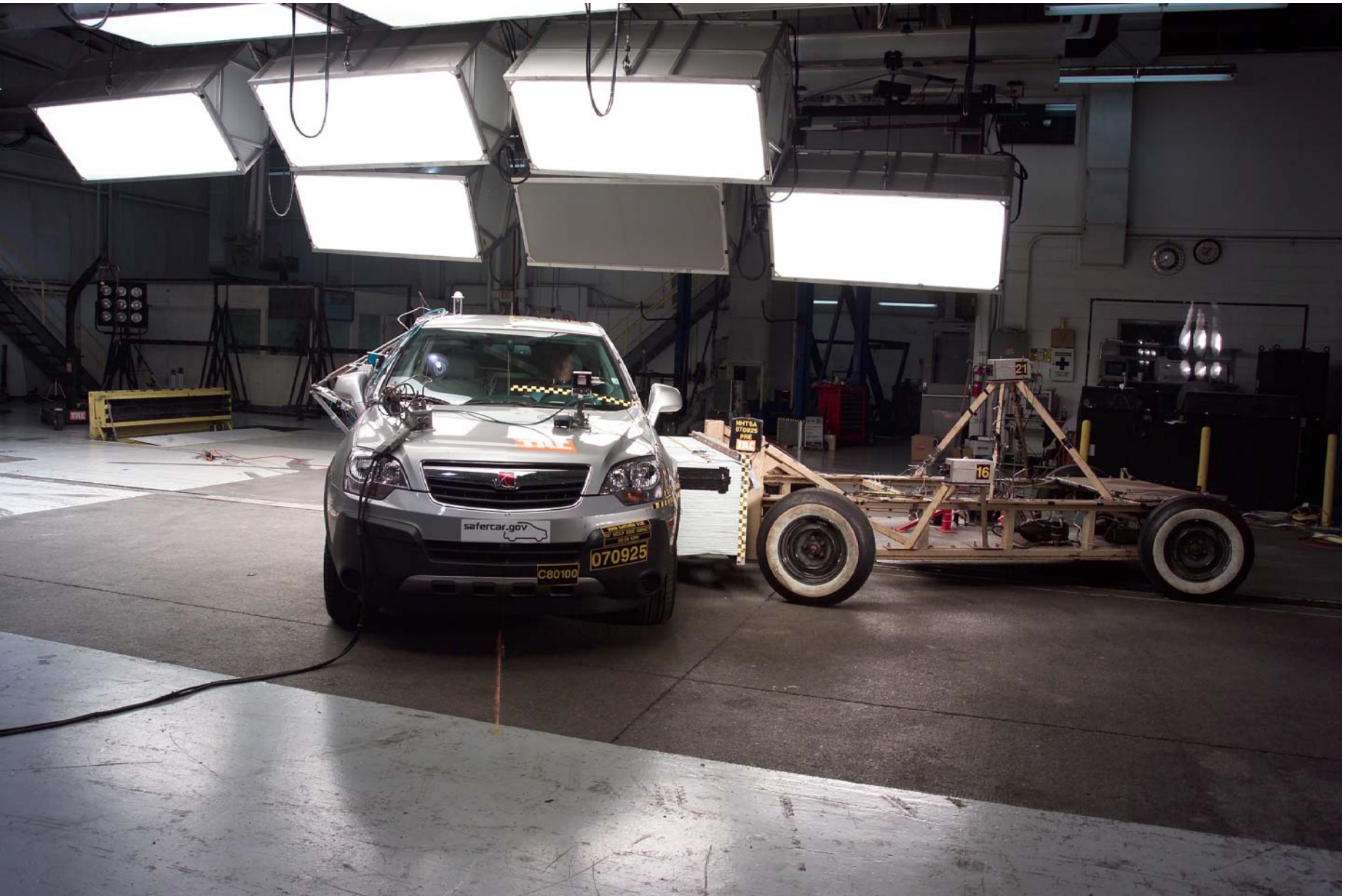
Figure A-64 Pre-Test Left Side View of MDB with Impactor Face in Position
