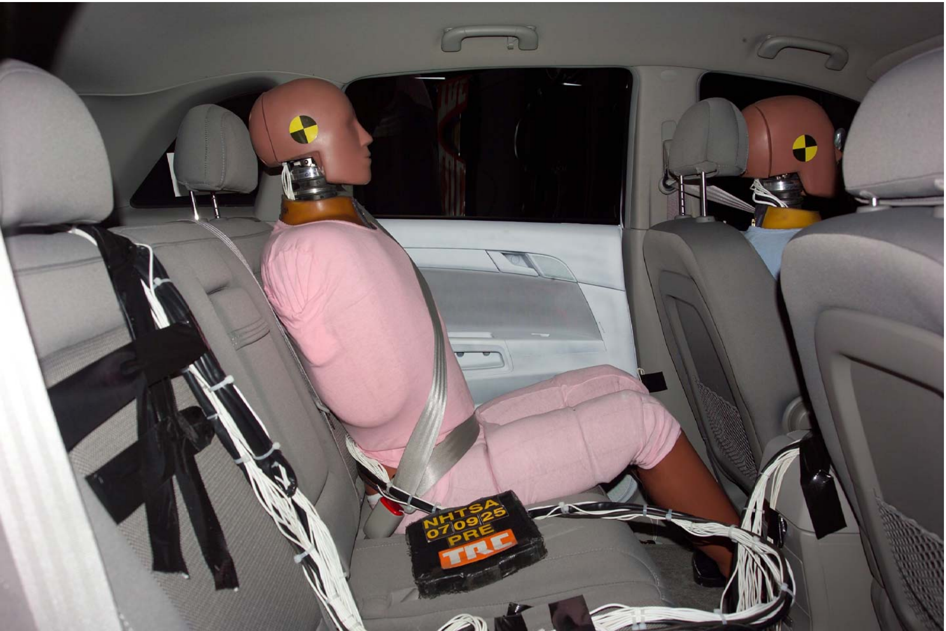
Figure A-43 Pre-Test Right Occupant Compartment View of Rear SID
