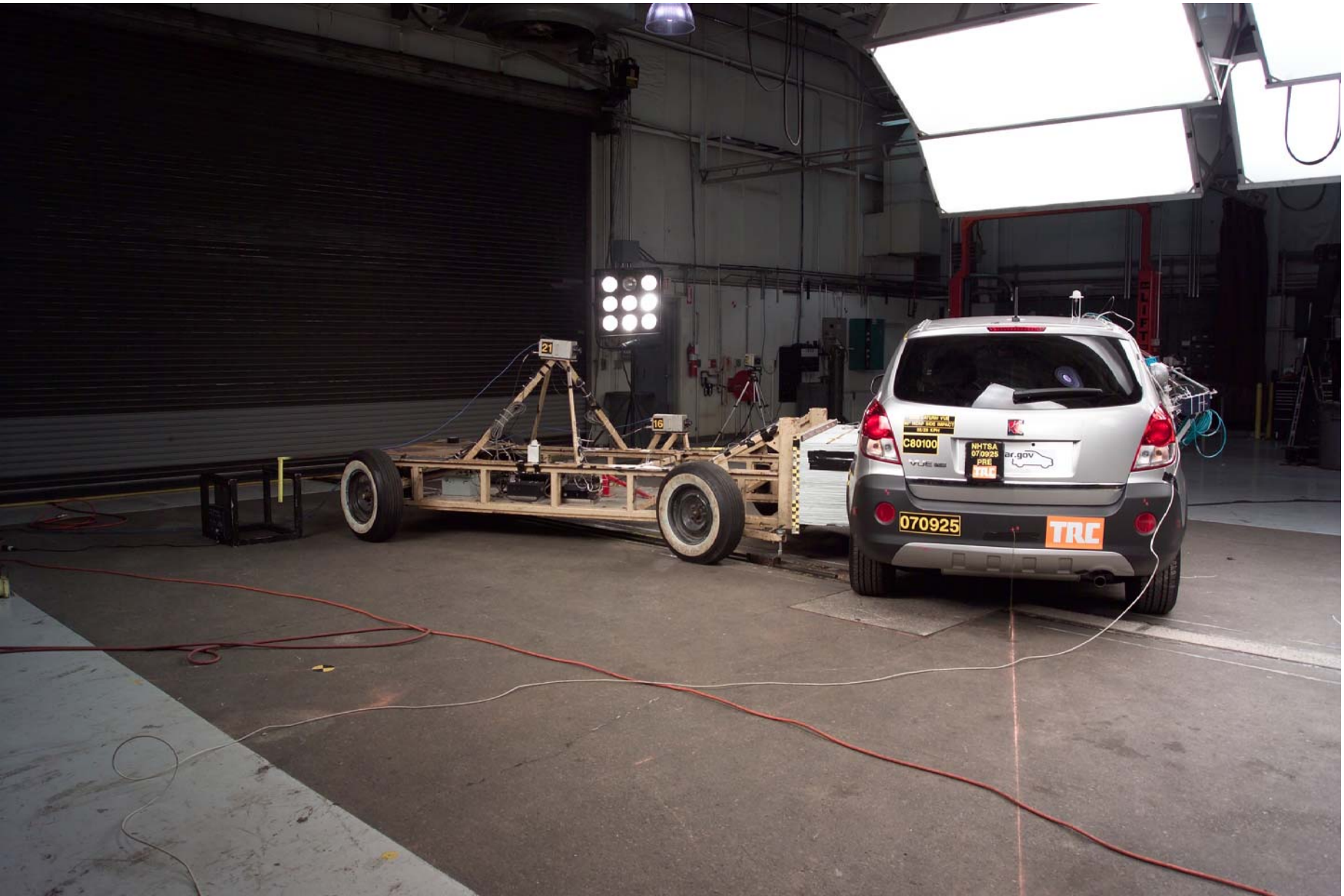
Figure A-68 Pre-Test Right Side View of MDB with Impactor Face in Position
