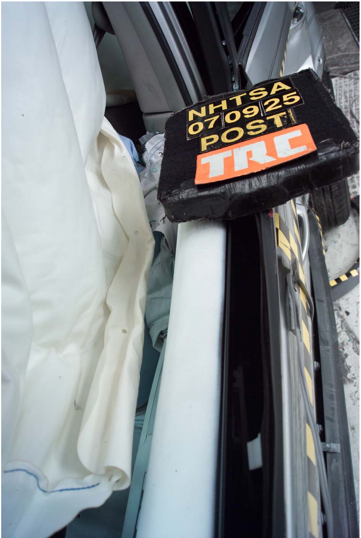
Figure A-49 Post-Test Left View of Front SID and Door Clearance
