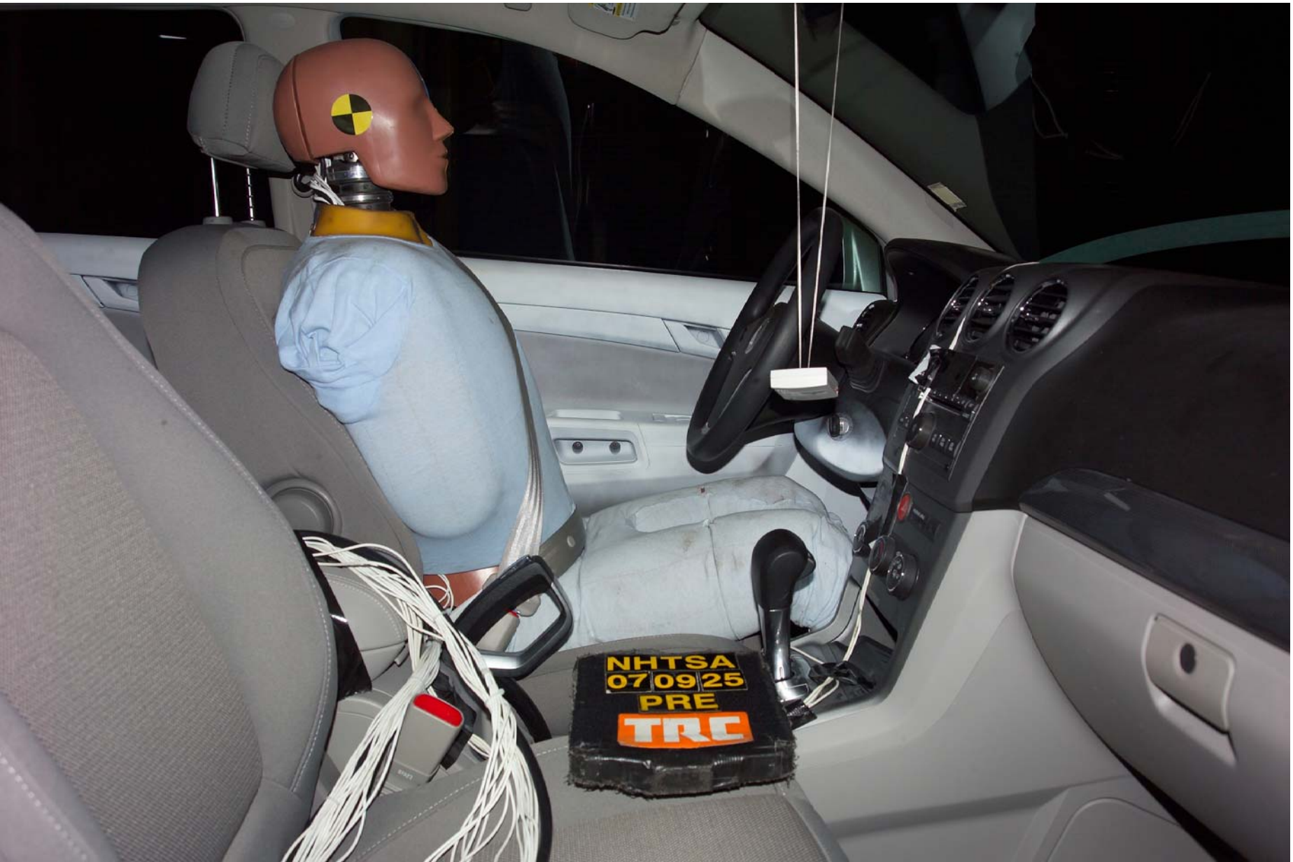
Figure A-41 Pre-Test Right Occupant Compartment View of Front SID
