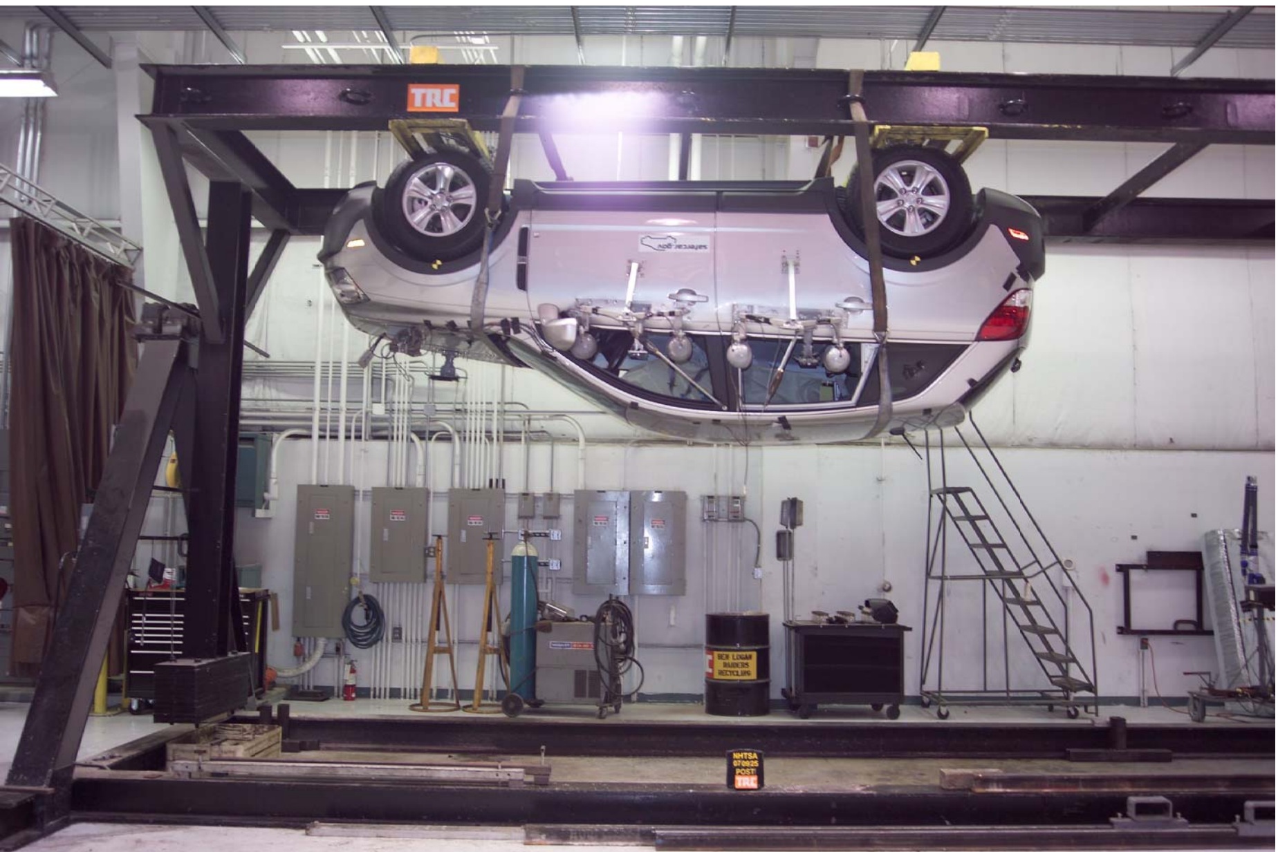
Figure A-83 FMVSS 301 Rollover View at 180°
