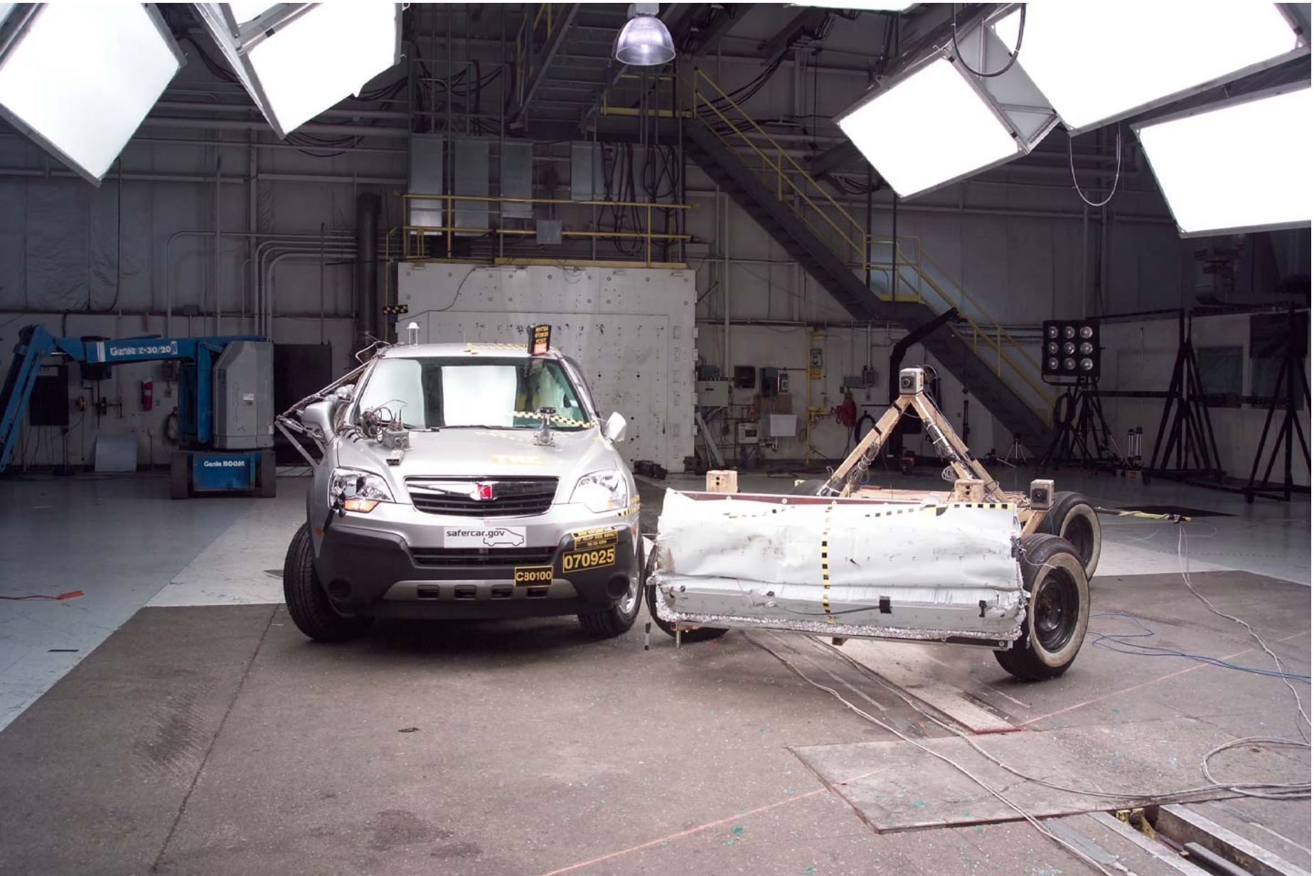
Figure A-65 Post-Test Left Side View of MDB with Impactor Face in Position
