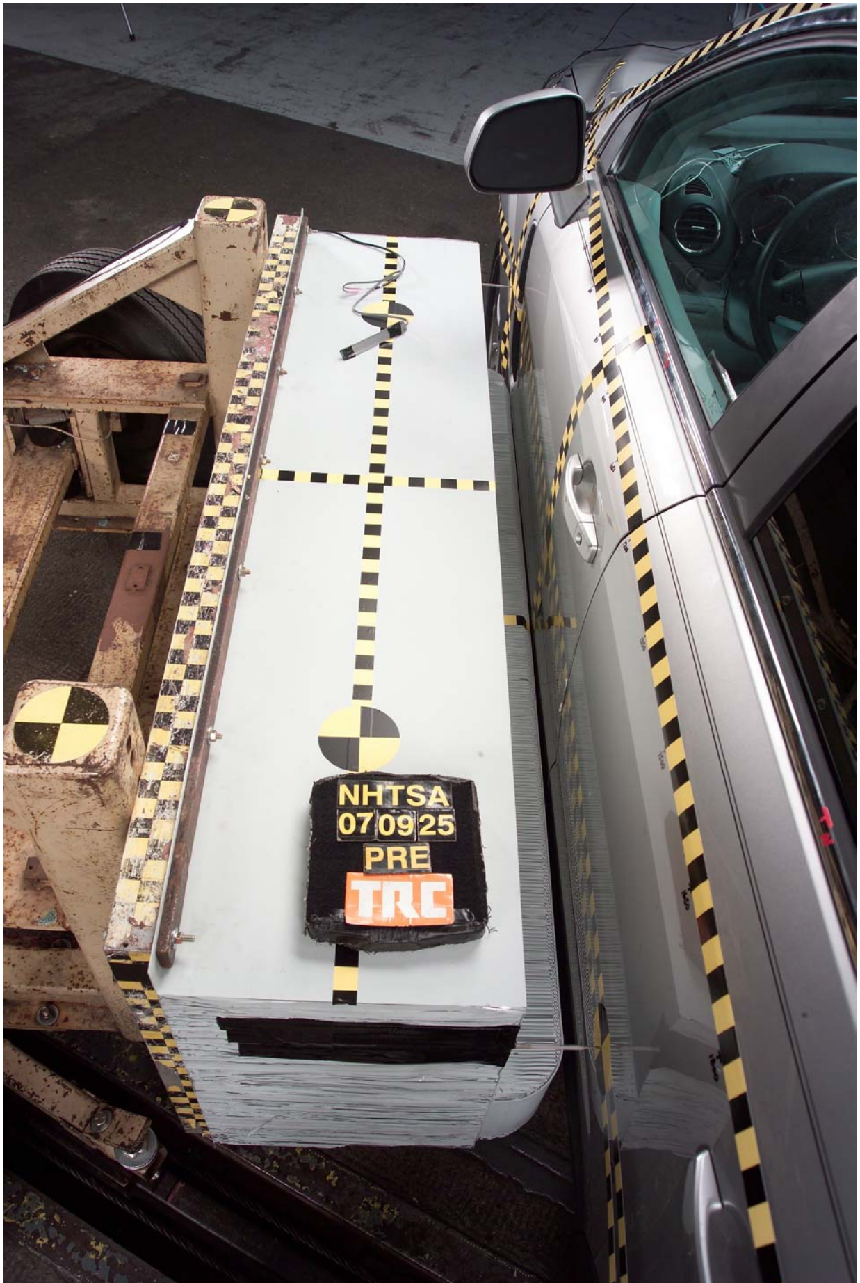
Figure A-39 Pre-Test Overhead View of MDB Aligned with Vehicle
