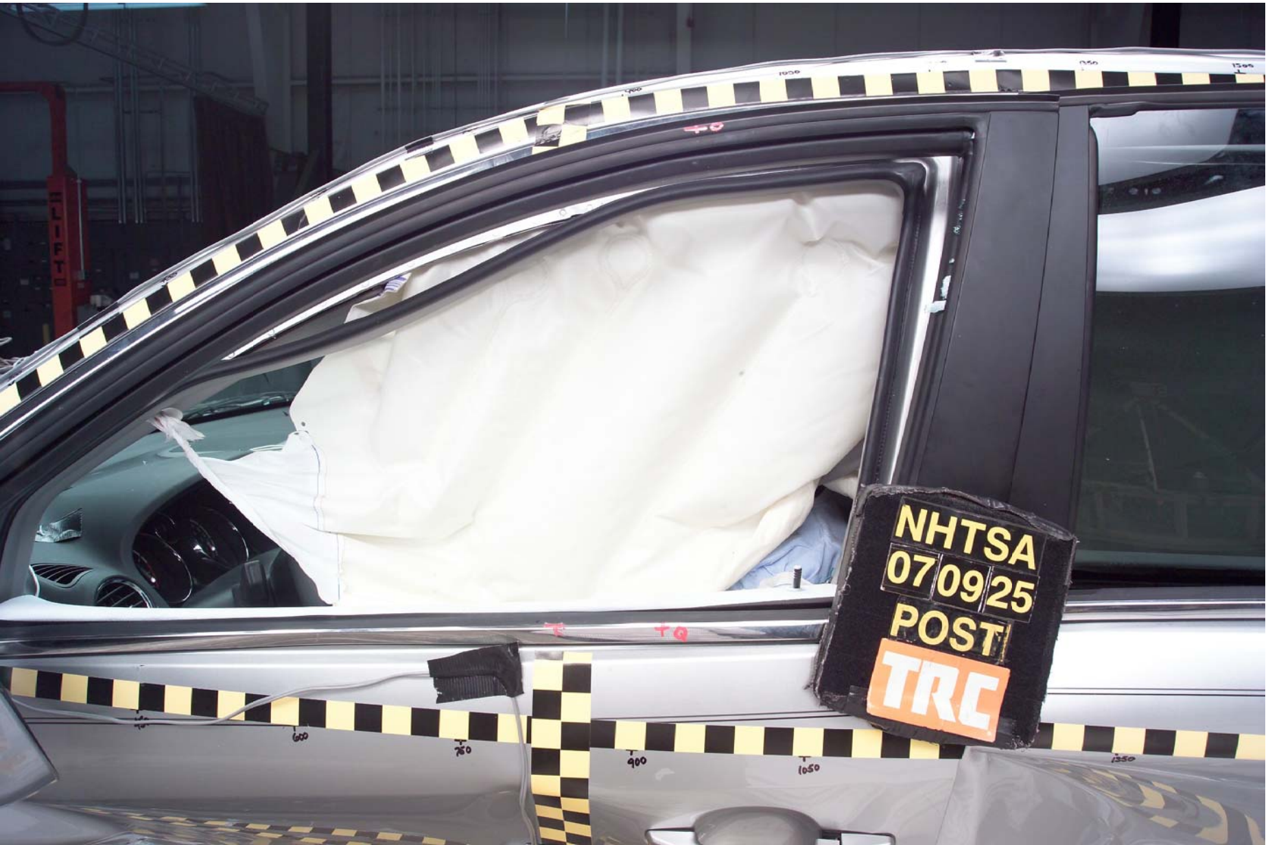
Figure A-46 Post-Test Left View of Front SID
