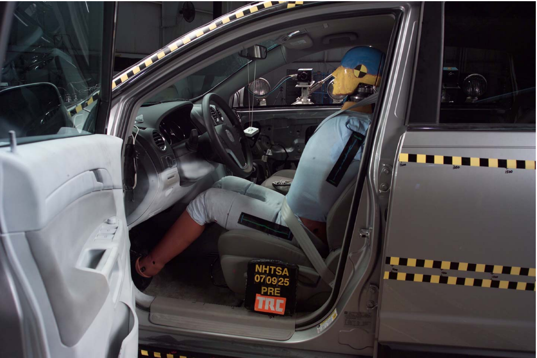
Figure A-47 Pre-Test Left View of Front SID and Belt Position
