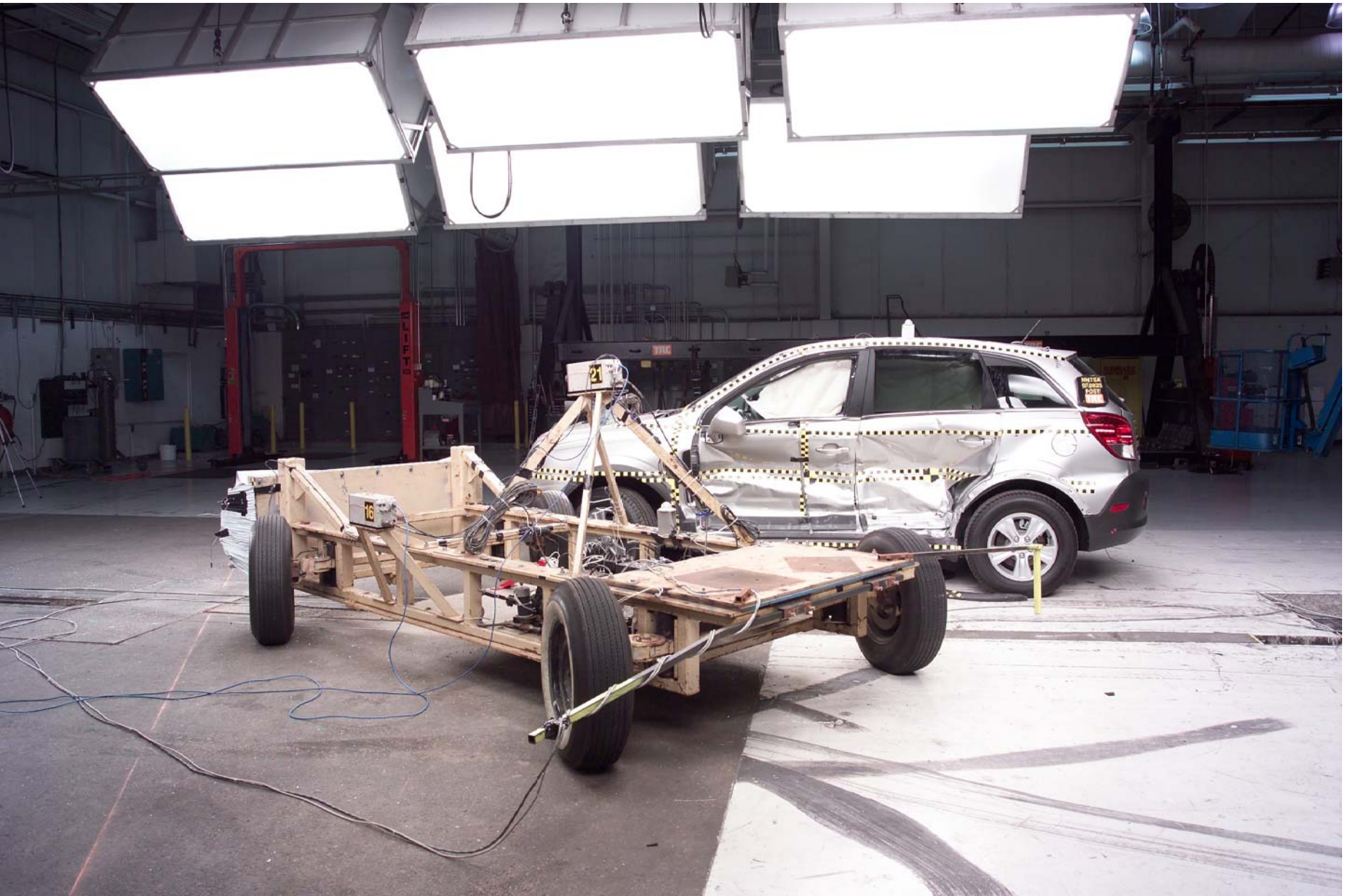
Figure A-34 Post-Test Rear Overall View of Impactor
