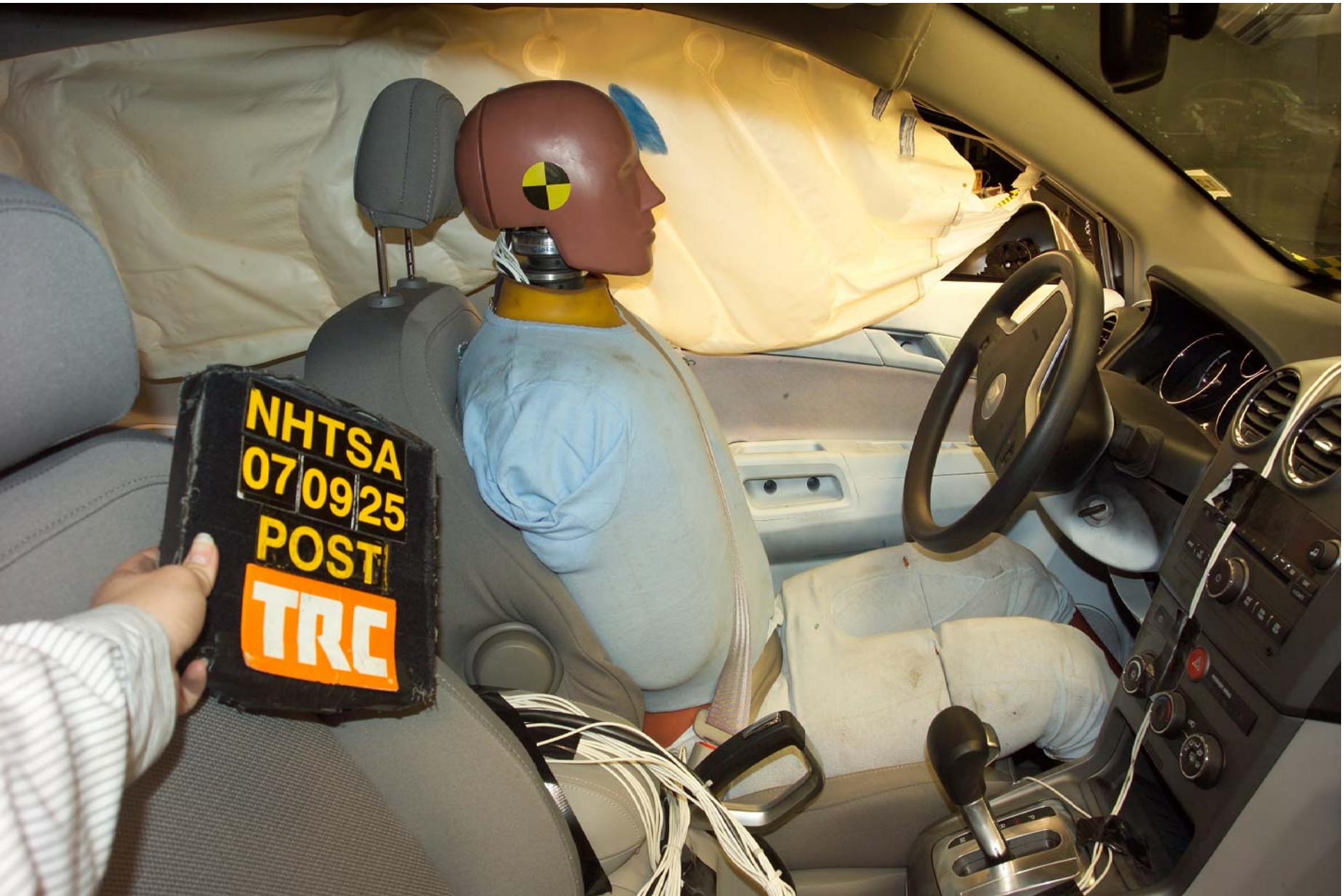
Figure A-42 Post-Test Right Occupant Compartment View of Front SID
