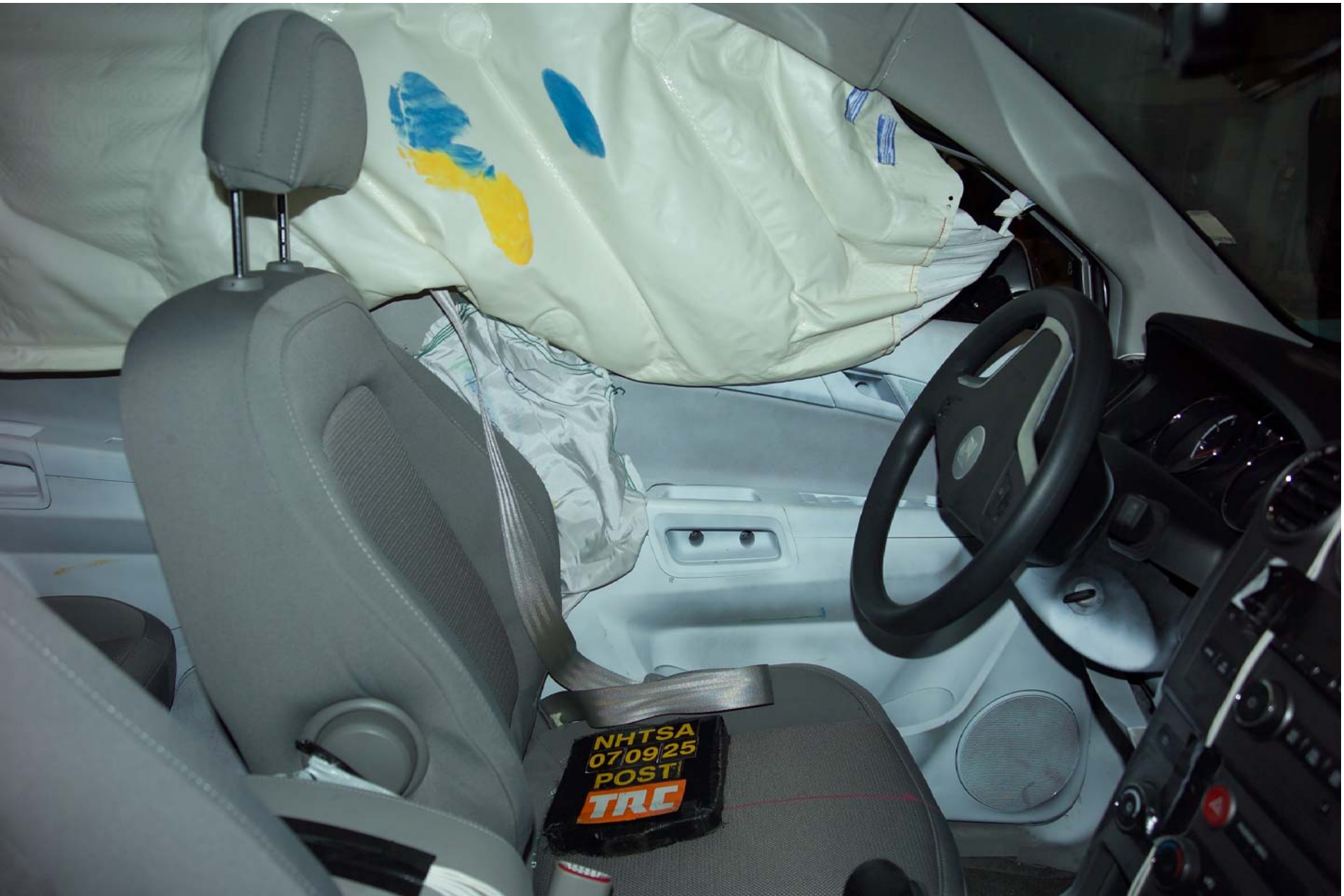
Figure A-56 Post-Test Interior of Front Door Showing SID Impact Locations
