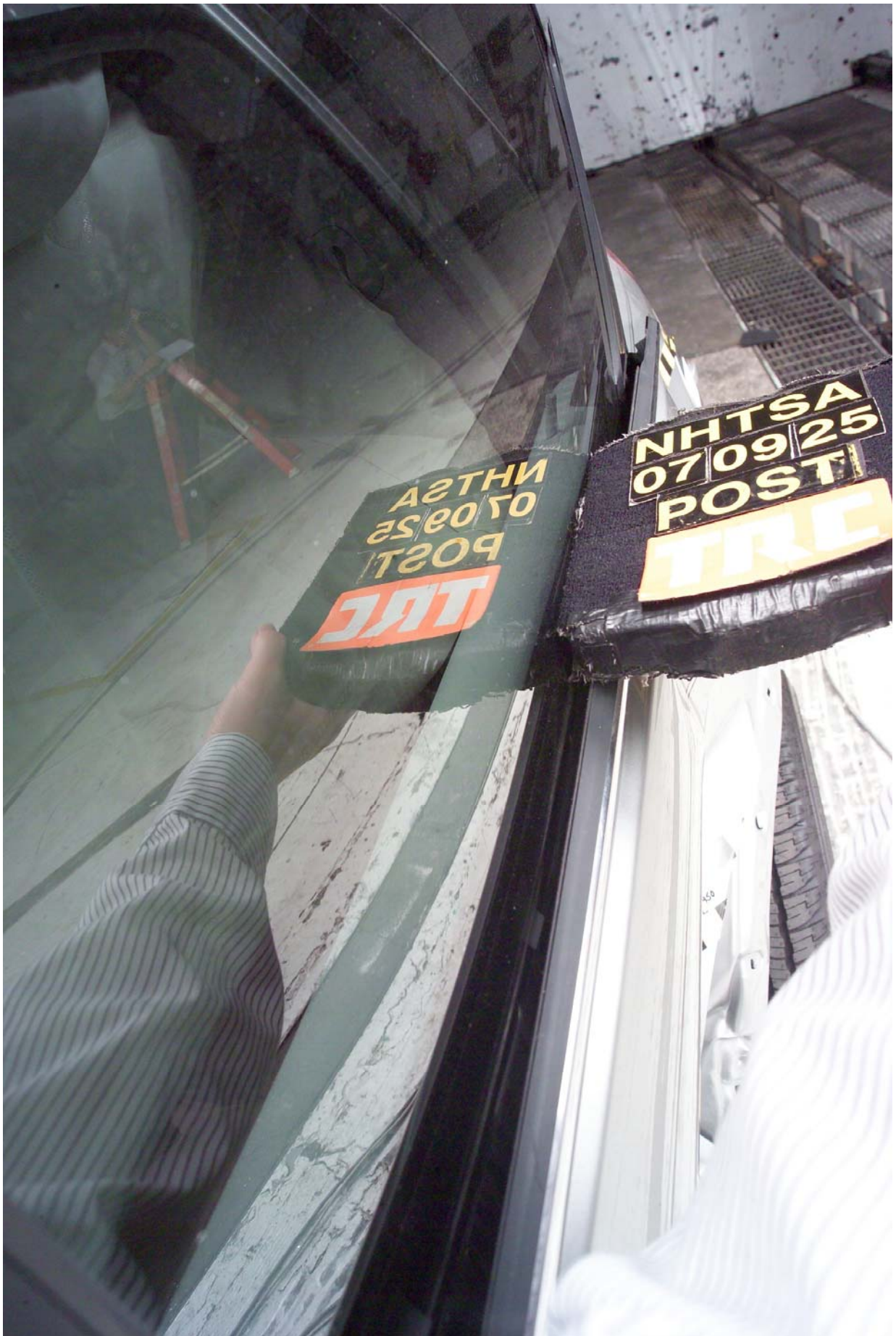
Figure A-54 Post-Test Left View of Rear SID and Door Clearance
