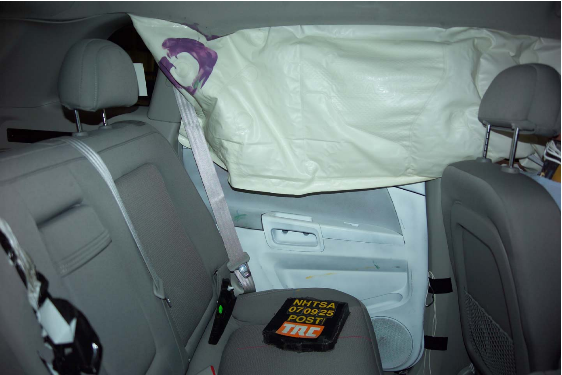
Figure A-60 Post-Test Interior of Rear Door Showing SID Impact Locations
