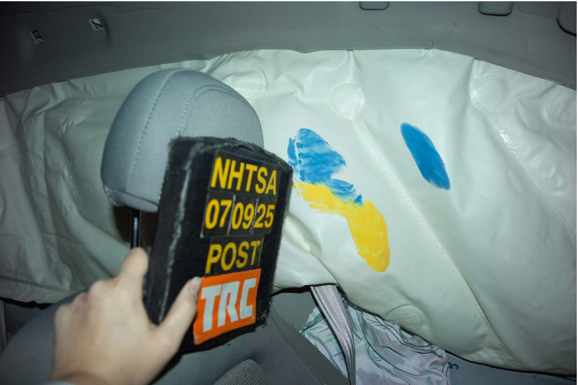
Figure A-57 Post-Test Front SID Contact – View 1
