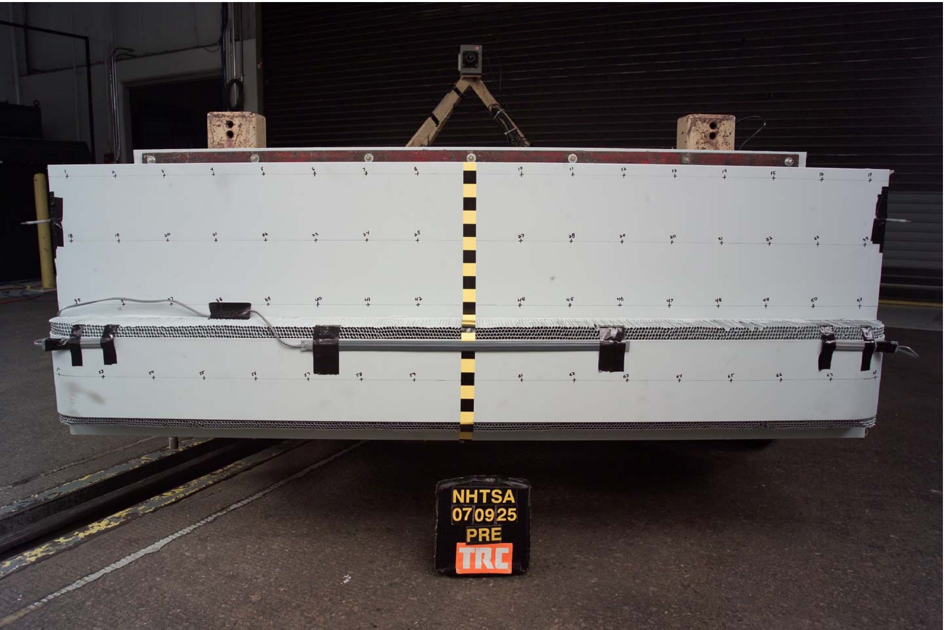
Figure A-37 Pre-Test View of MDB Showing Contact Switches in Place
