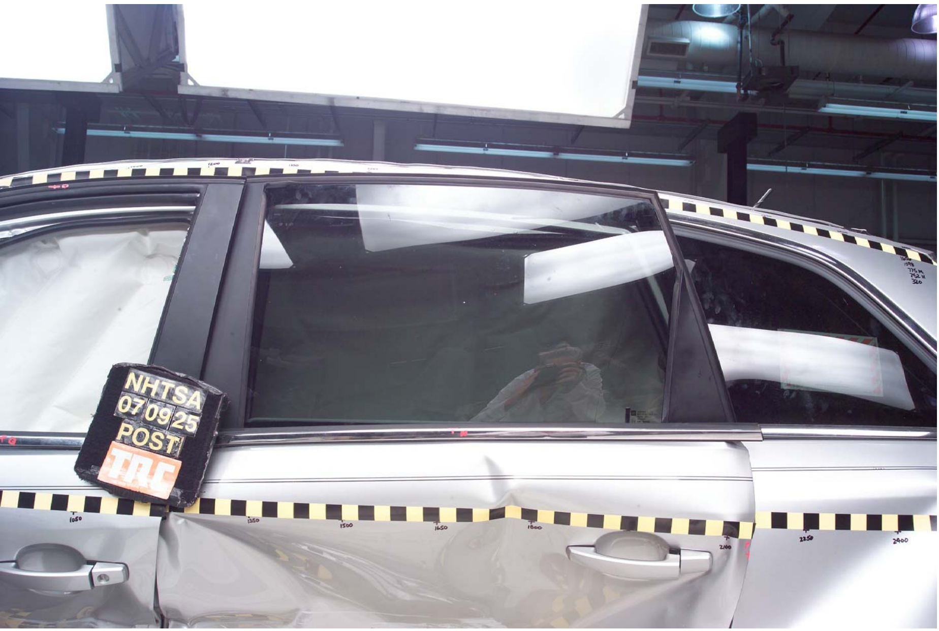
Figure A-51 Post-Test Left View of Rear SID
