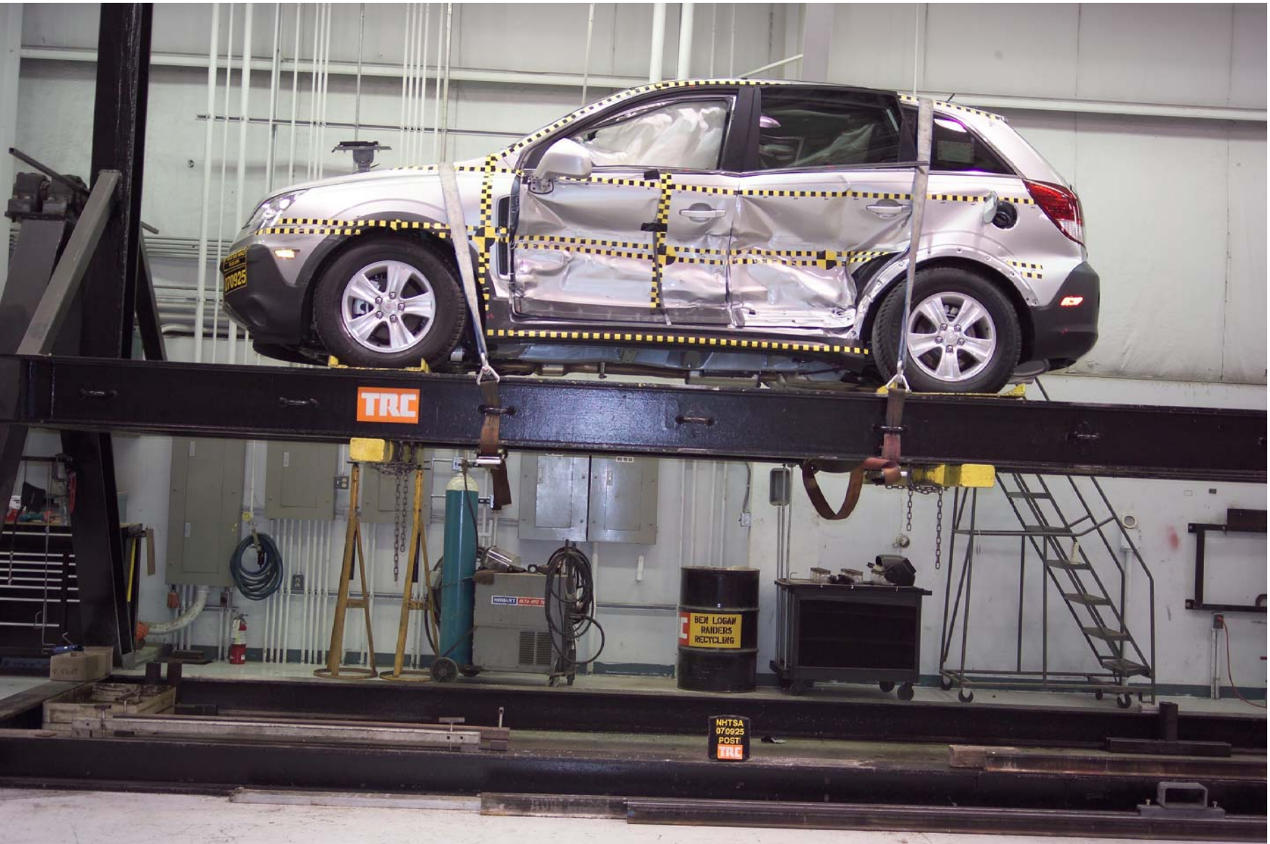
Figure A-85 FMVSS 301 Rollover View at 360°
