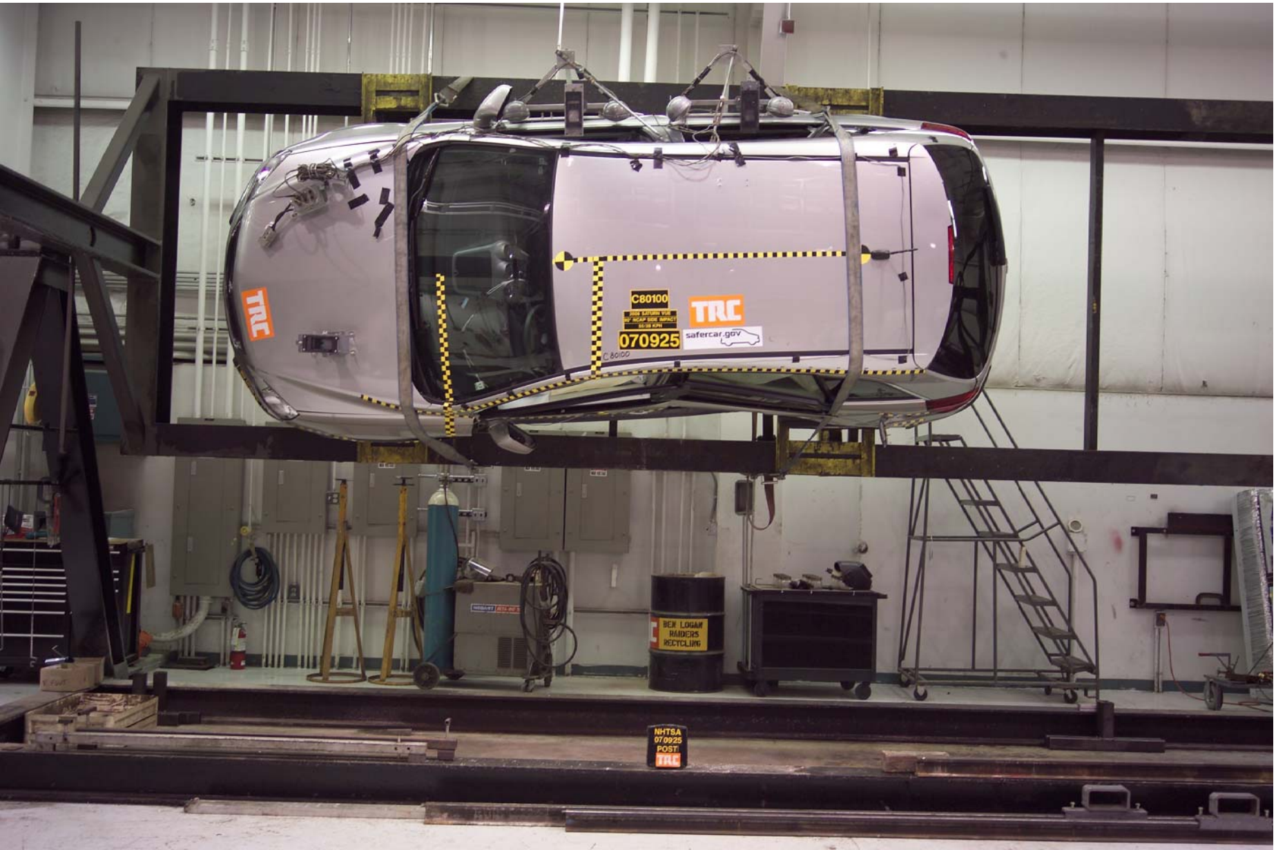
Figure A-82 FMVSS 301 Rollover View at 90°
