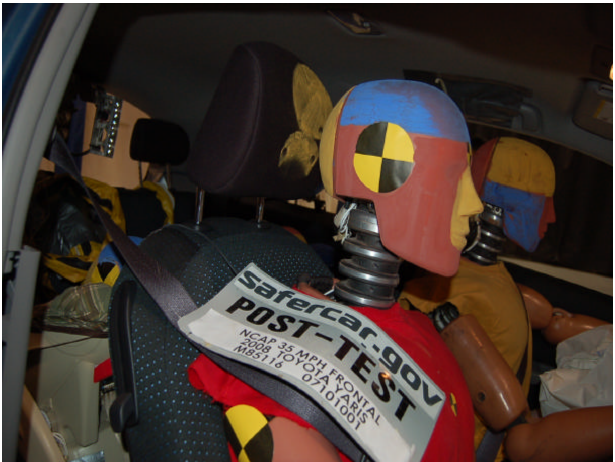
Post-Test Passenger Dummy Head Contact (headrest)
