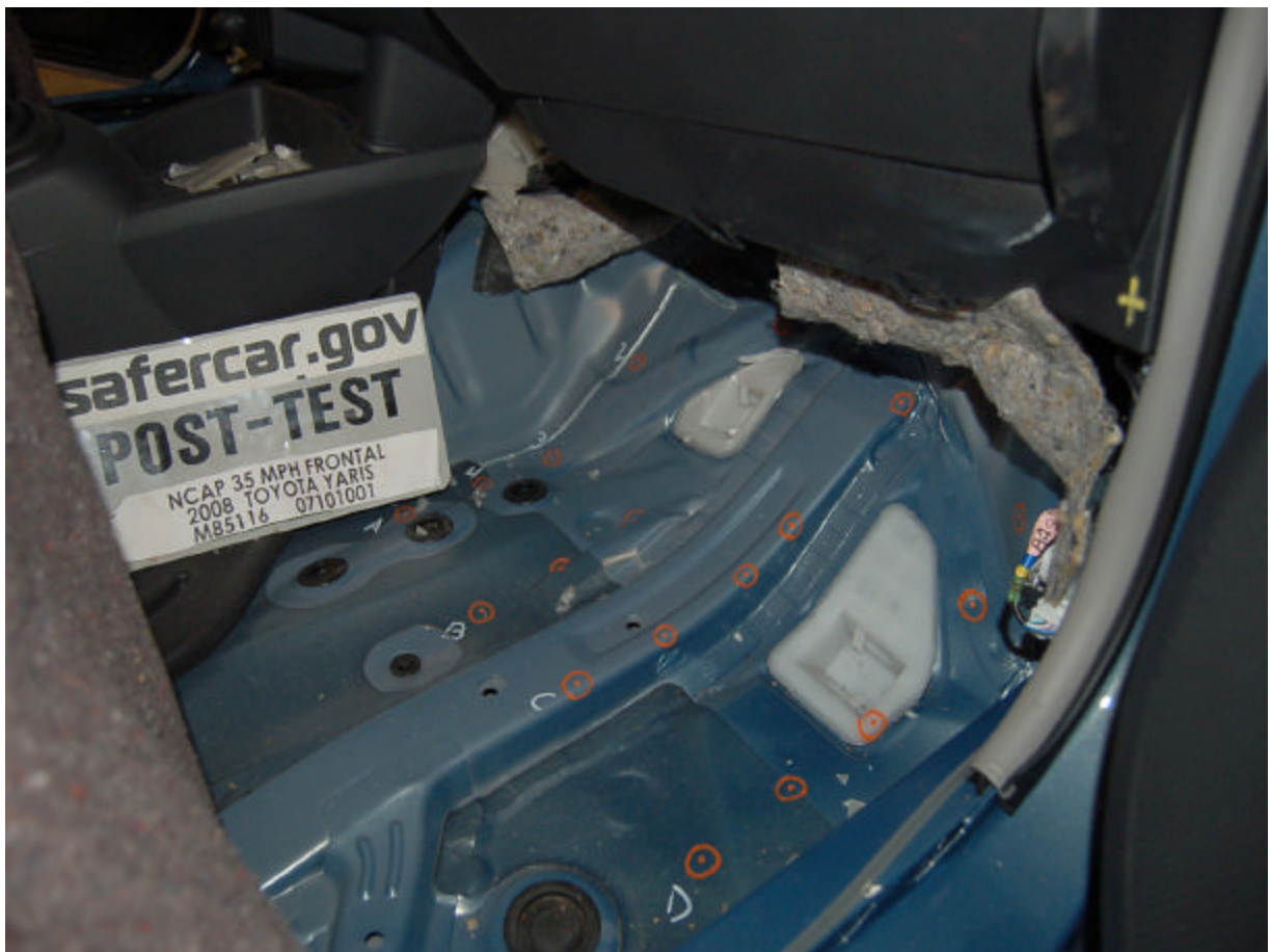
Post-Test Passenger Side Floor Pan
