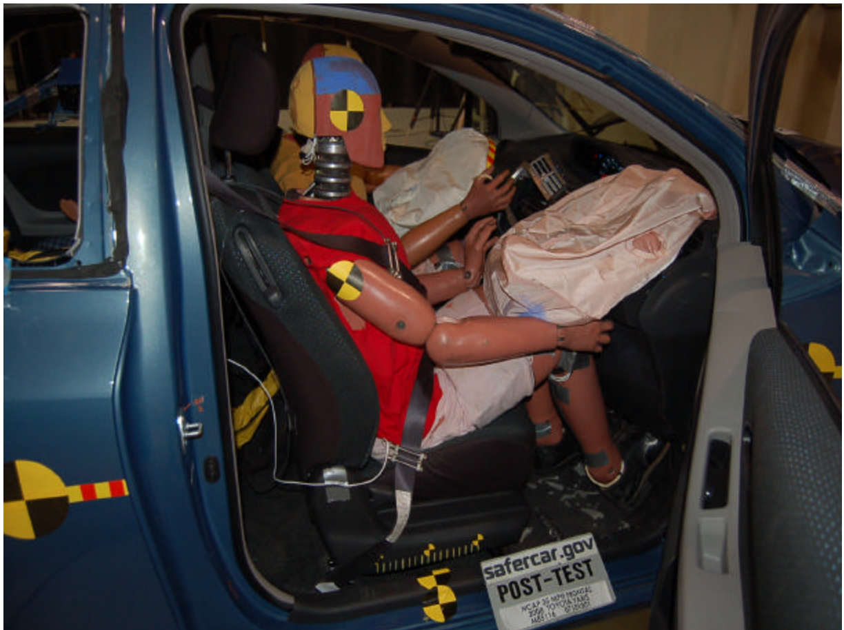
Post-Test Passenger Dummy (Door Open)
