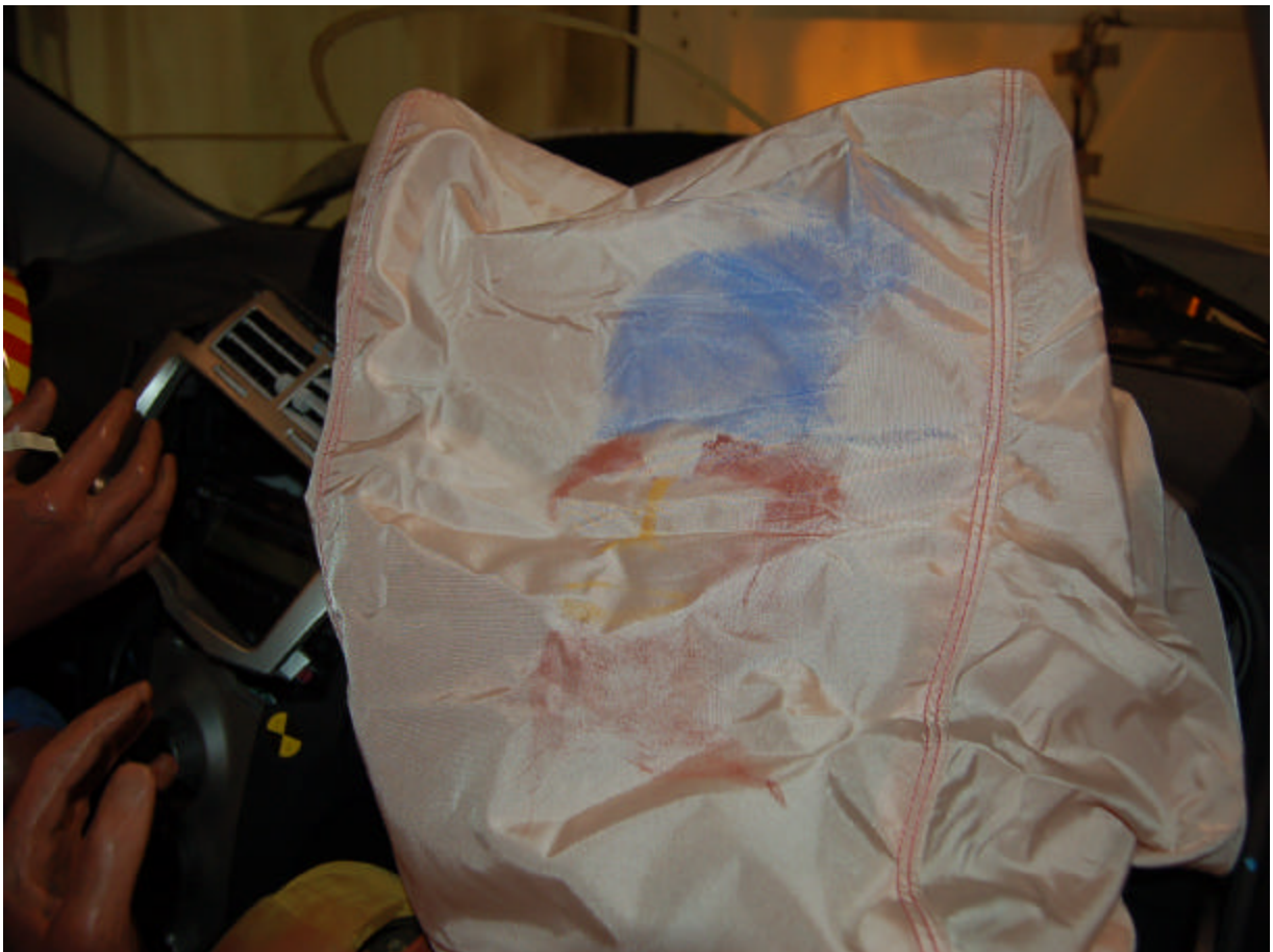
Post-Test Passenger Dummy Airbag Contact
