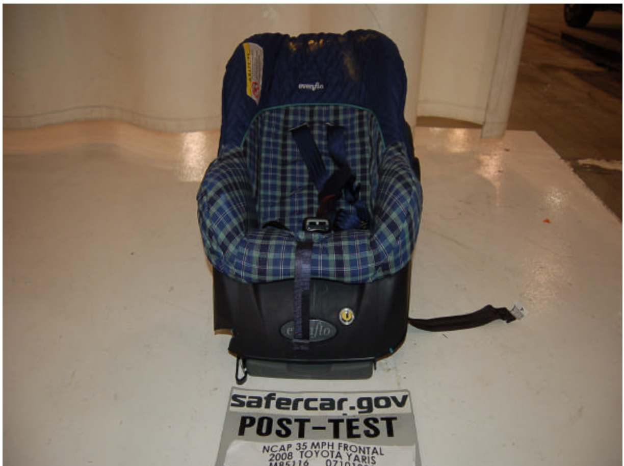
Post-Test Front View of Position 4 CRS
