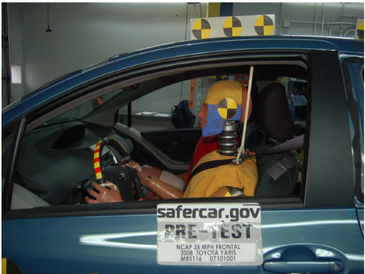
Pre-Test Driver Dummy (Through Window)
