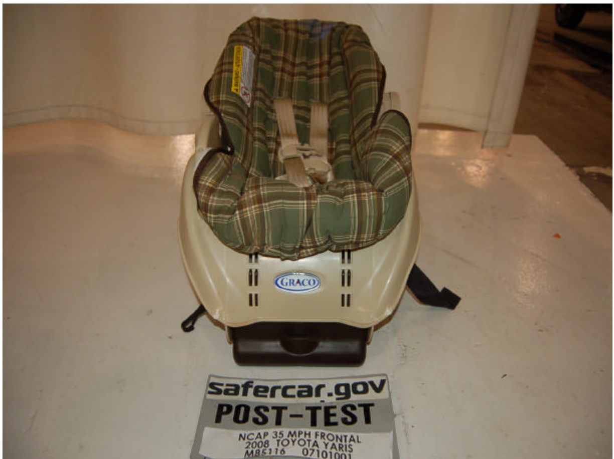
Post-Test Front View of Position 3 CRS
