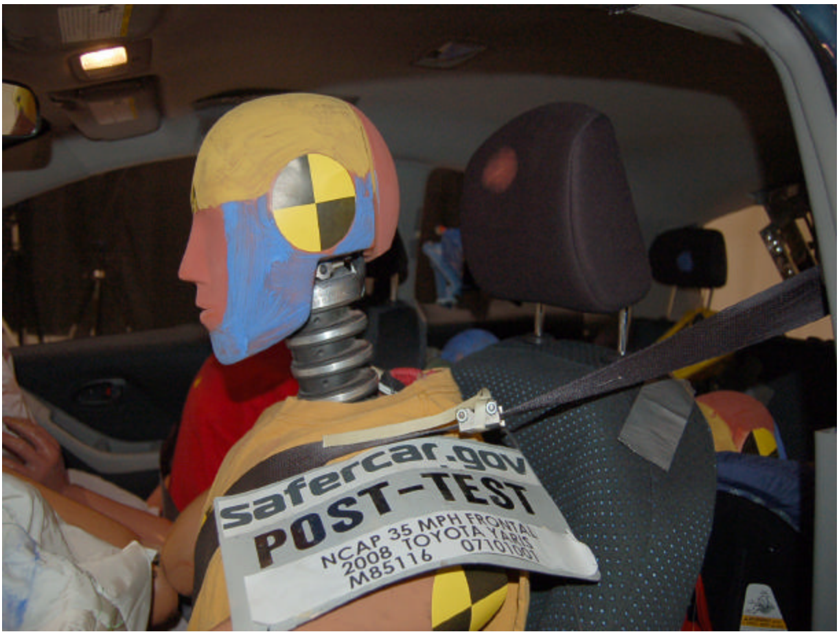
Post-Test Driver Dummy Head Contact (headrest)
