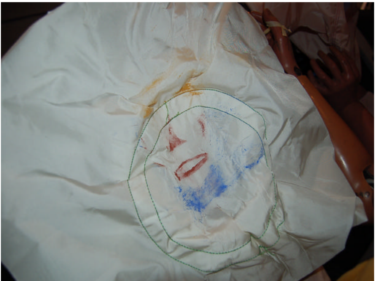
Post-Test Driver Dummy Airbag Contact
