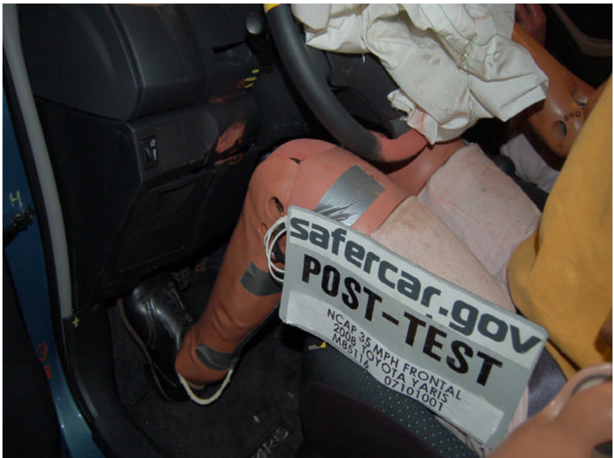
Post-Test Driver Side Knee Bolster
