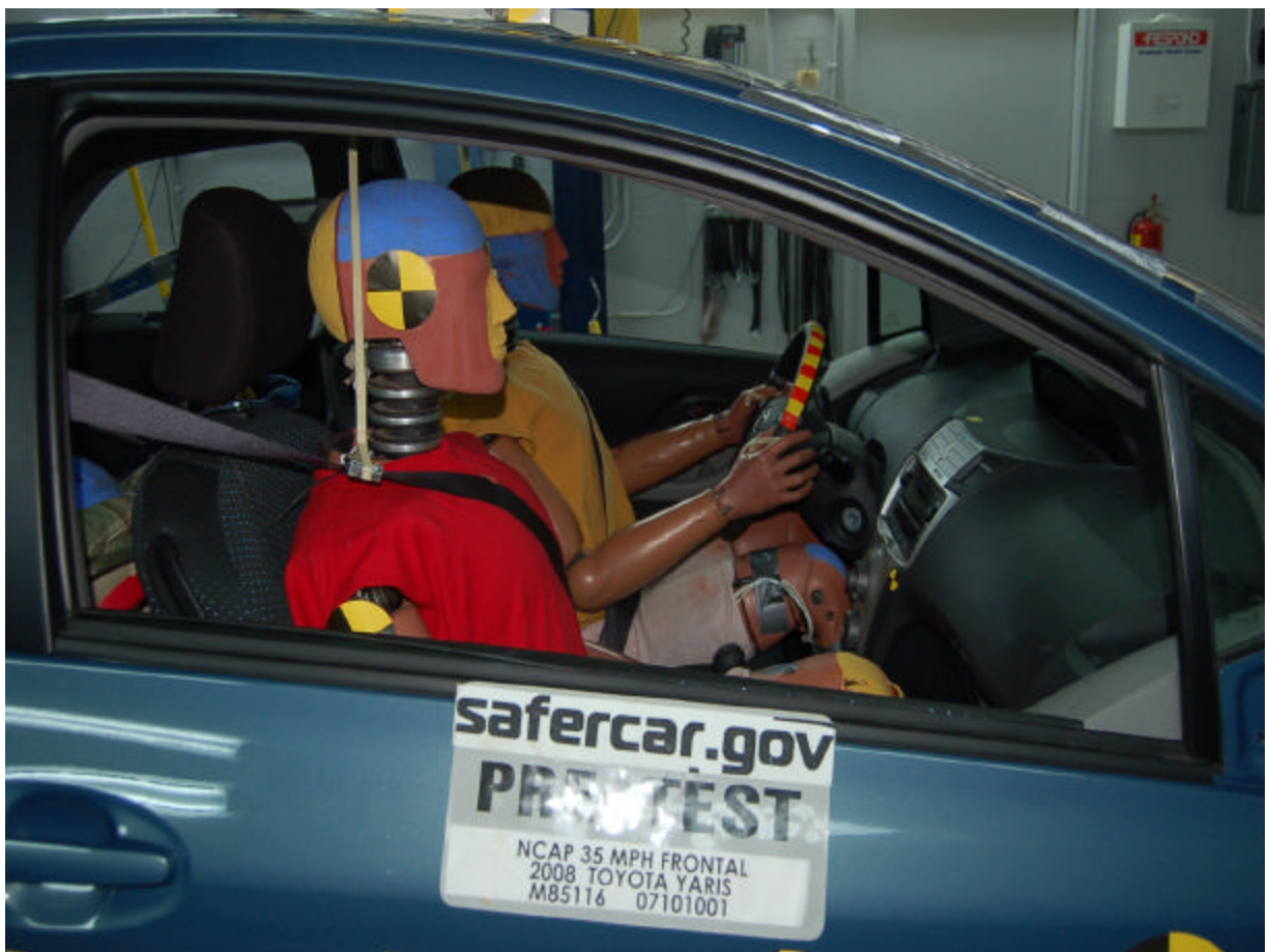
Pre-Test Passenger Dummy (Through Window)
