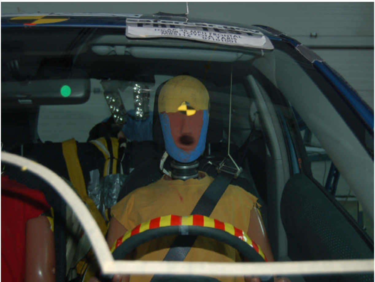
Pre-Test Driver Dummy Front View (Head Position)
