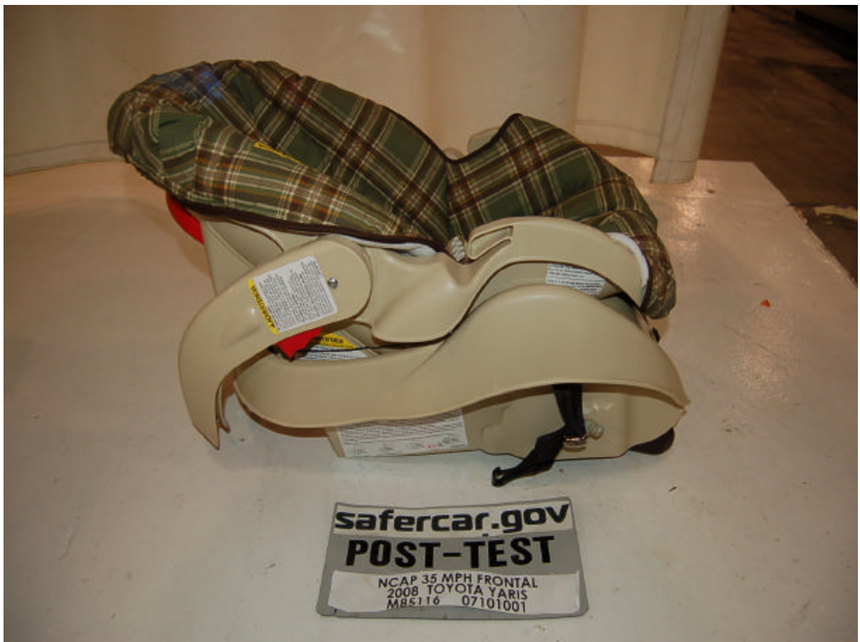
Post-Test Right Side View of Position 3 CRS
