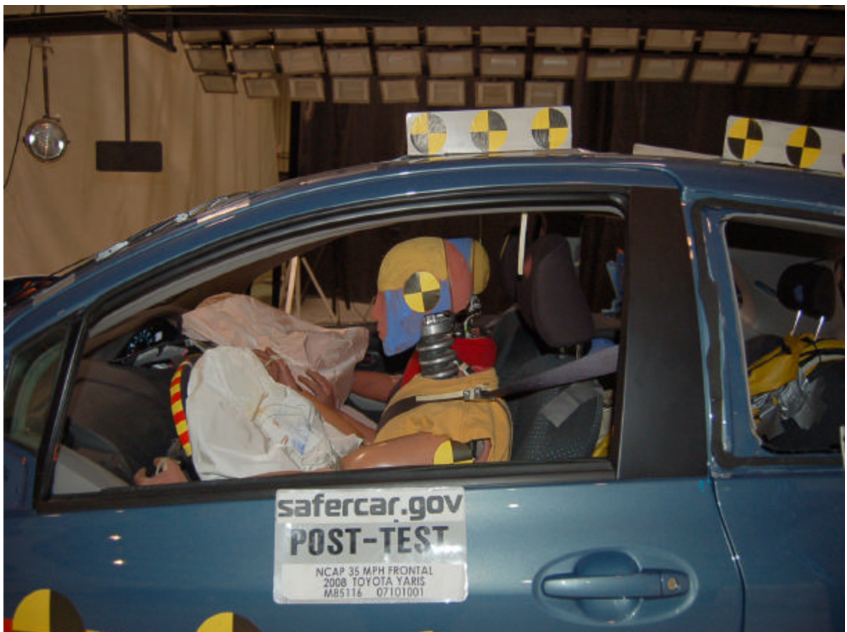
Post-Test Driver Dummy (Through Window)
