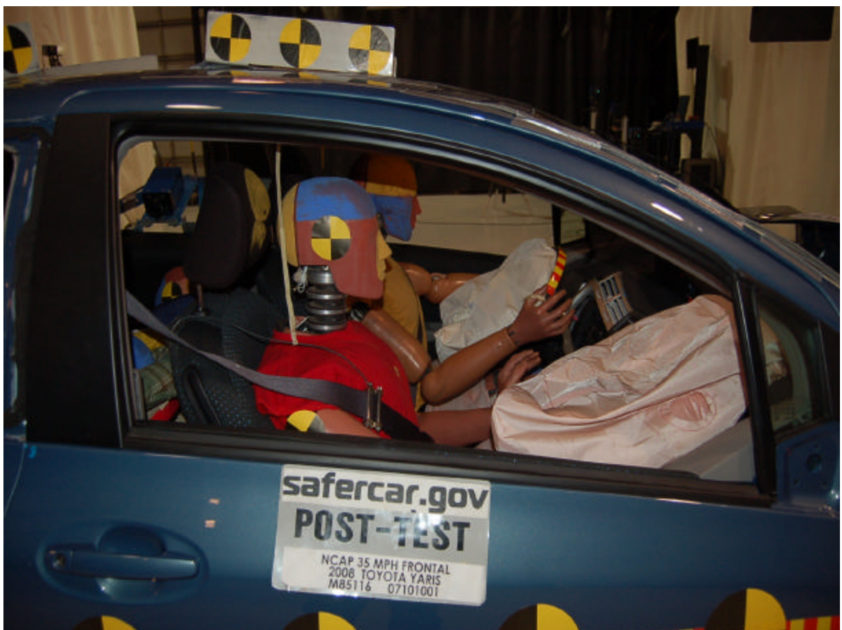
Post-Test Passenger Dummy (Through Window)
