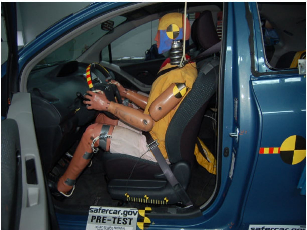
Pre-Test Driver Dummy (Door Open)
