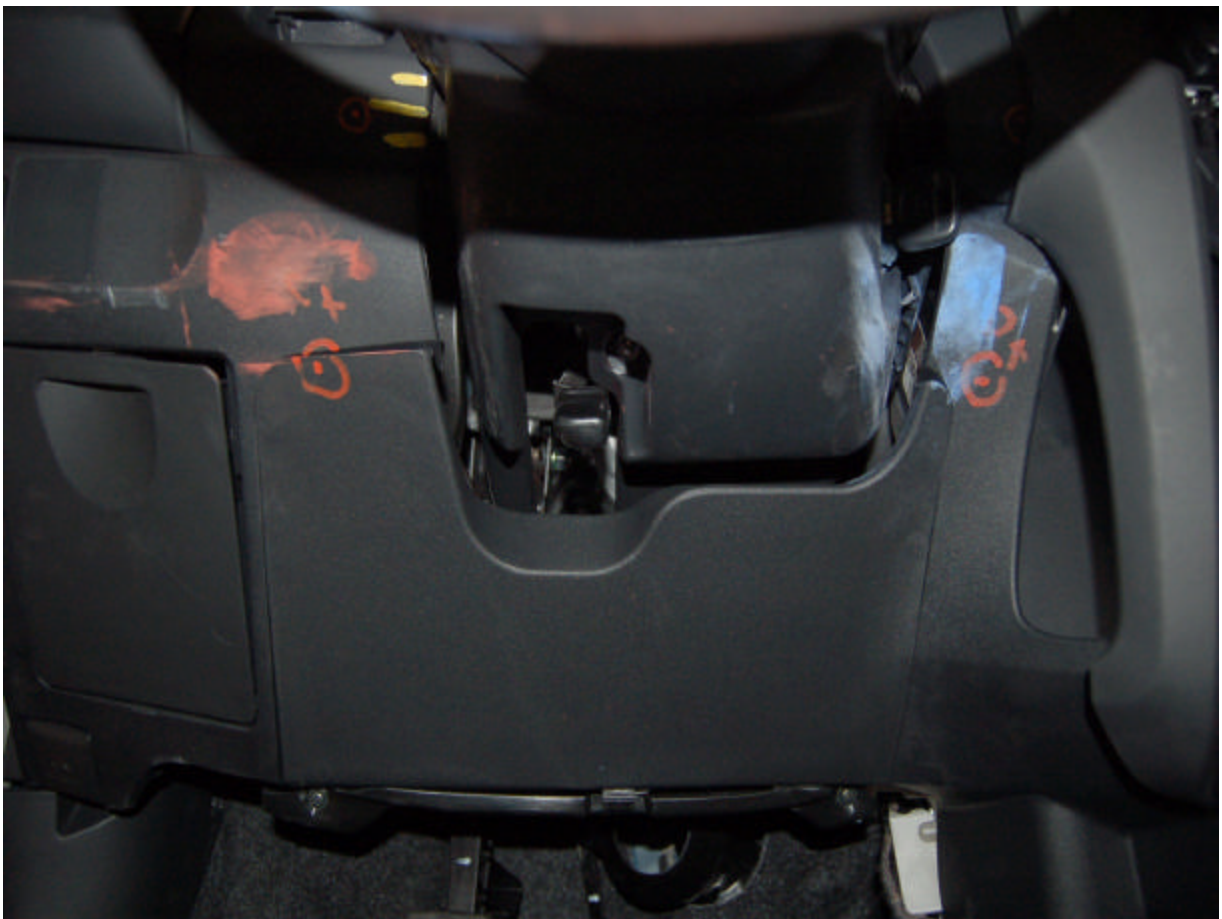
Post-Test Driver Dummy Knee Contact
