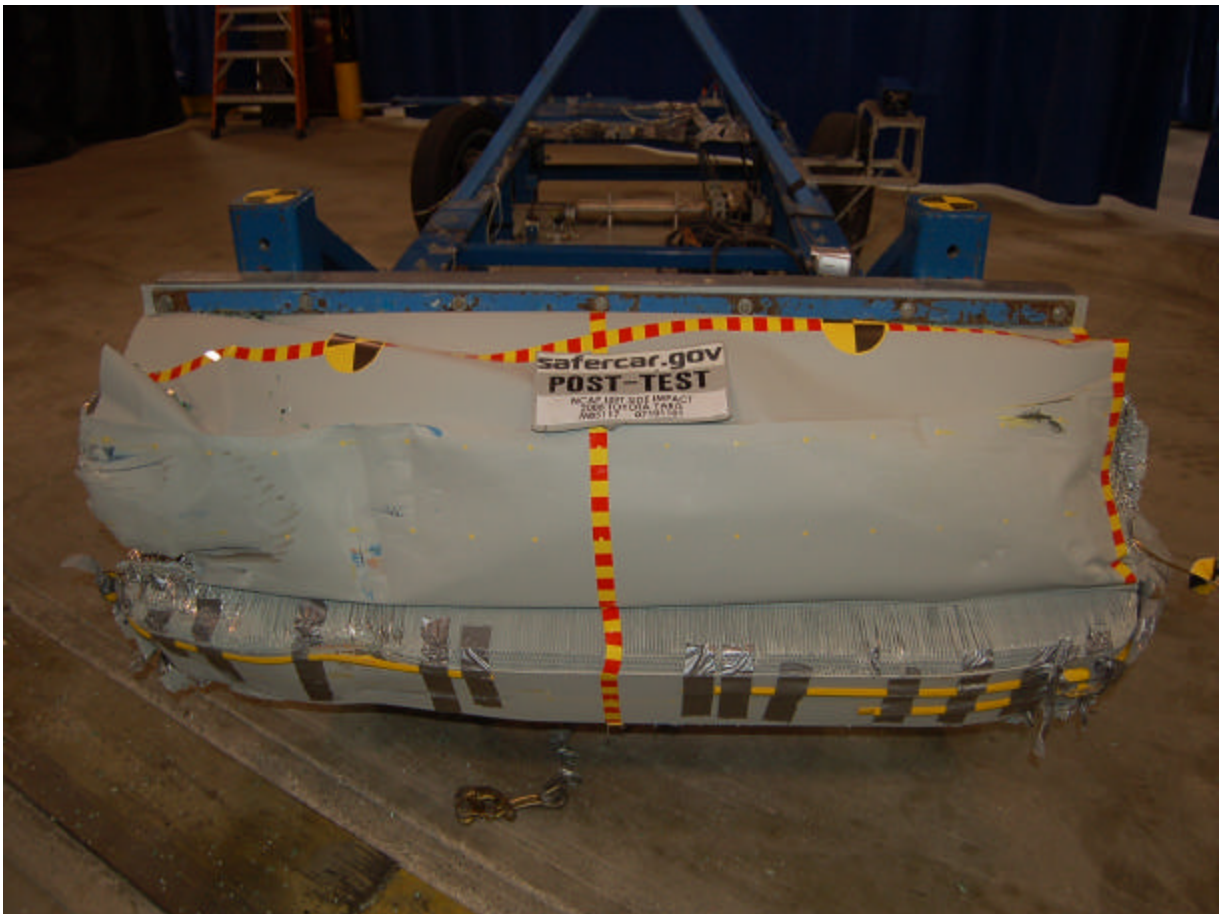
Post-Test Front View of Deformable Barrier
