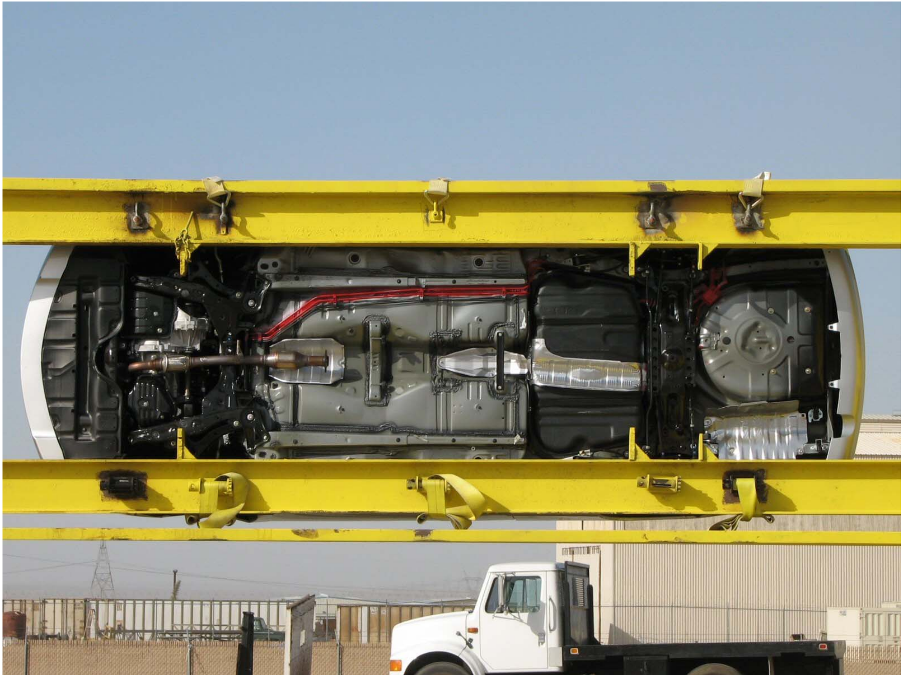
Figure A-64: Vehicle on Rollover Device (270°)
