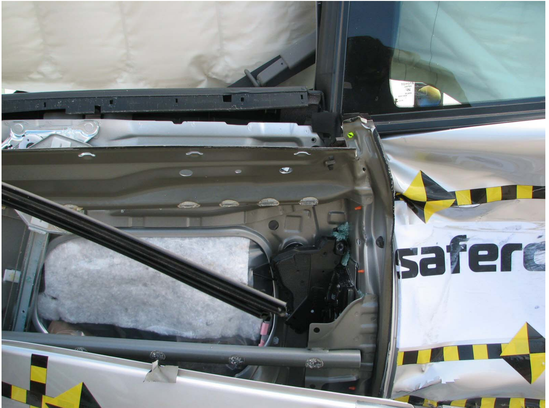
Figure A-32: Post-Test Left Front Door
