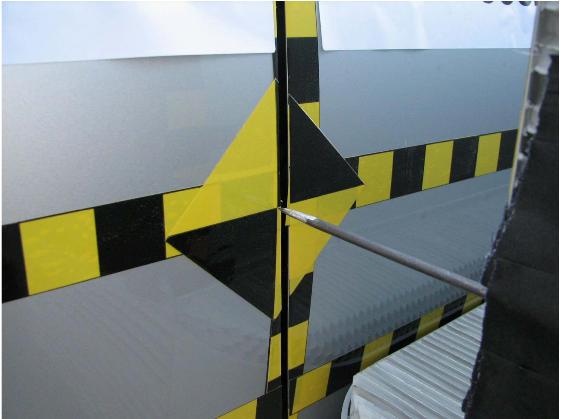
Figure A-25: Pre-Test Left Impact Point
