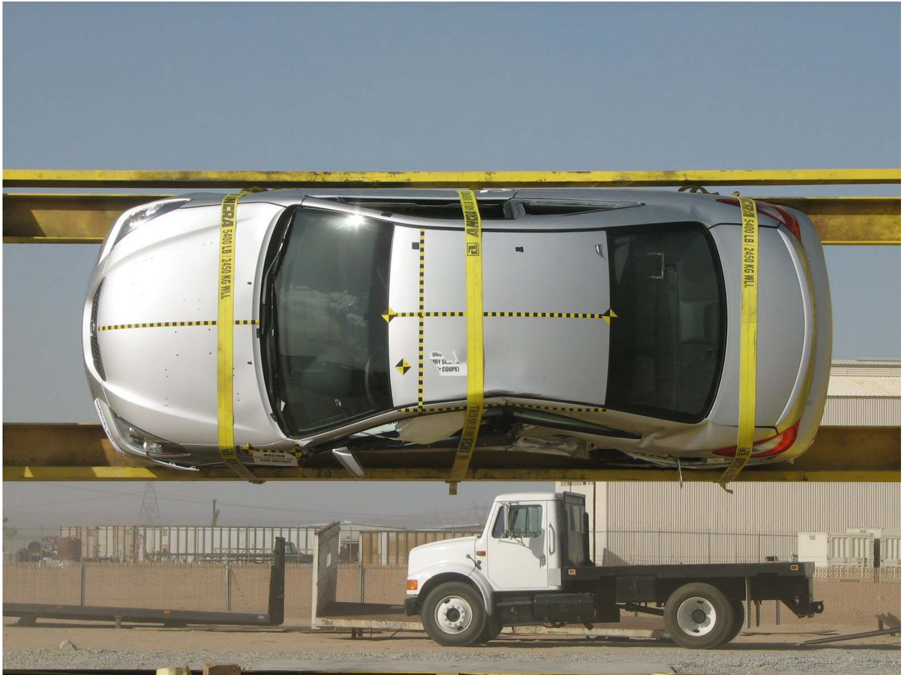
Figure A-62: Vehicle on Rollover Device (90°)
