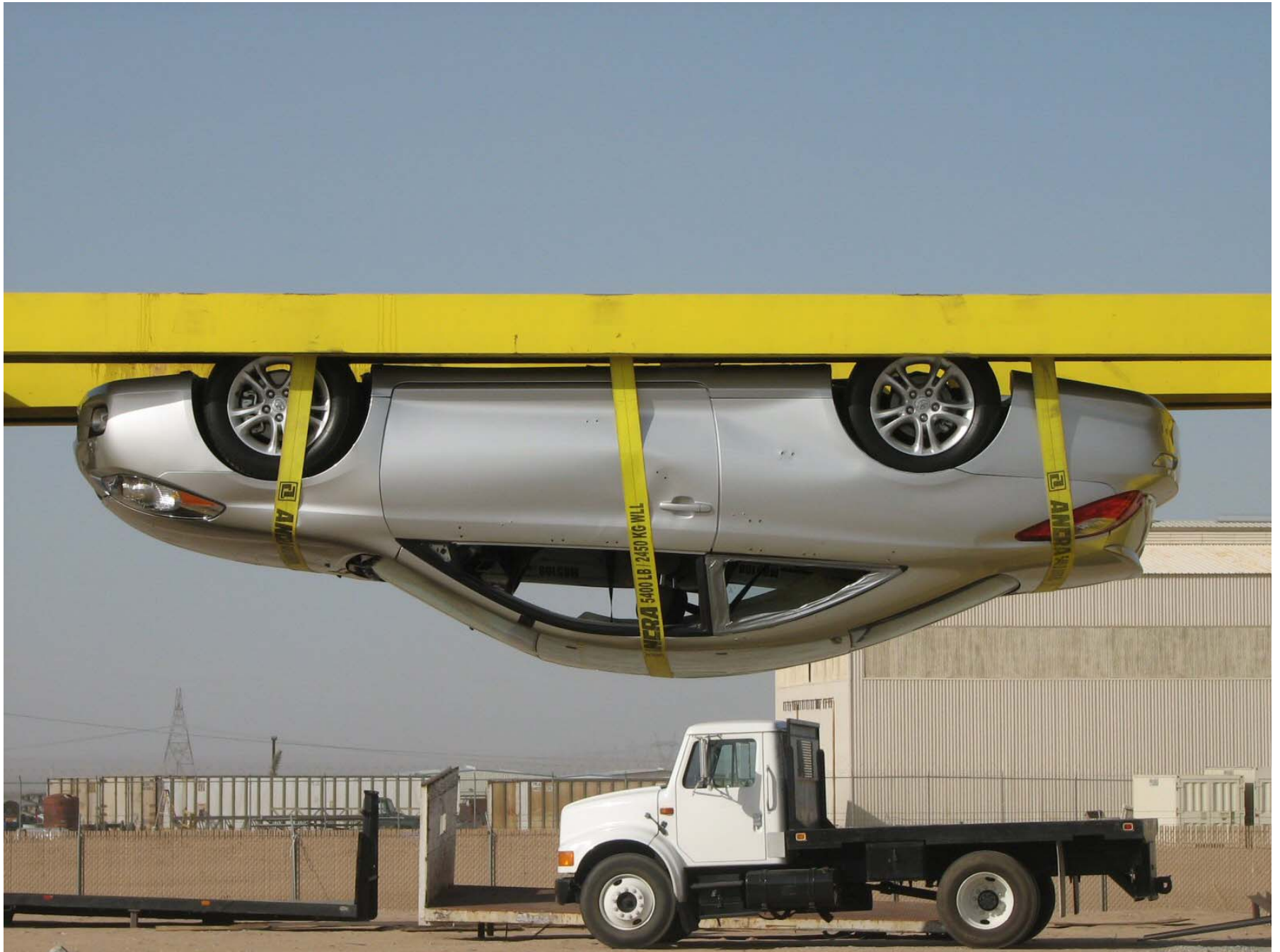
Figure A-63: Vehicle on Rollover Device (180°)
