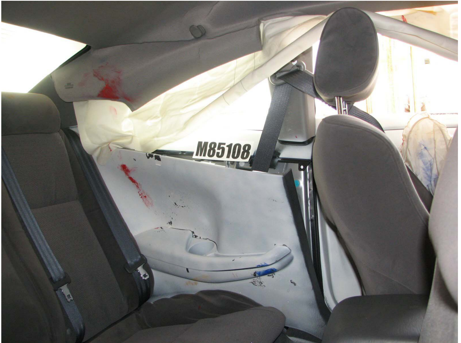
Figure A-52: Post-Test Rear Door Panel (Interior)
