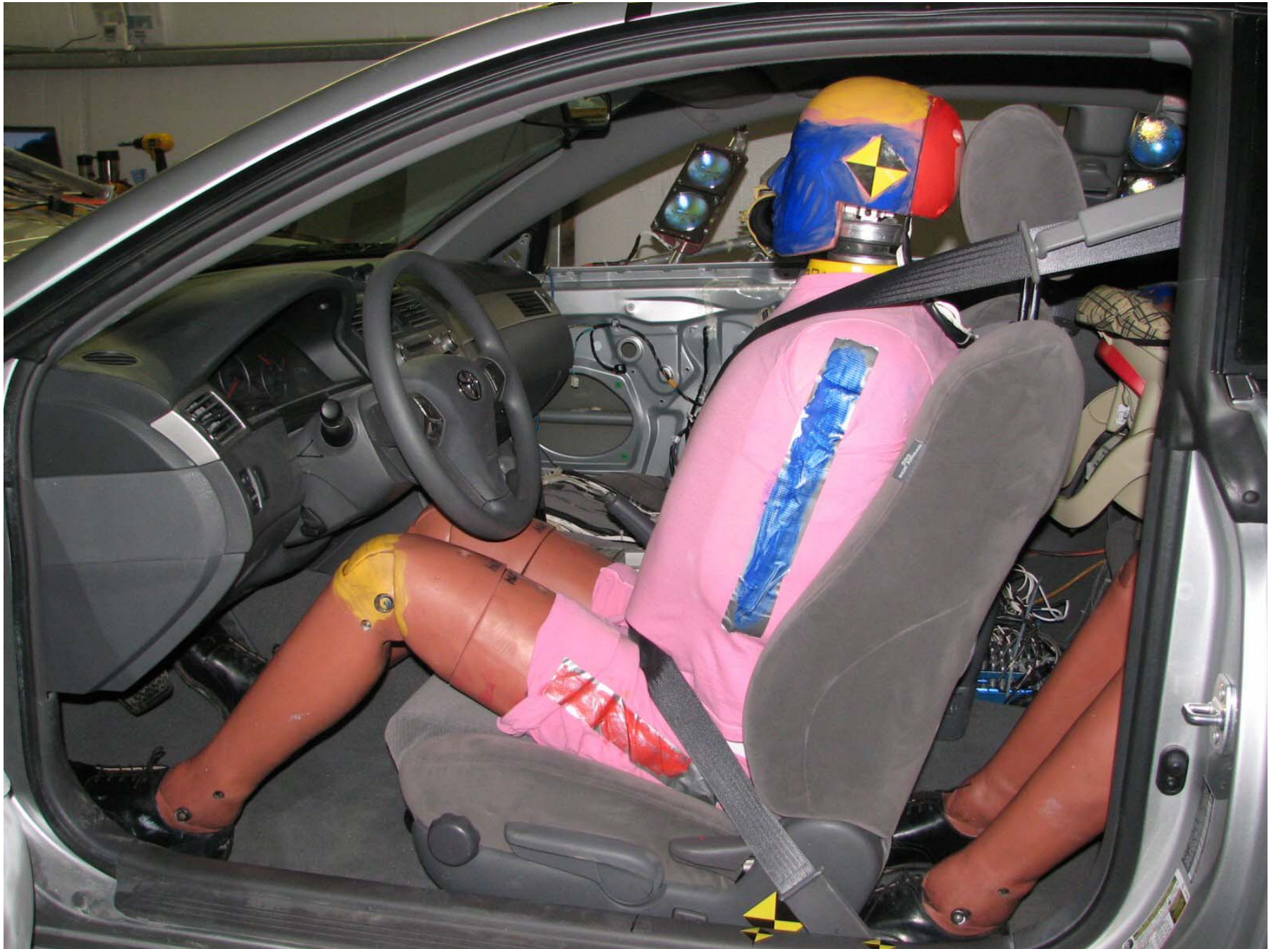
Figure A-35: Pre-Test Driver Dummy (Door Open)
