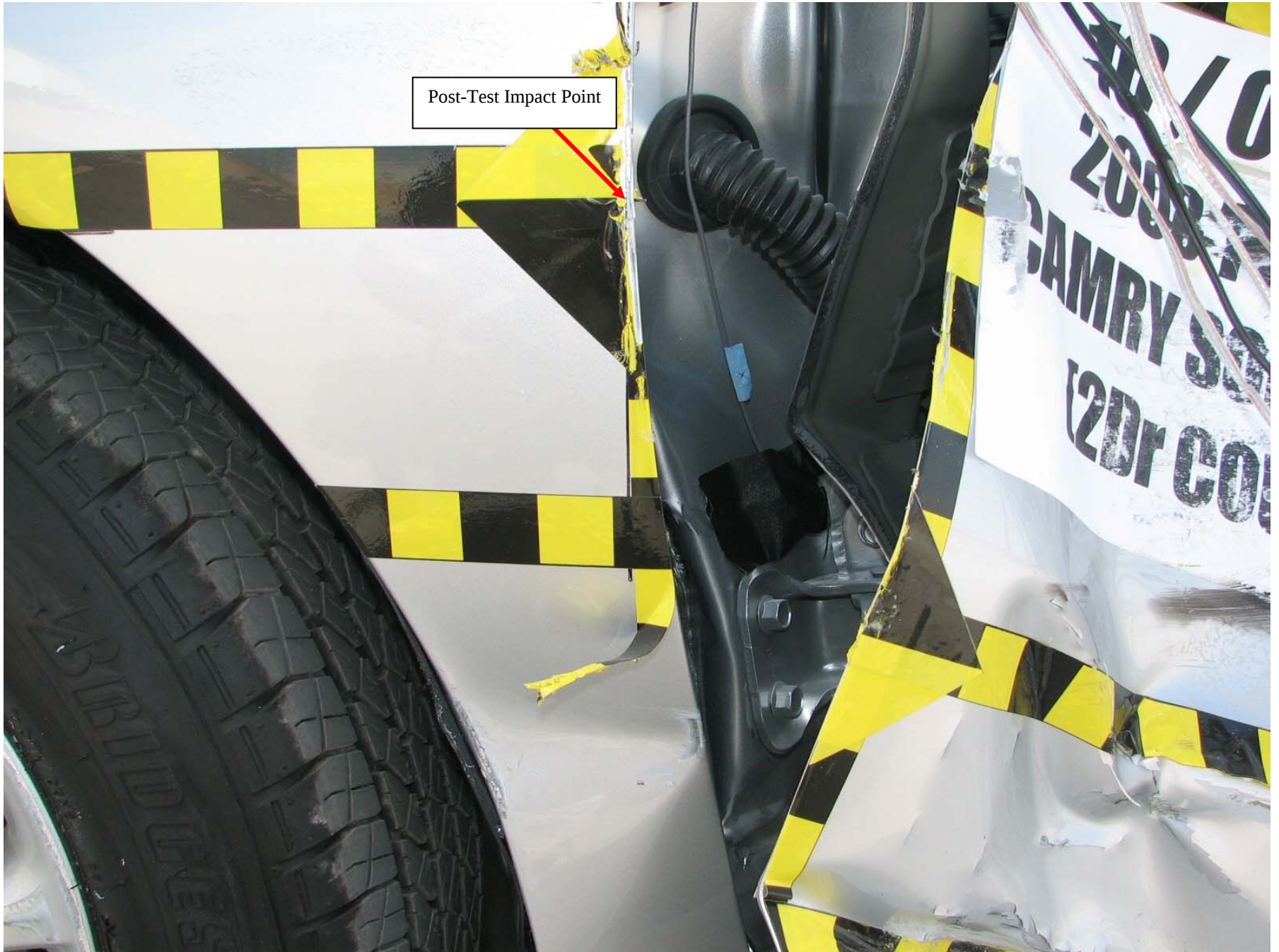
Figure A-26: Post-Test Left Impact Point
