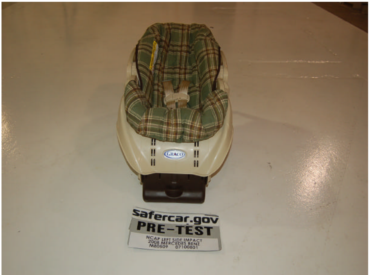
Pre-Test Front View of Position 3 CRS
