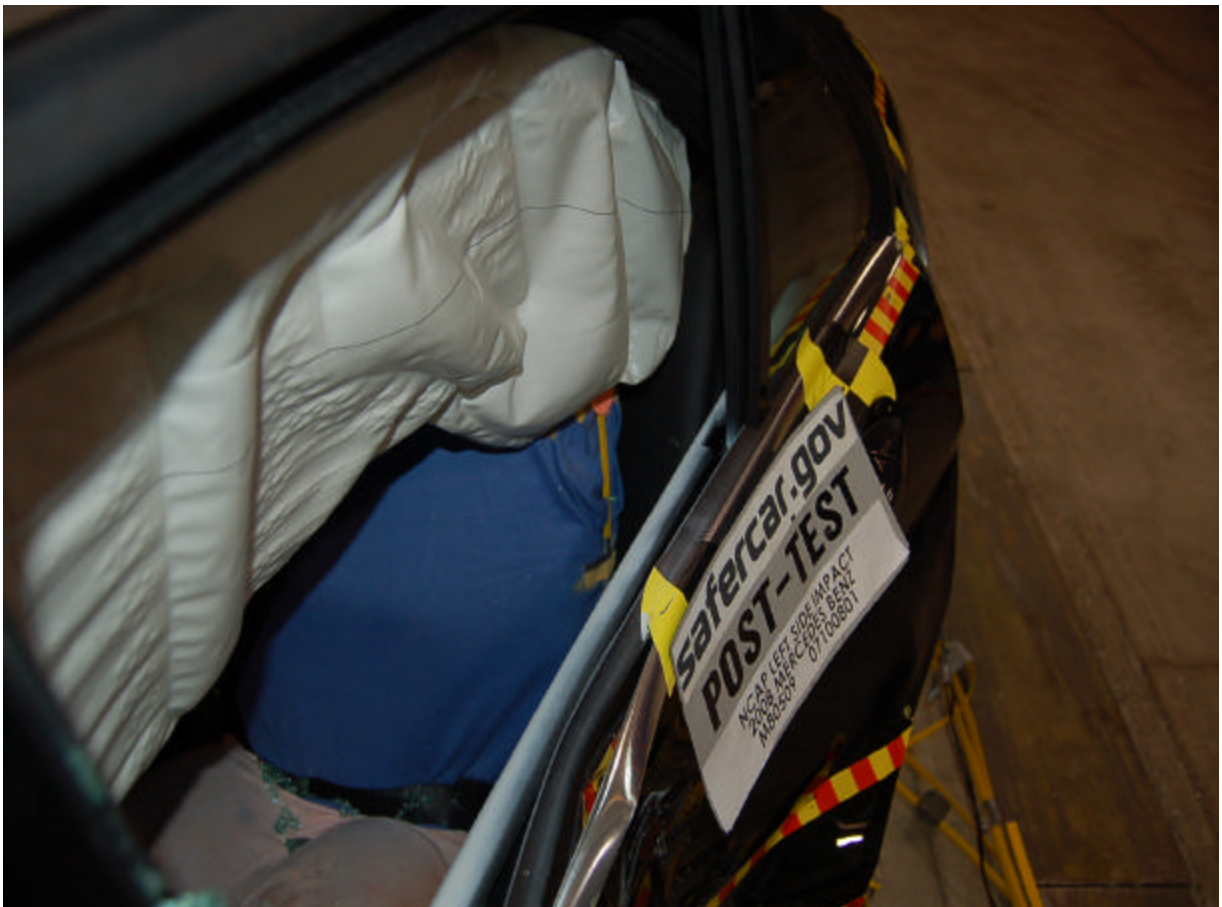
Post-Test Passenger Dummy Clearance From Door
