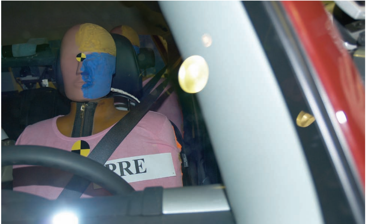
Figure A-37: Pre test driver shoulder clearance
