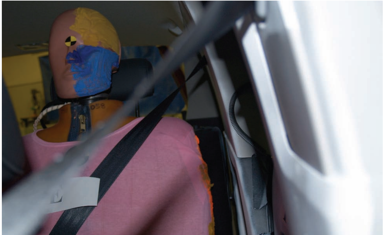
Figure A-45: Pre test passenger shoulder clearance
