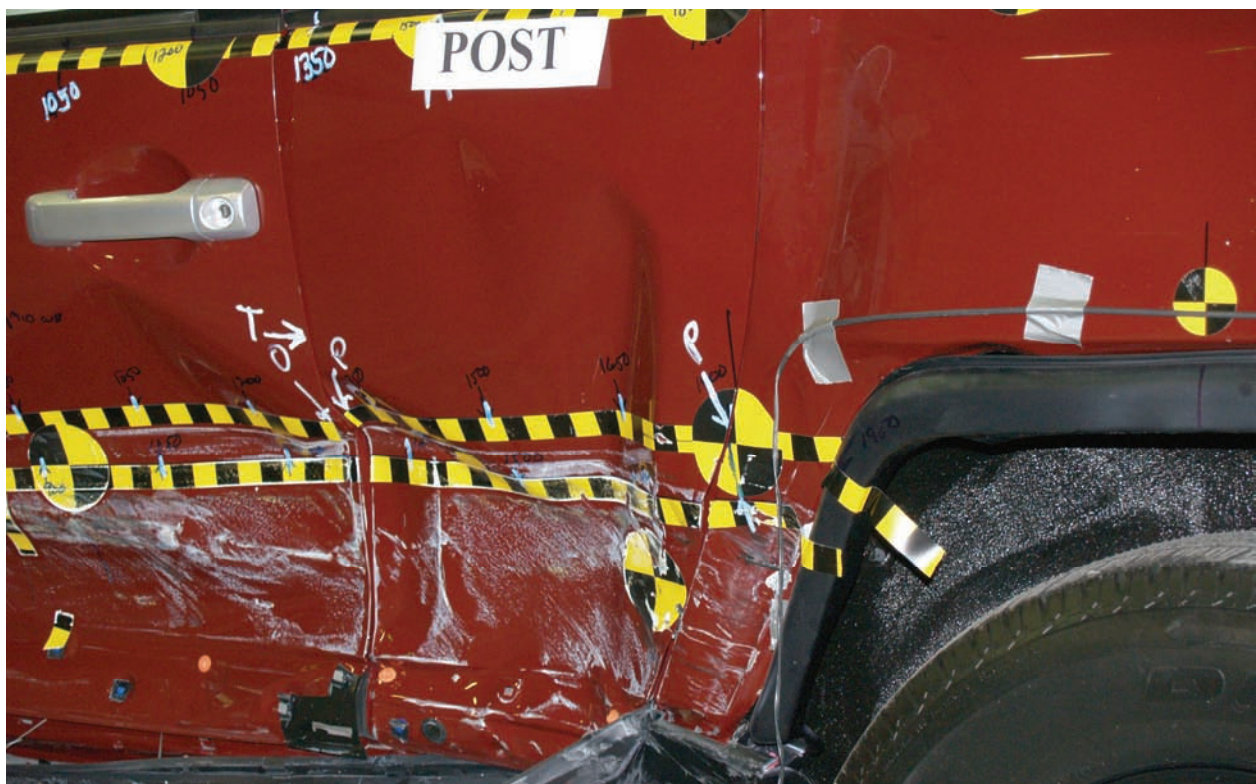
Figure A-34: Post test left rear door
