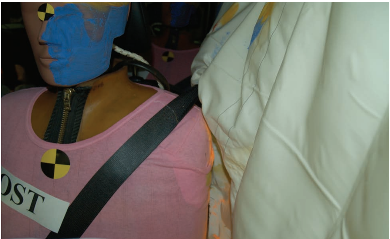
Figure A-38: Post test driver shoulder clearance
