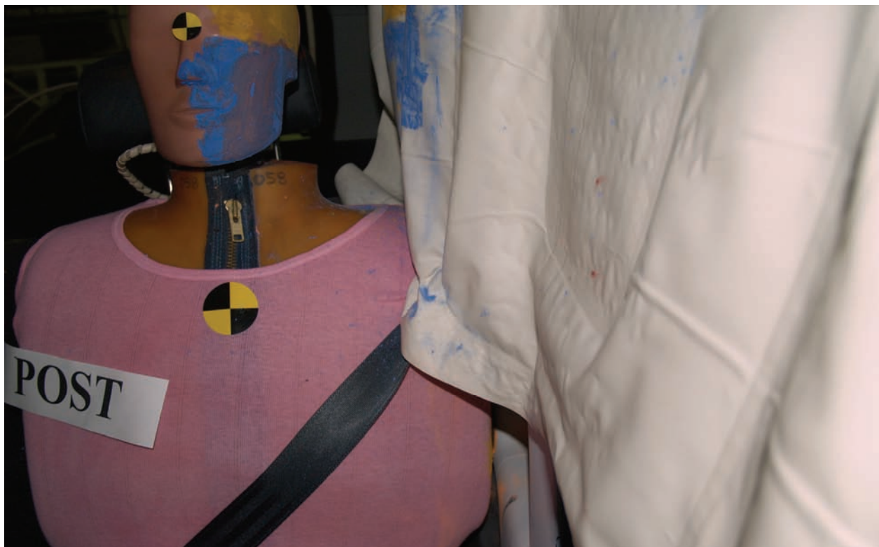
Figure A-46 Post test passenger shoulder clearance
