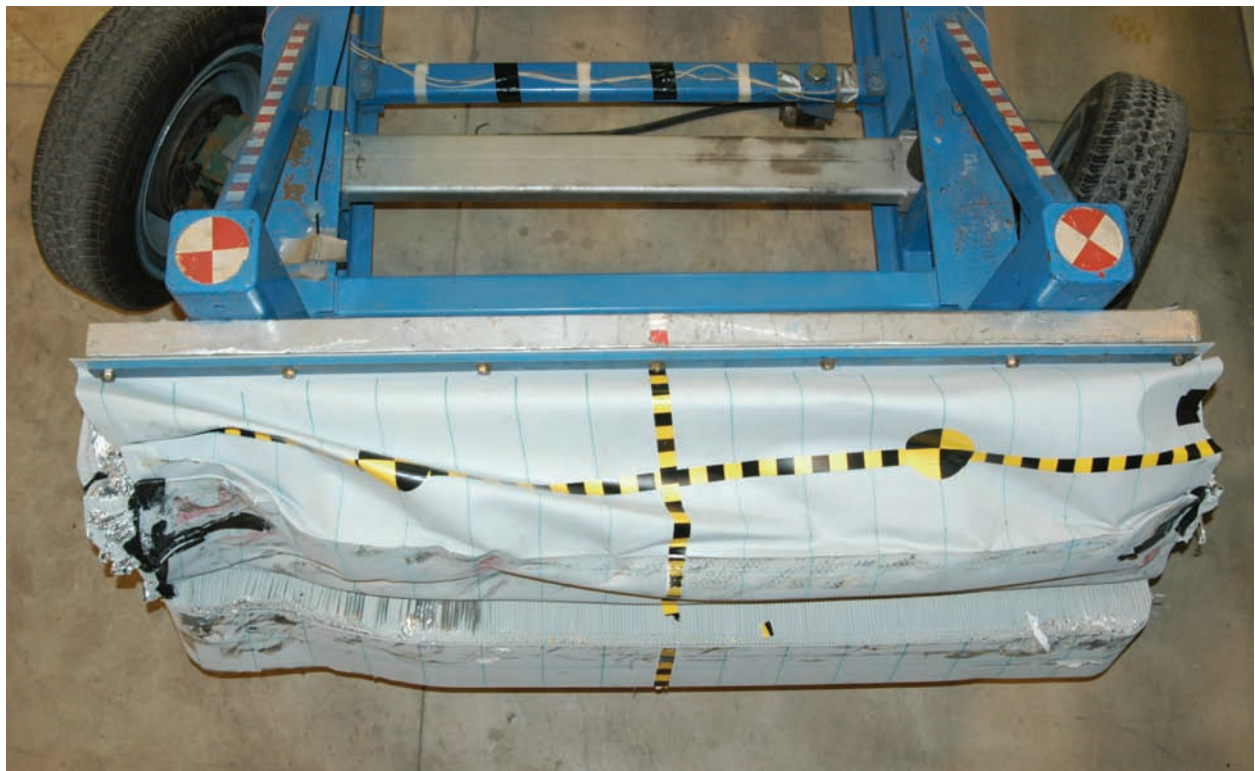
Figure A-54: Post test overhead view of MDB barrier face
