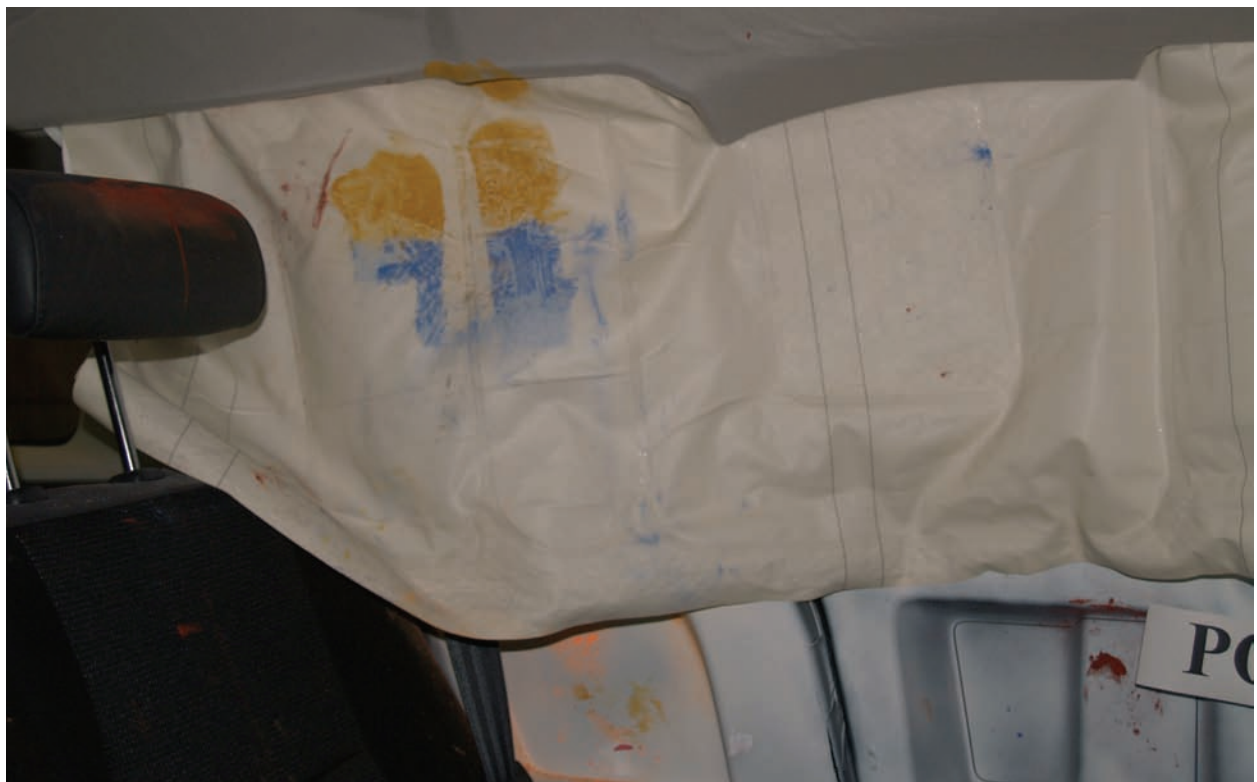
Figure A-50: Post test passenger contact locations (2)
