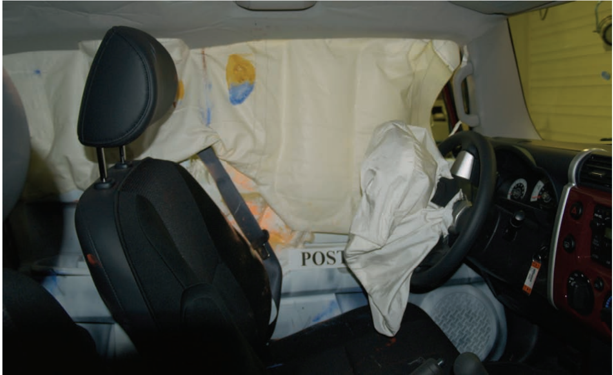
Figure A-41: Post test driver contact locations (1)
