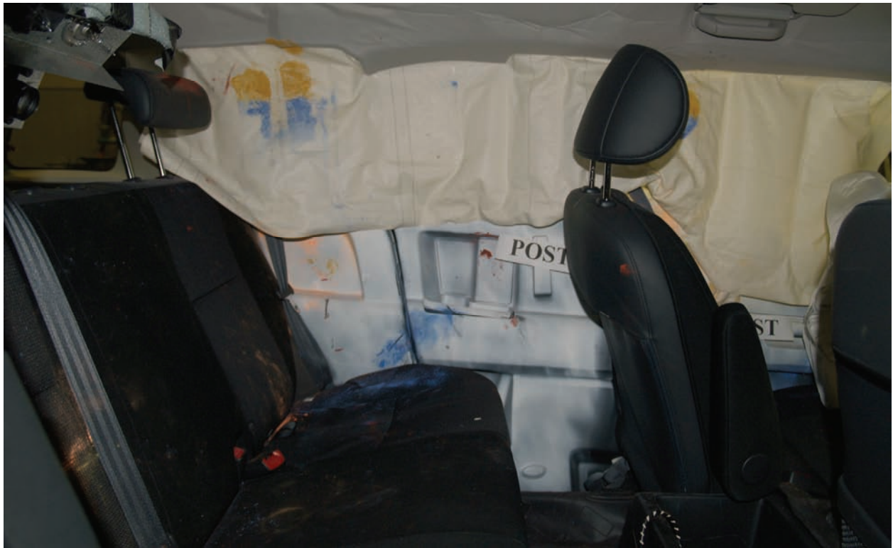
Figure A-49: Post test passenger contact locations (1)
