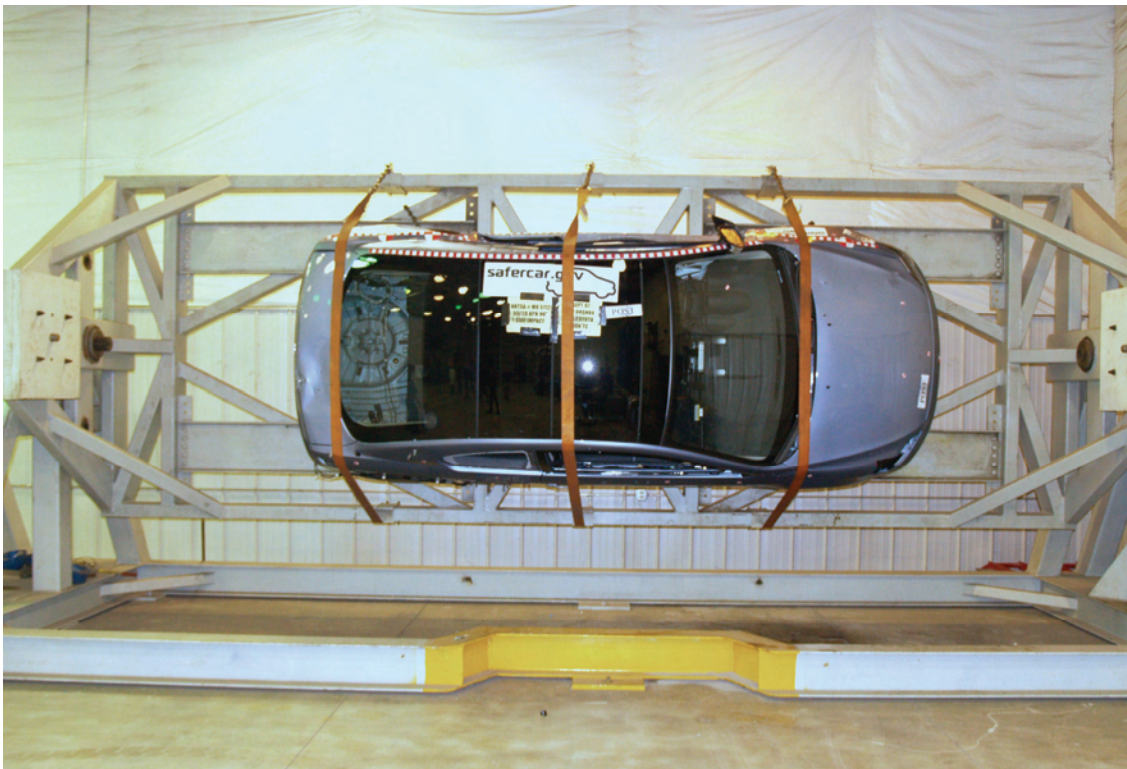
Figure A-60: FMVSS 301 270 degrees
