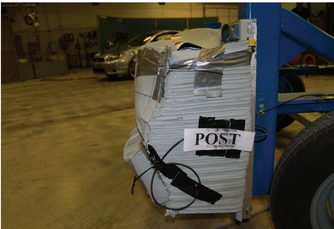
Figure A-56: Post test left side view of MDB barrier face
