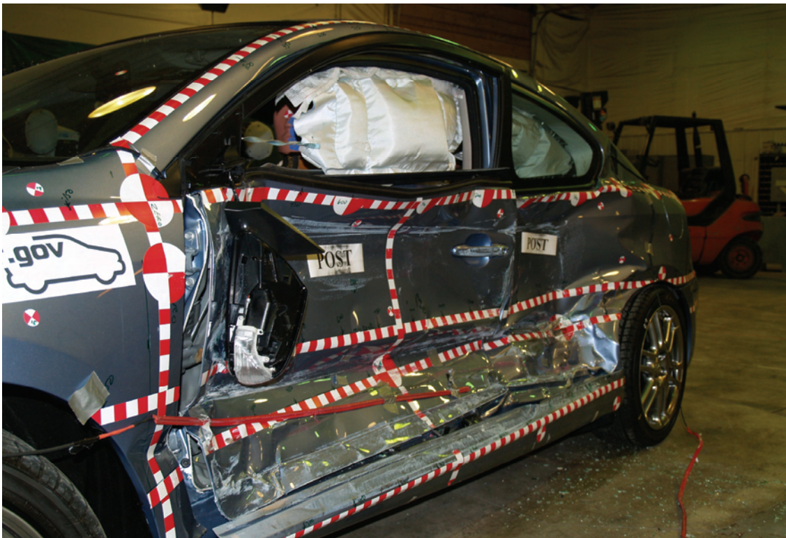
Figure A-28: Post test front 3/4 view of left side doors
