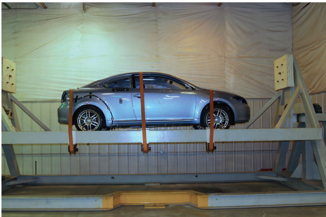
Figure A-61: FMVSS 301 360 degrees
