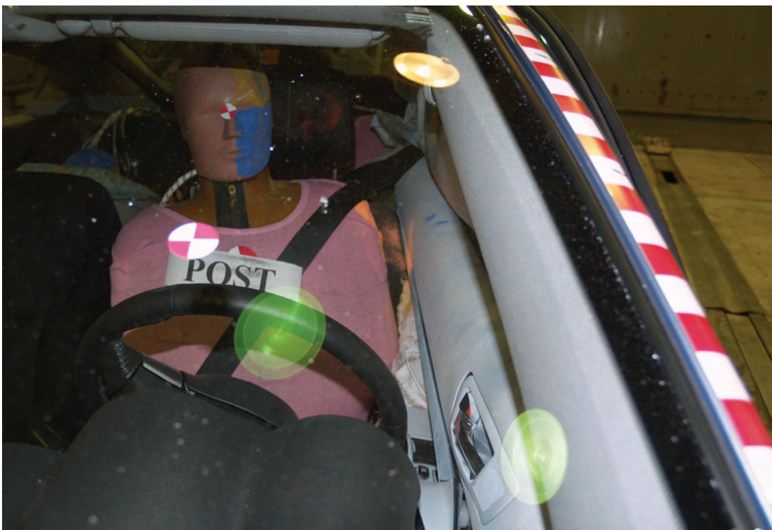
Figure A-36: Post test driver shoulder clearance
