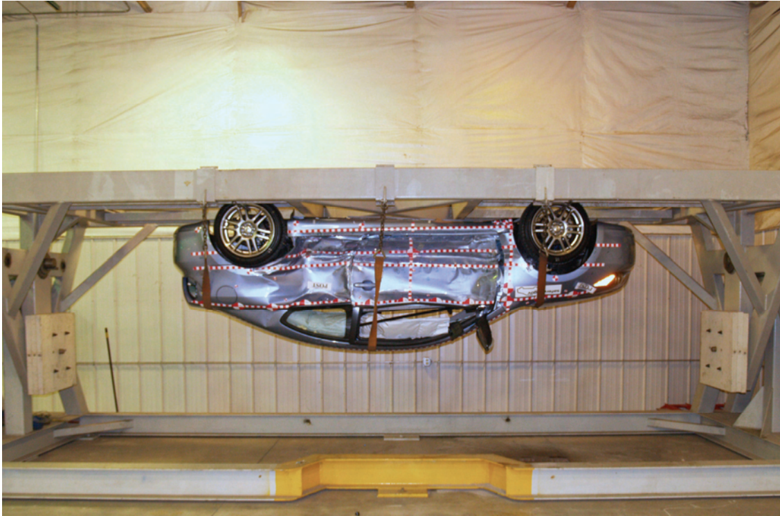
Figure A-59: FMVSS 301 180 degrees
