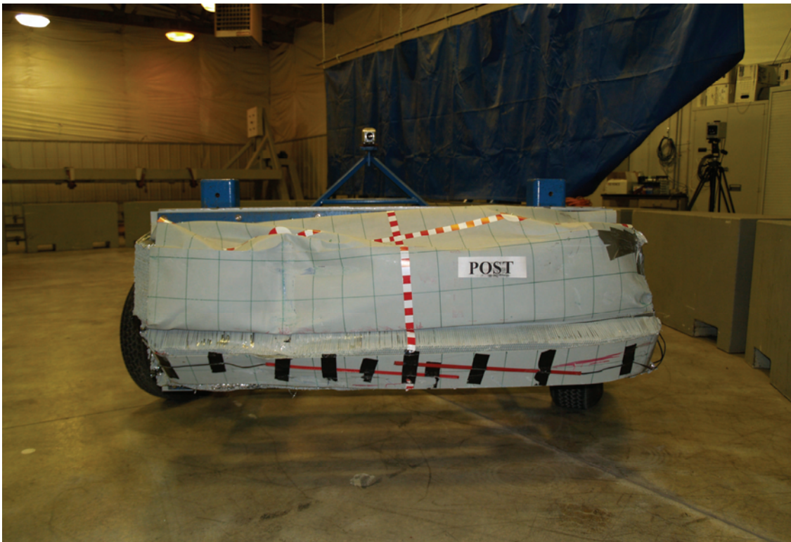
Figure A-50: Post test front view of MDB barrier face
