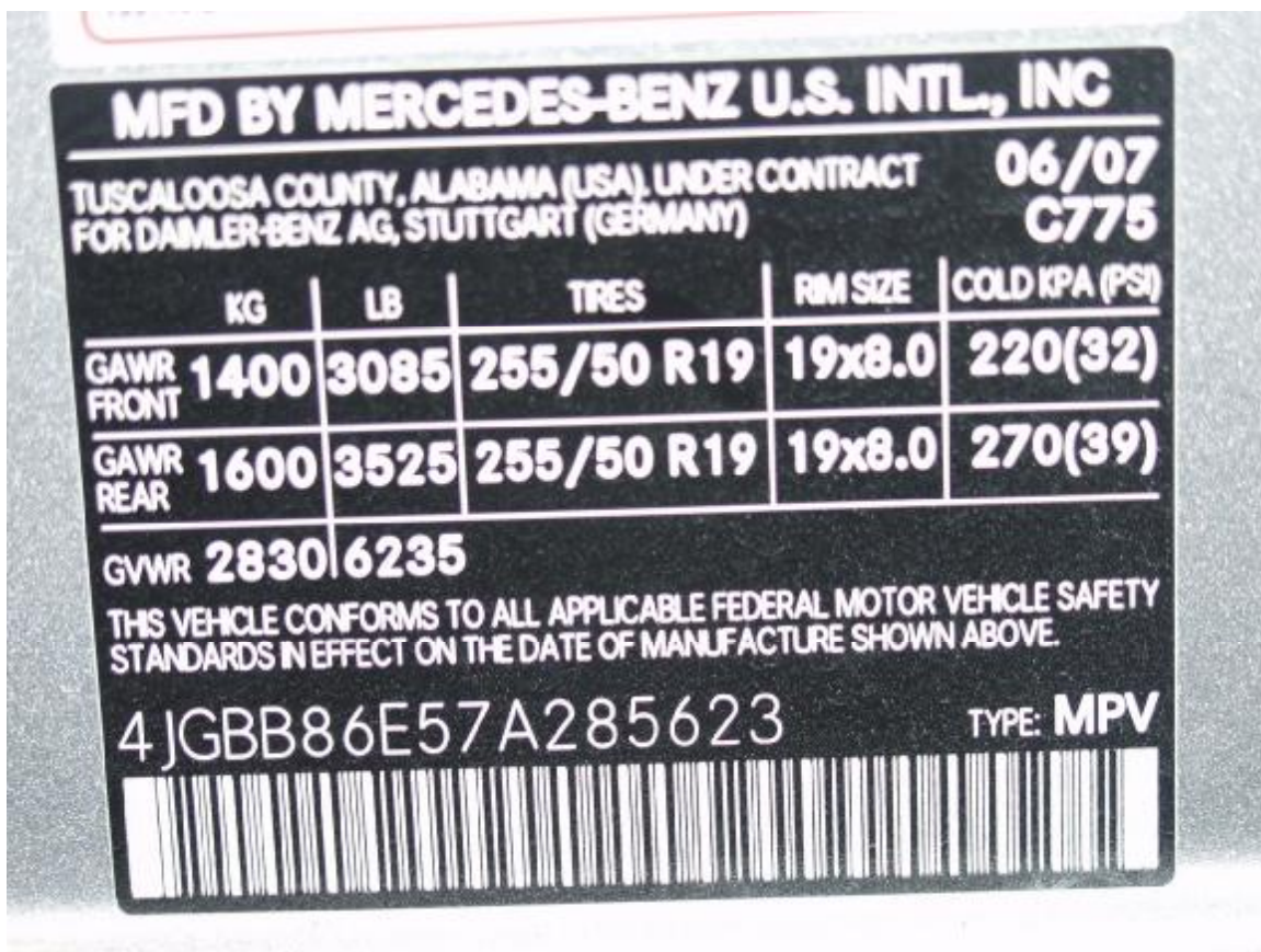
Figure A-3: Vehicle Certification Label
