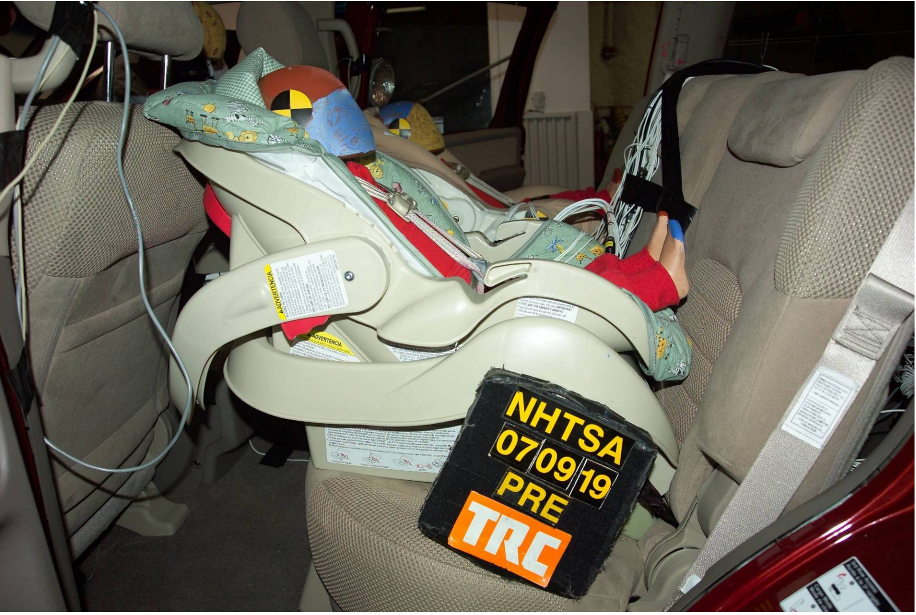
Figure D2-13 Pre-Test Left View of Left Rear Dummy
