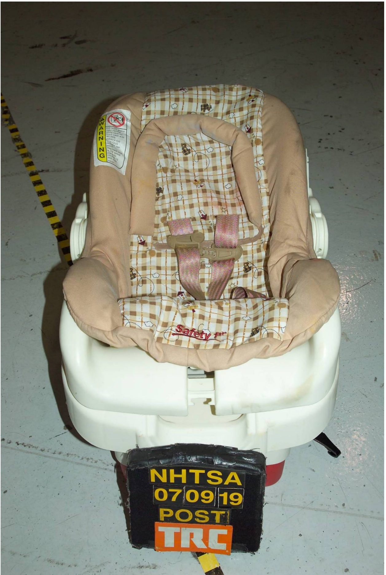
Figure D2-23 Post-Test Front View of Right Rear CRS
