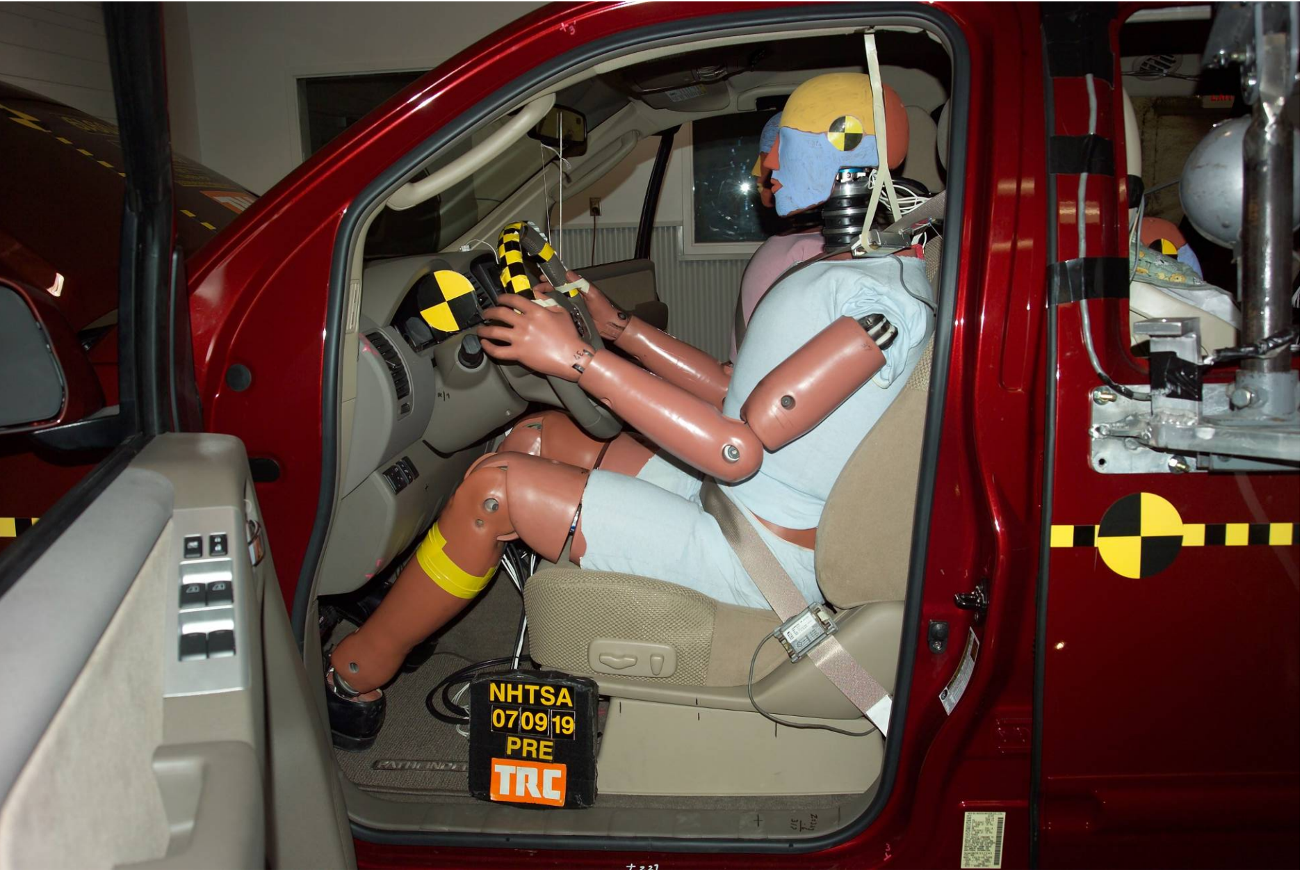
Figure A-43 Pre-Test Driver Dummy - View 3
