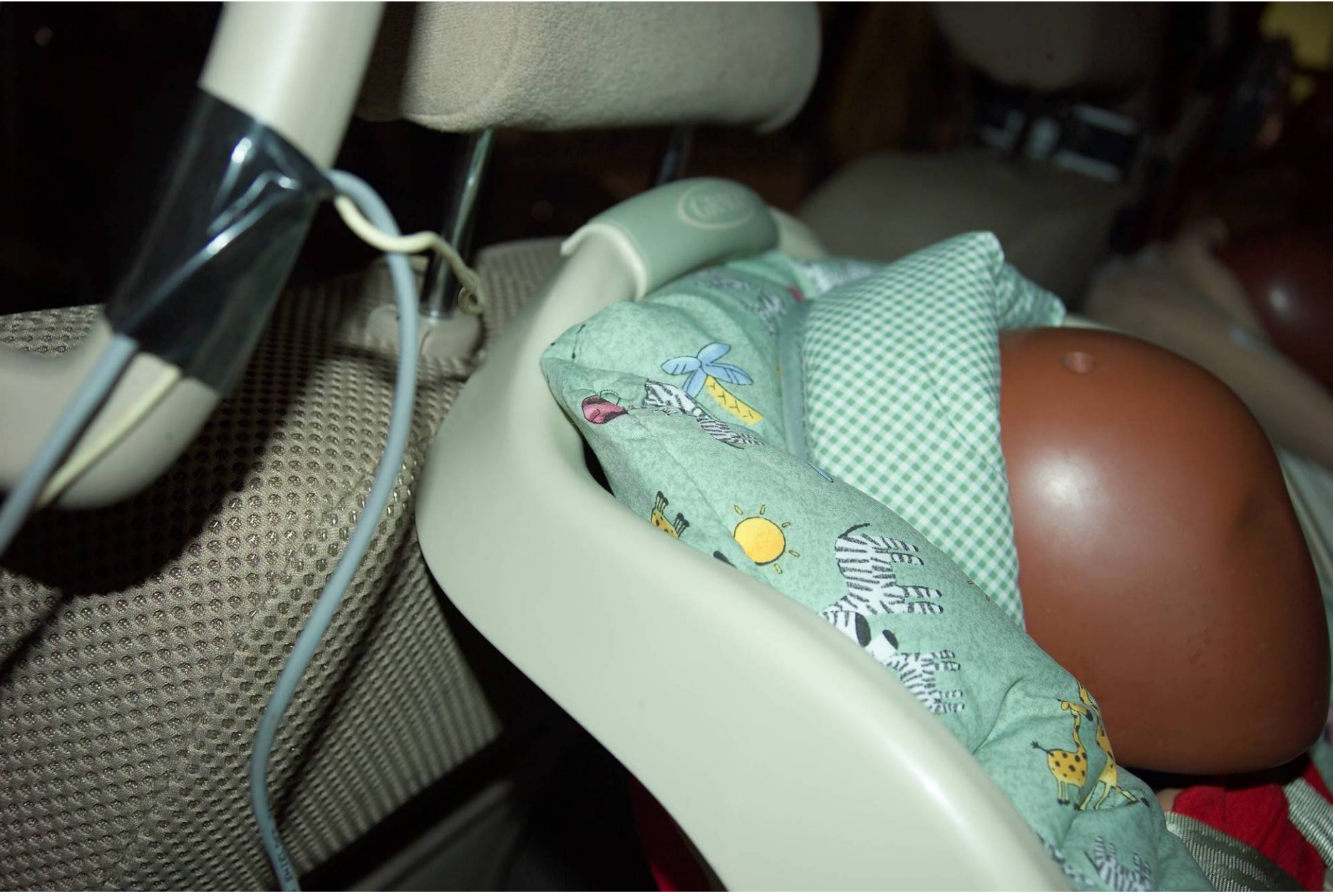
Figure D2-18 Pre-Test Left Rear CRS Intrusion into Driver Seat - View 2
