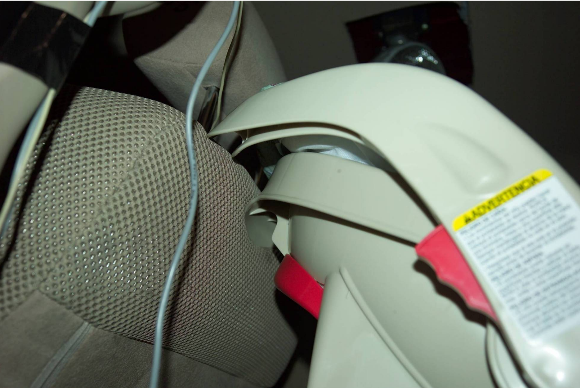
Figure D2-17 Pre-Test Left Rear CRIS Intrusion into Driver Seat - View 1
