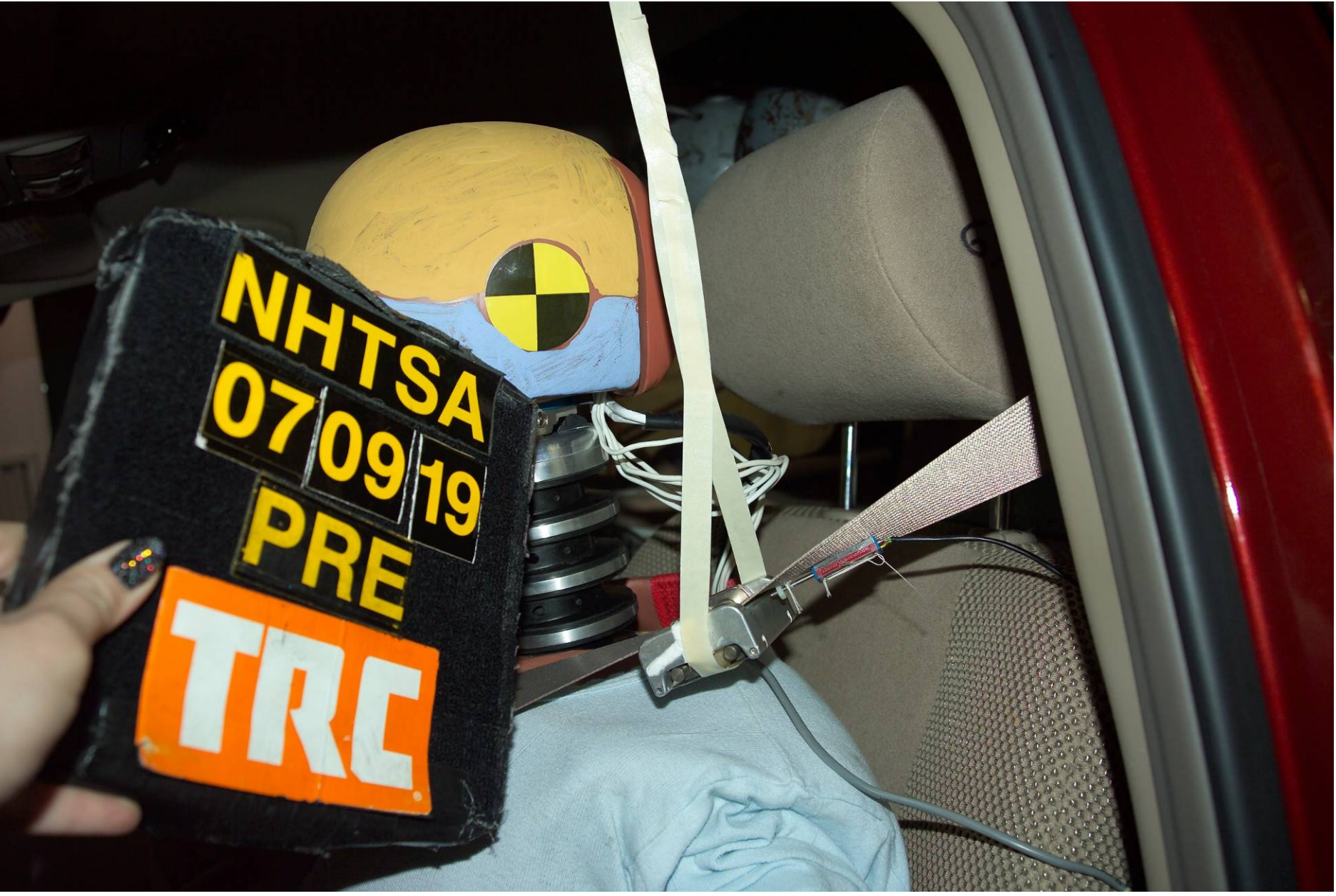
Figure A-51 Pre-Test Driver Dummy Head Position View
