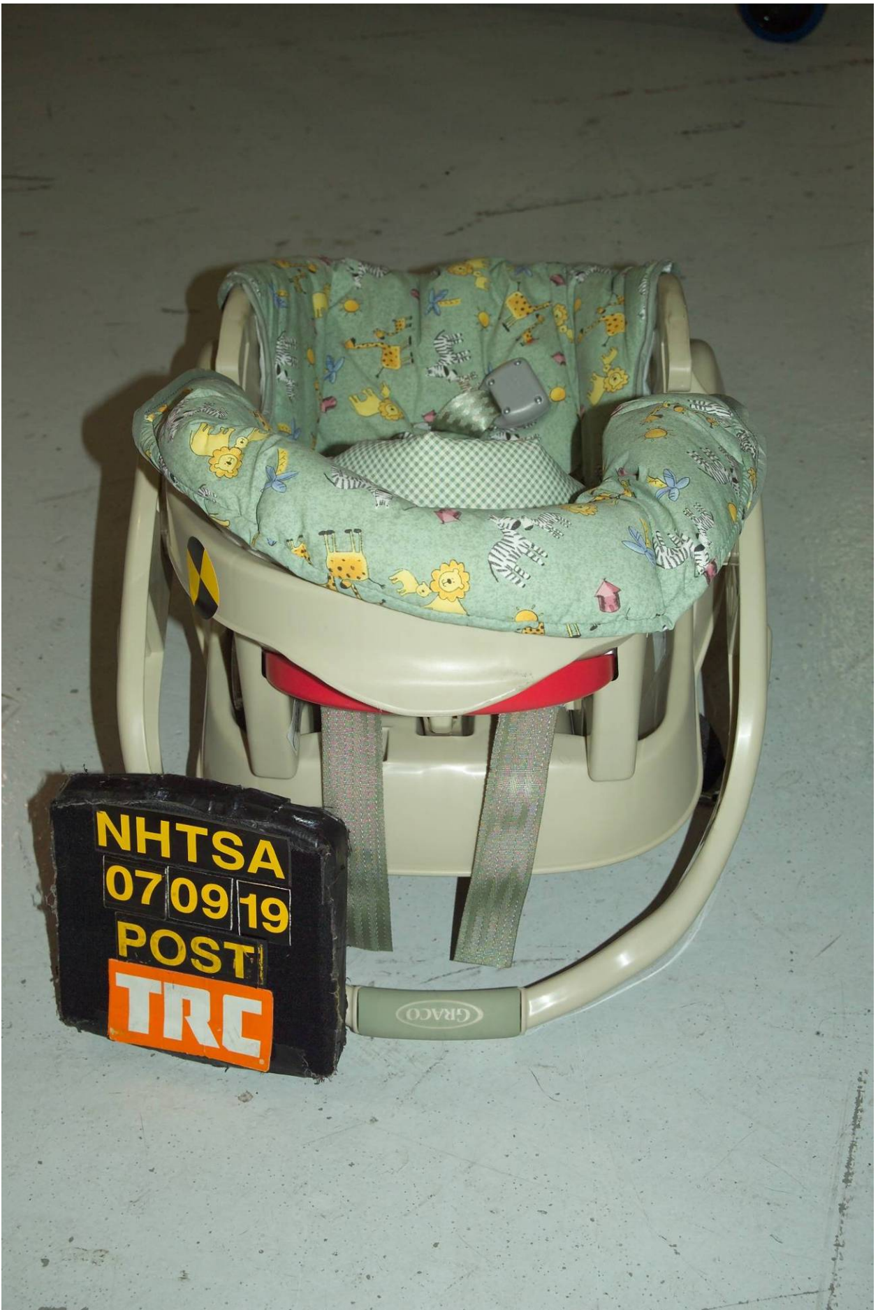
Figure D2-6 Post-Test Rear View of Left Rear CRS
