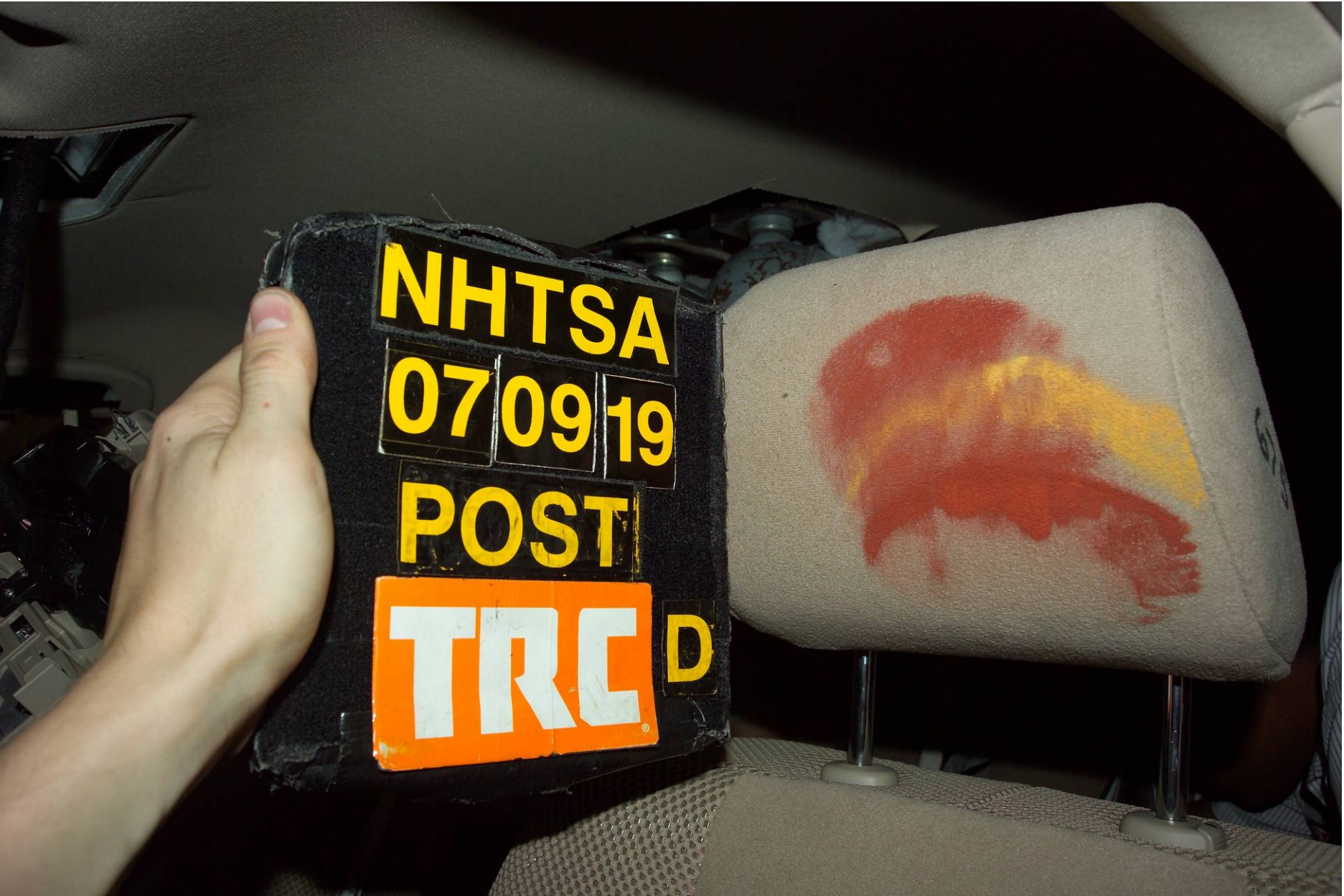
Figure A-56 Post-Test Driver Dummy Head Contact - View 2
