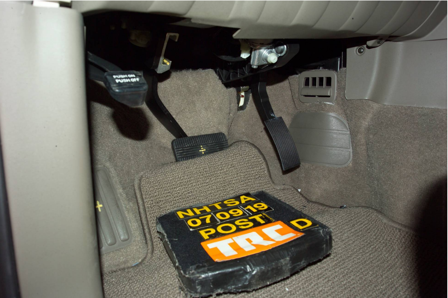
Figure A-58 Post-Test Driver Toeboard Deformation View
