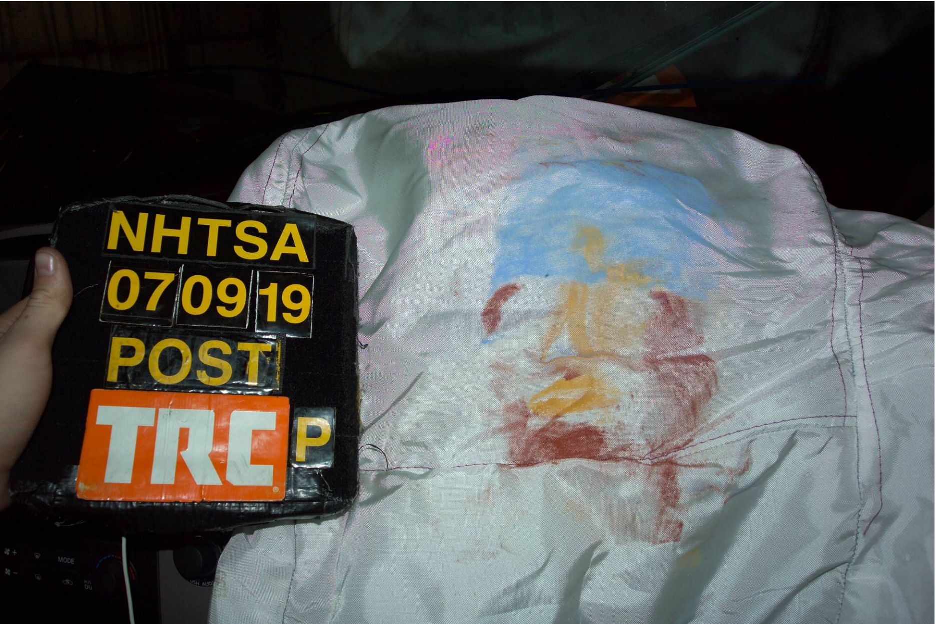
Figure A-74 Post-Test Right Front Passenger Dummy Head Contact - View 1
