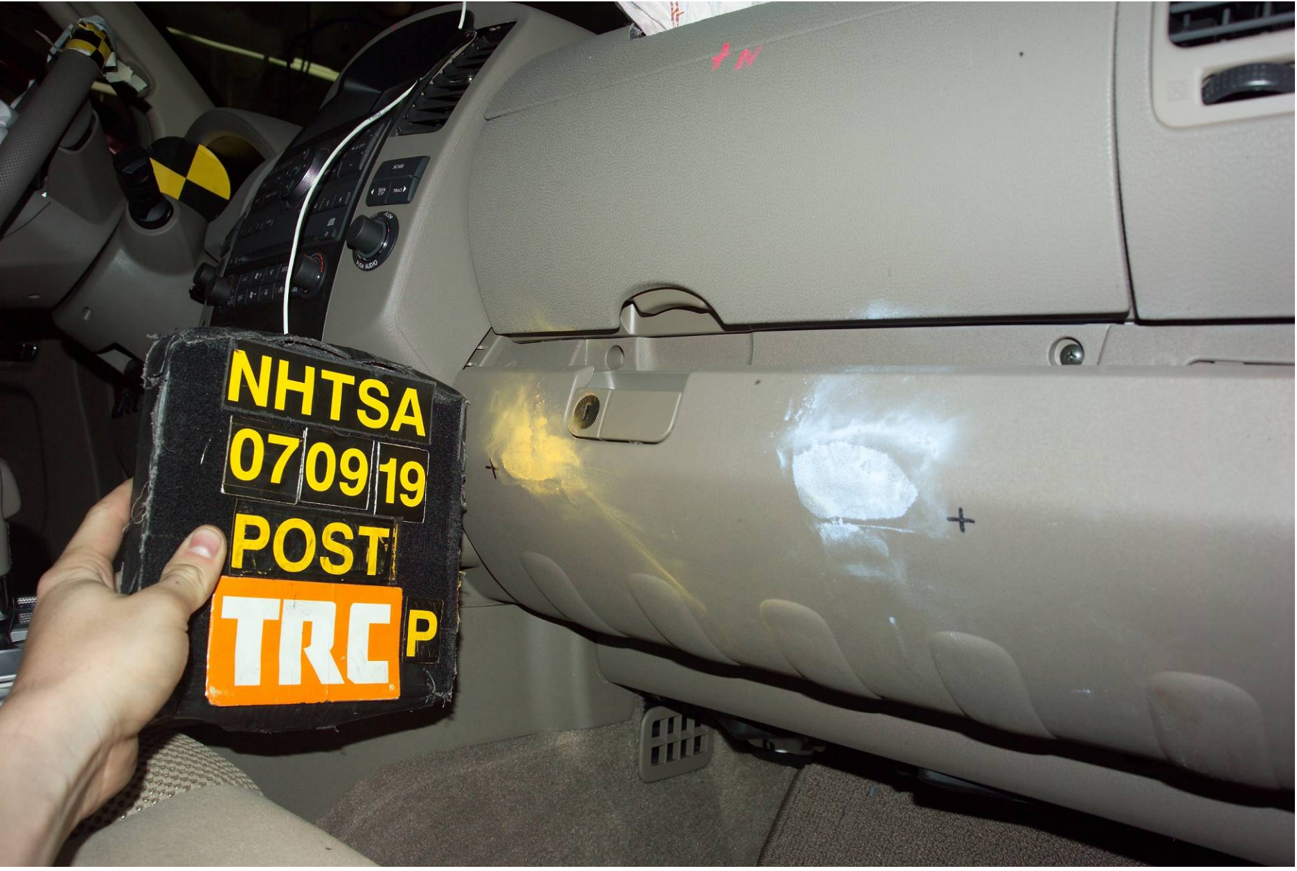
Figure A-76 Post-Test Right Front Passenger Dummy Knee Contact View
