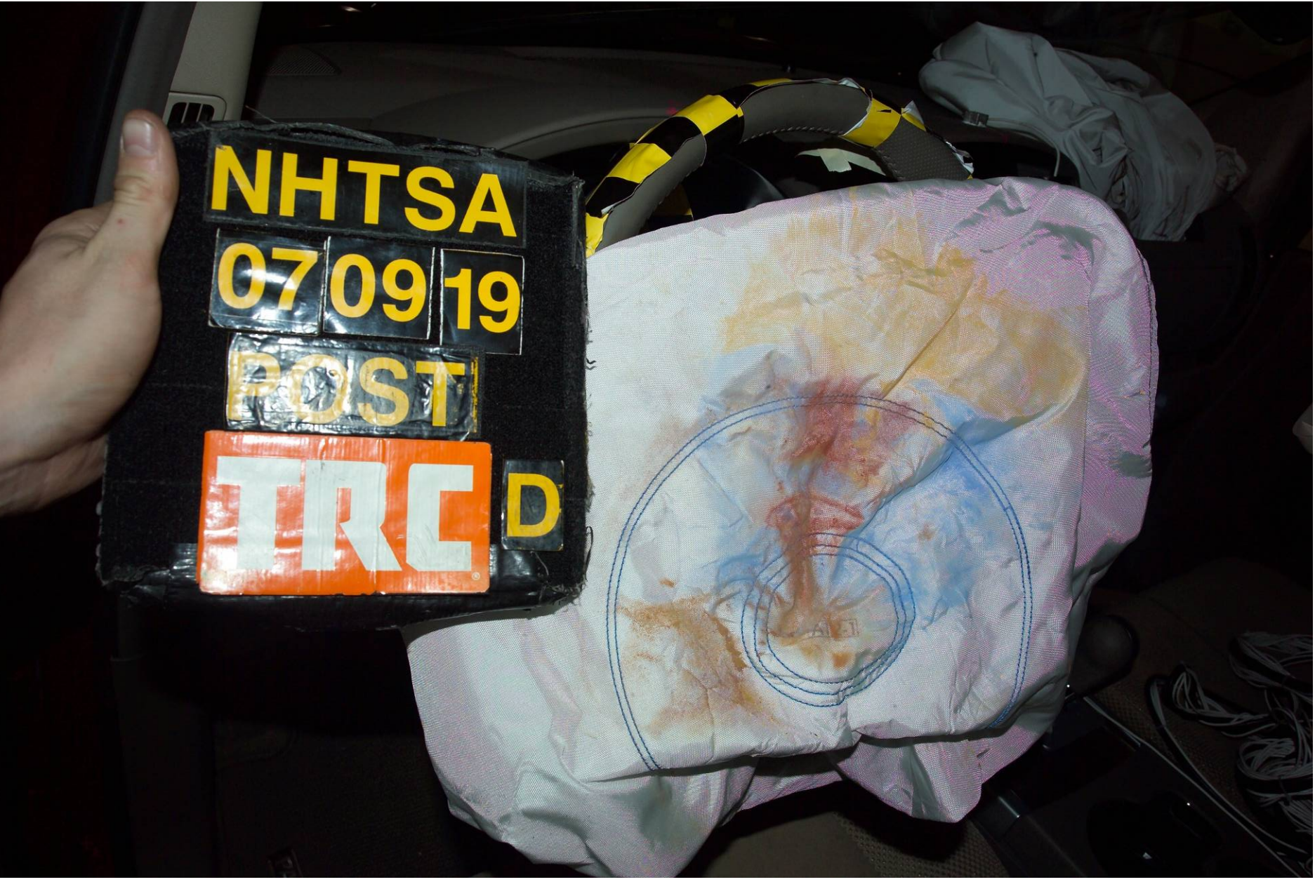
Figure A-55 Post-Test Driver Dummy Head Contact - View 1
