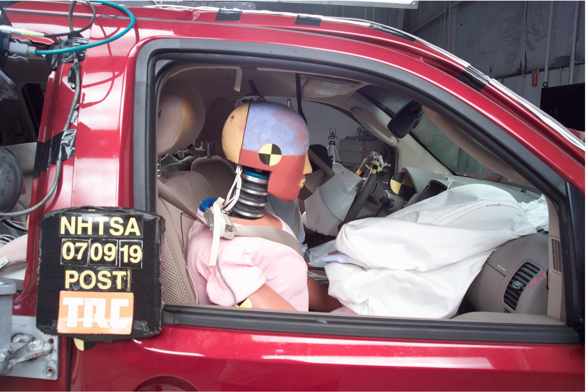
Figure A-62 Post-Test Right Front Passenger Dummy - View 2
