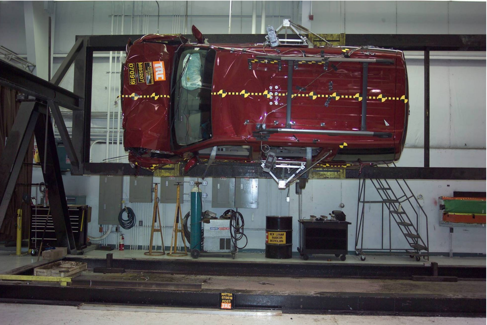
Figure A-82 FMVSS 301 Rollover View at 90°
