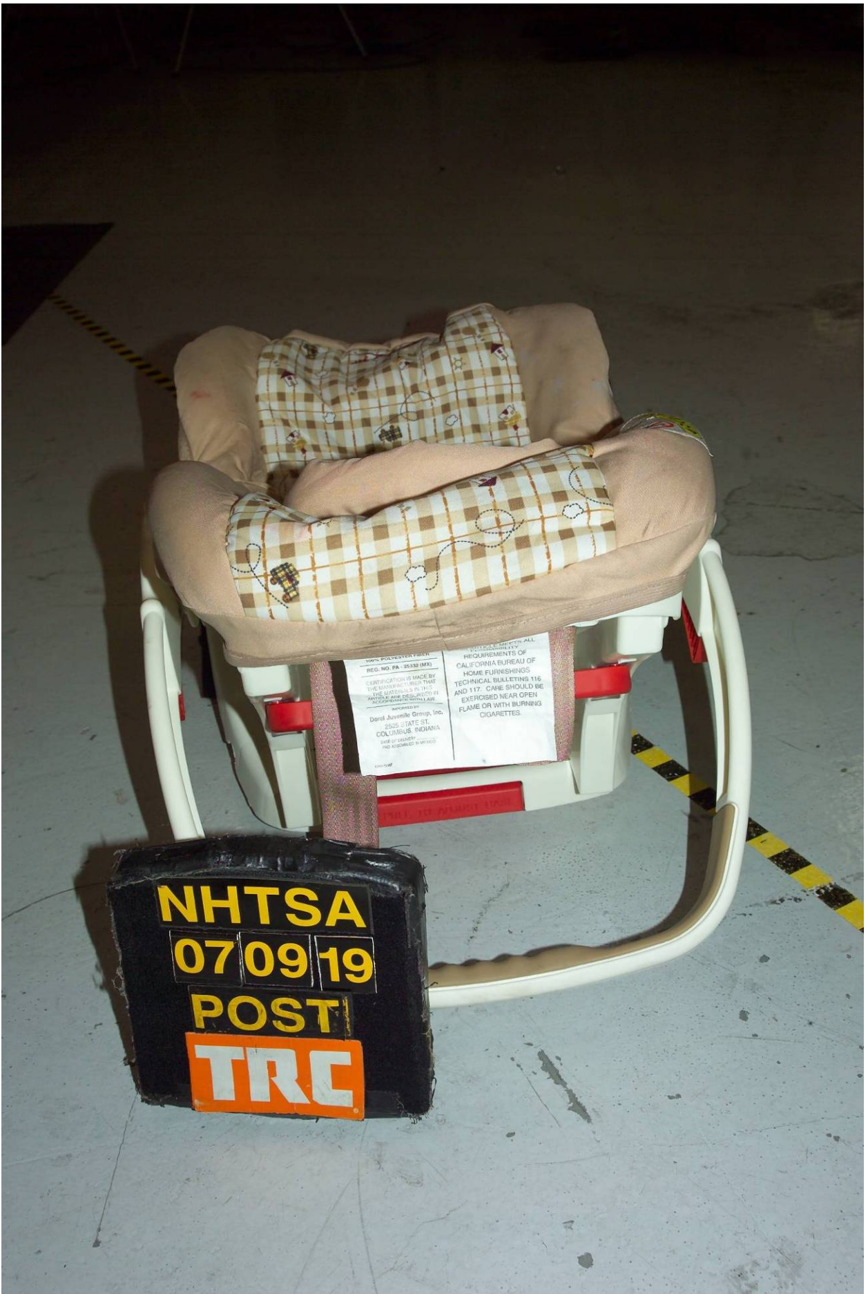
Figure D2-25 Post-Test Rear View of Right Rear CRS
