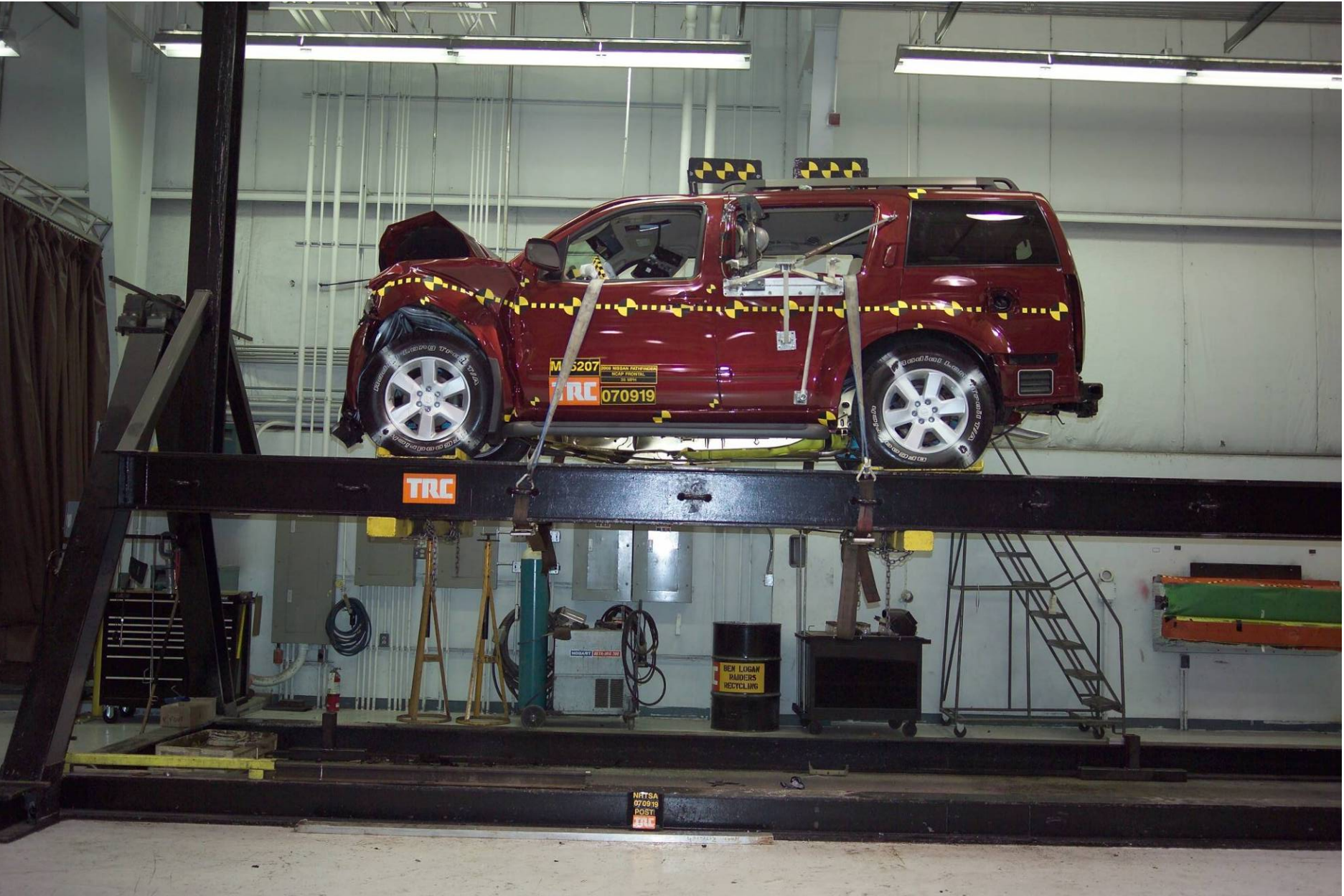
Figure A-85 FMVSS 301 Rollover View at 360°
