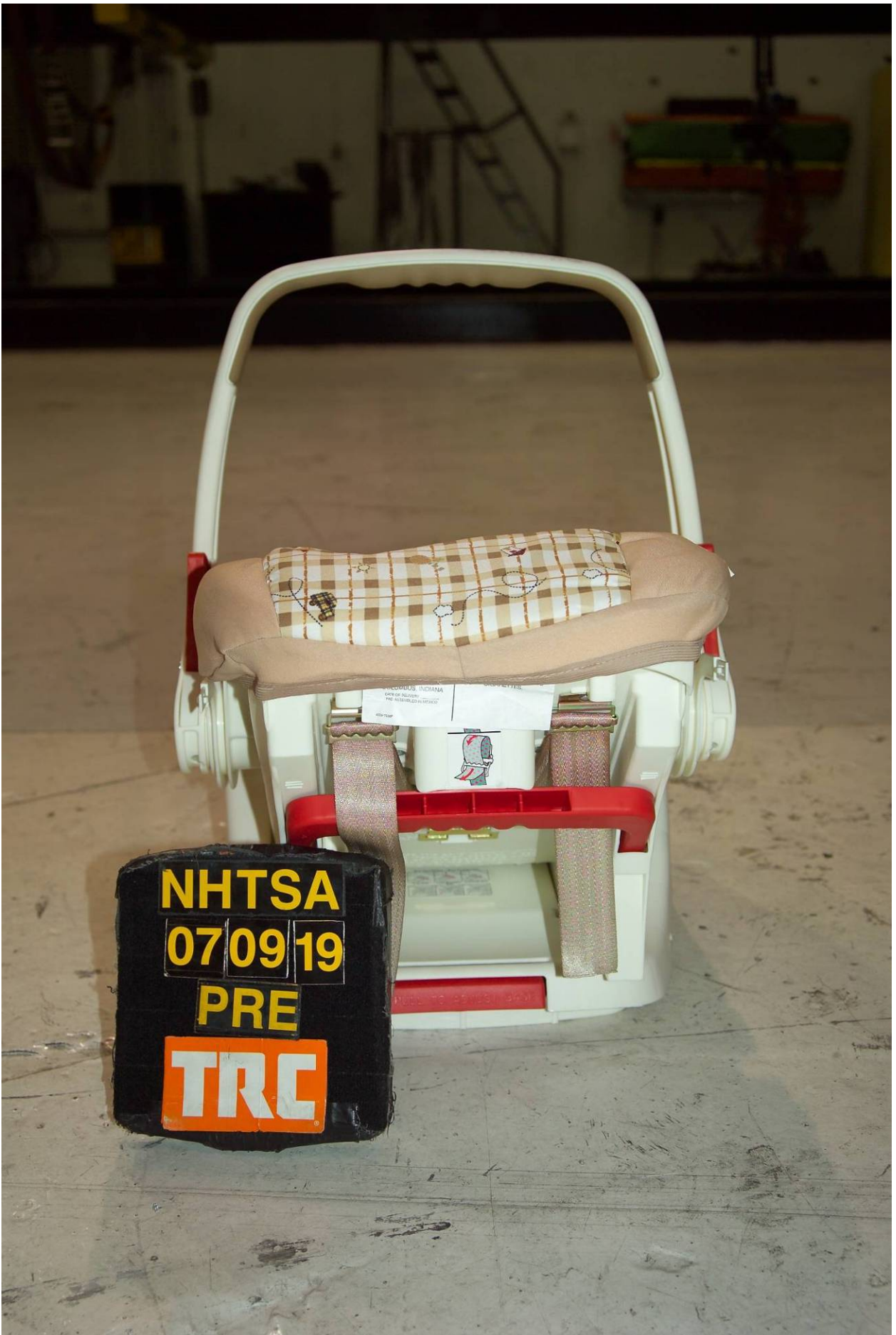
Figure D2-24 Pre-Test Rear View of Right Rear CRS
