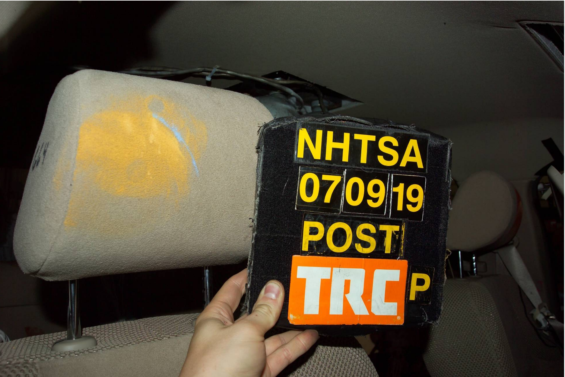
Figure A-75 Post-Test Right Front Passenger Dummy Head Contact - View 2
