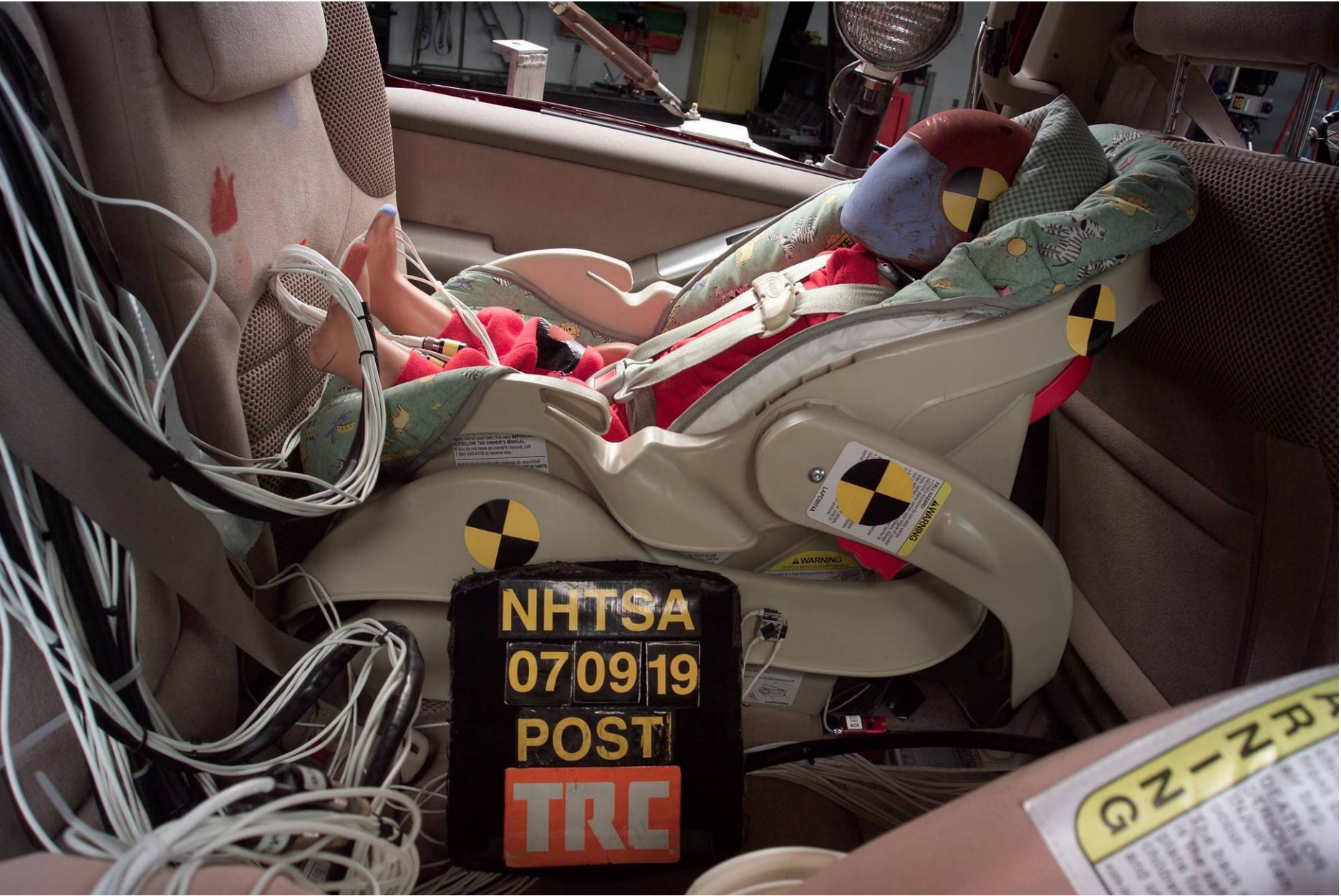
Figure D2-16 Post-Test Right View of Left Rear Dummy
