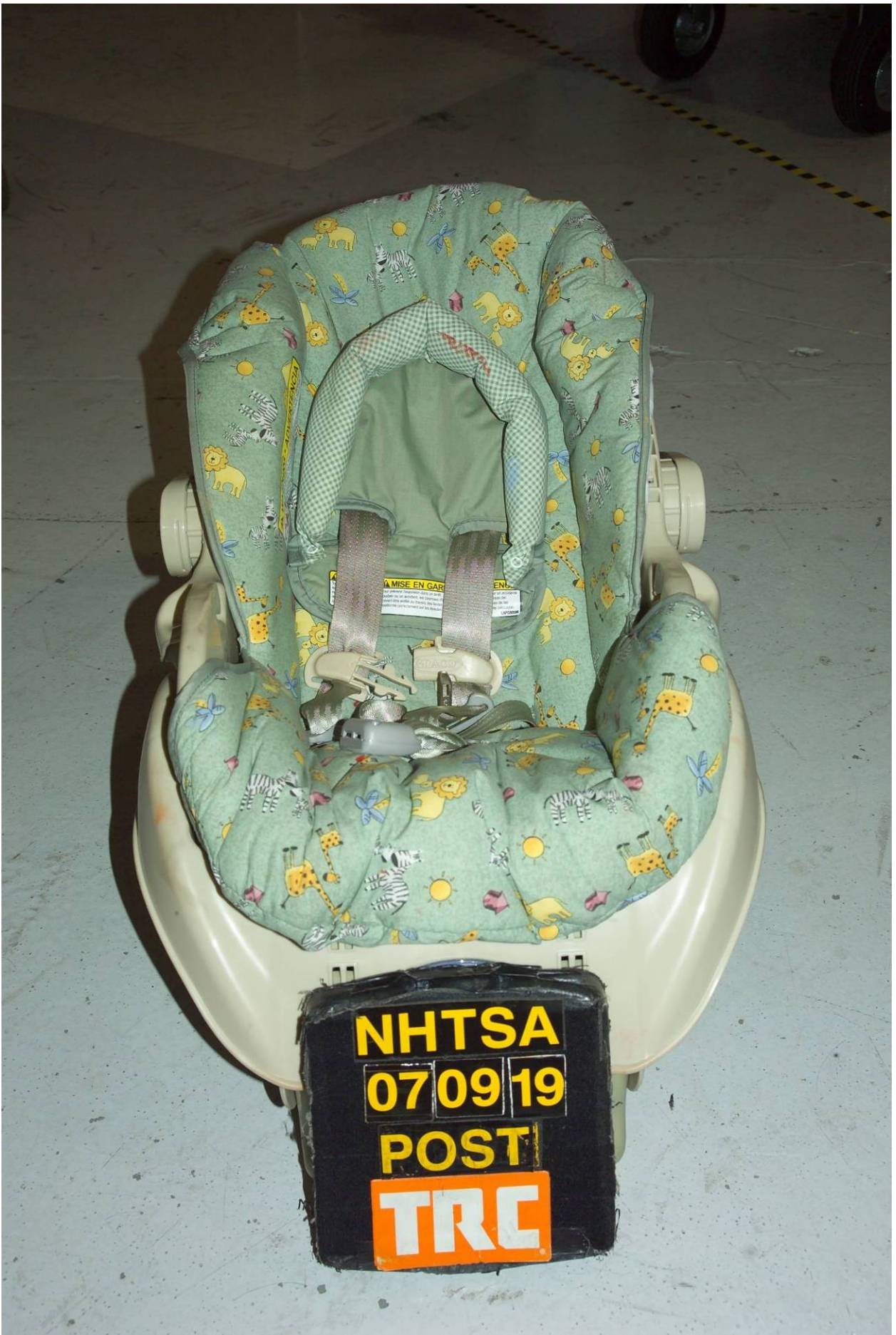
Figure D2-4 Post-Test Front View of Left Rear CRS
