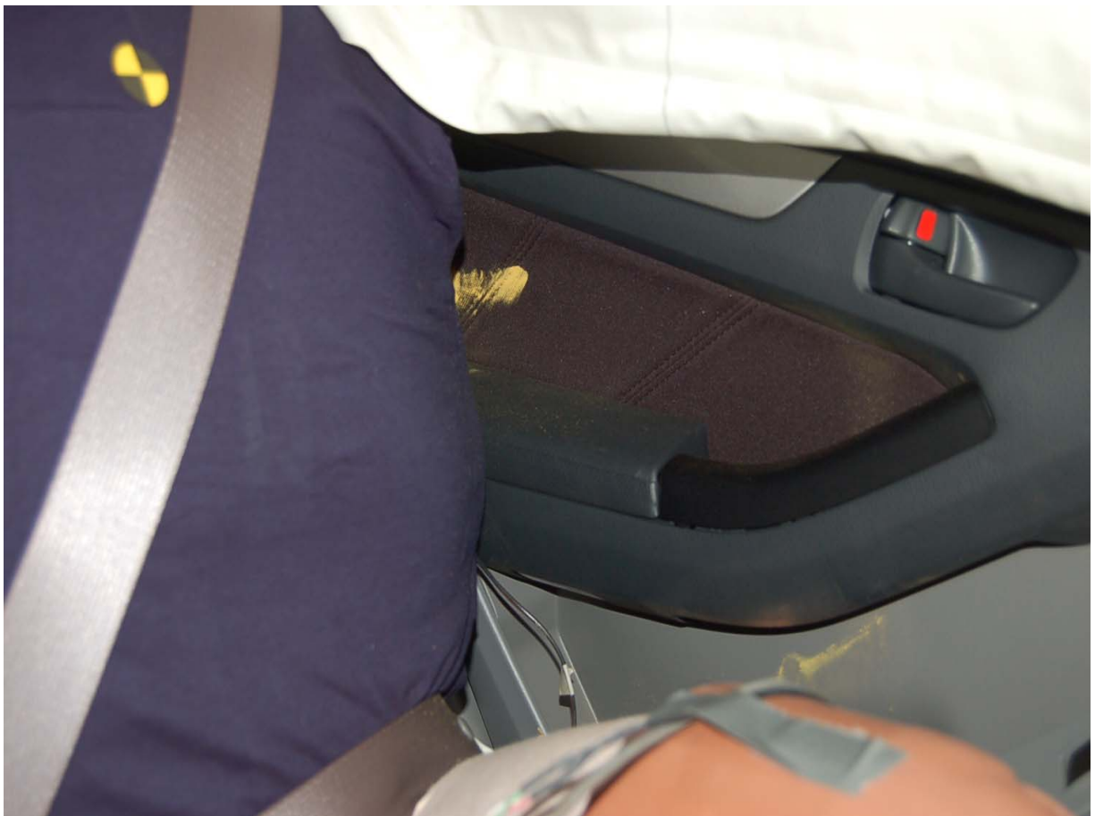
Post-Test Passenger Dummy Torso Contact
