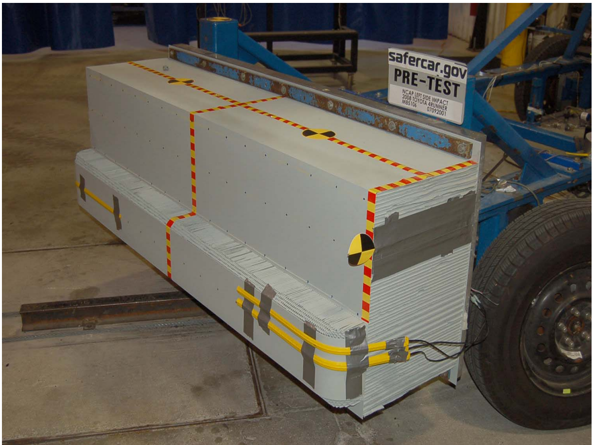
Pre-Test Left Side View of Deformable Barrier
