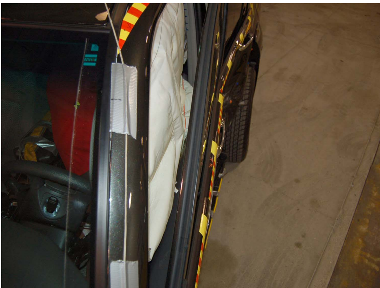
Post-Test Driver Dummy Clearance From Door
