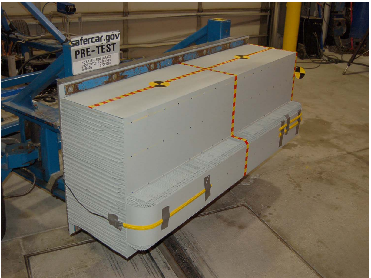
Pre-Test Right Side View of Deformable Barrier
