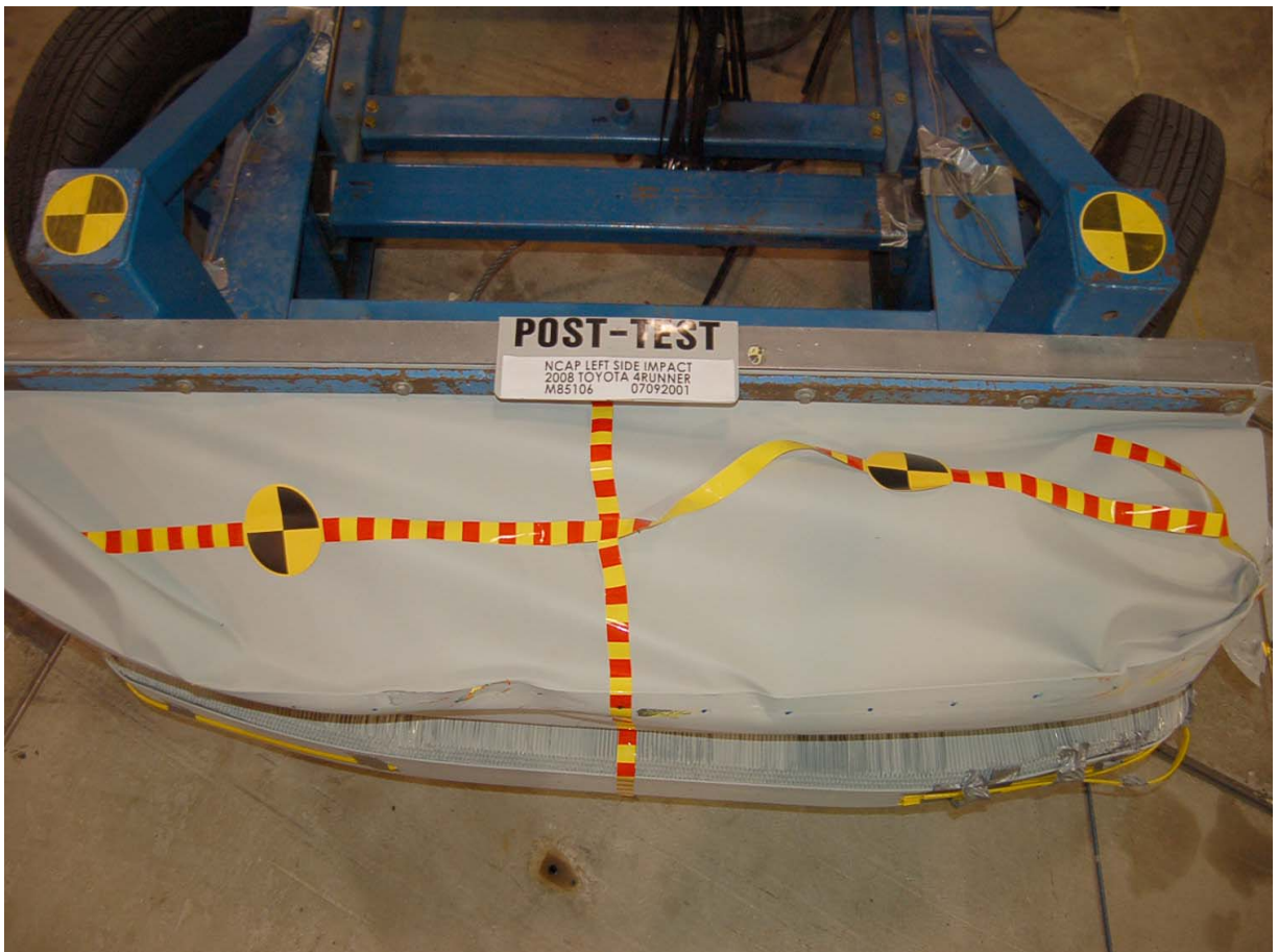
Post-Test Top View of Deformable Barrier
