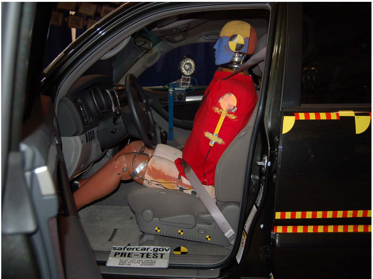
Pre-Test Driver Dummy (Door Open)
