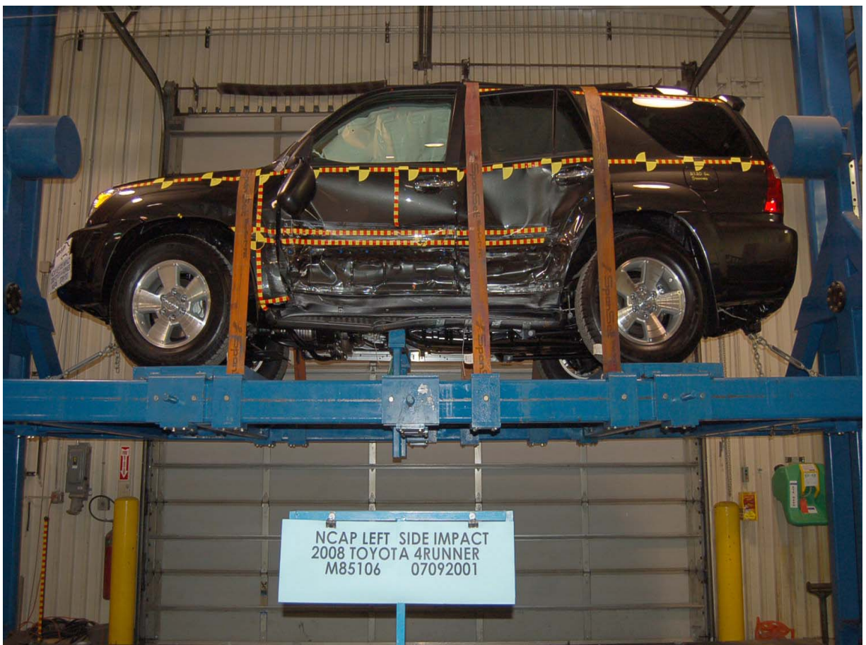
Vehicle on Rollover Device (360 Degrees)
