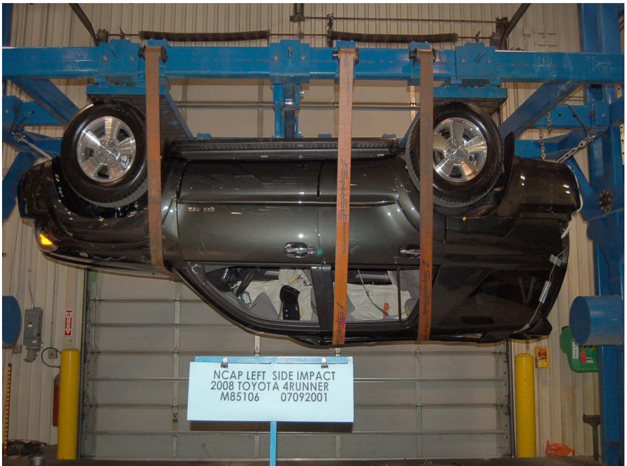
Vehicle on Rollover Device (180 Degrees)
