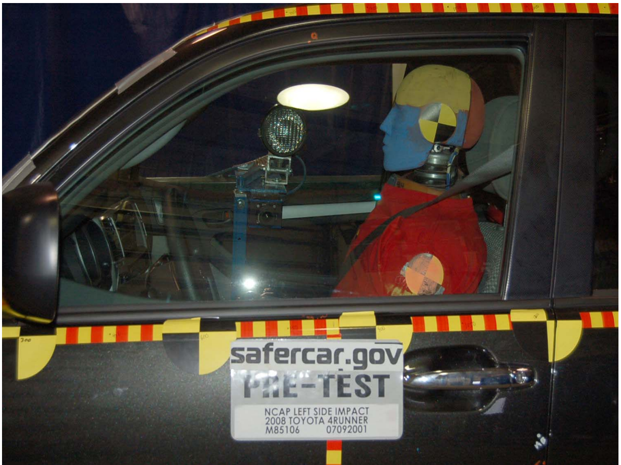
Pre-Test Driver Dummy (Through Window)
