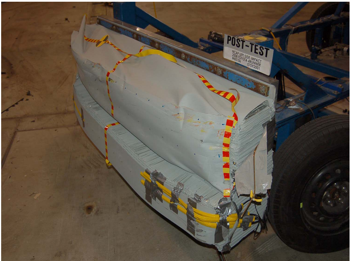
Post-Test Left Side View of Deformable Barrier
