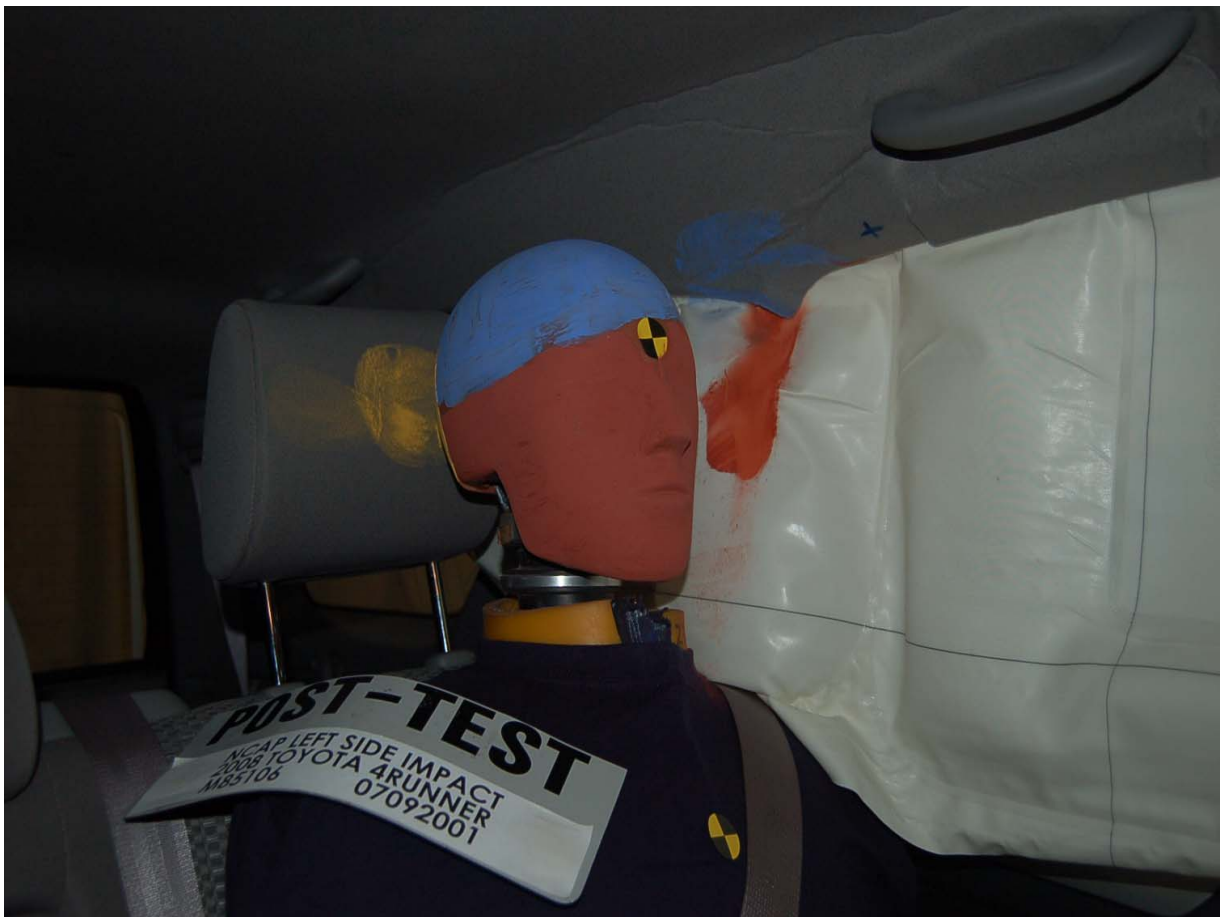
Post-Test Passenger Dummy Head Contact
