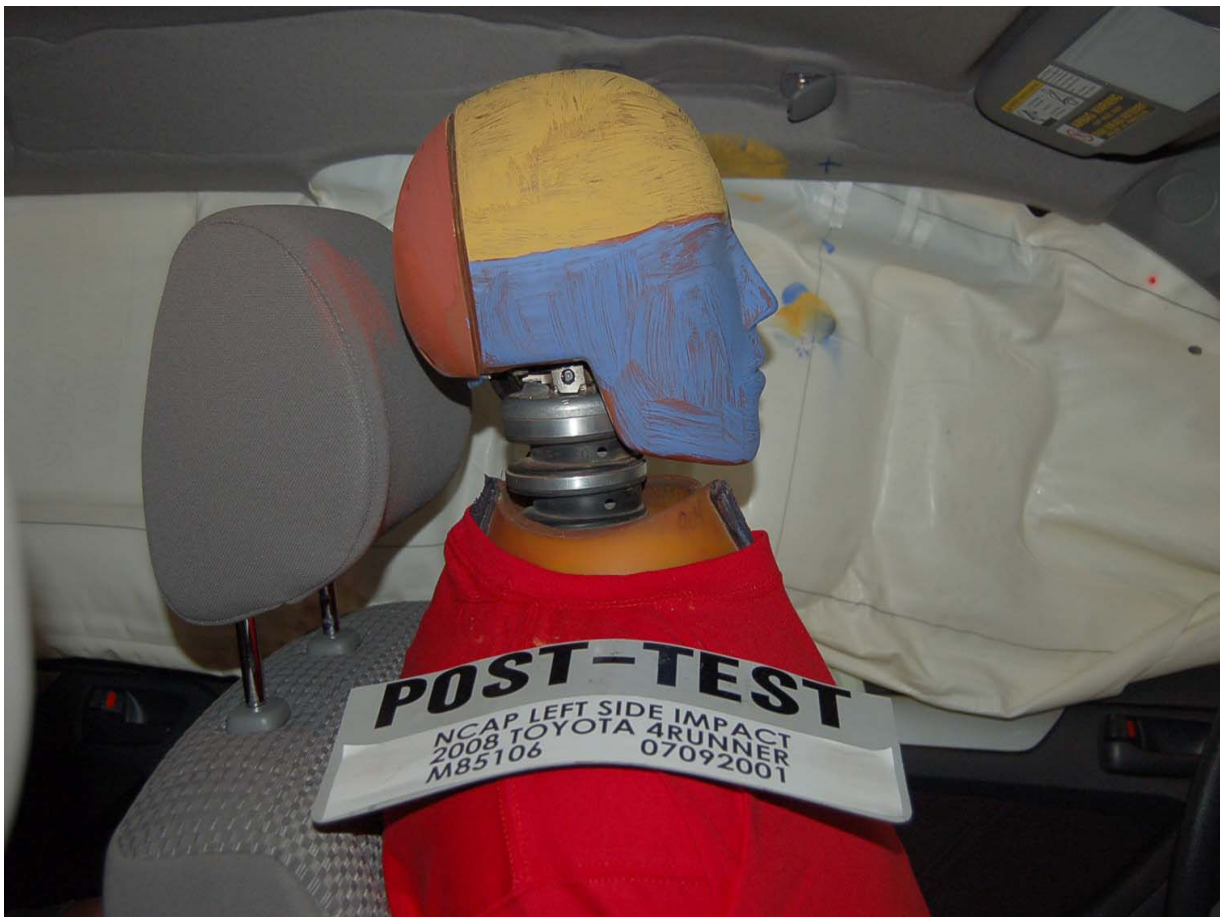
Post-Test Driver Dummy Head Contact
