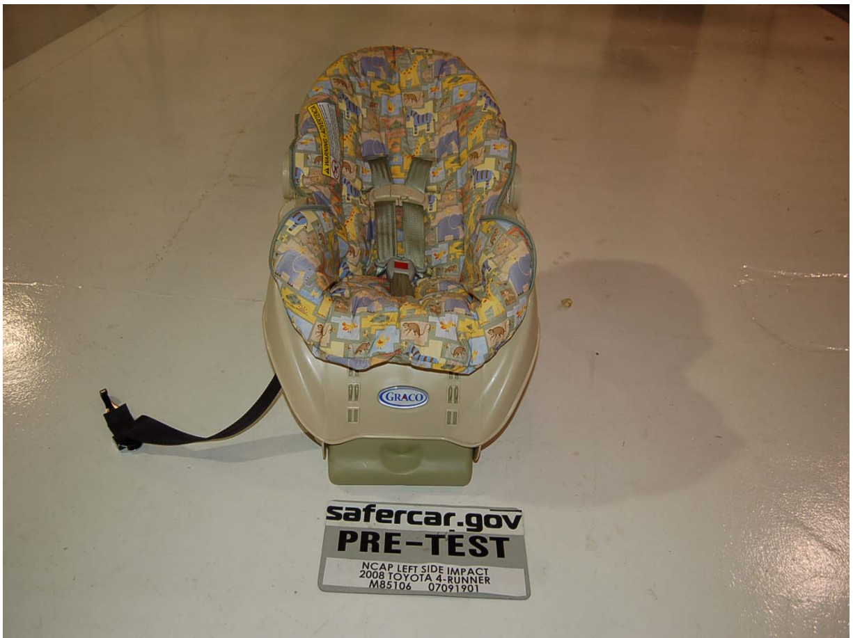
Pre-Test Front View of Position 3 CRS
