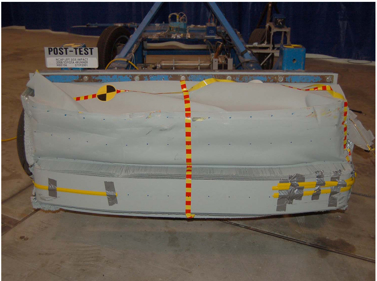
Post-Test Front View of Deformable Barrier
