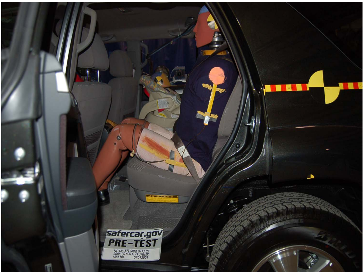
Pre-Test Passenger Dummy (Door Open)
