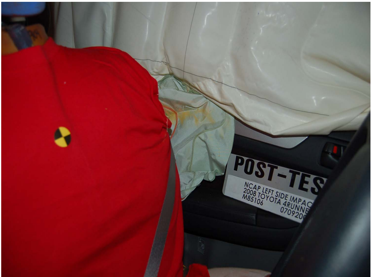
Post-Test Driver Dummy Torso Contact
