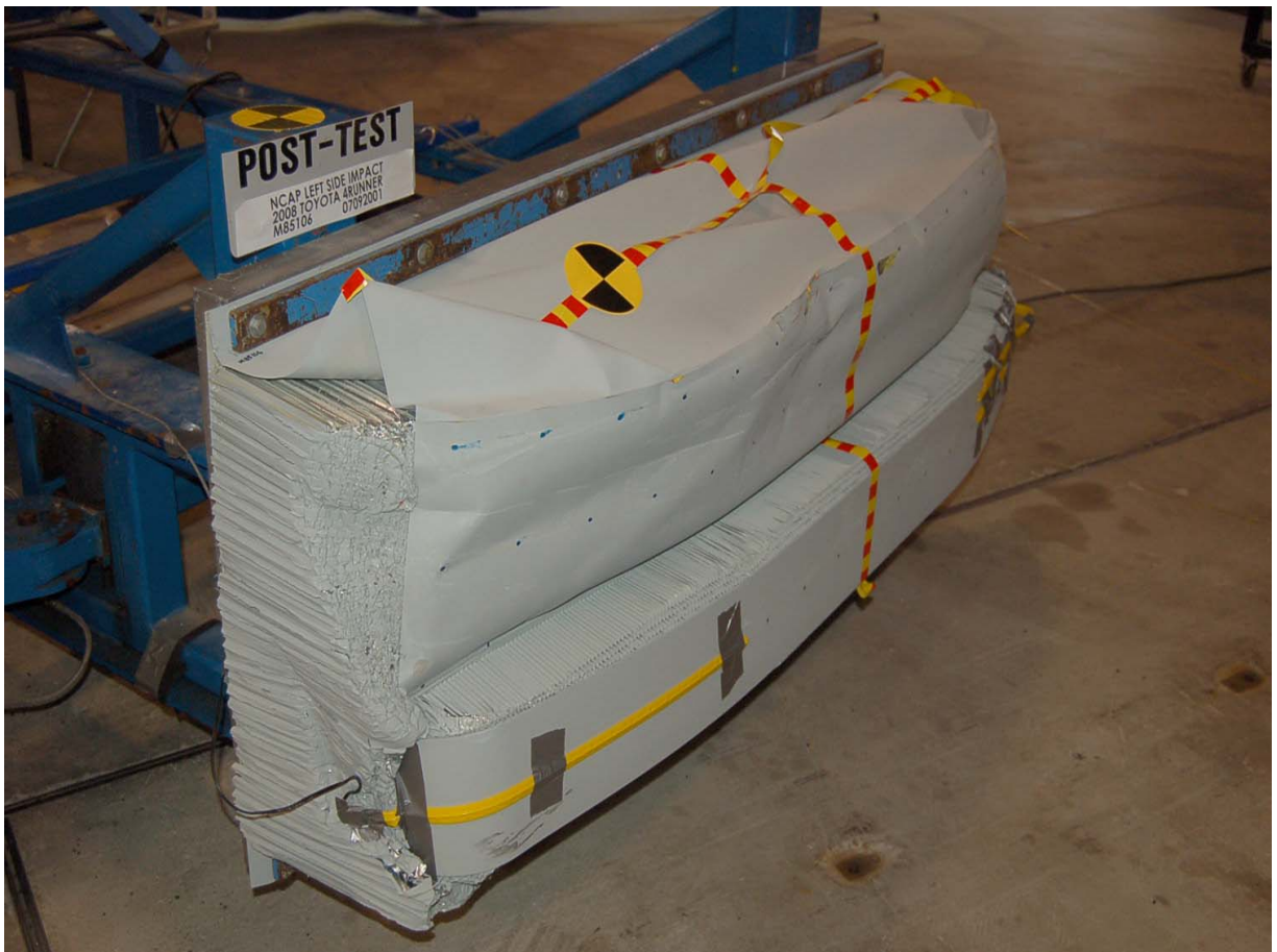
Post-Test Right Side View of Deformable Barrier
