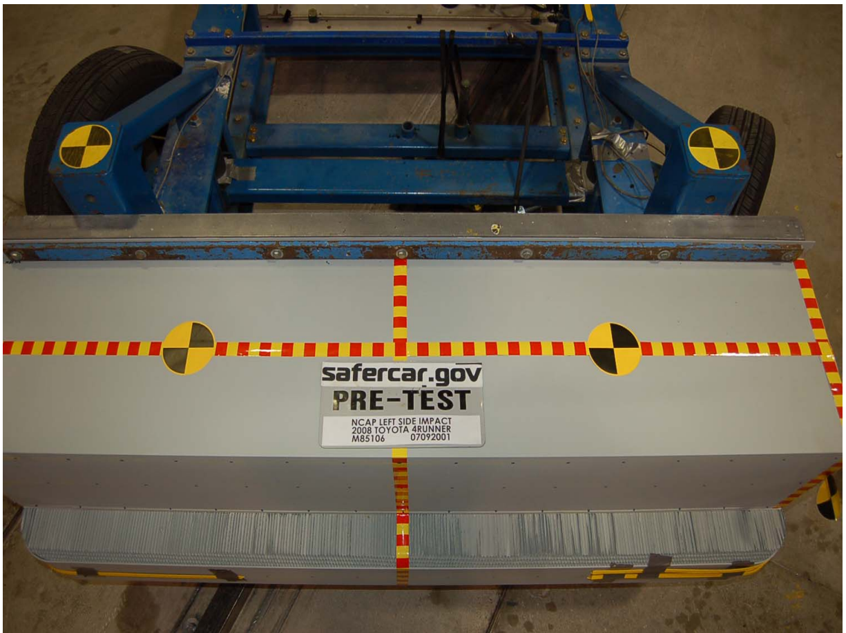
Pre-Test Top View of Deformable Barrier
