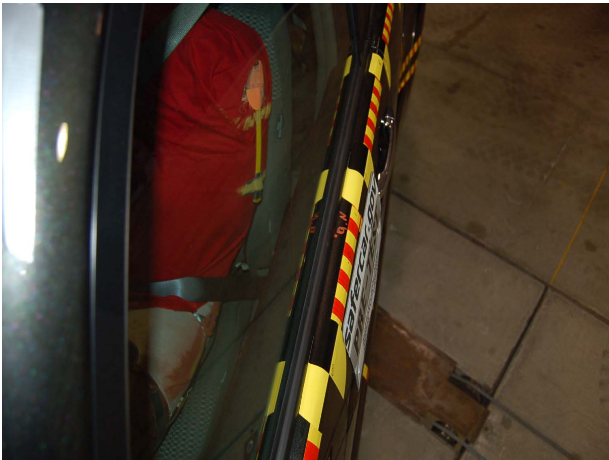
Pre-Test Driver Dummy Clearance From Door
