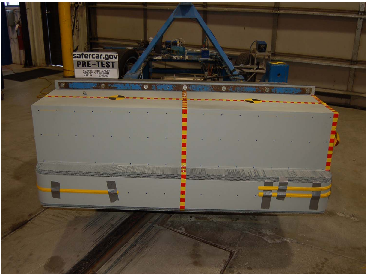
Pre-Test Front View of Deformable Barrier
