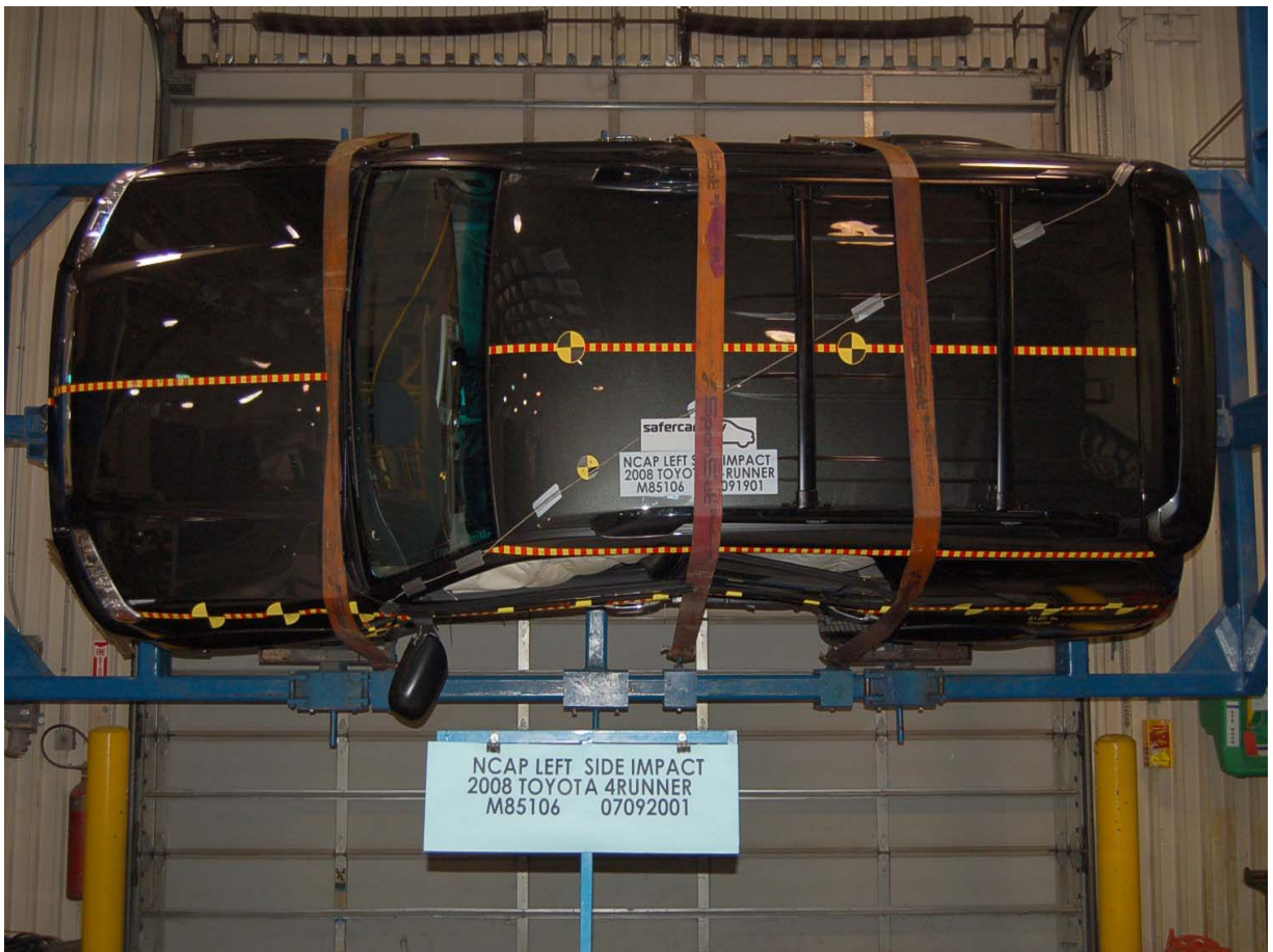
Vehicle on Rollover Device (90 Degrees)
