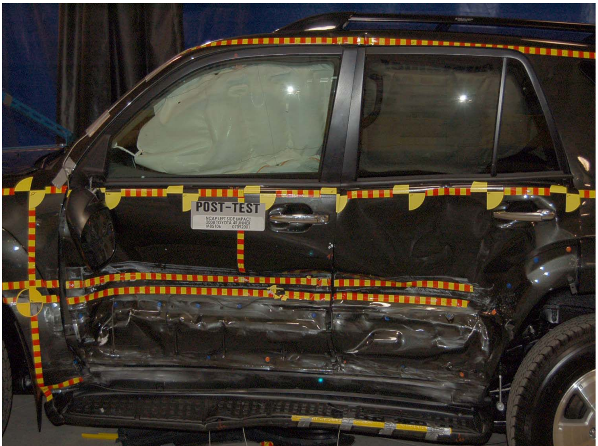
Post-Test Left Side Impact Close-up
