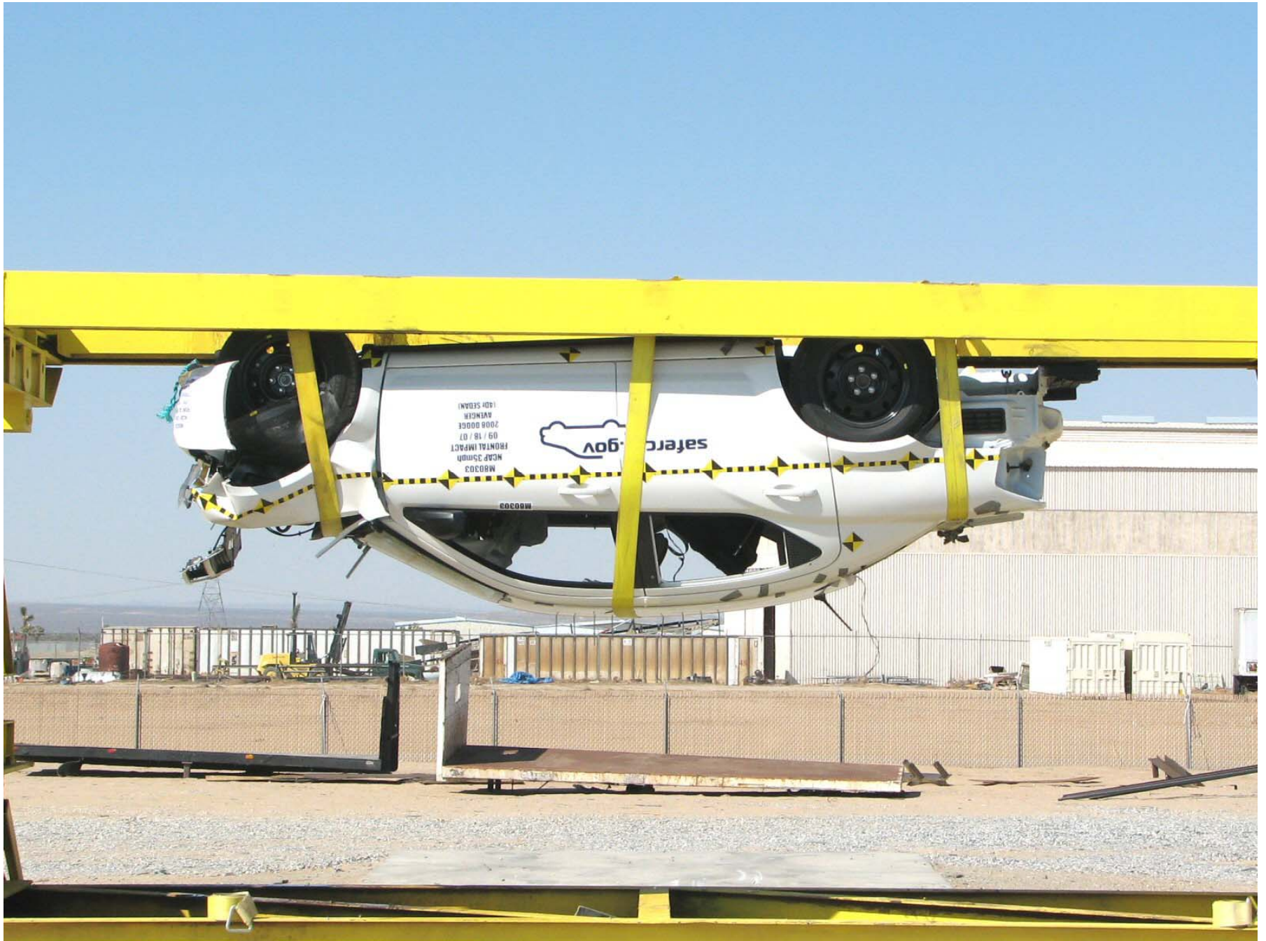
Figure A-60: Vehicle on Rollover Device (180°)
