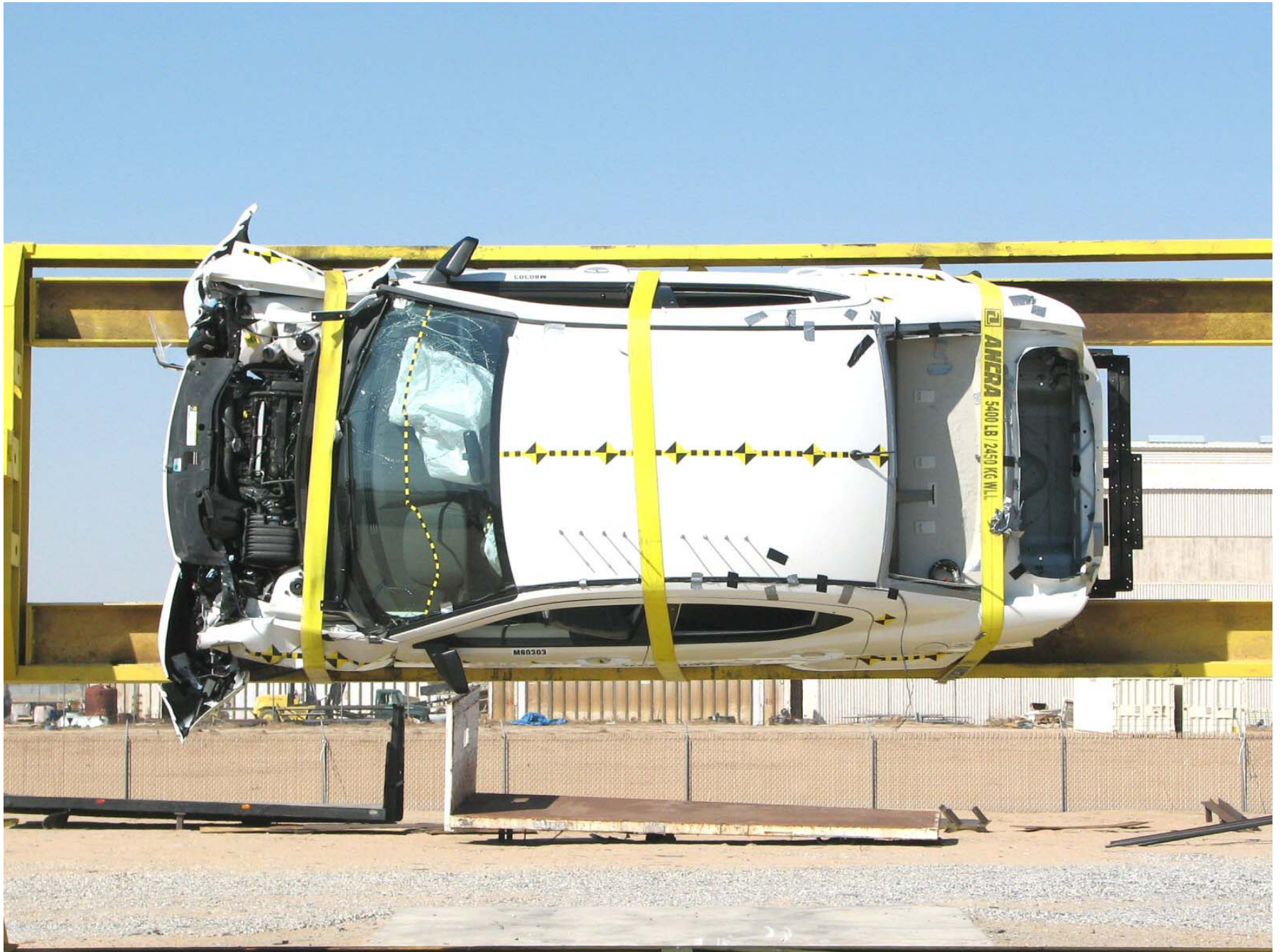
Figure A-59: Vehicle on Rollover Device (90°)
