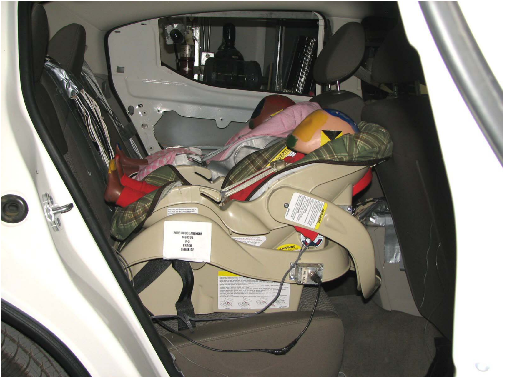
Figure D2-14: Pre-Test Position 3 Right Side View
