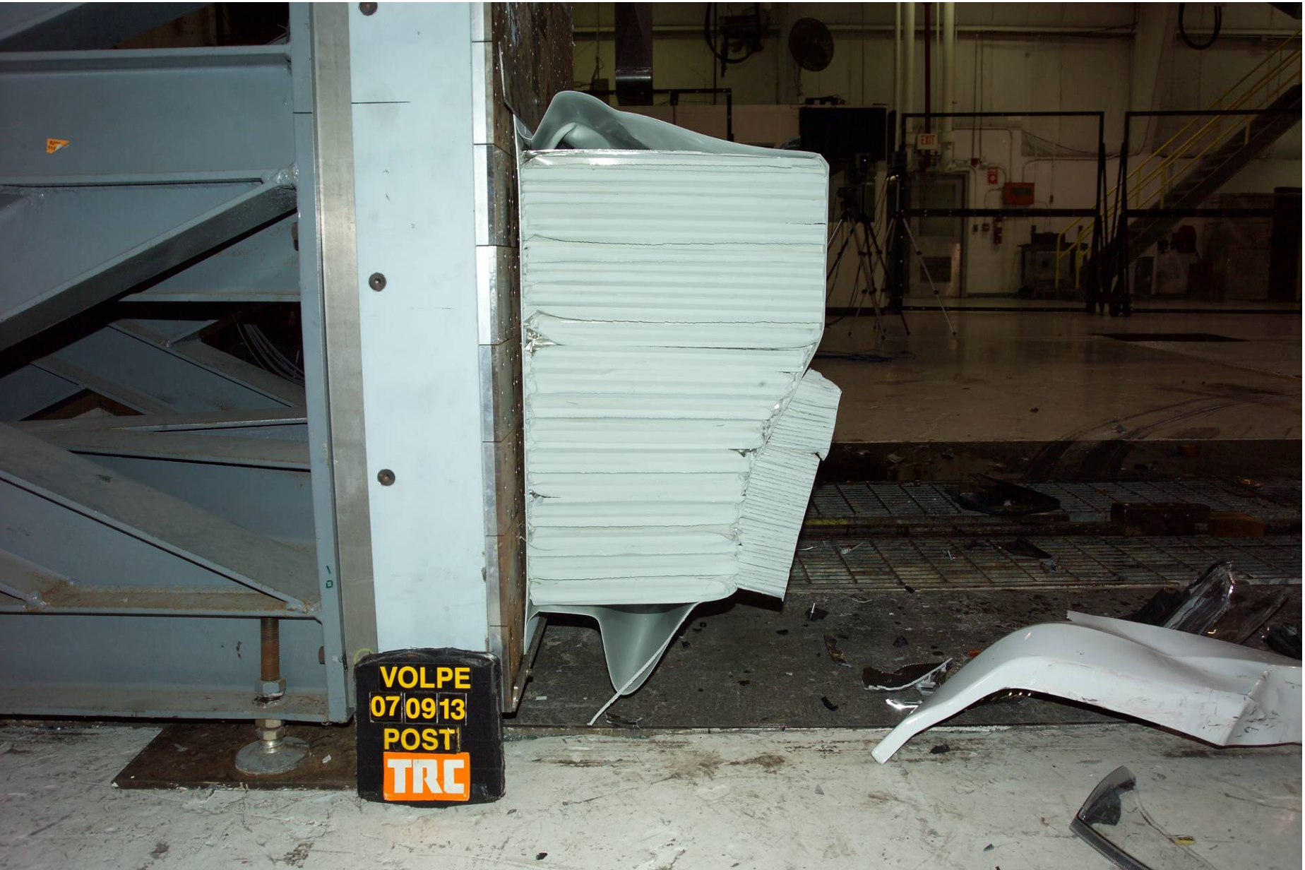
Figure A-80 Post-Test Barrier Left Side View
