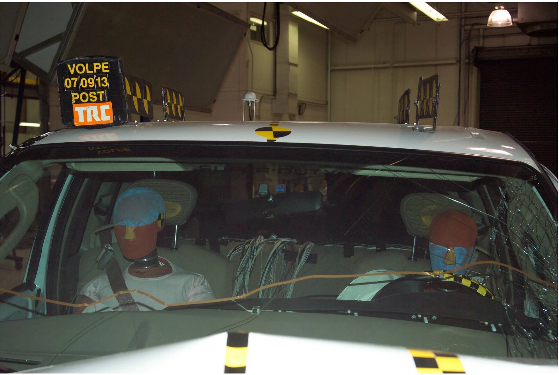
Figure A-41 Post-Test Windshield - Driver and Right Front Passenger Dummies View
