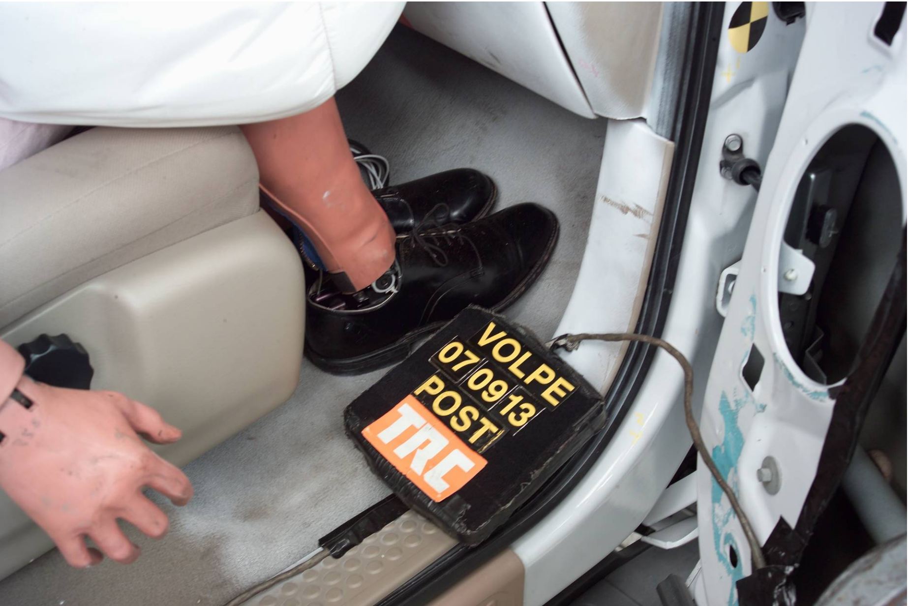
Figure A-73 Post-Test Right Front Passenger Floorboard Deformation - View 1
