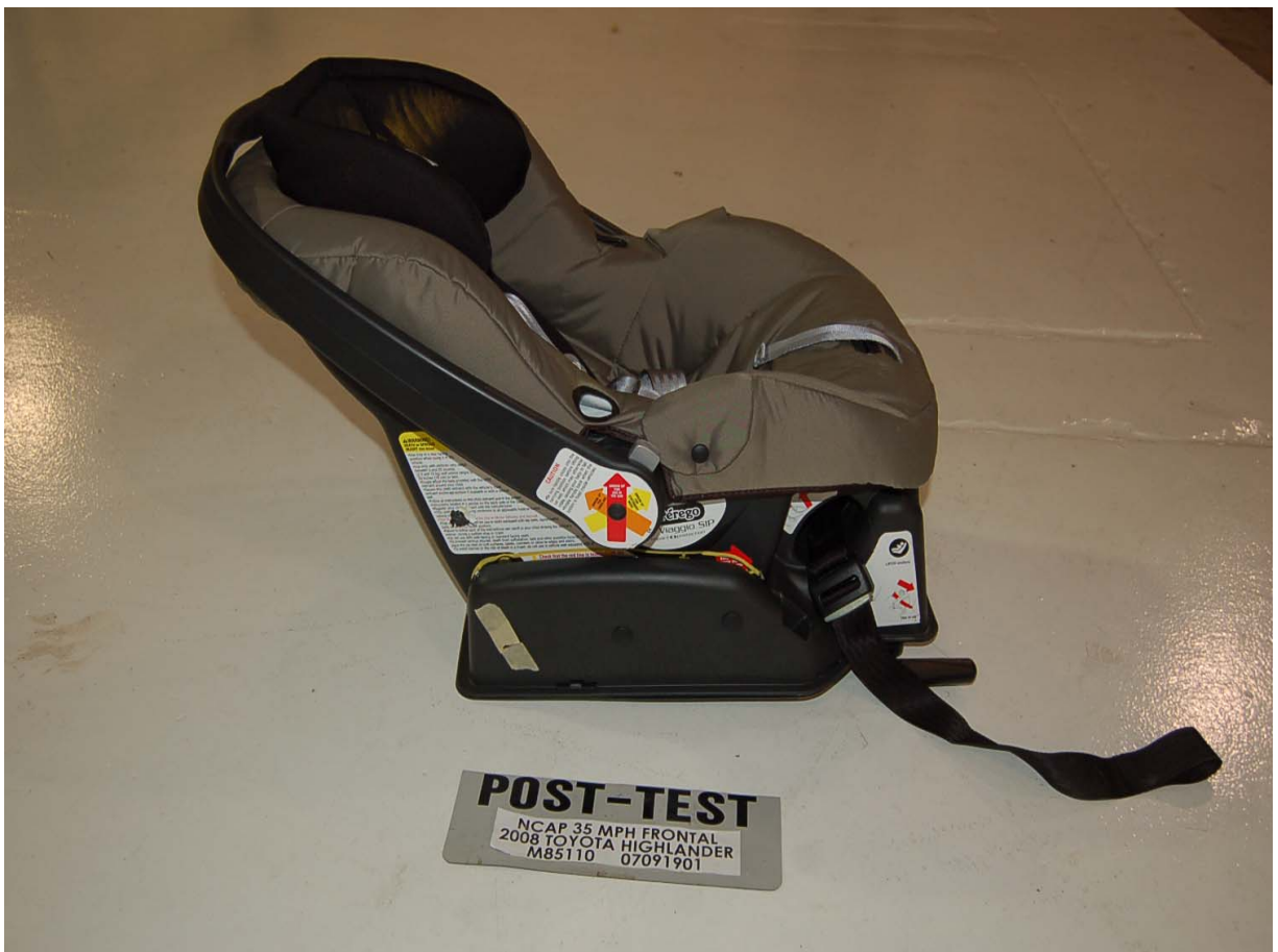
Post-Test Right Side View of Position 4 CRS
