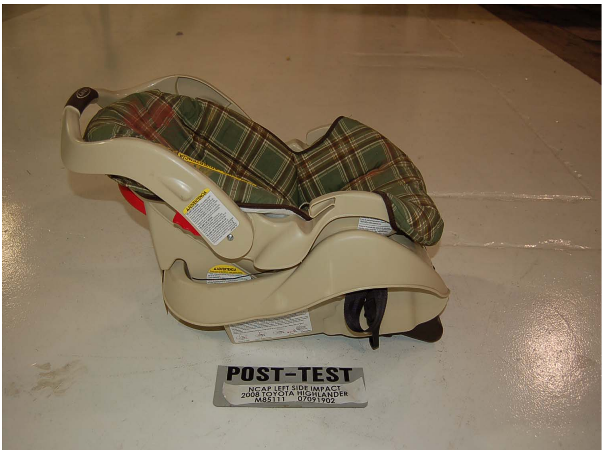
Post-Test Right Side View of Position 3 CRS
