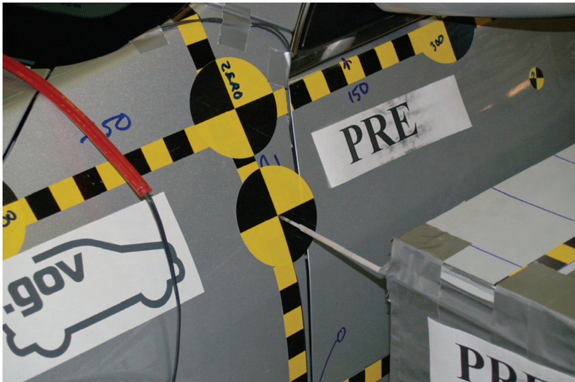
Figure A-25: Pre test impact point
