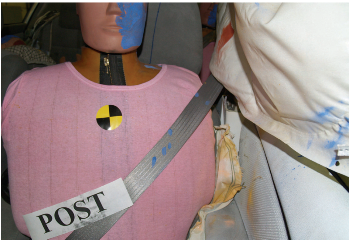
Figure A-38: Post test driver shoulder clearance
