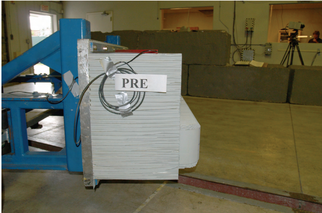
Figure A-53: Pre test right side view of MDB barrier face
