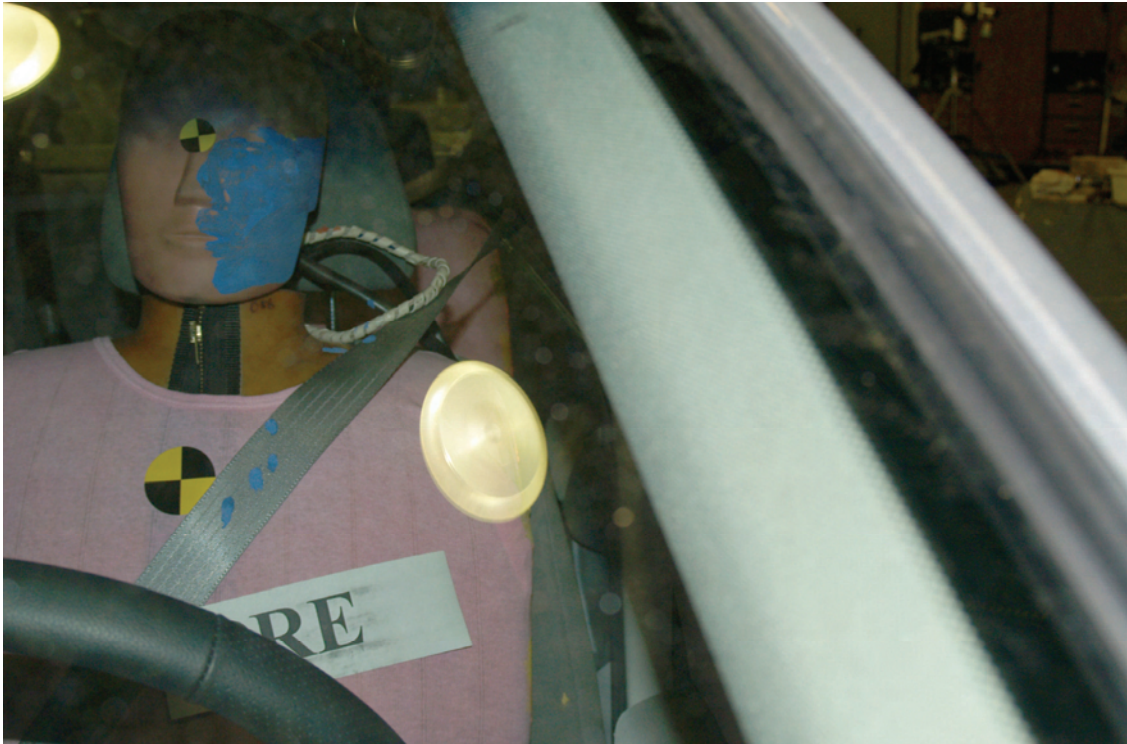
Figure A-37: Pre test driver shoulder clearance
