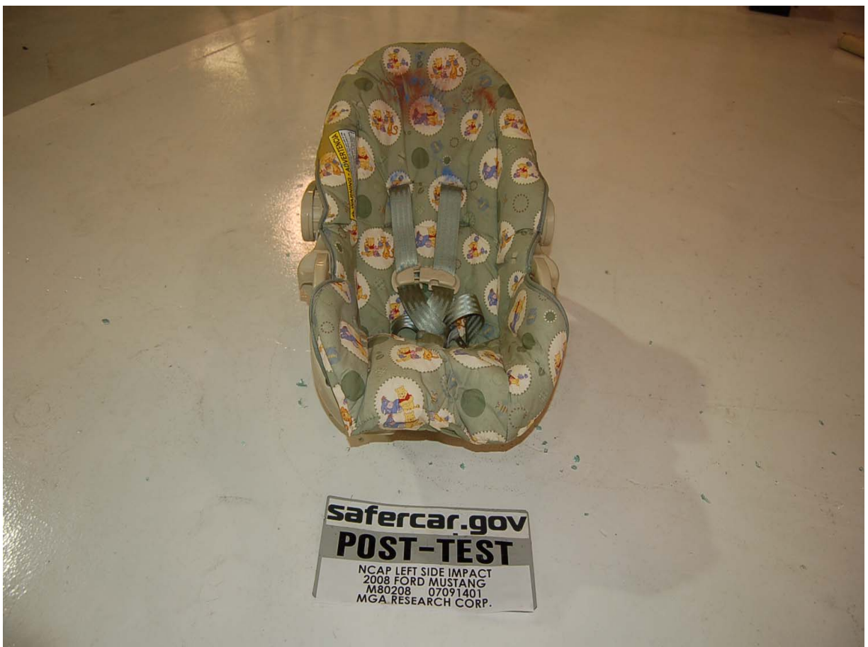
Post-Test Front View of Position 3 CRS
