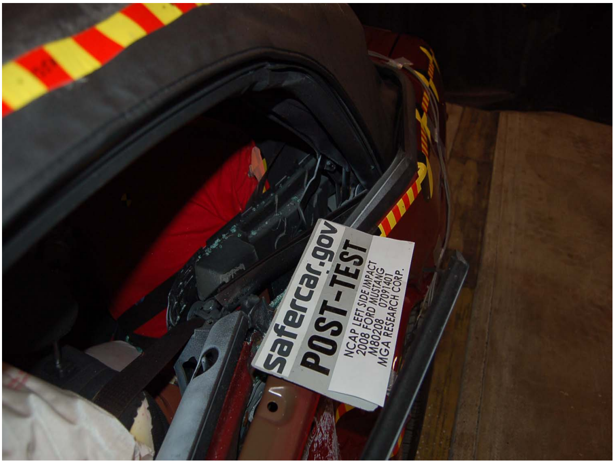
Post-Test Passenger Dummy Clearance From Door
