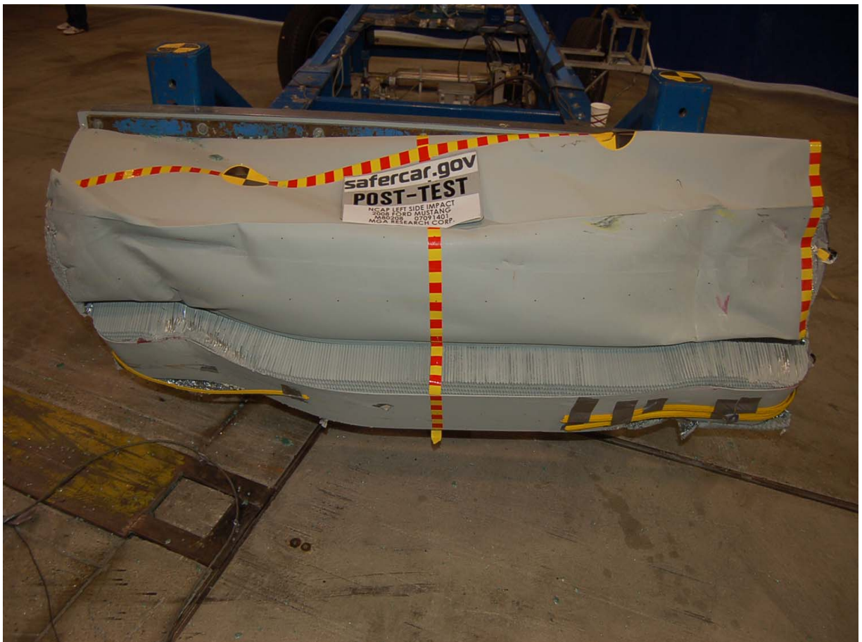
Post-Test Front View of Deformable Barrier
