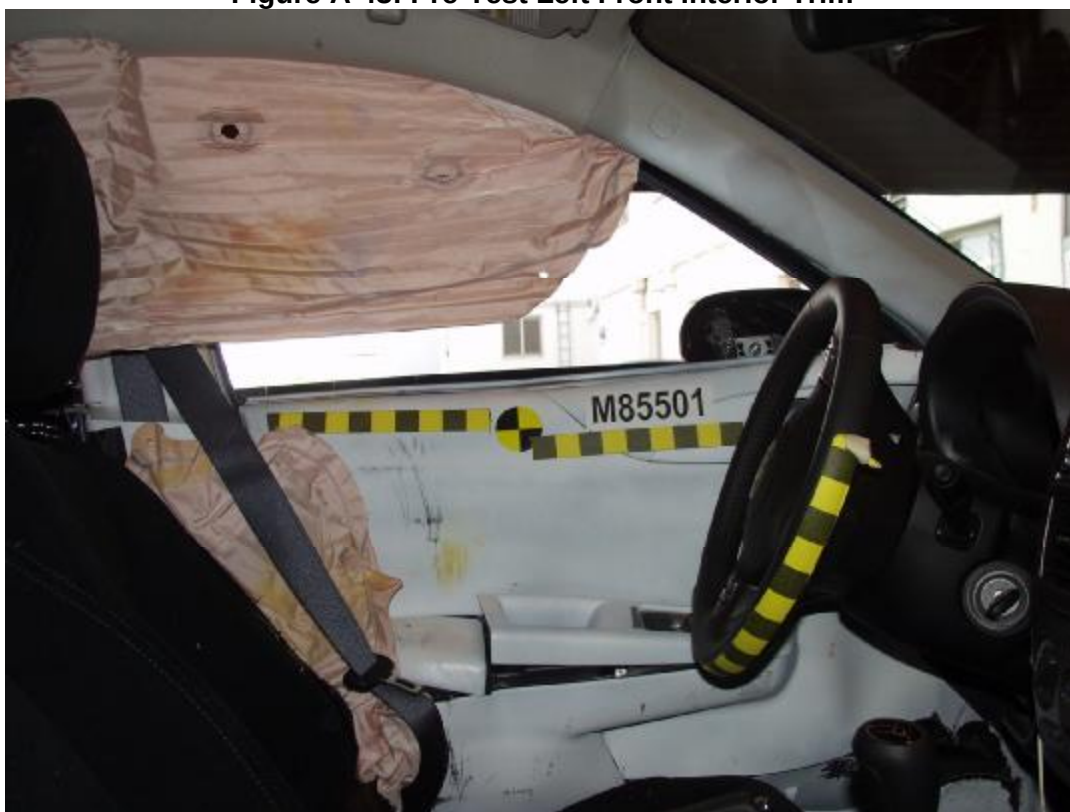
Figure A-44: Post-Test Left Front Interior Trim
