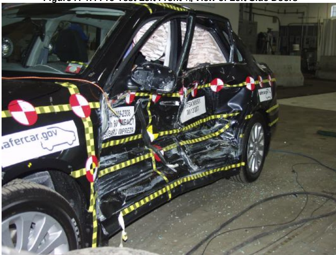
Figure A-48: Post-Test Left Front \frac{3}{4} View of Left Side Doors
