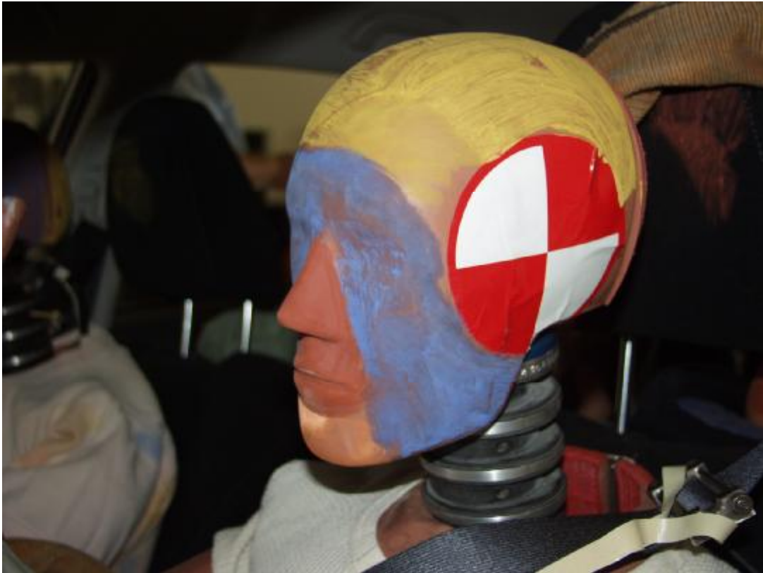
Figure A-42: Post-Test Driver Head View
