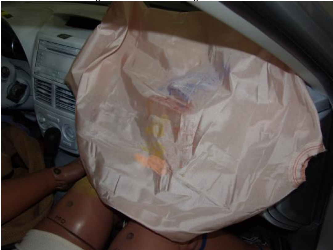
Figure A-57: Post-Test Passenger Contact to Airbag
