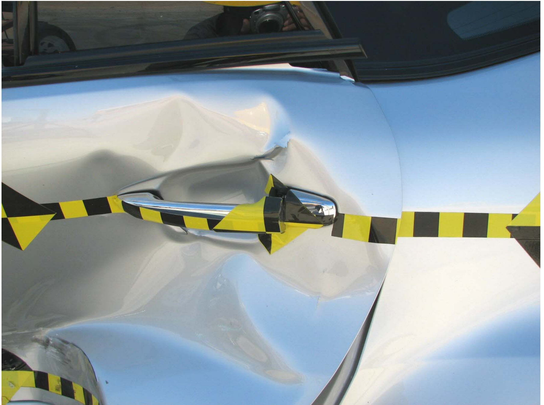
Figure A-34: Post-Test Left Rear Door
