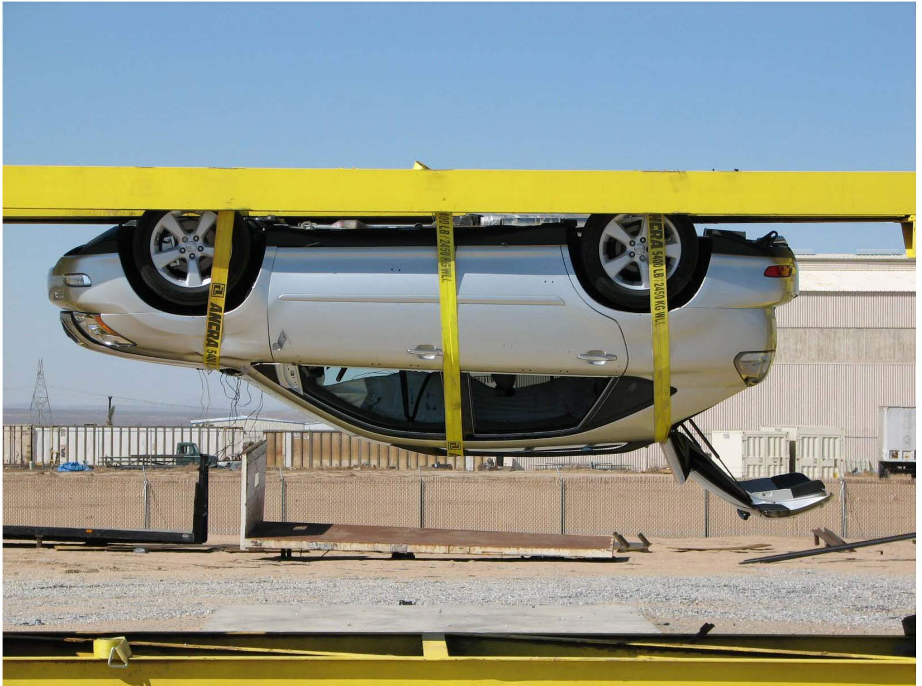
Figure A-63: Vehicle on Rollover Device (180°)
