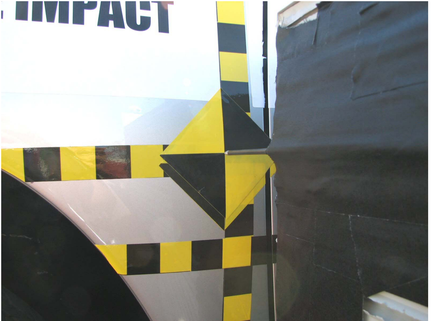
Figure A-25: Pre-Test Left Impact Point
