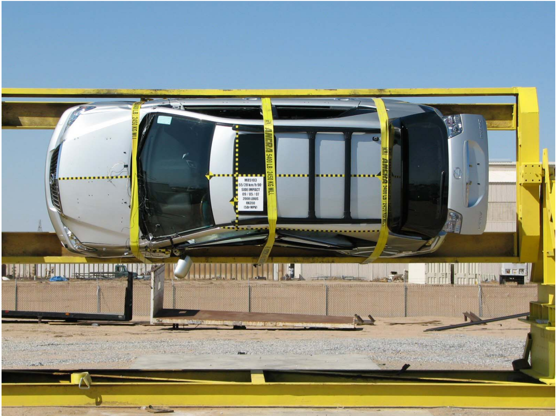
Figure A-62: Vehicle on Rollover Device (90°)
