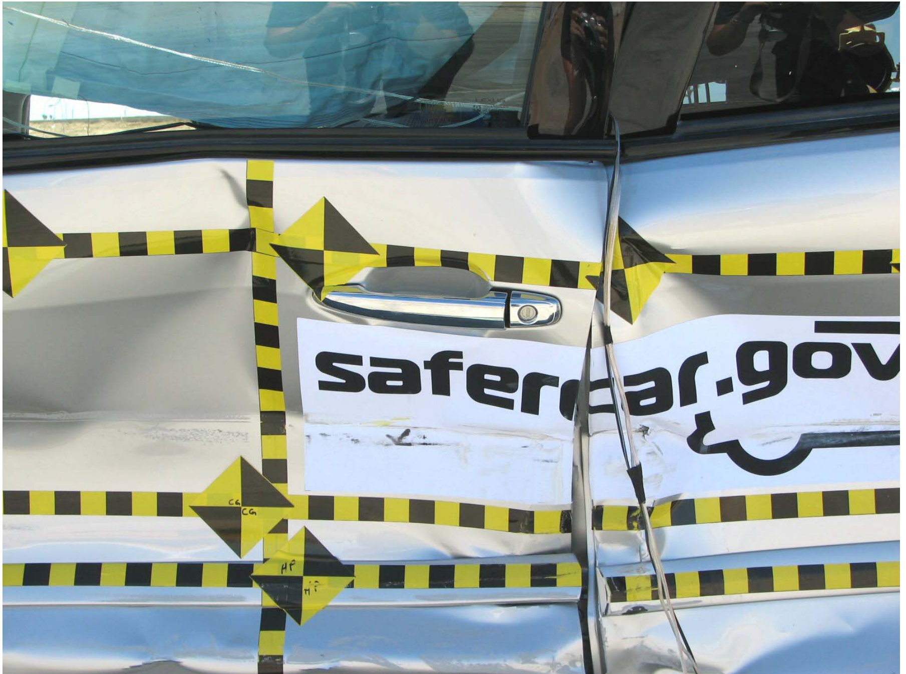
Figure A-32: Post-Test Left Front Door
