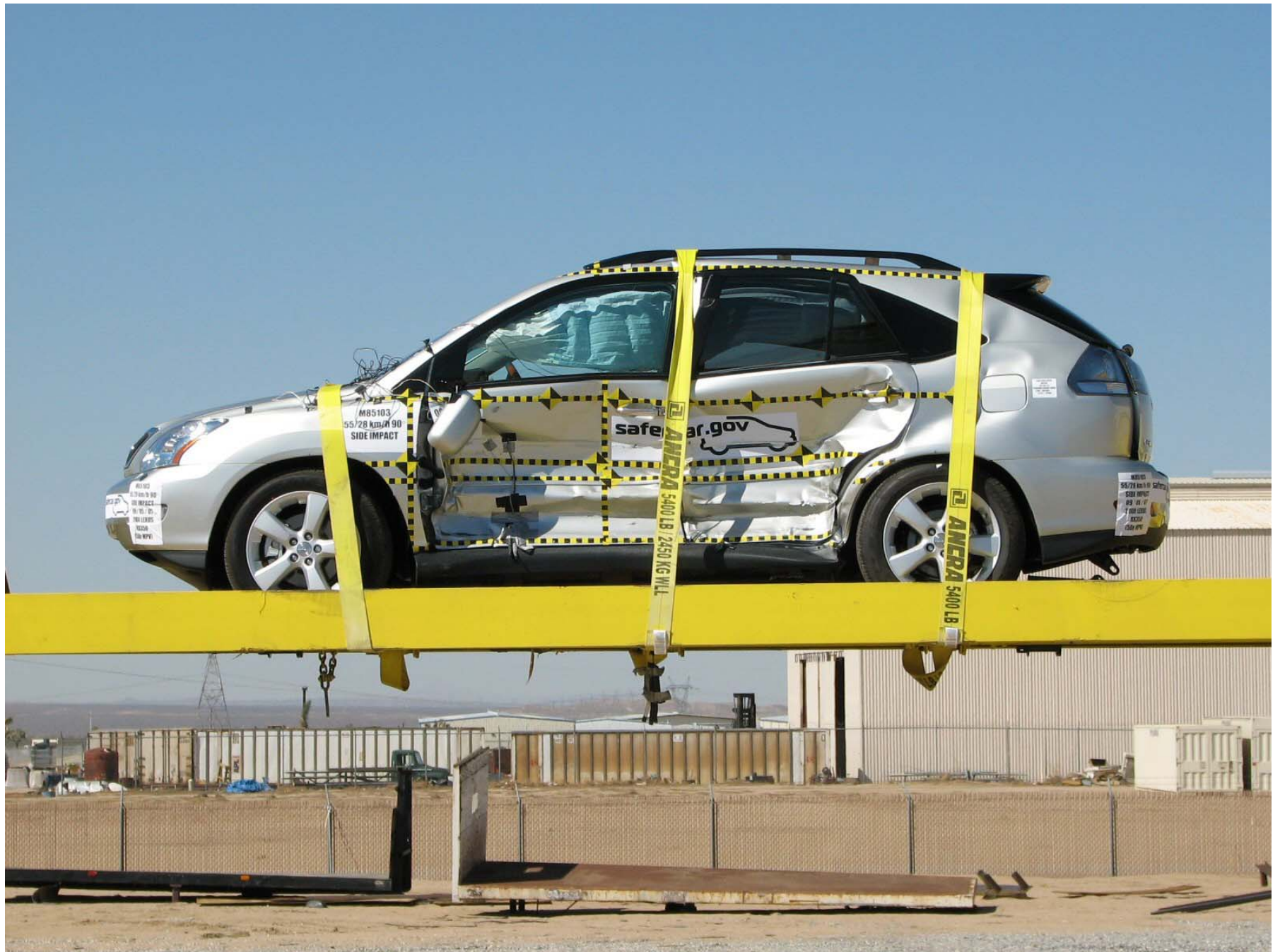
Figure A-61: Vehicle on Rollover Device (0°)
