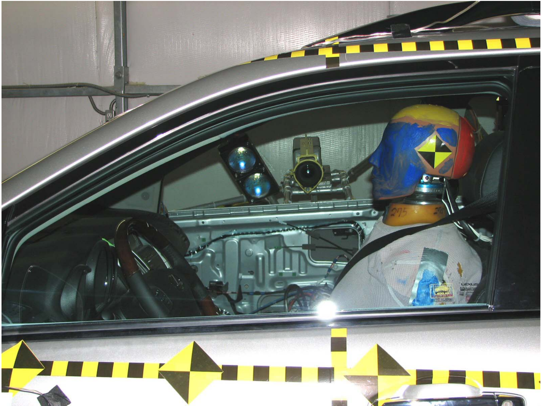
Figure A-36: Pre-Test Driver Dummy (Through Window)
