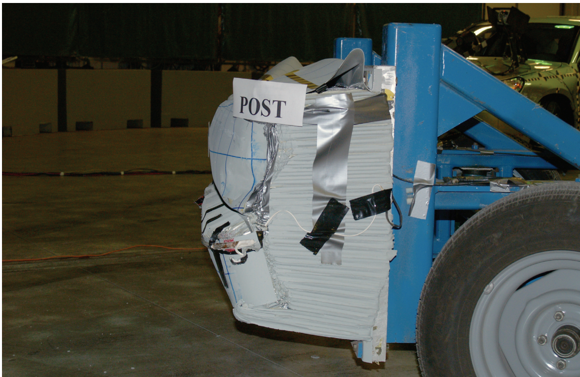
Figure A-56: Post test left side view of MDB barrier face
