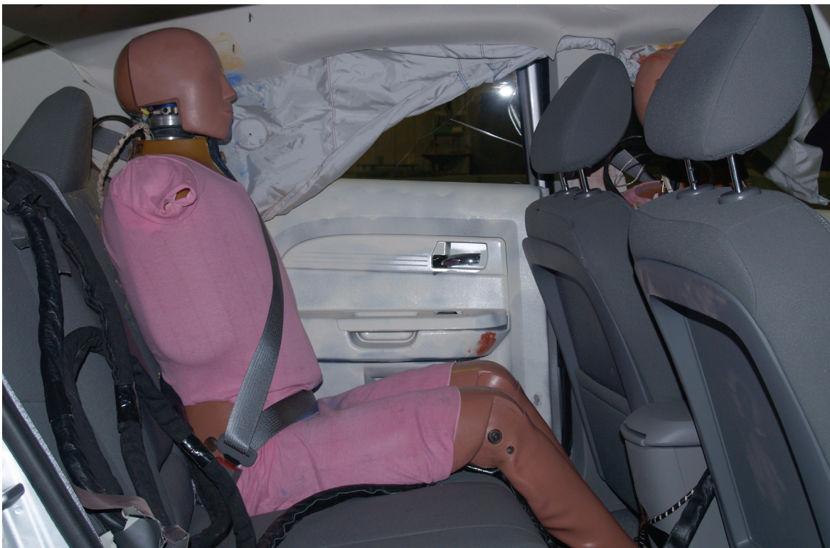
Figure A-46: Post test passenger right side view
