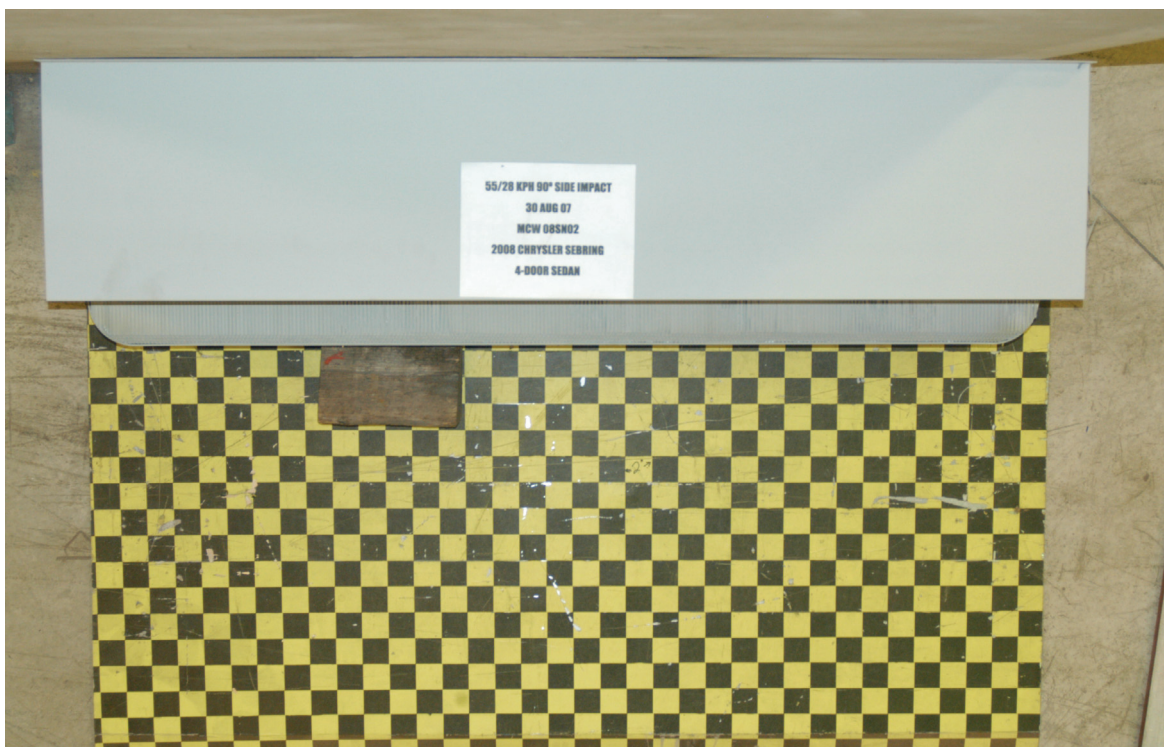
Figure A-51: Pre test overhead view of MDB barrier face
