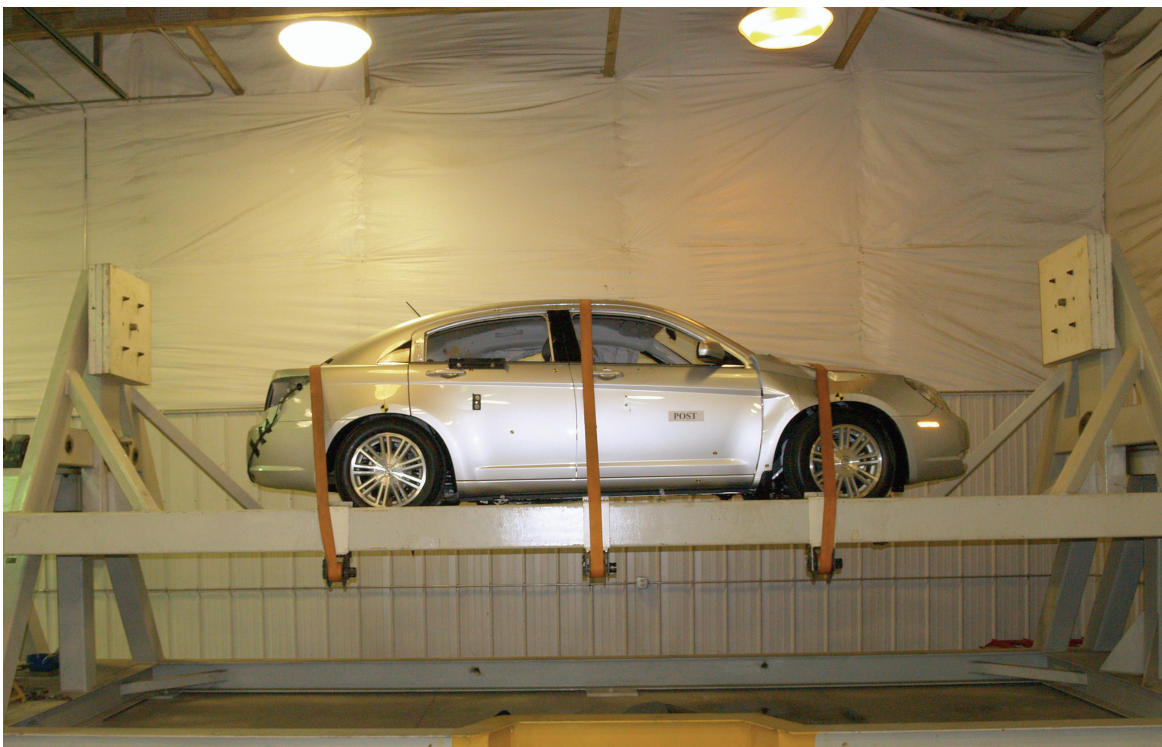
Figure A-61: FMVSS 301 360 degrees
