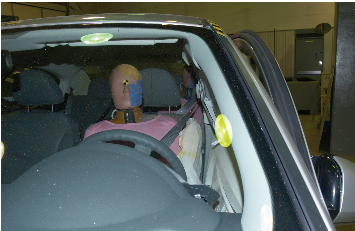
Figure A-36: Post test driver shoulder clearance
