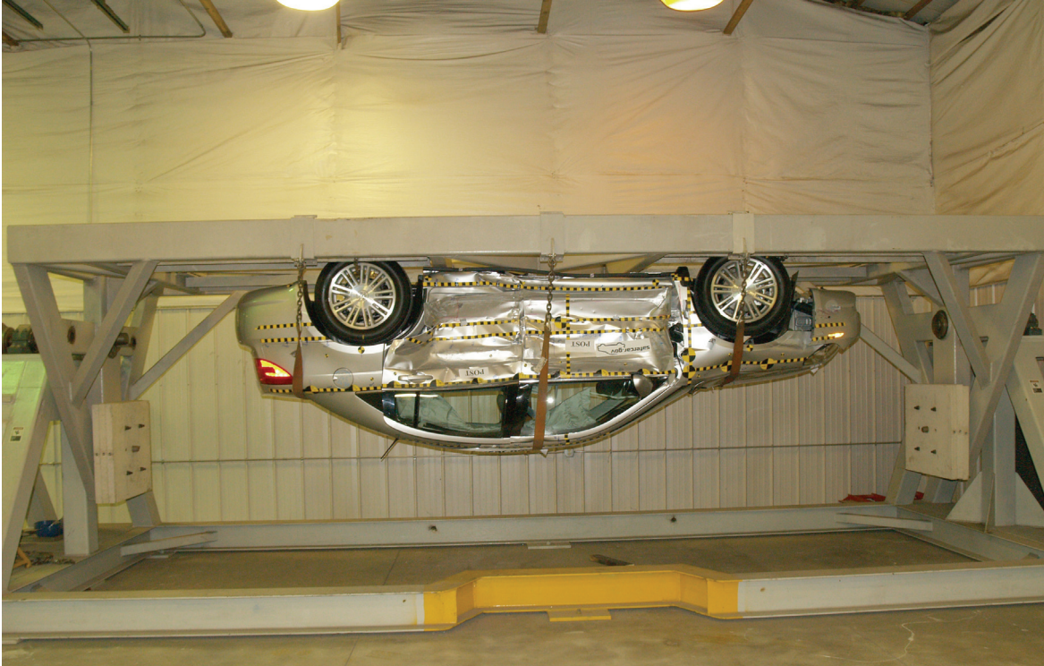
Figure A-59: FMVSS 301 180 degrees
