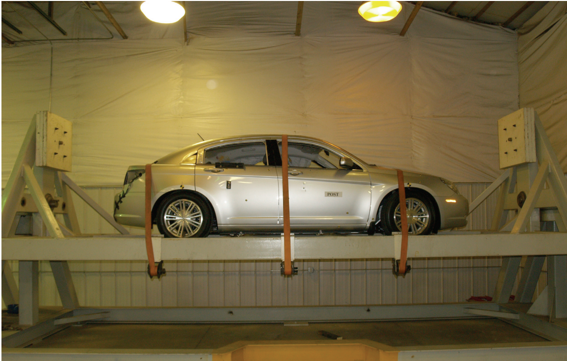
Figure A-57: FMVSS 301 0 degrees
