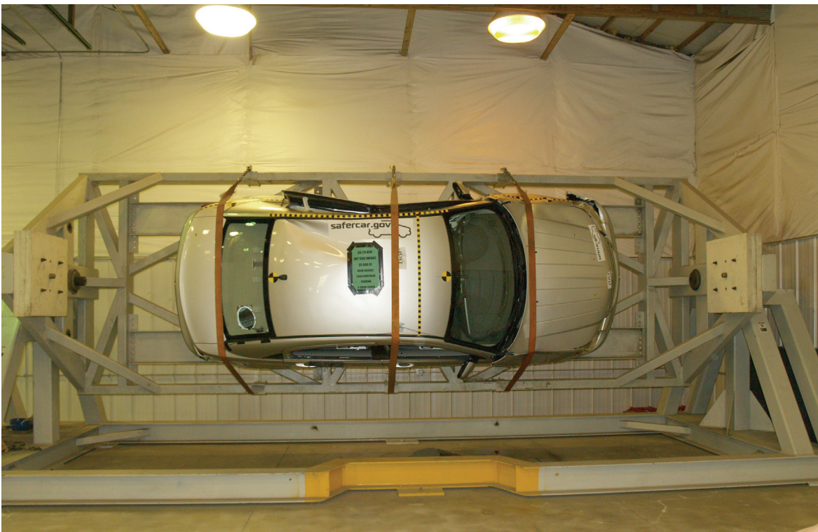
Figure A-60: FMVSS 301 270 degrees
