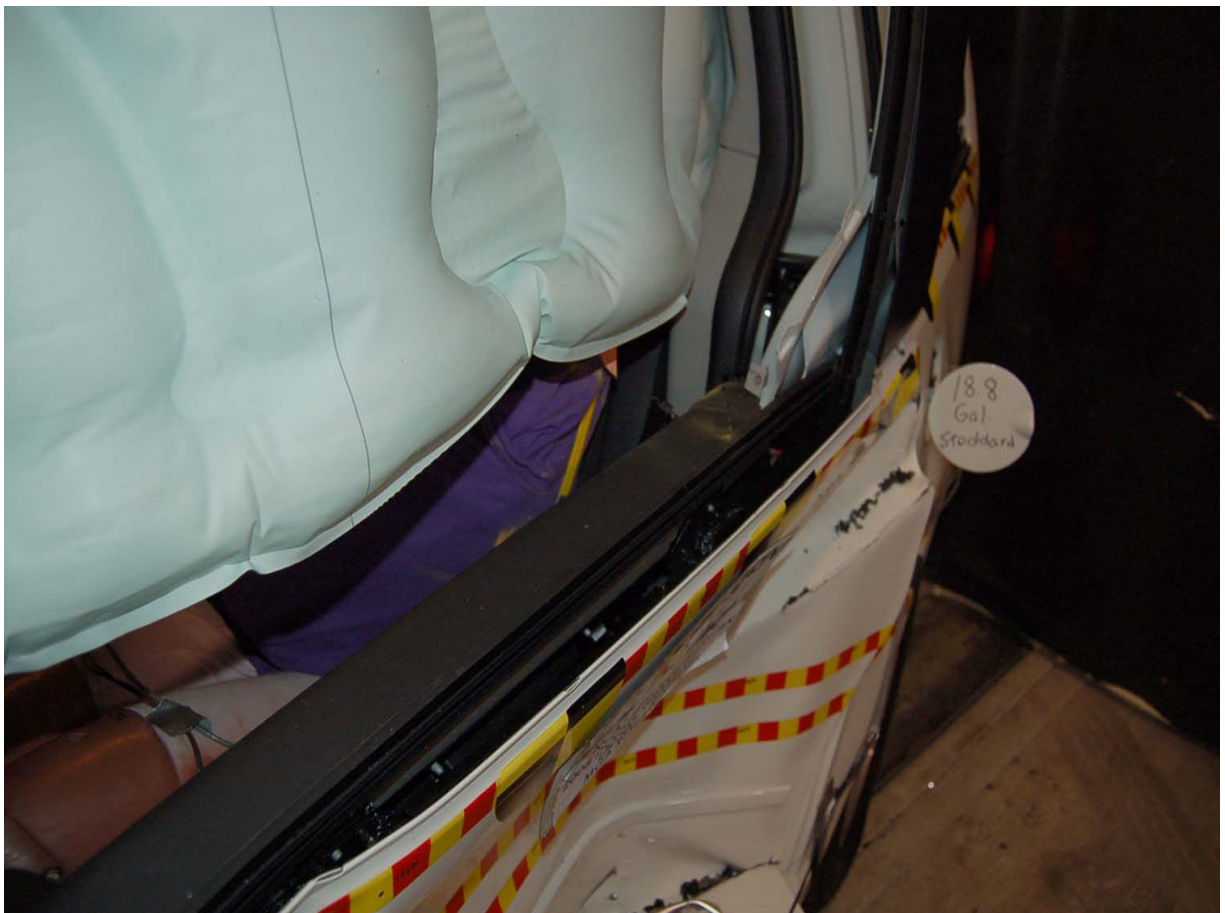
Post-Test Passenger Dummy Clearance From Door
