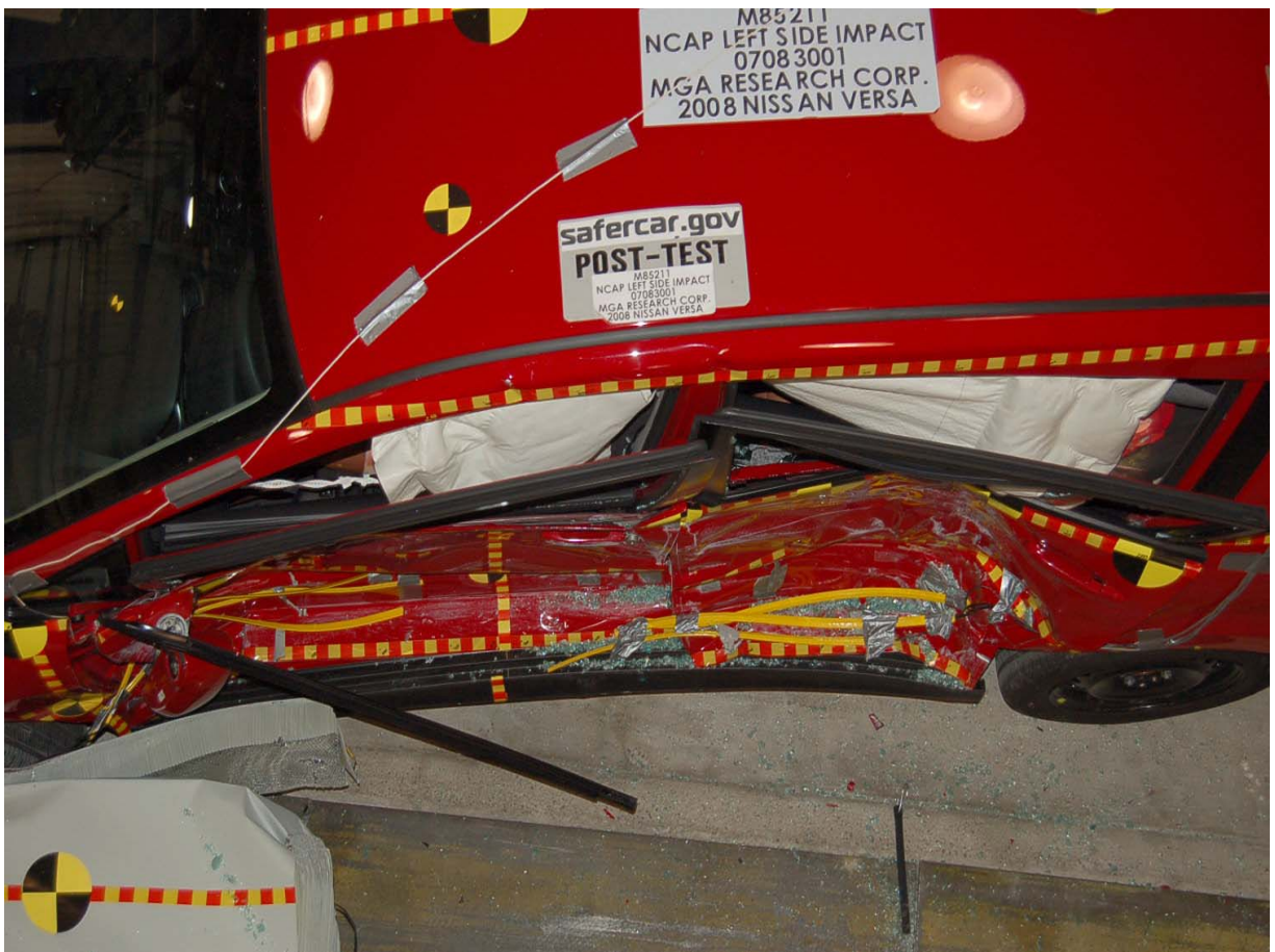
Post-Test Overhead View
