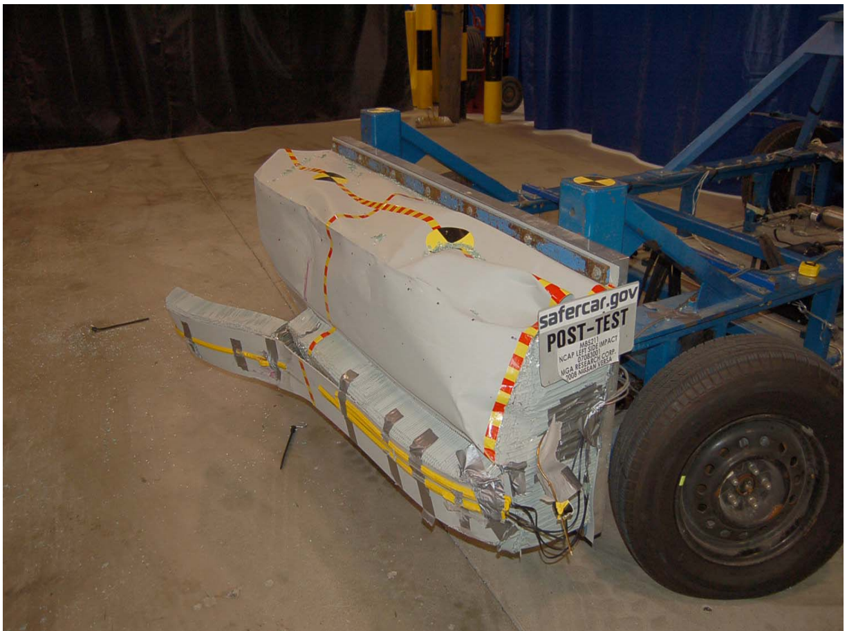
Post-Test Left Side View of Deformable Barrier
