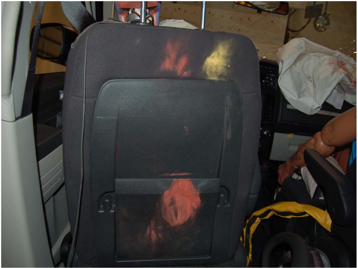
Post-Test Position 4 Head and Feet Contact
