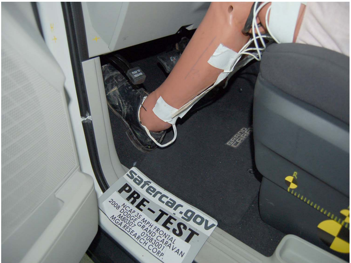
Pre-Test Driver Dummy Feet
