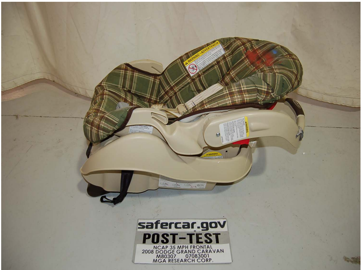
Post-Test Left Side View of Position 3 CRS
