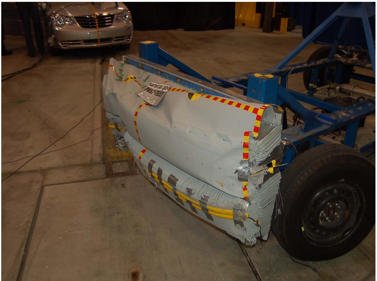
Post-Test Left Side View of Deformable Barrier
