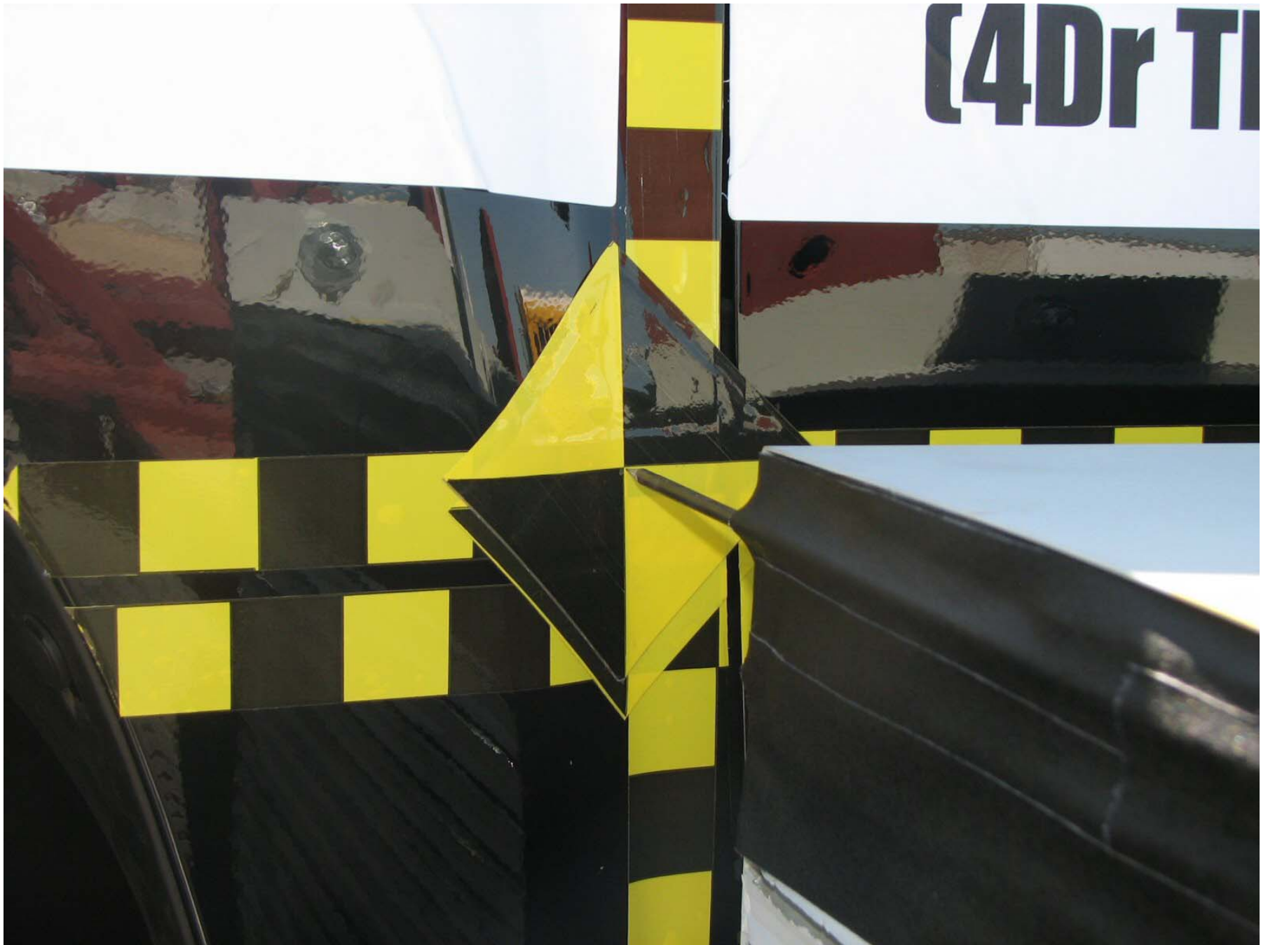
Figure A-25: Pre-Test Left Impact Point
