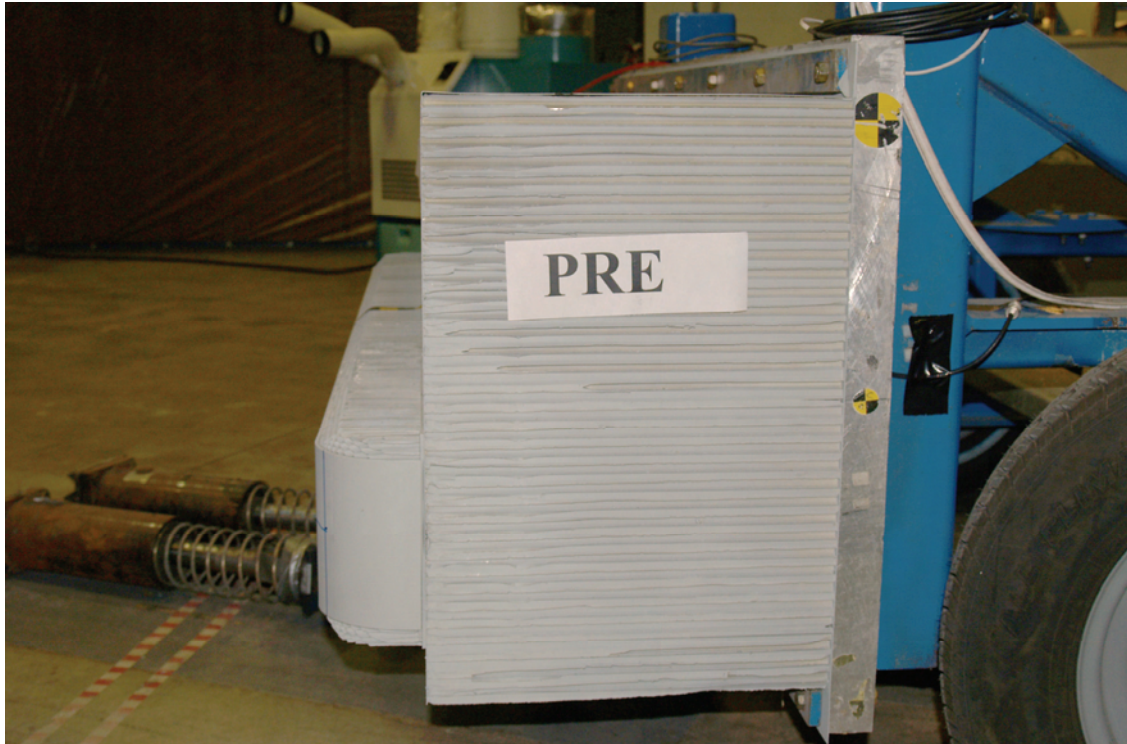
Figure A-53: Pre test left side view of MDB barrier face
