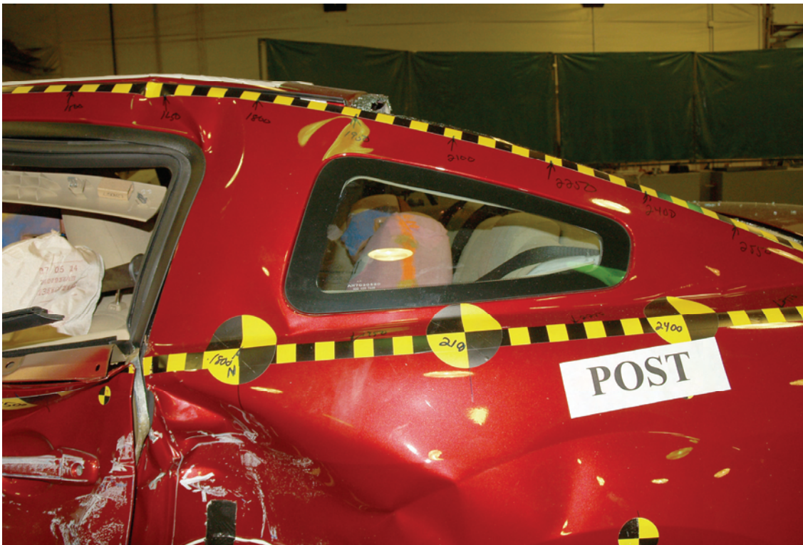
Figure A-42: Post test passenger left side view
