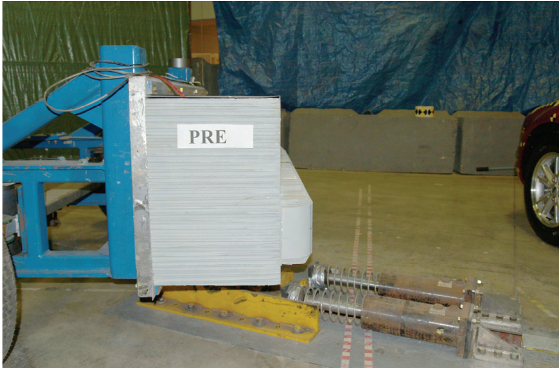
Figure A-51: Pre test right side view of MDB barrier face
