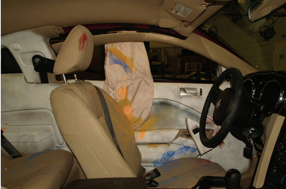
Figure A-39: Post test driver contact locations (1)
