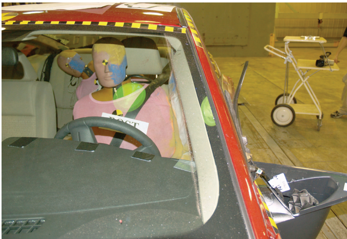
Figure A-36: Post test driver shoulder clearance
