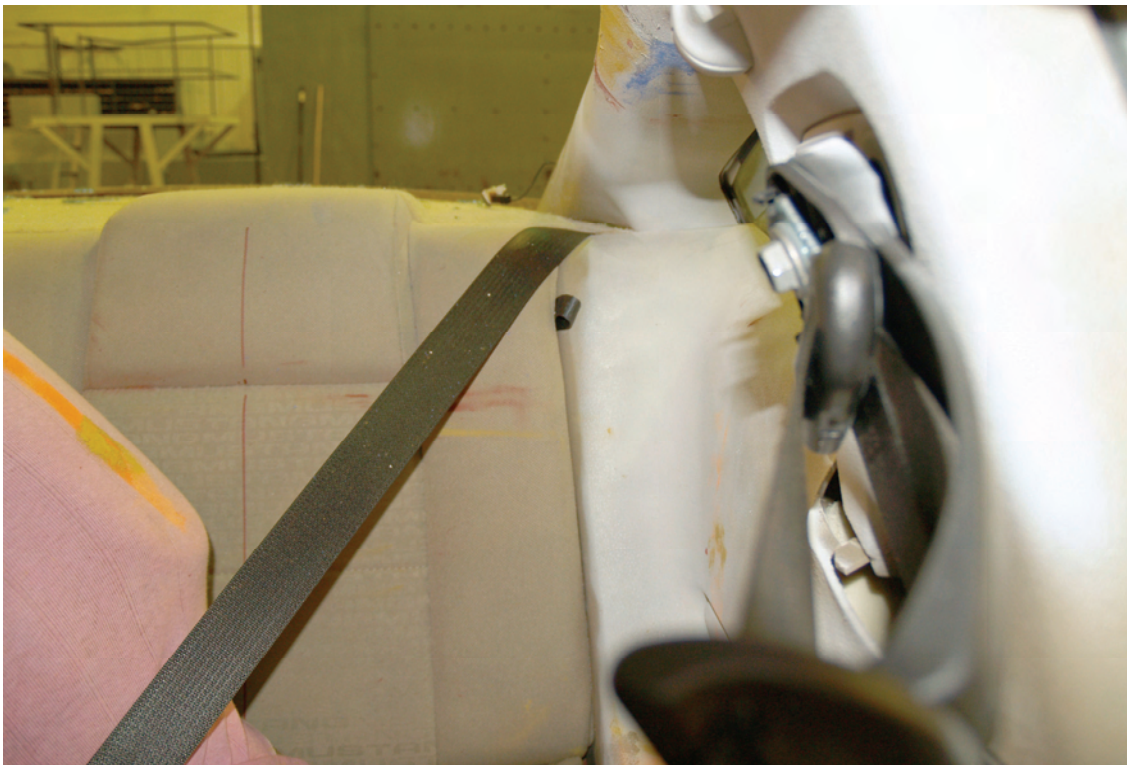
Figure A-44: Post test passenger shoulder clearance
