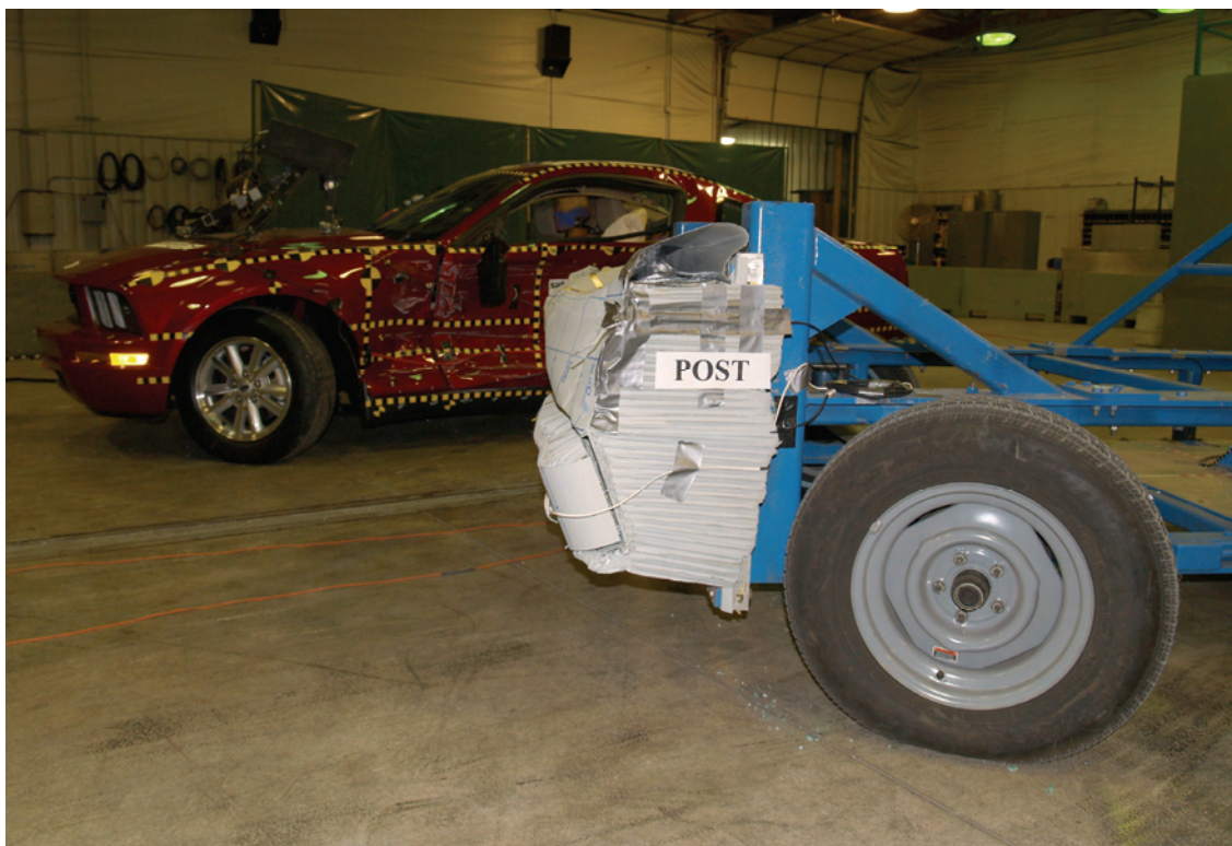
Figure A-54: Post test left side view of MDB barrier face
