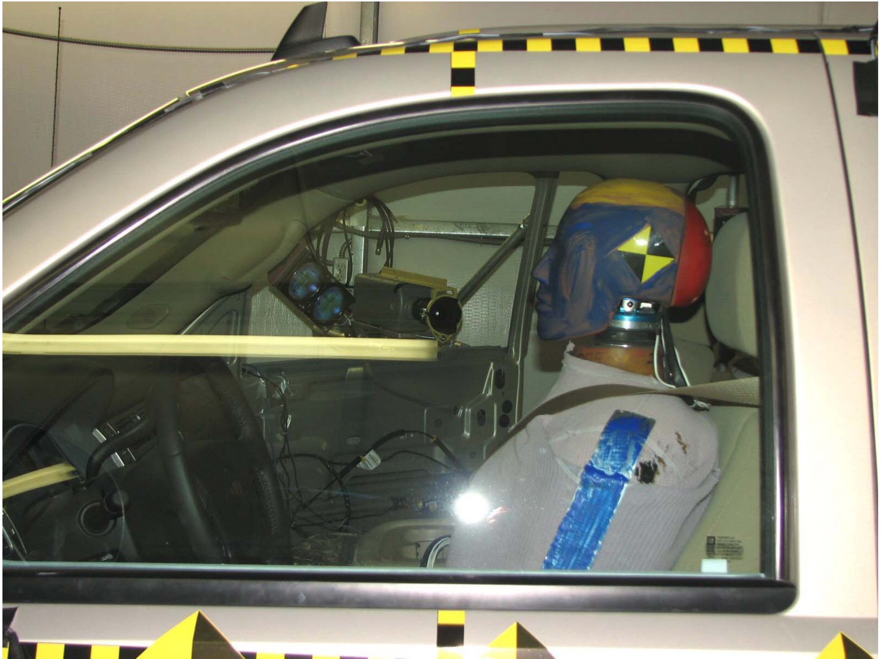
Figure A-36: Pre-Test Driver Dummy (Through Window)
