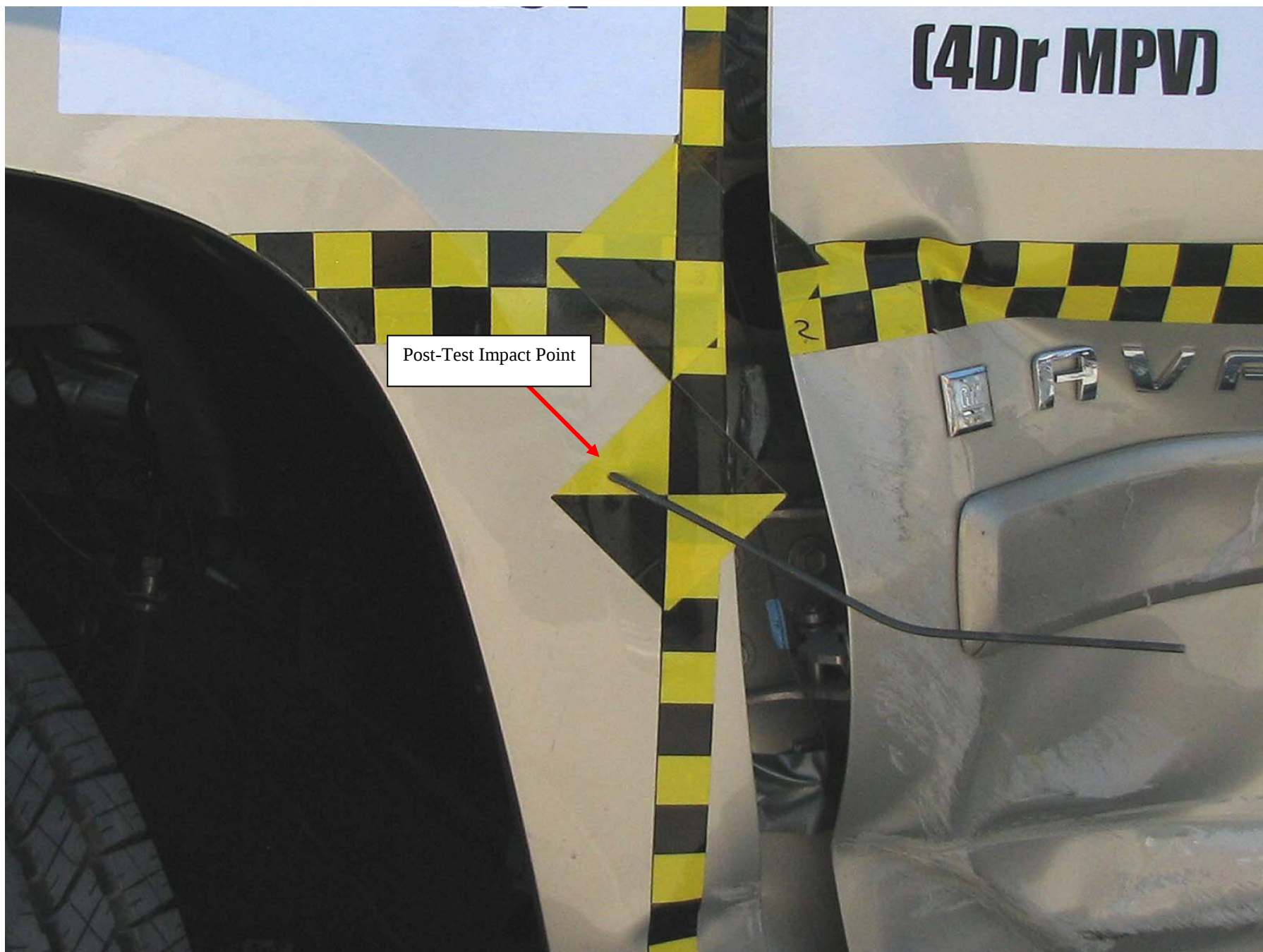
Figure A-26: Post-Test Left Impact Point
