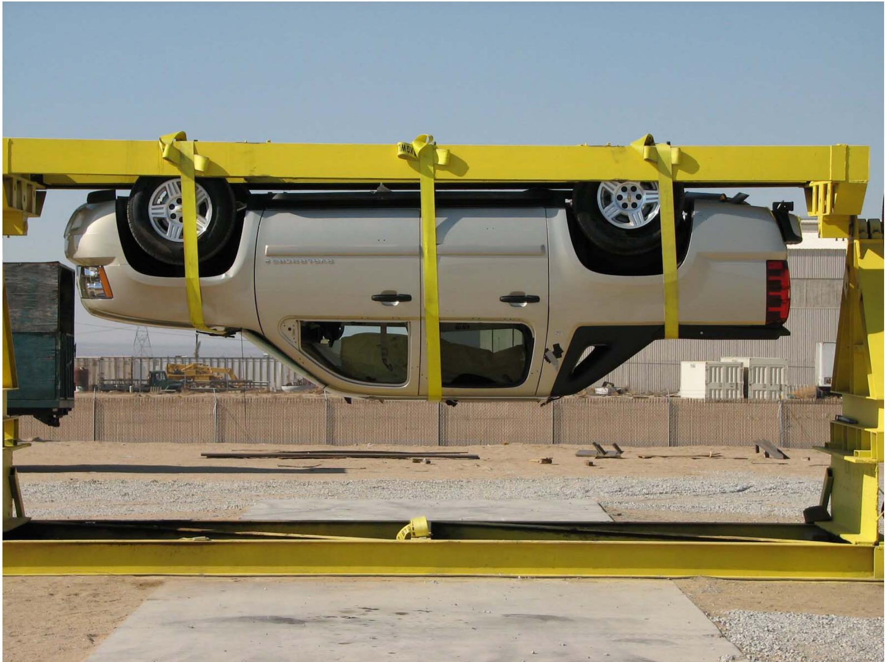
Figure A-63: Vehicle on Rollover Device (180°)
