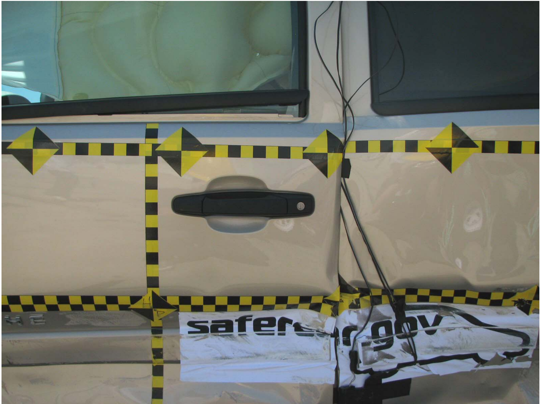
Figure A-32: Post-Test Left Front Door
