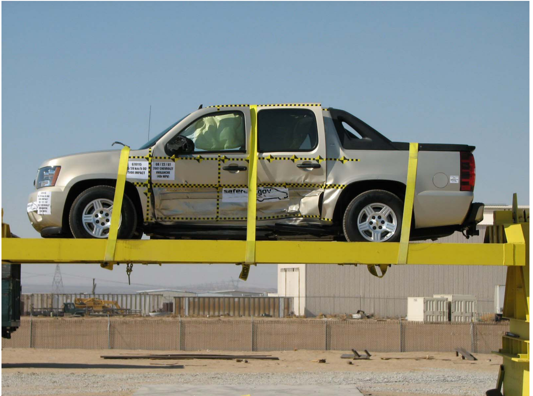
Figure A-61: Vehicle on Rollover Device (0°)
