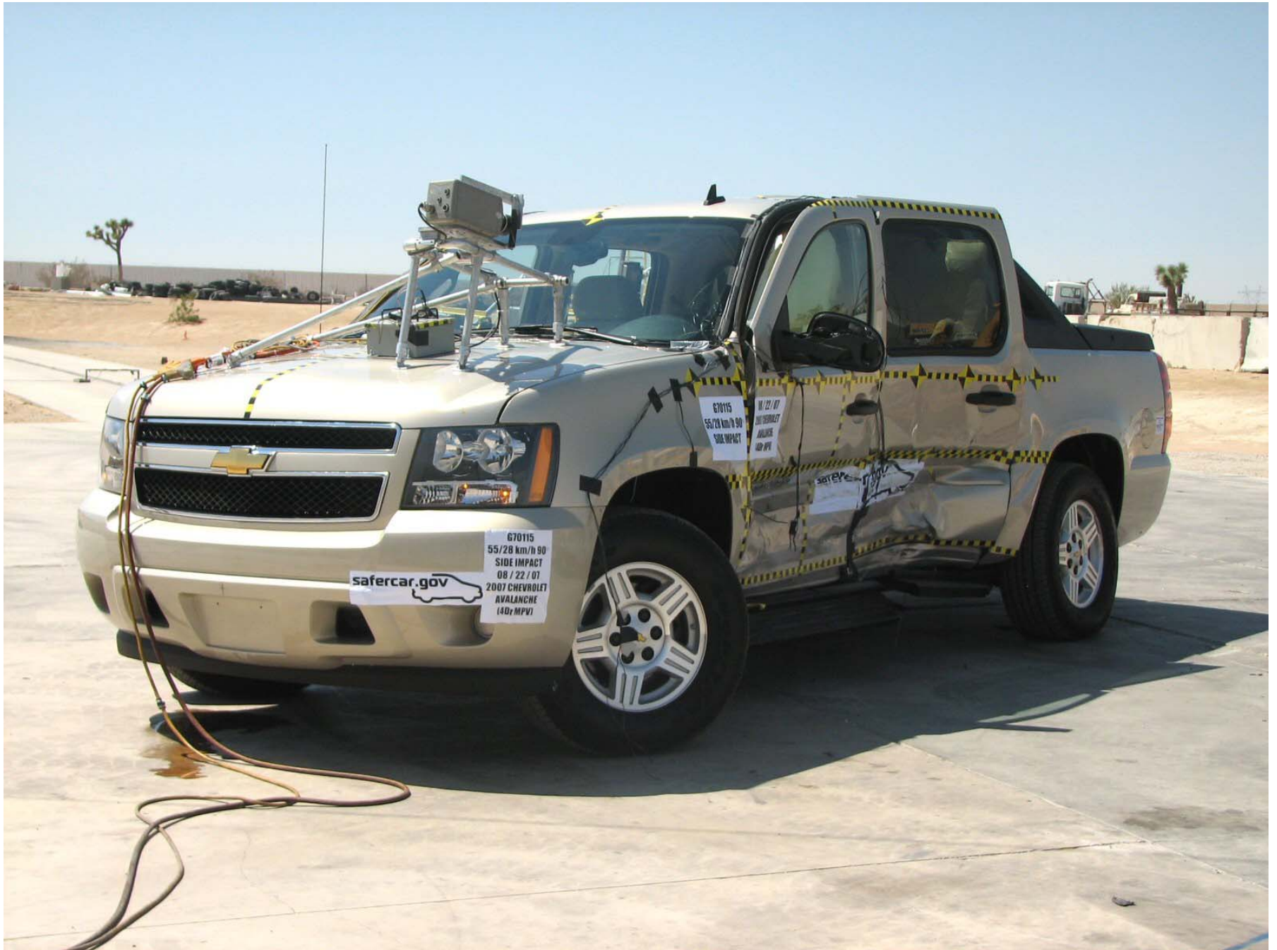
Figure A-8: Post-Test Left Front \frac{3}{4} View
