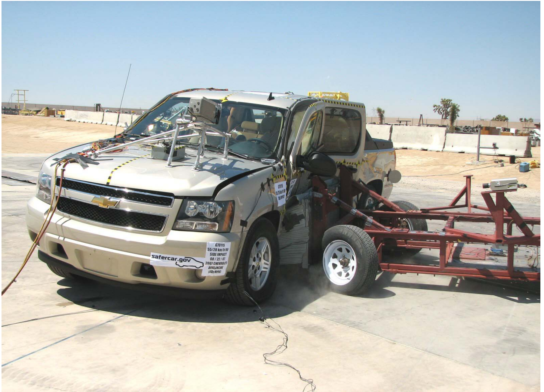
Figure A-65: Vehicle Impact
