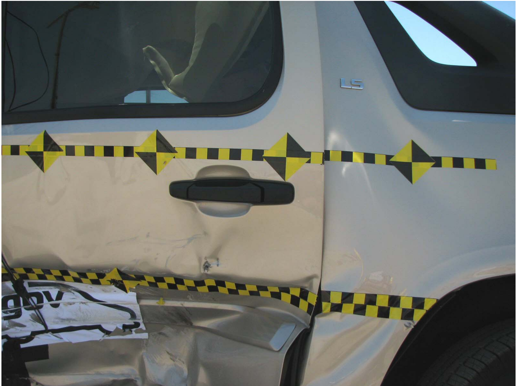
Figure A-34: Post-Test Left Rear Door
