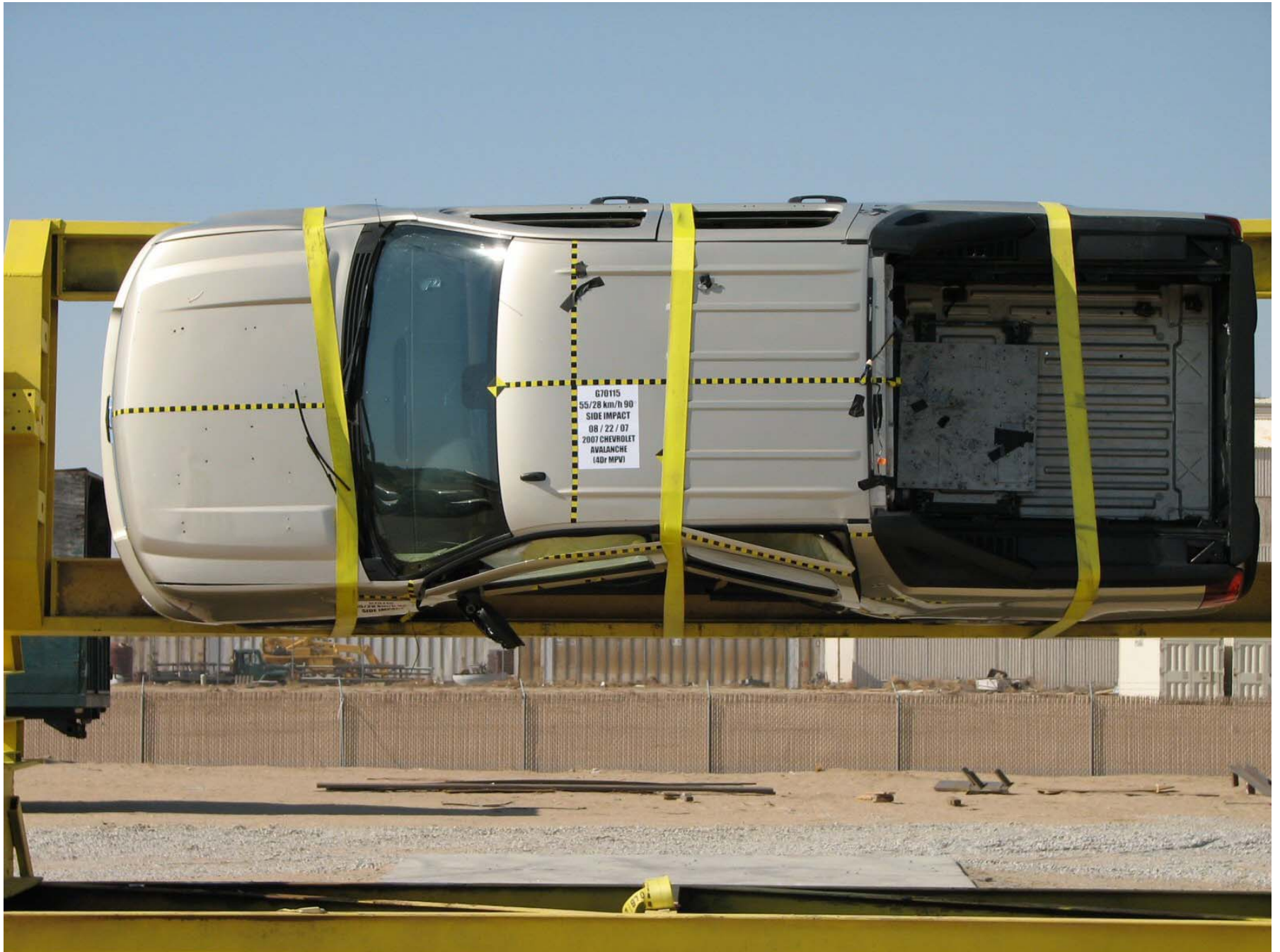
Figure A-62: Vehicle on Rollover Device (90°)
