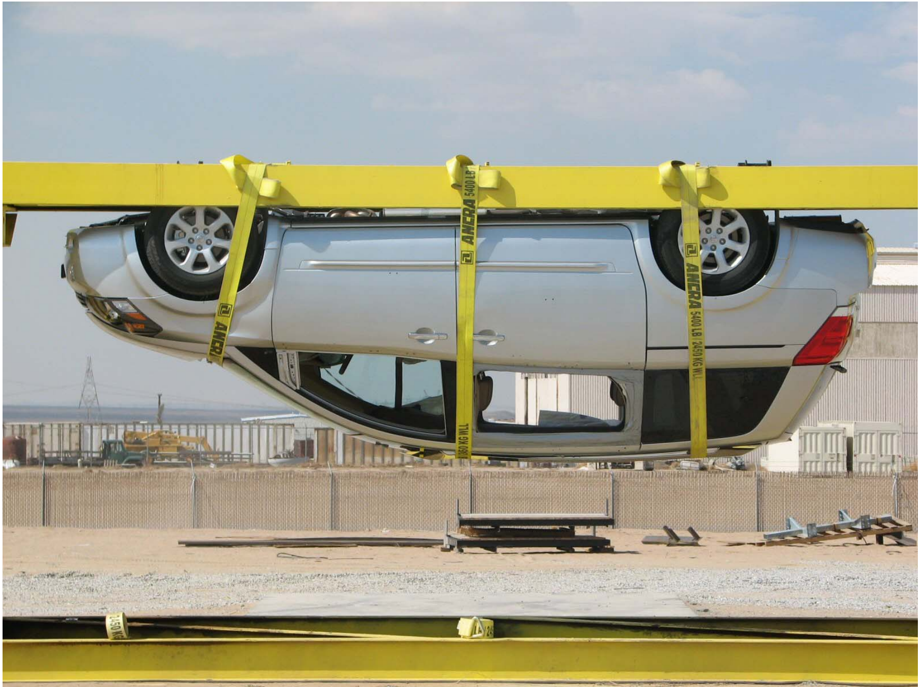
Figure A-63: Vehicle on Rollover Device (180°)
