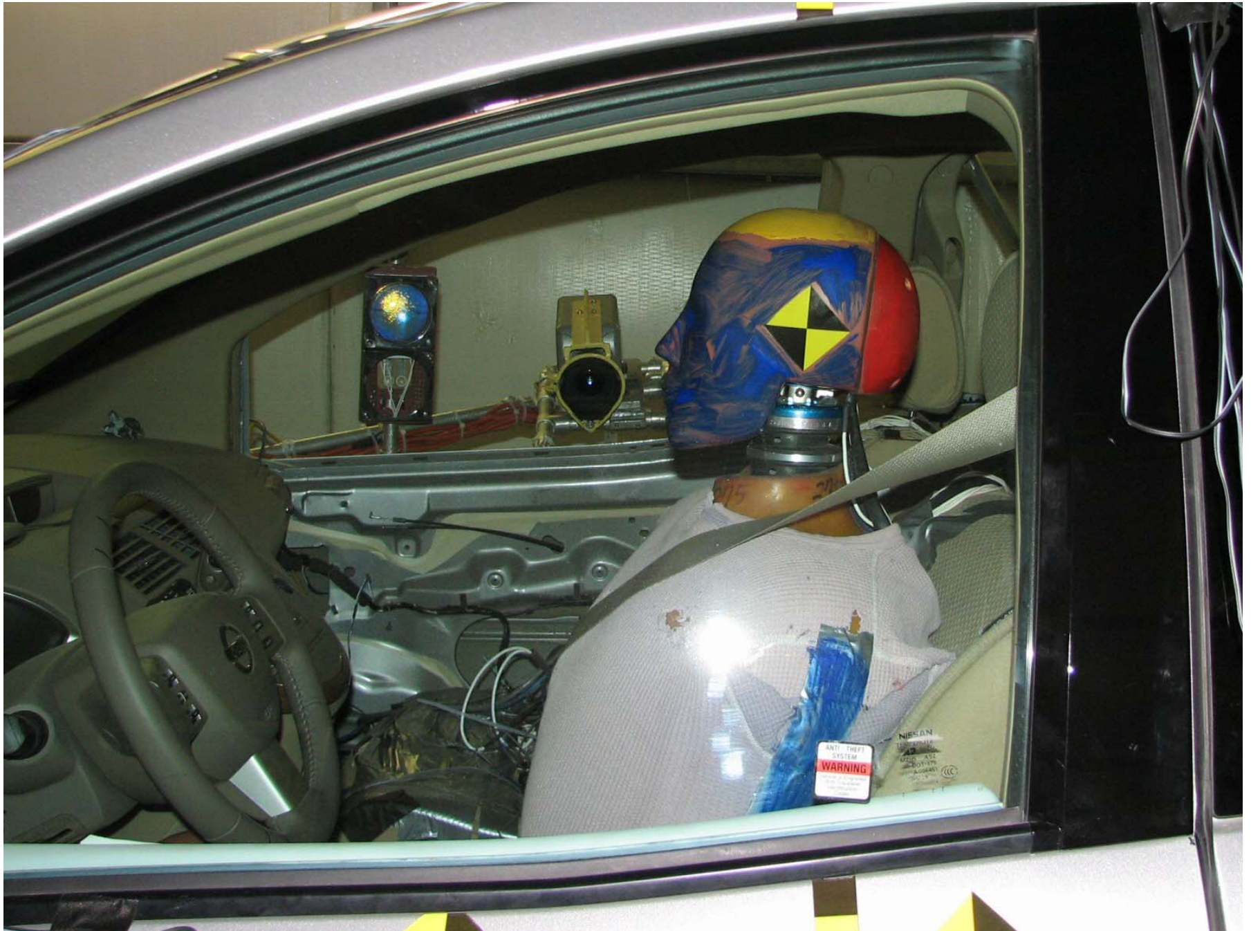
Figure A-36: Pre-Test Driver Dummy (Through Window)
