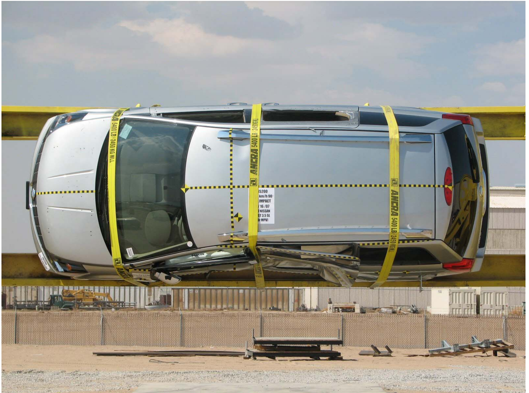
Figure A-62: Vehicle on Rollover Device (90°)
