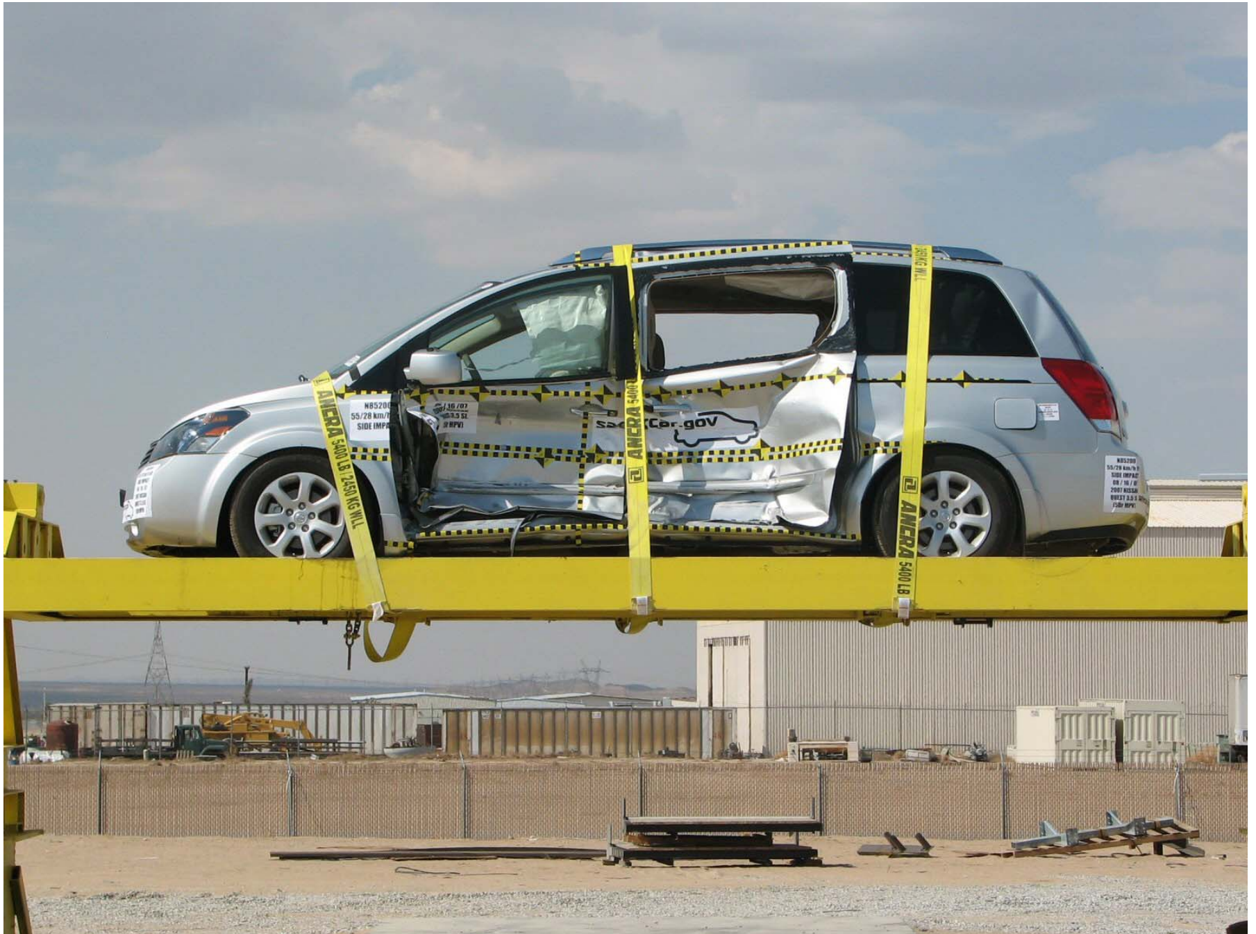
Figure A-61: Vehicle on Rollover Device (0°)
