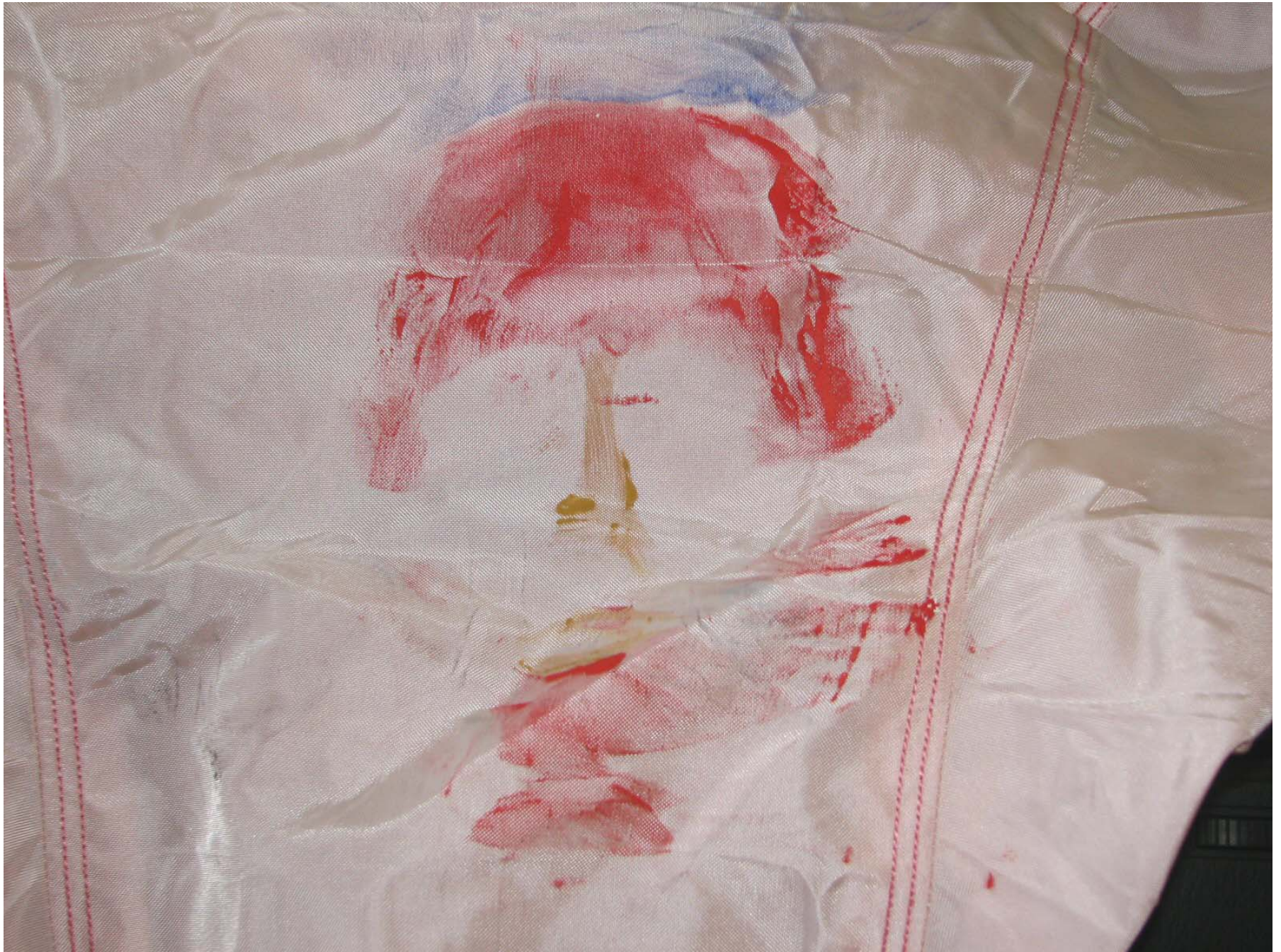
Figure A-57: Post-Test Passenger Dummy Airbag Contact
