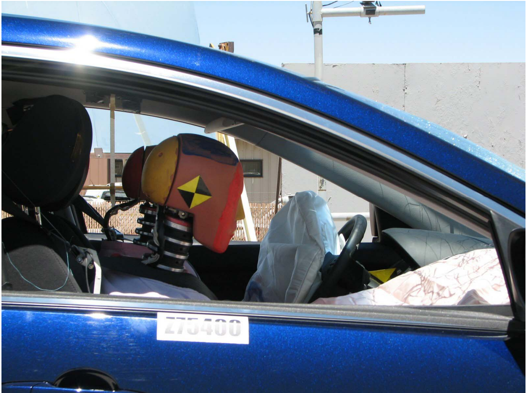
Figure A-47: Post-Test Passenger Dummy (Through Window)
