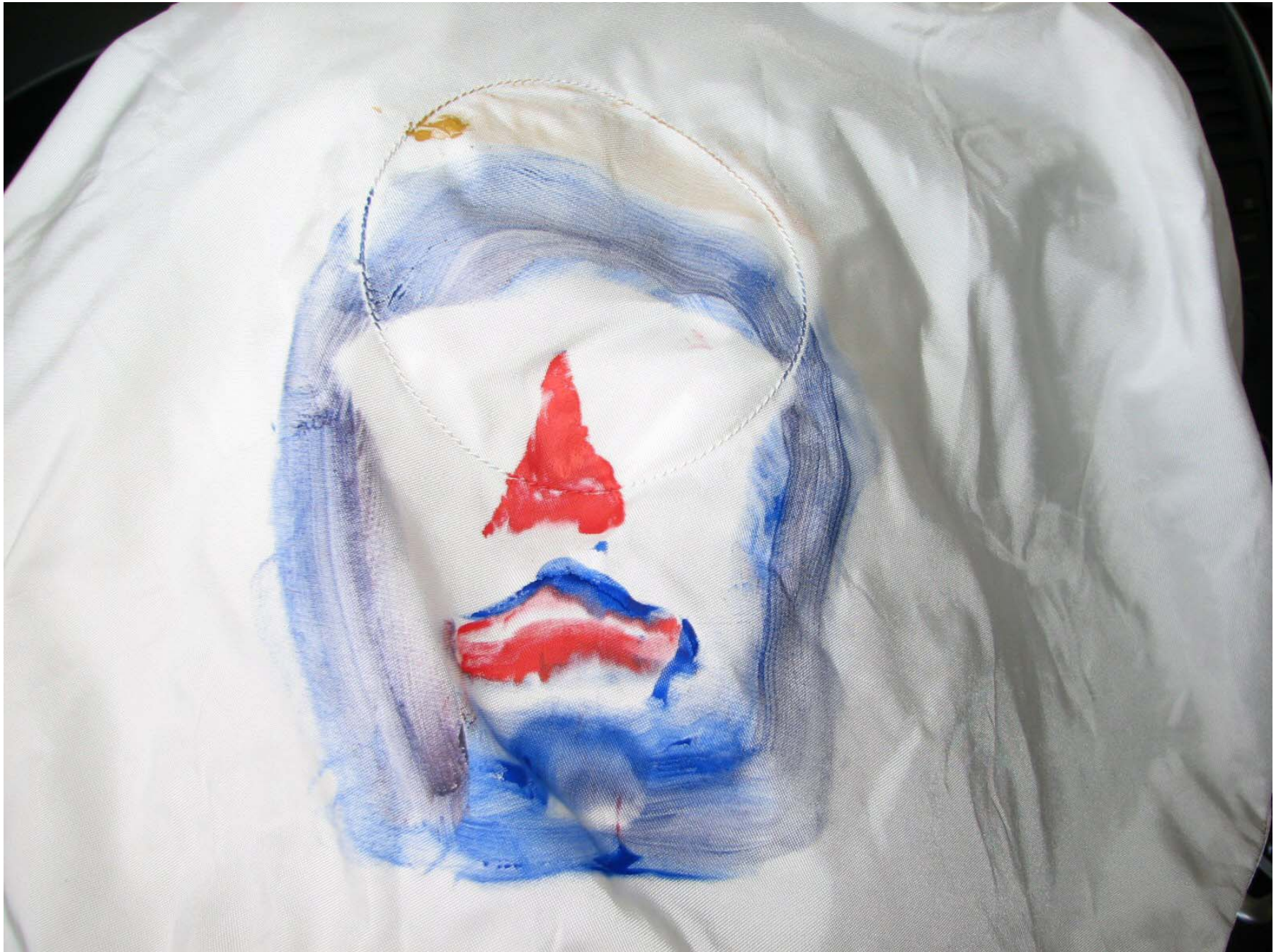
Figure A-43: Post-Test Driver Dummy Airbag Contact
