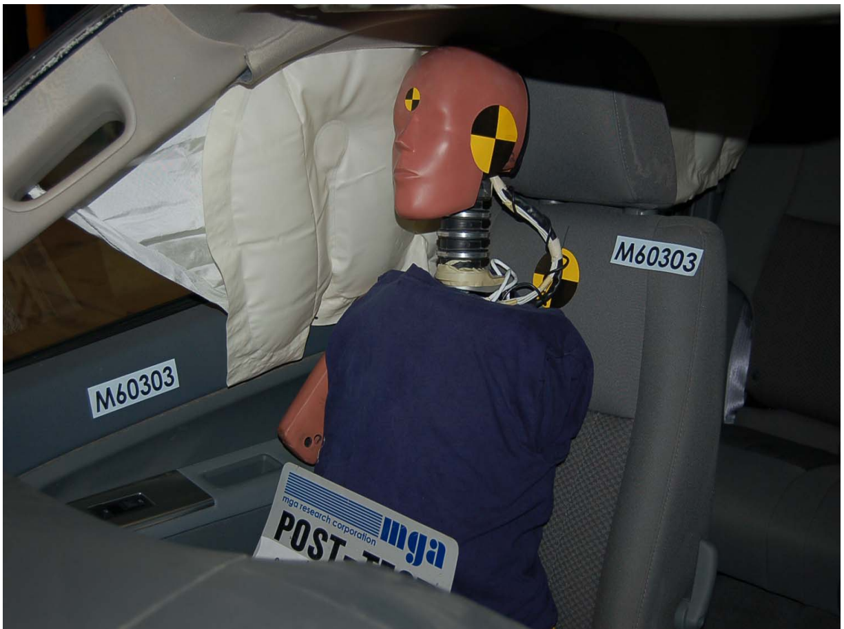
Post-Test SID-IIs Dummy Left Side \frac{3}{4} View
