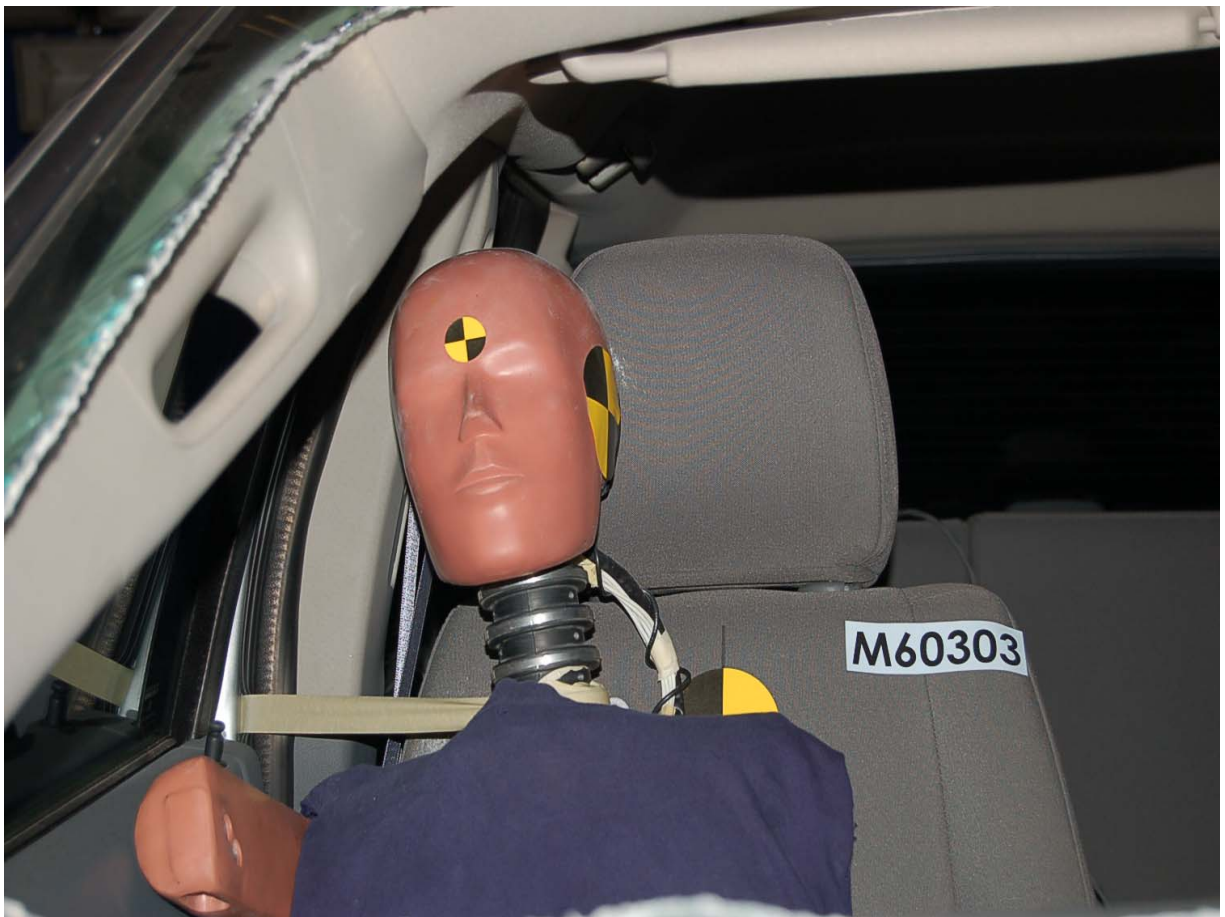
Pre-Test SID-IIs Dummy Front Head View
