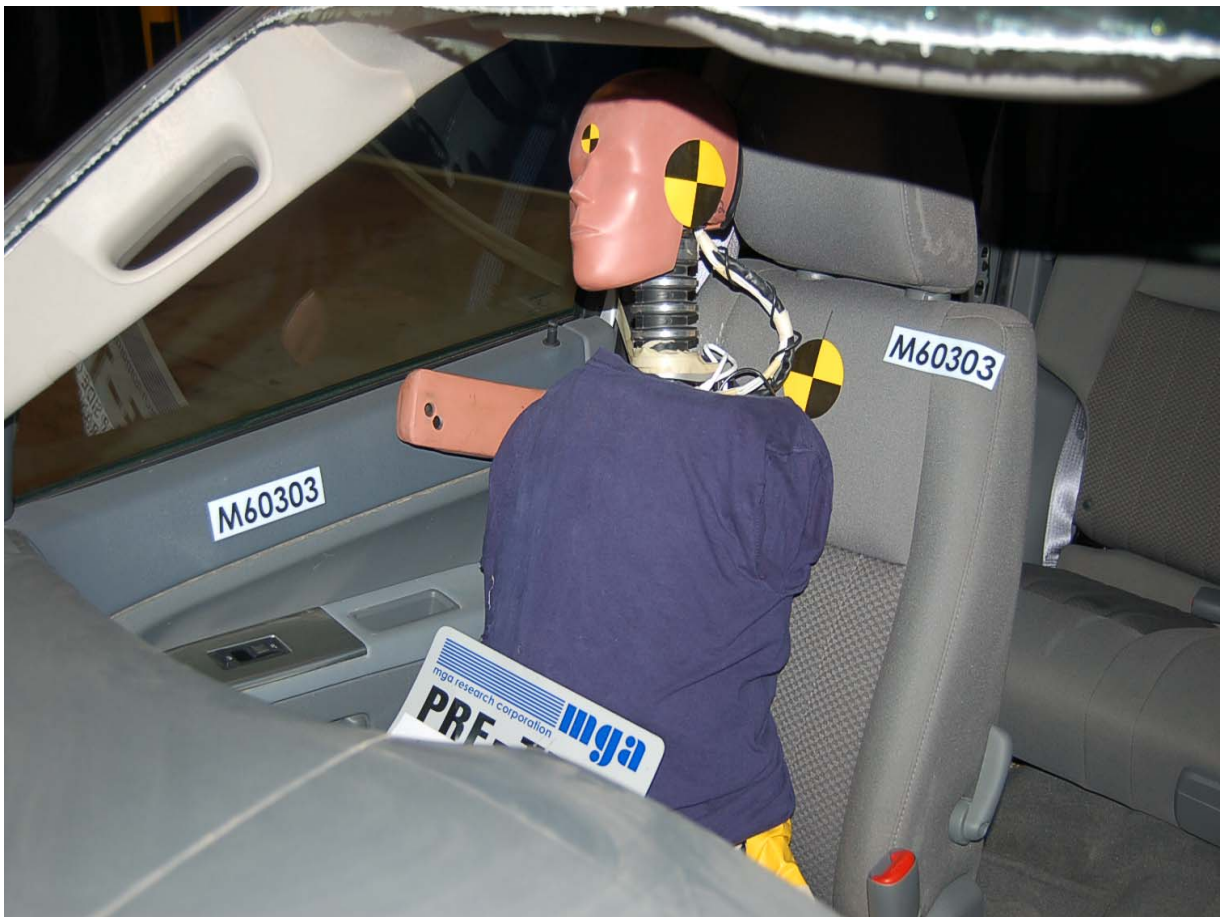
Pre-Test SID-IIs Dummy Left Side \frac{3}{4} View
