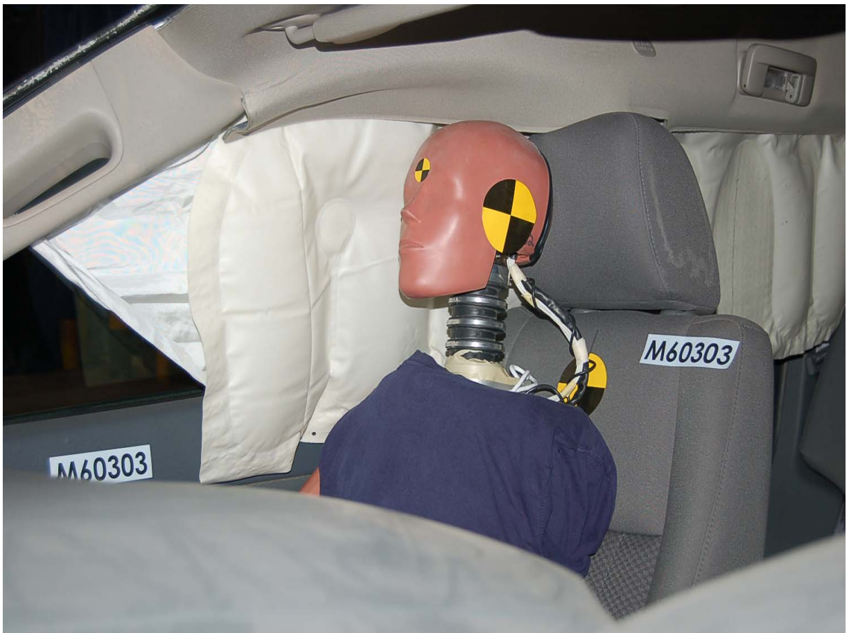
Post-Test SID-II's Dummy Left Side \frac{3}{4} Closeup View
