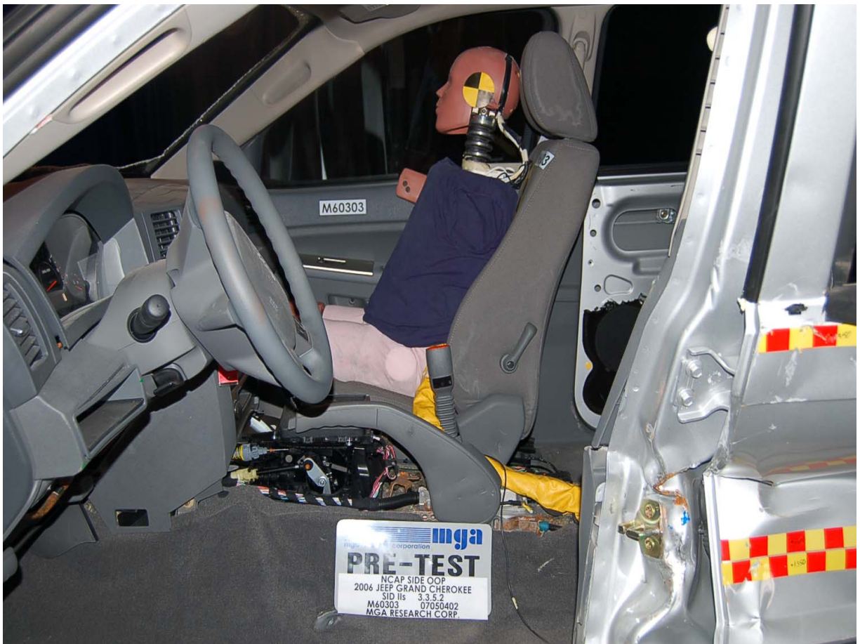
Pre-Test SID-IIs Dummy Left Side View
