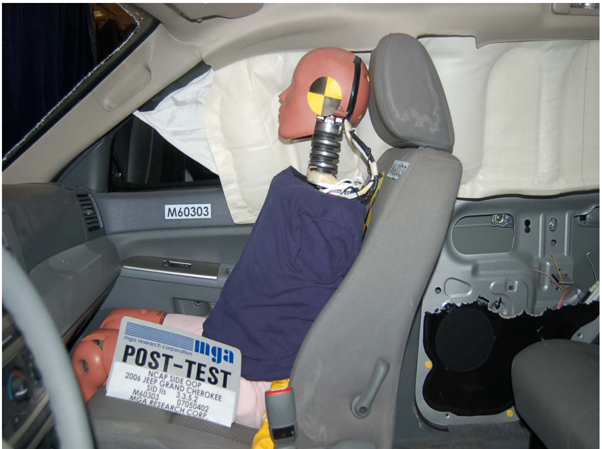
Post-Test SID-IIs Dummy Left Side Closeup View
