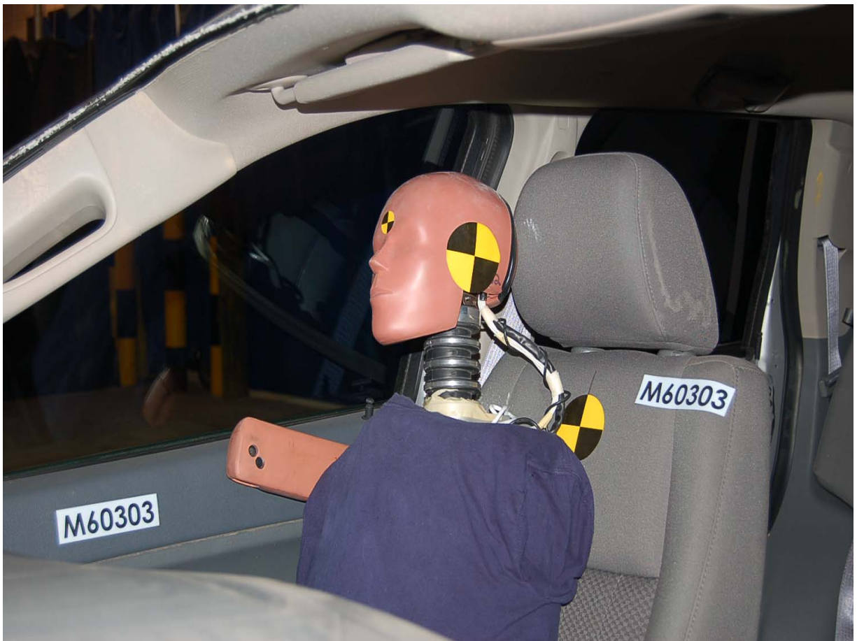
Pre-Test SID-II's Dummy Left Side \frac{3}{4} Closeup View
