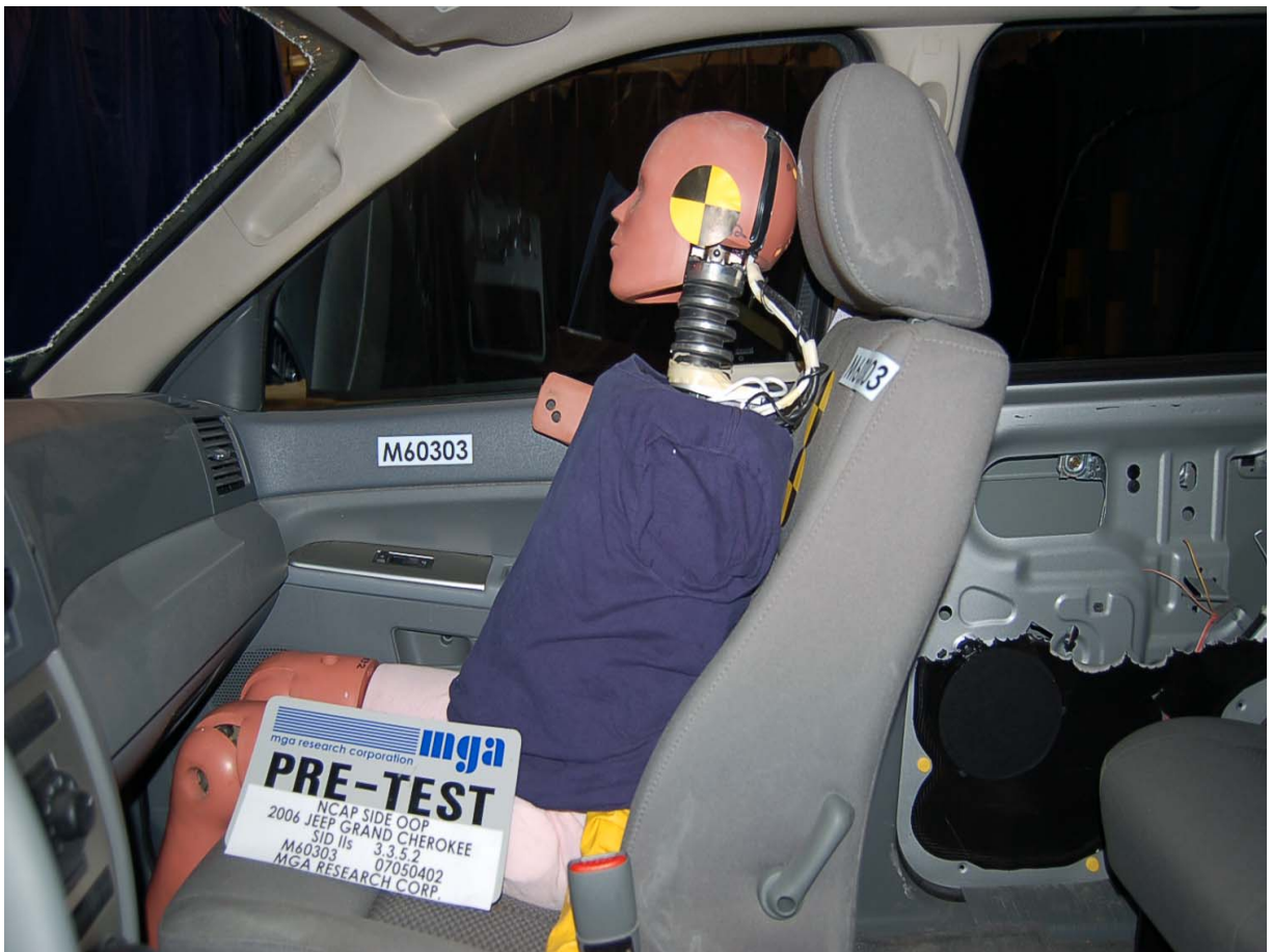
Pre-Test SID-IIs Dummy Left Side Closeup View
