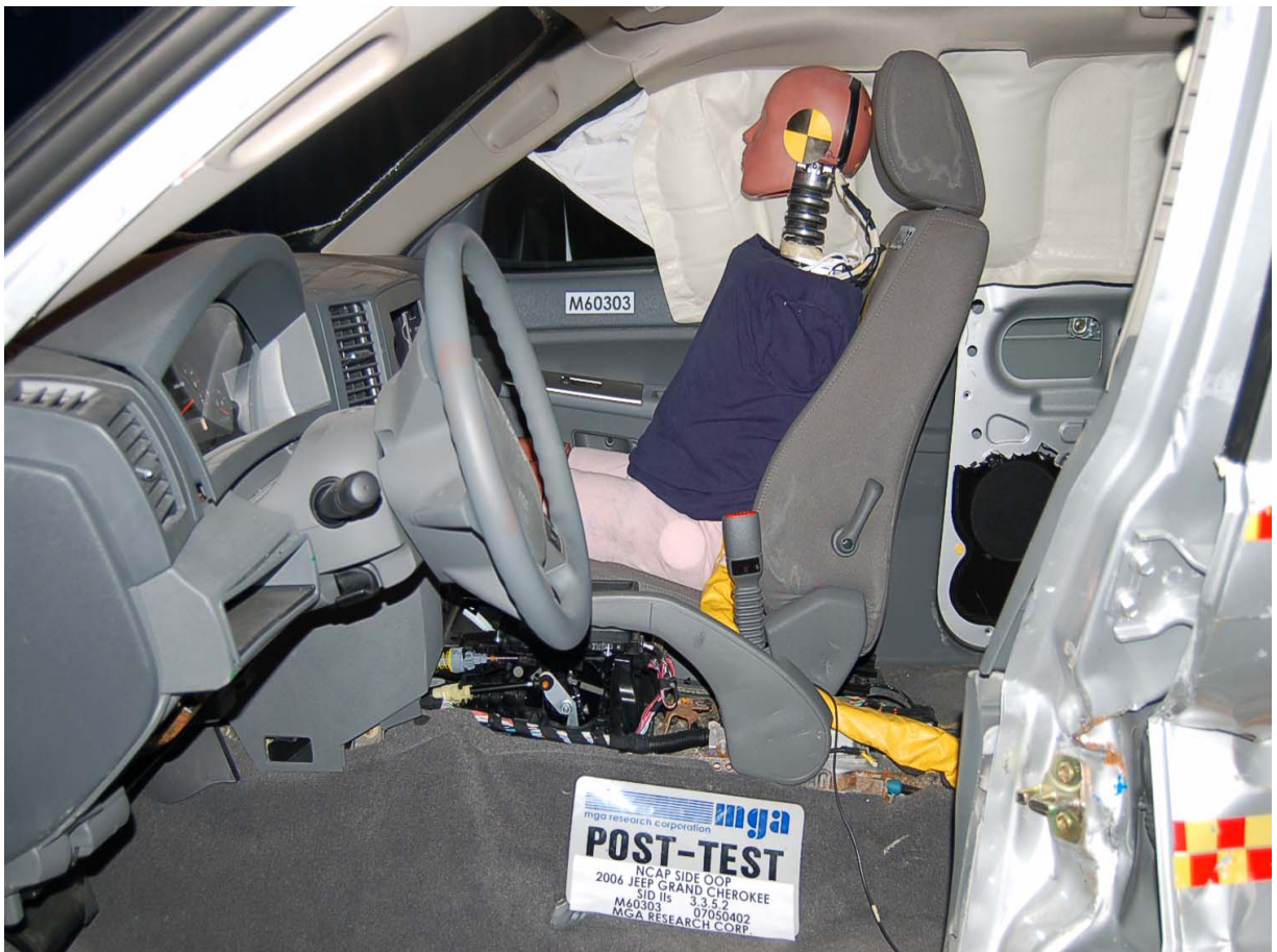
Post-Test SID-IIs Dummy Left Side View
