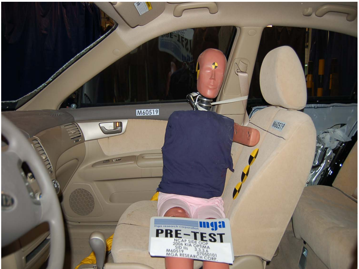
Pre-Test SID-IIs Dummy Frontal Closeup View
