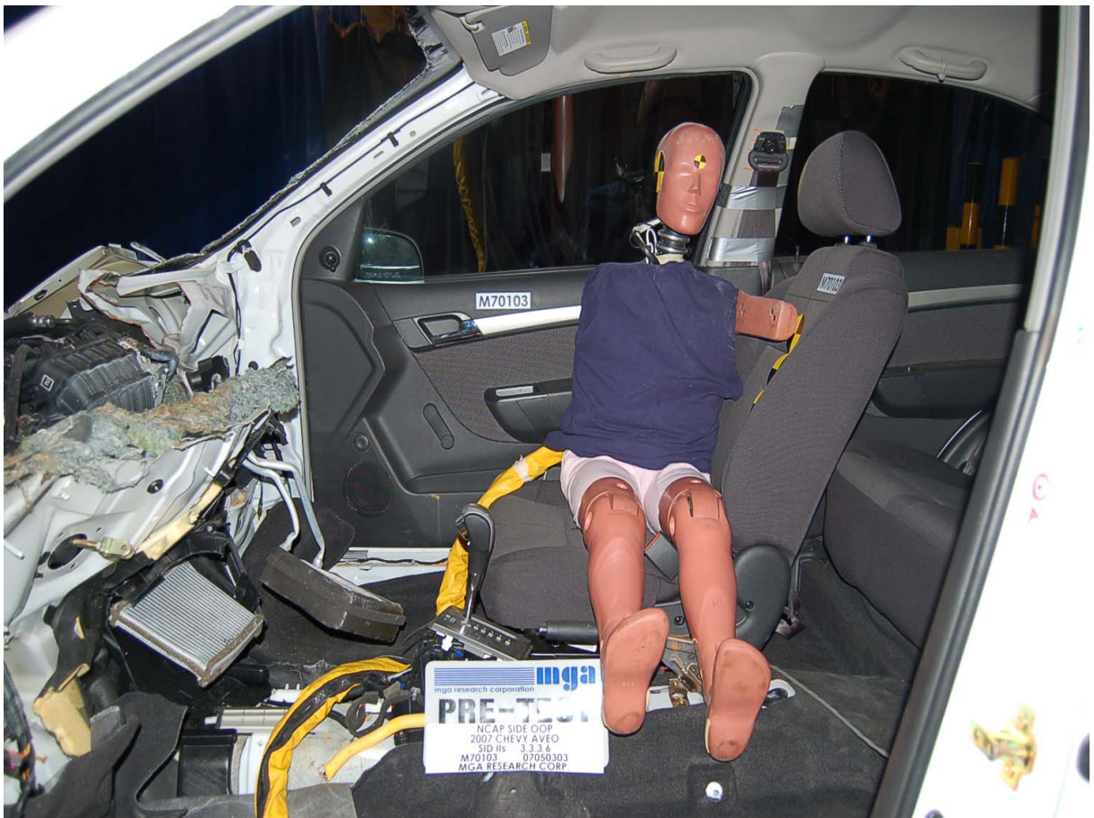
Pre-Test SID-III Dummy Frontal View
