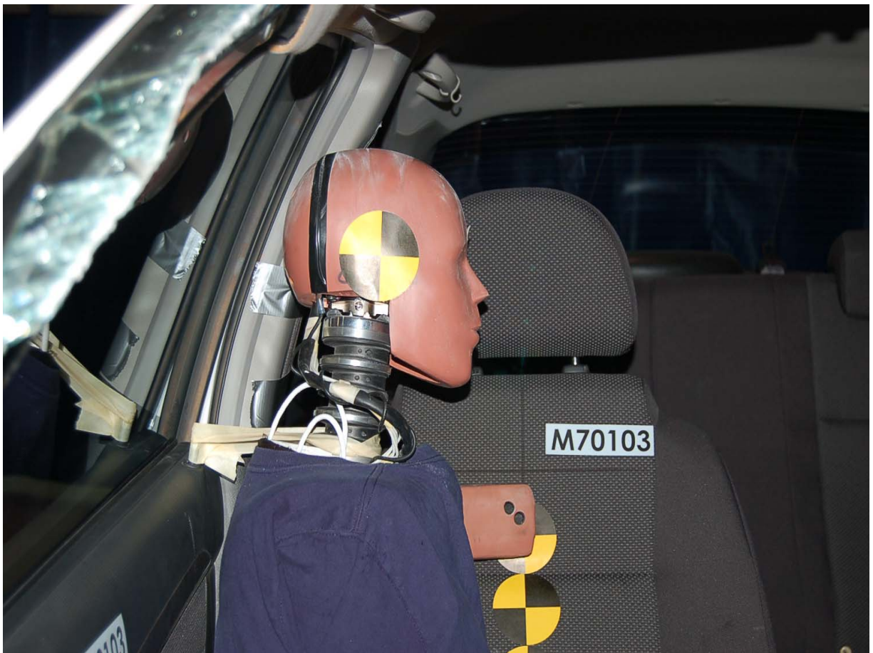
Pre-Test SID-IIs Dummy Right Side Head View
