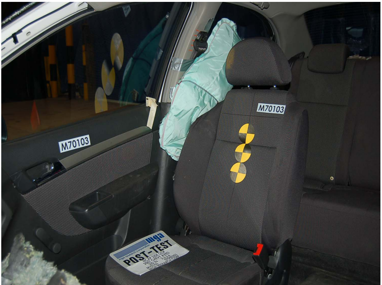
Post-Test Torso Airbag View
