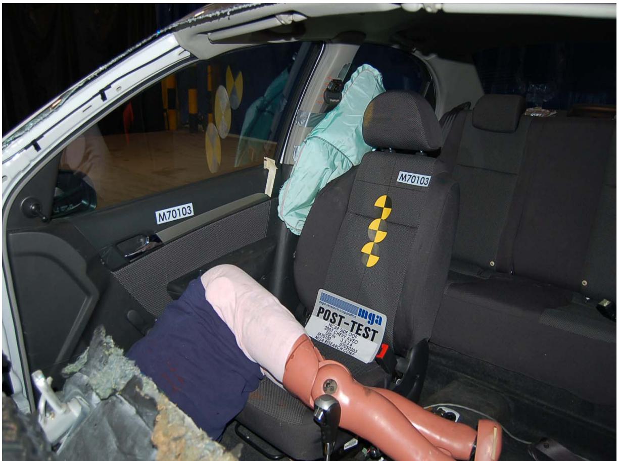
Post-Test SID-11s Dummy Right 3/4 Front View
