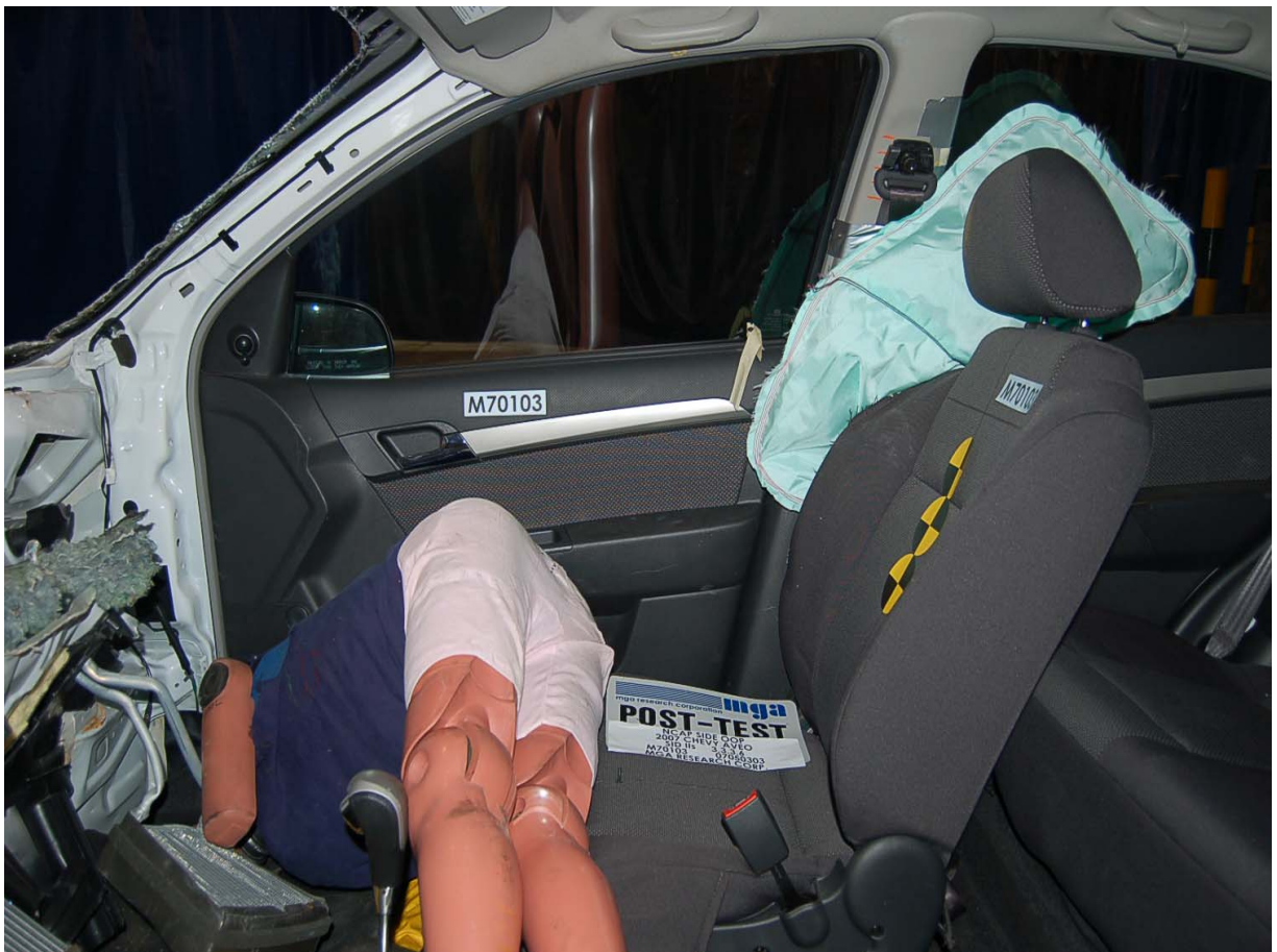
Post-Test SID-IIs Dummy Frontal Closeup View
